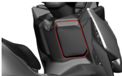
1. Open the right storage box cover shown in Figure 1. (For model 368M, when removing the side cover, first press the center of the expansion pin, then pull it outward from the side closest to the pin. For model 368D, simply pull open the inner cover as shown in the diagram.)
