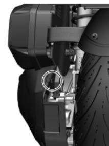
2. Remove the 2 expansion pins.
