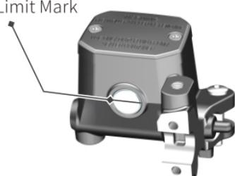
Front Disc Brake Master Cylinder
