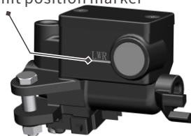
Front brake master cylinder
