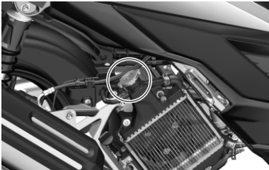
1. Coolant main tank cover
