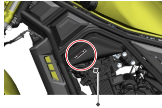
And the cover of the main water tank.
