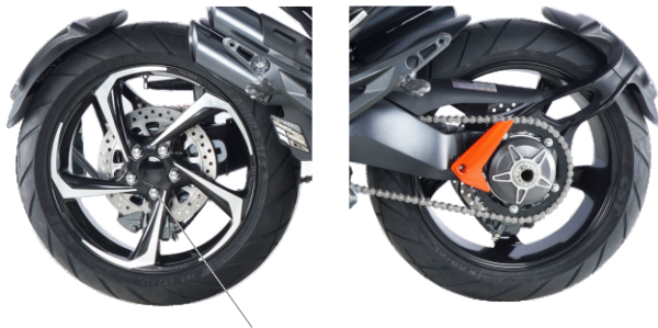
M12×1.5 nuts Rear wheel nut tightening torque: 110N.m
