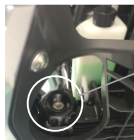
Water tank cover
