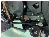
Engine oil drain bolt
