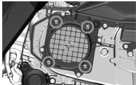
4. Remove 5 screws, remove the filter element of the engine air inlet and replace it with a new one.
