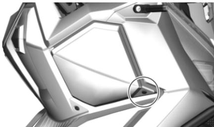
1. Remove the 1 expansion pin on the outer cover of the right front storage compartment and detach the cover.
