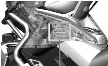
The starter relay is located under the head cover. Refer to the "Lithium-Ion Battery" section for instructions on removing the head cover to access it.
