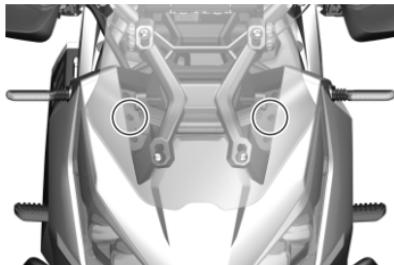
1. Remove the 2 expansion pins on the head cover and detach the front cover.
