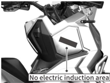
When the inductive key battery is low or there is no key battery, it can be powered on through the non-electric induction mode. The specific steps are as follows:
