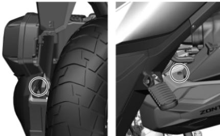
2. Remove the 2 expansion pins.
