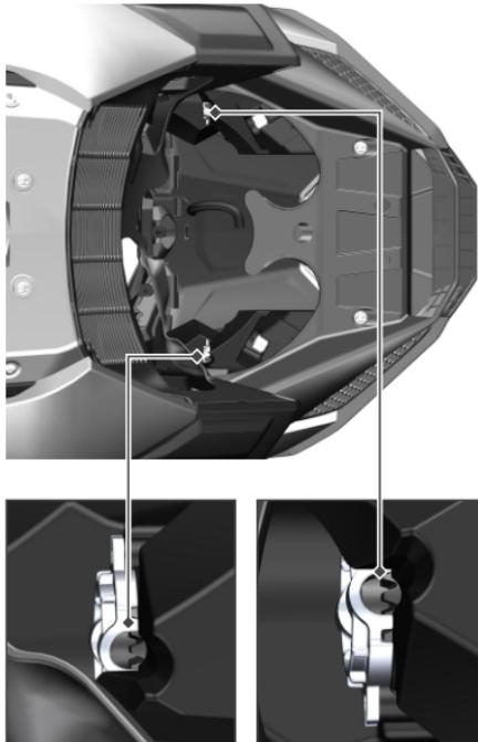
2. Use a  $6 \times 150-200$  mm cross-head screwdriver inserted into the adjustment hole.
