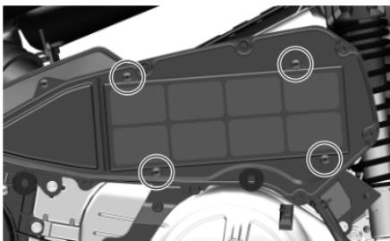
6. Remove the 4 screws and take out the filter element. Use a high-pressure air gun to blow away dust from the clean side of the element.
