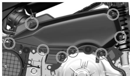
5. Remove the 10 screws in the figure above and remove the air filter cover.
