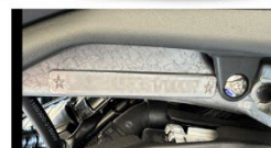
① Name plate ② muffler regulatory code ③ VIN
