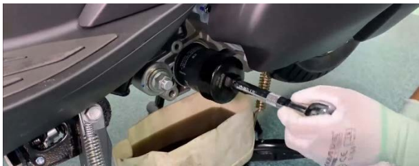
c. Drain the engine oil from the fine filter.
