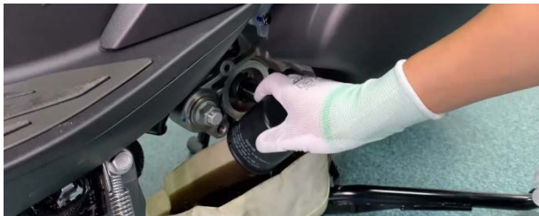
c. Drain the engine oil from the fine filter.
