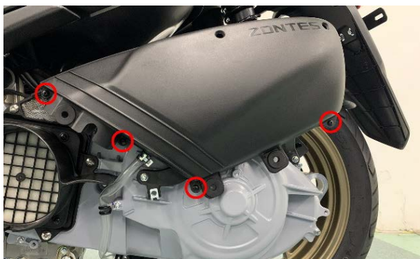
d. Remove the air filter housing.
