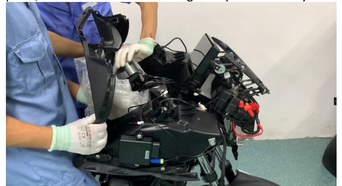
n. Pass the handle assembly through the front storage box panel, and remove the front storage box panel assembly.
