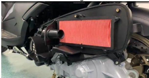
e. Place the rubber plug and tapping screw properly to avoid loss.
