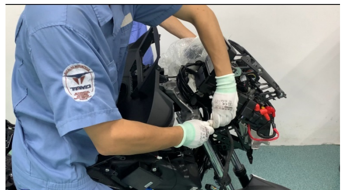
n. Pass the handle assembly through the front storage box panel, and remove the front storage box panel assembly.
