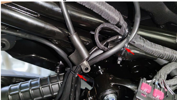
M125 loosen the rubber buckle and the wire clamp.
