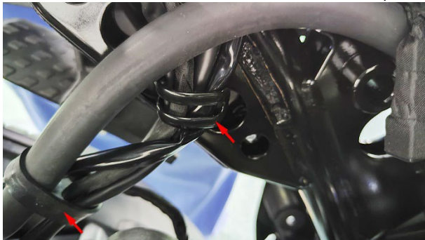
M125 loosen the rubber buckle and the wire clamp.
