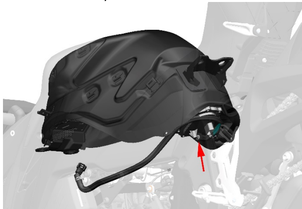
g. Lift the rear of the fuel tank by hand, disconnect the fuel pump connector, power off the vehicle and lock it. Press the anti-disengagement buckle in the direction of the arrow and then pull out the high-pressure fuel pipe, then remove the fuel tank assembly.
