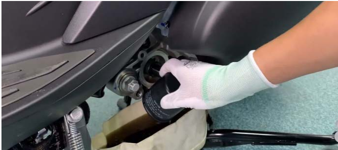
d. Use a clean non-woven cloth to wipe off the residual oil and impurities on the engine.
