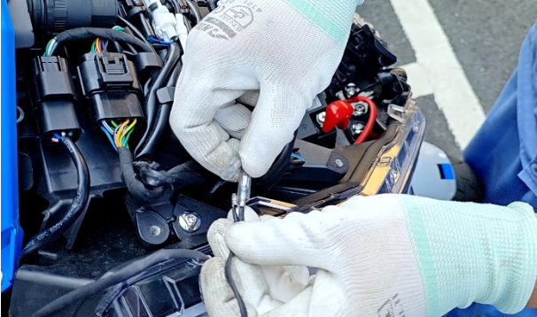
e . Remove the right side panel of the head. The removal method of the left side panel of the head refers to the removal of the right side panel.
