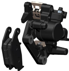
b. Remove the brake pads from the caliper.
