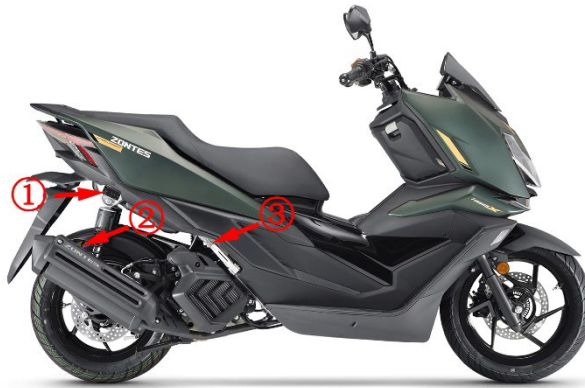
① Name plate ② muffler regulatory code ③ VIN
