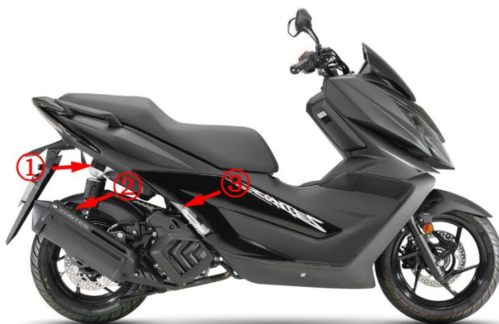
① Name plate ② muffler regulatory code ③ VIN
