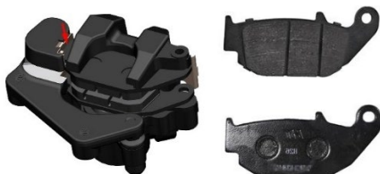
e. Use 5 #inner hexagon to lock the anti-loosening plug.
