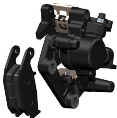
b. Remove the brake pads from the caliper.
