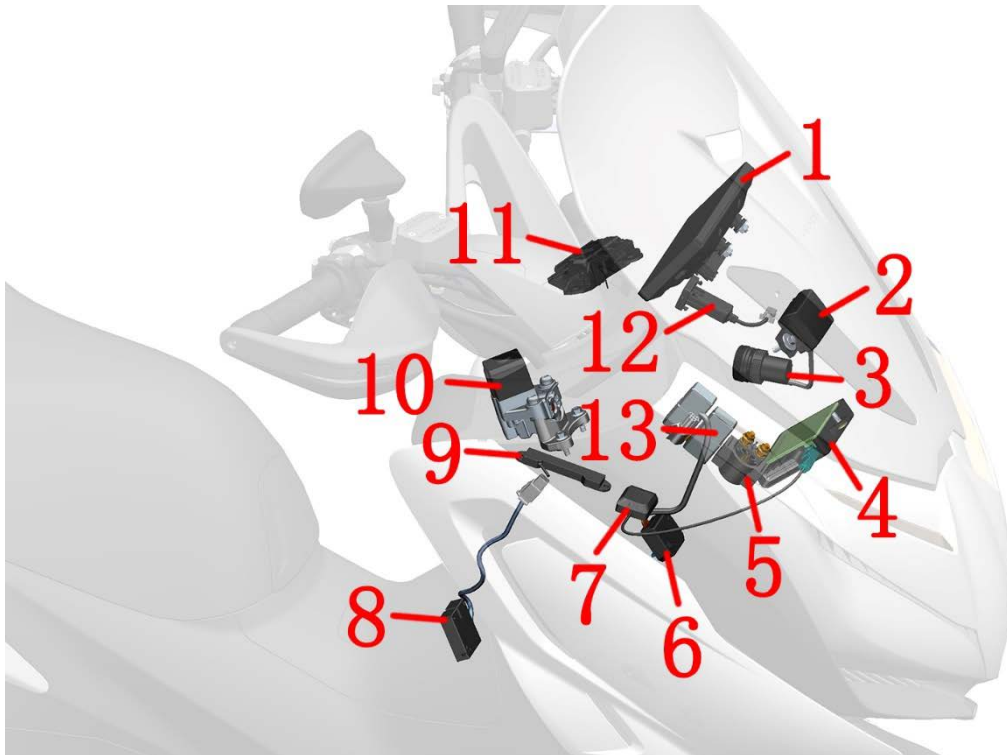
1- TFT instrument 2-Windshield motor controller 3-Dual Port Universal USB Charging Cable 4-PKE 5-Starting relay 6-Charging port 7-GPS antenna 8-Electronic fuel tank lock 9-Non-inductive antenna 10-Main lock 11-Left front luggage box lock 12-Single port universal USB charging cable 13-EFI Relay
