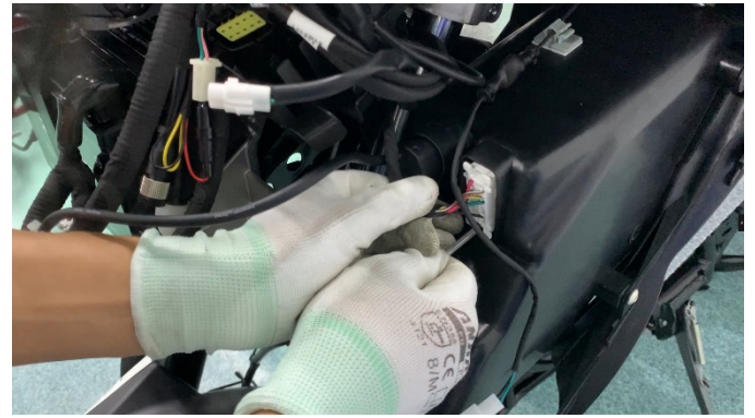
j. Use 4# inner hexagon to remove 2 M6×14 bolts (2), use 6# inner hexagon to remove 2 M6×25 bolts (1) to fix the main lock, and pull out the main lock connector.
