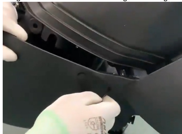
d. Use 4# inner hexagon to install the other 4 M6×14 bolts. Replace the decorative buckle.
