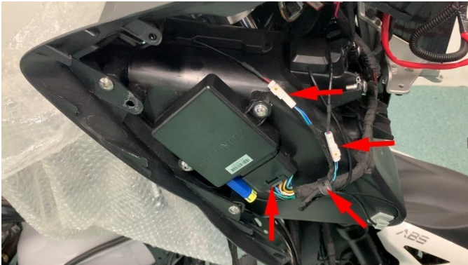
i. Open the buckle and remove the OBD diagnostic connector
