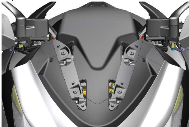
Removal of the upper part of the hood and the windshield liner
