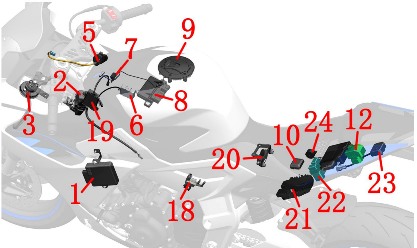
1-LCM Lighting Controller 2-Faucet Lock 3-Horn 4-Cable Assembly (shown in yellow) 5-Dual-port universal USB charging cable 6-Tire pressure receiver 7-Electronic fuel tank lock substrate 8-Engine controller (ECU) 9-Electronic fuel tank lock 10- GPS antenna 11- PKE external antenna 12-Starting relay 13-Cushion lock 14-Third generation PKE host 15-Non-electric induction antenna 16-Lithium battery 17-Side kill switch 18-Carbon canister solenoid valve 19-Frame grid atmosphere light driver 20-Tilt switch 21-Rectifier 22-Relay 23-Charging port holder 24-Buzzer
