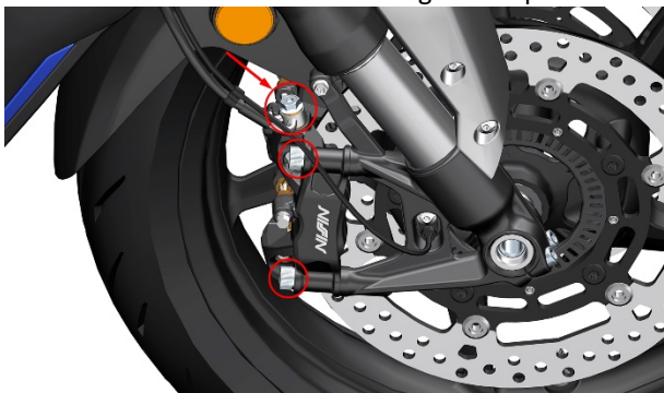
b. Front disc brake caliper disassembly
