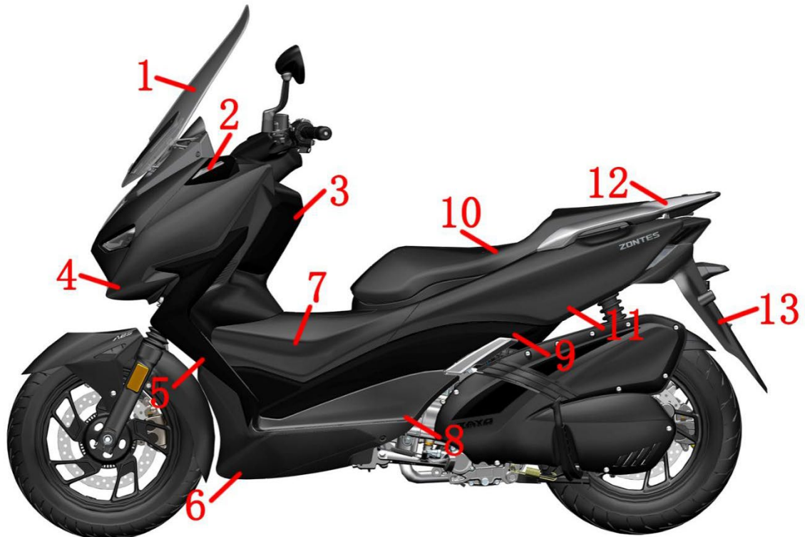
1. Windshield 2.Left front turn light 3. Left cover front storage box 4. Front left panel 5. Front storage box panel left decorative cover 6. Left pedal decorative cover 7.Left fuel tank cover plate 8. Left pedal 9. Left side cover 10. Cushion 11. Tail skirt left part 12. Rear rack 13. Rear mudguard
