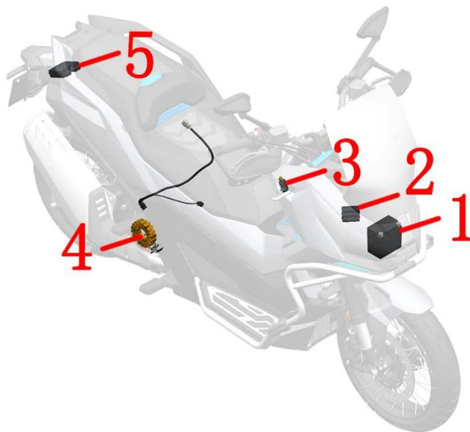
1-Battery 2-Main fuse ( 25A ) 3-Charging port ( PKE ) 4 - Magneto 5 – Rectifier
