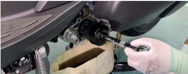
c. Drain the engine oil from the fine filter.
