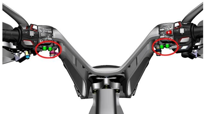
d. Wrap the handle assembly with a bubble bag to prevent the cover from being scratched. Use a one-word batch to cover the non-woven fabric, and remove the upper cover in the direction.
