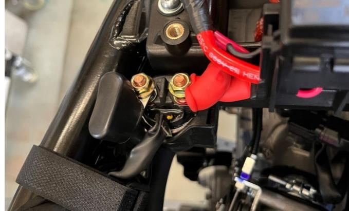
When reinstalling, the yellow/red and green/red wires of the relay correspond to the color of the main cable, and the nuts are not distinguished. Be sure to close the protective cap after tightening the nut.
