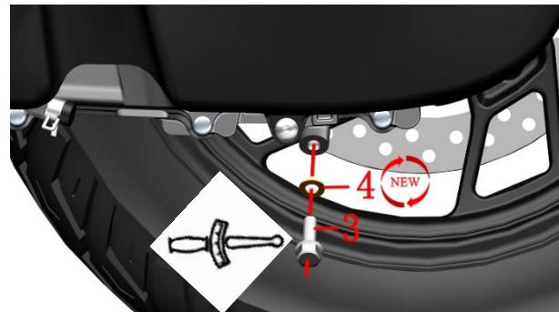
c. Use a #10 socket for the ETC model, and a #14 socket for other models to remove the M8x25 drain bolt (3) and the 8.3x16x1.5 copper washer (4).
