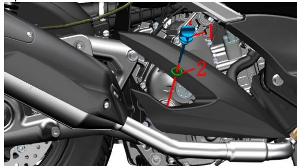
e. Apply a layer of oil to the new fine filter seal and install it on the engine. Torque: 20 N.m (2 kgf.m, 15 lbf.ft).
