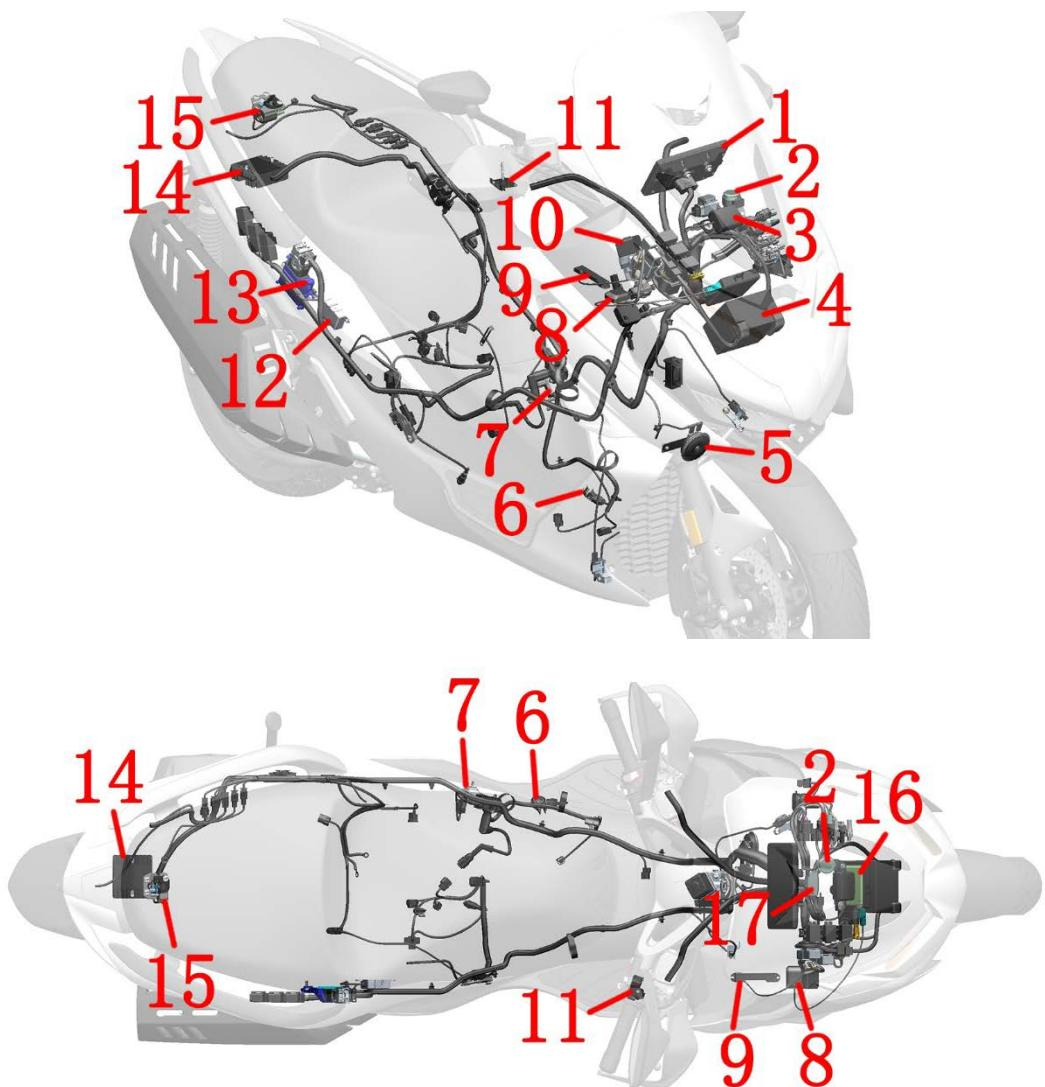
1-TFT instrument 2-Flasher 3-Windshield motor controller 4-Battery 5-Horn 6-Side bracket flame-out switch
