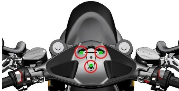
f. Pull out the cable fixed on the steering handle. Remove the steering handle.
