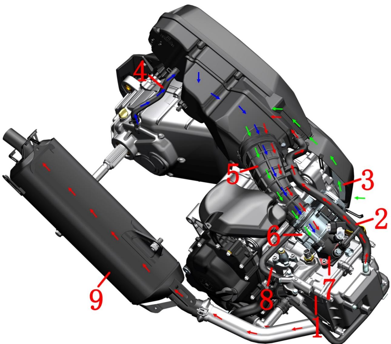
1- Cylinder head 2-Cylinder head exhaust pipe3- Air filter intake inlet 4-Crankshaft Box exhaust pipe5-Air filter outlet pipe6- Throttle valve body assembly 7-Intake manifold8- Cylinder 9- Muffler
