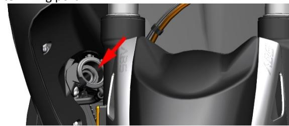
d. Tighten the filler cap of the Radiator. Tighten the exhaust bolt; torque: 8~10N.m (0.8~1 kgf.m, 6~7 lbf.ft).
