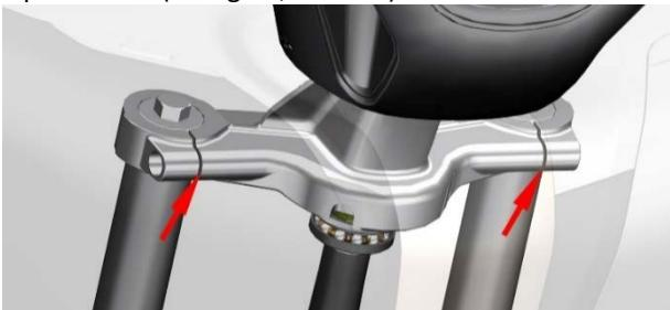
c. Install the bolts (6) of the two M8×35 lower plates and use the same method to load another shock absorber.
