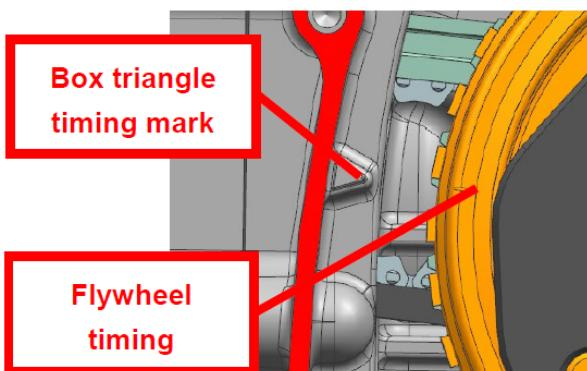
The triangle is aligned with the flywheel timing mark
