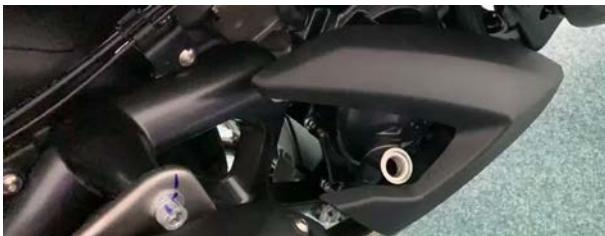
d. Use a clean non-woven fabric to wipe off the remaining oil and impurities on the engine. The O-ring used for the oil dipstick is sized 18x3x3.5.
