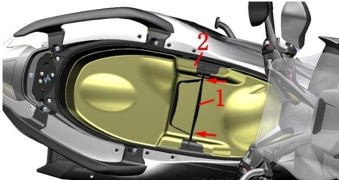
b. Old model: Use 4# inner hexagon to remove the 4 shoulder bolts at the rear and the middle (1), remove the front hexagonal bolt decorative buckle (2) and then remove the bolts (1).
