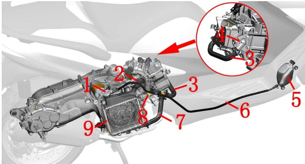
1- water tank water inlet 2-main water tank inlet pipe 3-engine inlet pipe 4-Water pump cover inlet pipe
