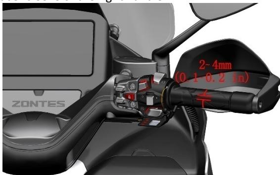
d. After starting the engine, turn the steering handle left and right to ensure that the idling speed does not change during the steering process, and then turn off the engine.
