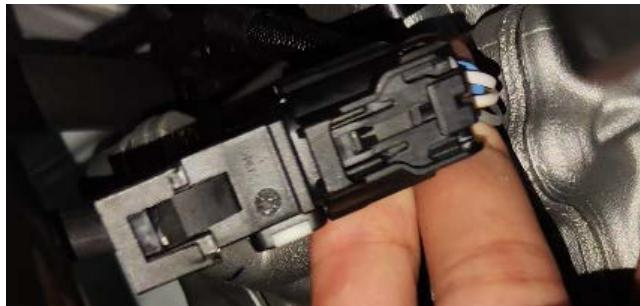
Use a multimeter to measure the resistance of the heating element of the two wires to  $9\pm2k\Omega$ ; E350 model can measure the current should be less than or equal to 2.1A. Otherwise, it can be judged that the oxygen sensor is faulty. The ceramic inside the oxygen sensor is hard and brittle. It is forbidden to knock with hard objects or blow with strong gas, otherwise it is easy to cause damage.
