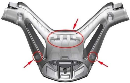
f. Replace the left and right expansion nails. Use the 4# Allen to replace the 2 bolts on the left and right sides. (Check whether the direction is crimped)
