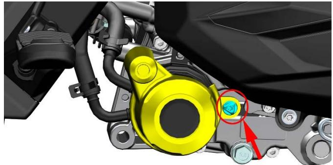
b.Place an oil pan under the fine filter cover.Remove the fine filter using a 14-side, 65mm cap filter wrench +1/2" (12.5mm) ratchet wrench counterclockwise. The filter wrench has a Skadden model 97401. Replacement every 1,000 km or 3 months (whichever comes first) and every 8,000 km or 30 months (whichever comes first).
