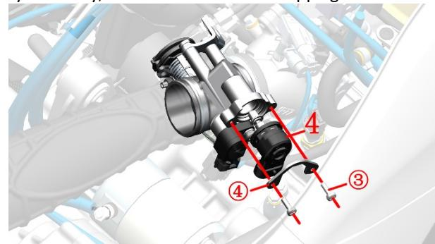
f. Use throttle cleaner to clean the carbon deposits on the head of the stepper motor. Spray a small amount of cleaning agent into the valve body hole. It is forbidden to soak the stepper motor with any liquid.
