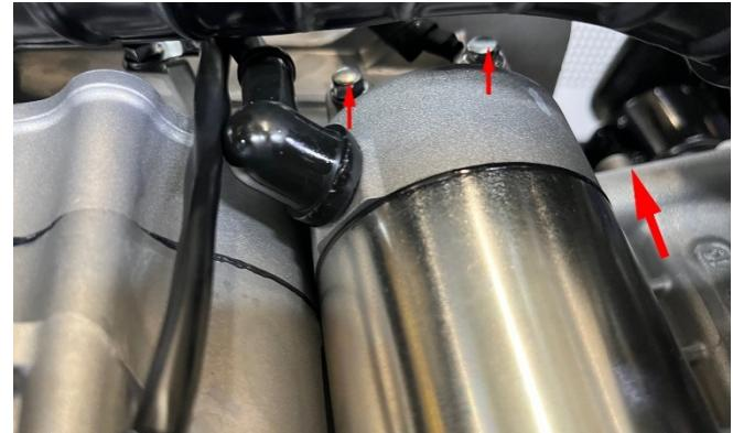
e. When reassembling, make sure not to omit the O ring that comes with the starter motor, and align the teeth of the electric starter reduction gear. Note that the O-ring needs to be correctly assembled into the box, as it will cause leakage if cut edges occur. Torque of the two bolts for fixing the starter motor:  $12\pm 1.5\text{ N.m}$  ( $1.2\pm 0.2\text{ kgf.m}$ ,  $9\pm 1\text{ lbf.ft}$ ). And mark with a marker.
