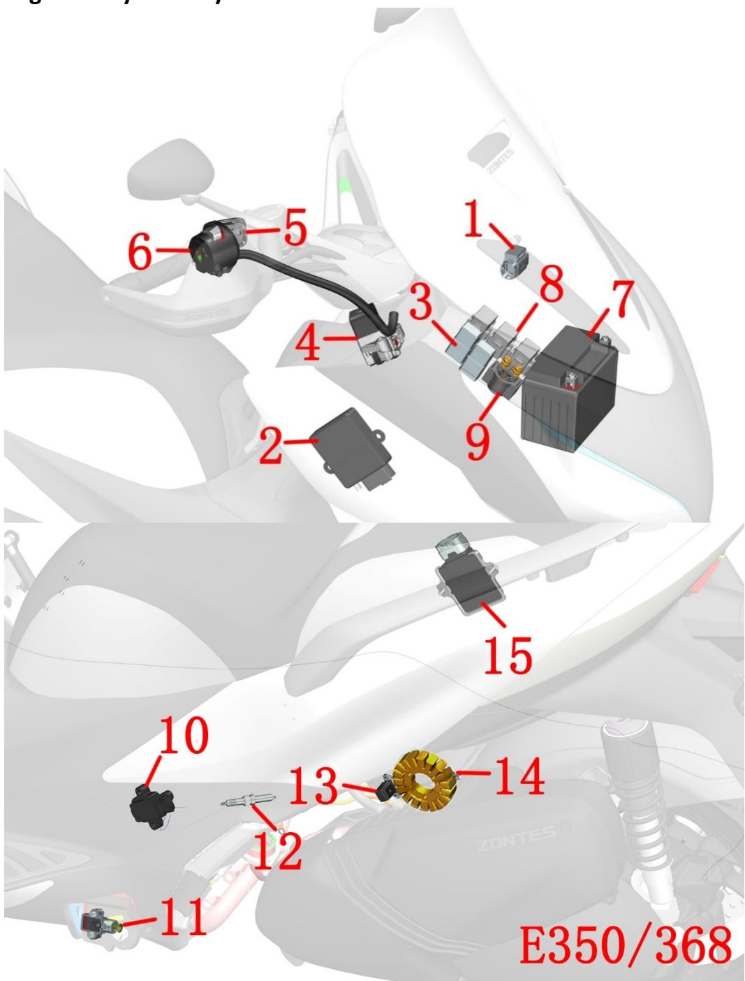
1 - Dump switch 2 - PKE 3 - relay 4 - main lock 5 - right handle bar auxiliary switch 6 - right handle bar switch 7 - battery
