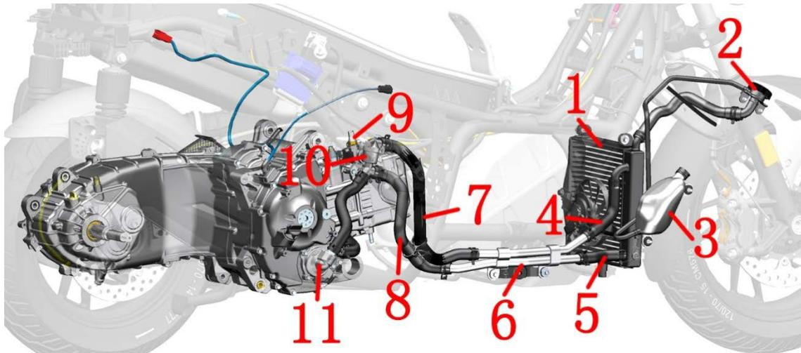
1-Main water tank 2-Water tank filling port 3-Auxiliary water tank 4-Main water tank inlet pipe 5-Main water tank outlet pipe 6-Aluminum water pipe 7-Thermostat outlet pipe 8-Engine inlet pipe 9-Water and oil common sensor 10-Thermostat 11-Water pump cover assembly
