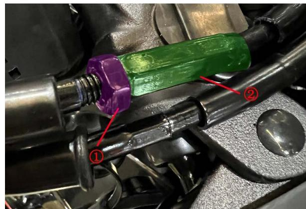
b. If the above adjustment fails to achieve the desired effect, please refer to the description in "Remove the throttle valve body assembly to clean up carbon deposits" to remove the throttle valve body assembly. Use a 10# open-end wrench to loosen the 2 nuts on the bracket to adjust. Torque: 3.0 N.m (0.3 kgf.m, 2.2 lbf.ft).
