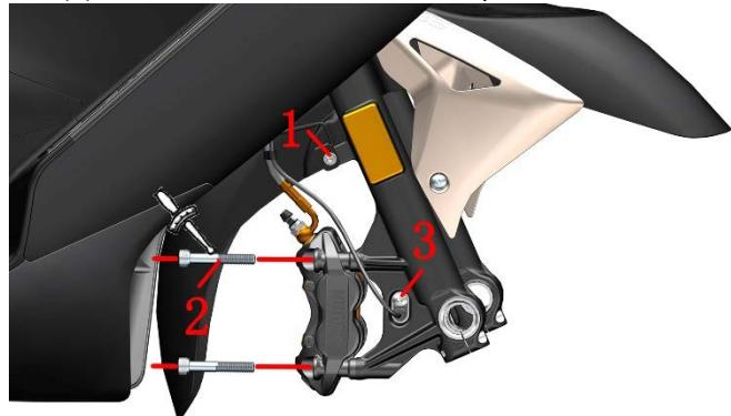
c. Use the 4# Allen to remove the 2 M6×14 shaft shoulder bolts (4) on the left and right sides of the front clay plate; Then use the 5# Allen to remove 1 M6×30 bolt (1) and remove the bullet pad (5).
