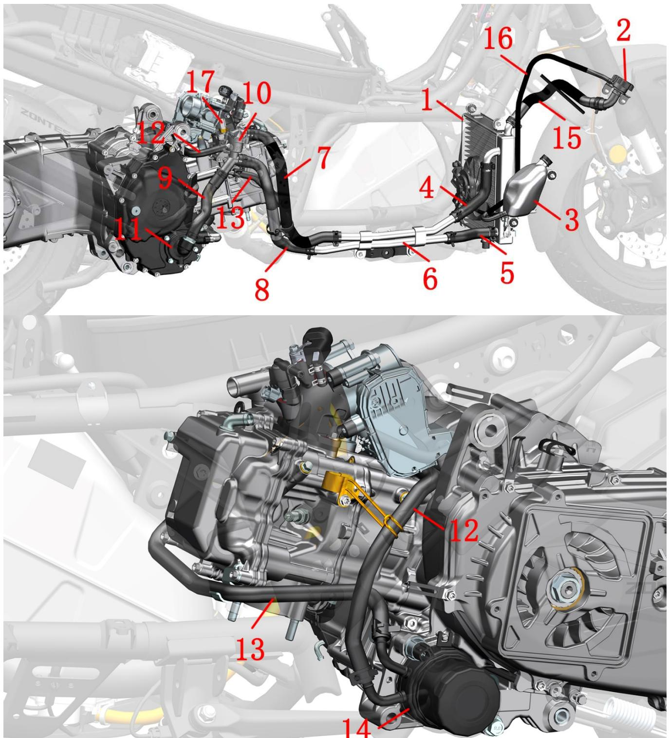
1-Main water tank 2-Water tank filling port 3-Auxiliary water tank 4-Main water tank inlet pipe 5-Main water tank outlet pipe
