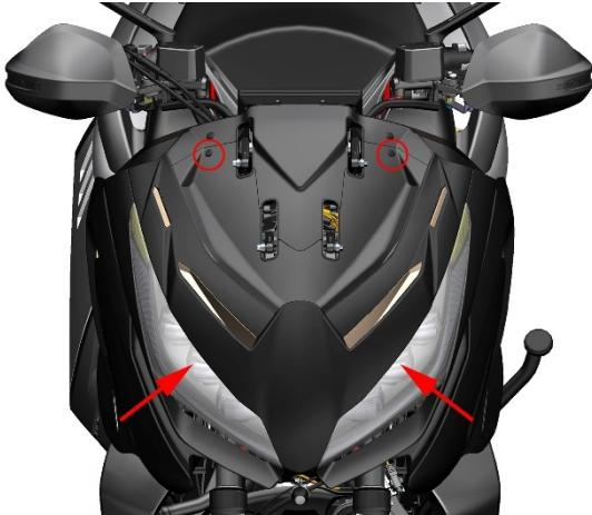
b. Lower the windshield to a low position, use 4# inner hexagon to remove the 2 front bolts, the 2 expansion bolts on the left and right sides of the rear, and the 2 left and right expansion nails on the inner
