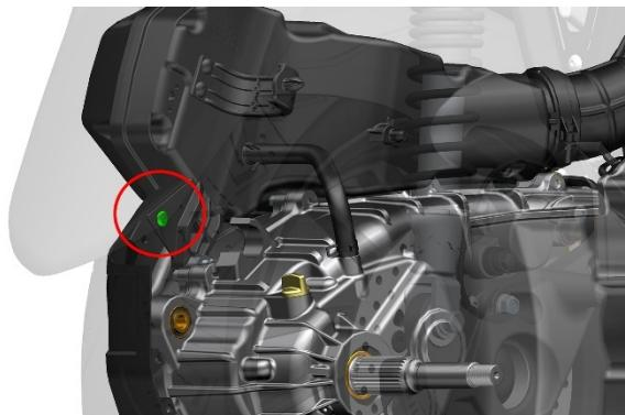
b. Use a 4# Hex key or T30 torx wrench to remove the 4 M6×14 shoulder bolt or hexagonal small flanges M6×16 torx bolts shown in the figure.
