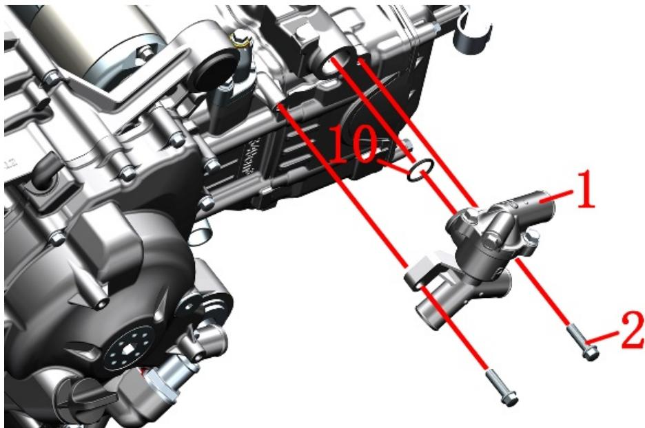
Before reassembly, the joint surface should be cleaned. Note that the O-ring cannot be missing and must be correctly assembled in place. The hoop should be clamped inside the boss to prevent loosening. Bolt(2) Torque:  $12\pm1.5$  N.m ( $1.2\pm0.2$  kgf.m,  $9\pm1$  lbf.ft).
