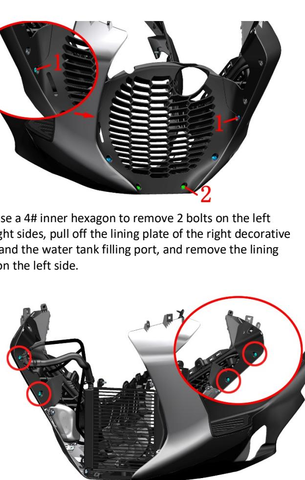
c. Press and pull out the 8 expansion nails at the bottom of the fairing, and remove the bottom of the lower fairing.
