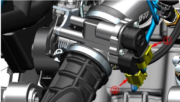
b. Place the small container under the high-pressure oil pipe, press the buckle indicated by③ and pull out the high-pressure oil pipe(1) in the direction of the arrow at the same time. A small amount of fuel will flow out when it is pulled out, and it is forbidden to drip onto the surface of the part.
