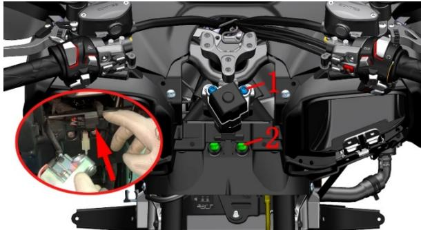
k. Remove the 4 bolts on the left and right sides that fix the panels of the front storage box.
