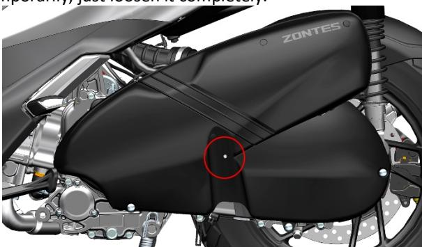
c. Use 4# inner hexagon to remove the 3 M6×14 bolts as shown in the figure. Use 4# inner hexagon to remove the screw for the air filter decorative cover bottom plate.
