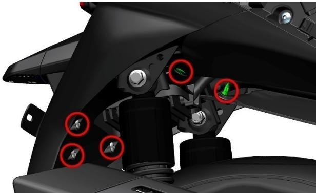
b. Use 4# inner hexagon to remove the 2 M6x14 bolts that fix the rear fender assembly on the frame.
