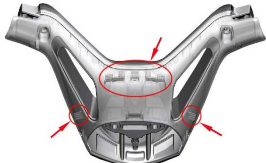
f. Replace the left and right expansion nails. Use the 4# Allen to replace the 2 bolts on the left and right sides. (Check whether the direction is crimped)
