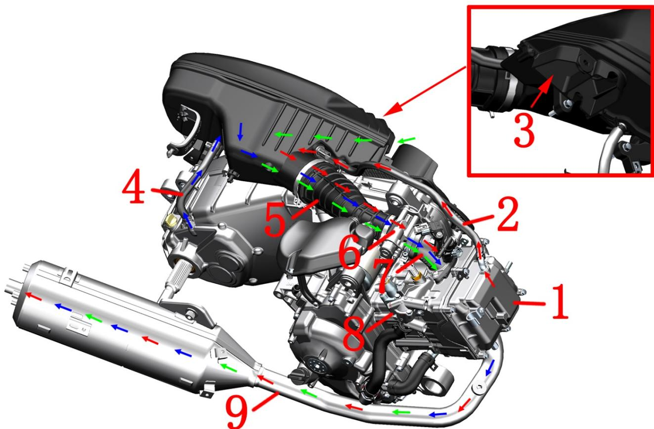
1- Cylinder head 2-Cylinder head exhaust pipe3- Air filter intake inlet 4-Crankshaft Box exhaust pipe5-Air filter outlet pipe6- Throttle valve body assembly 7-Intake manifold8- Cylinder 9- Muffler
