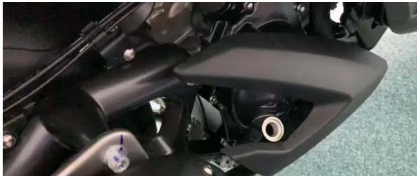
d. inspection O ring(2) Whether there is damage or aging, if not, wipe it clean, if any, replace it. The O-ring used for the oil dipstick is specified as 18x3x3.5.
