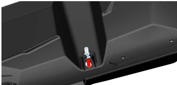
d. Align the left bolt with the mounting hole and tighten it. Put the 4 bolts back in with the 4# inner hexagon.
