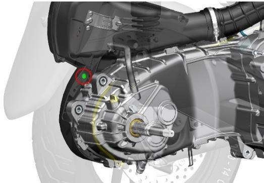
b. Use 4# inner hexagon to remove the M6×14 bolt as shown in the figure. The bolt here cannot be removed temporarily, just loosen it completely.
