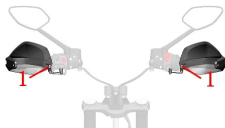
b. Use a #5 Allen wrench to loosen the balance block bolt a by 5-8 turns, then remove the left and right hand guards and the balance block assembly.
