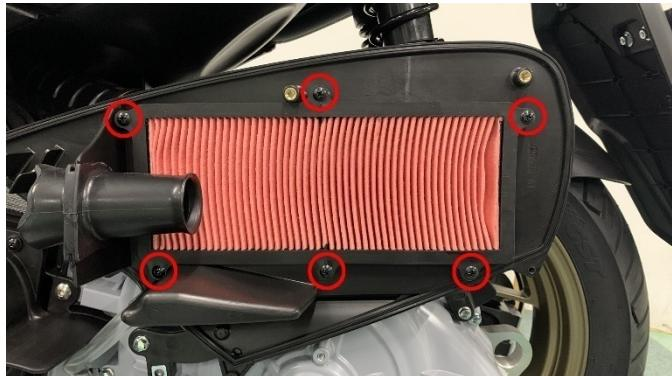
b. Remove the old air filter element. Blow the dust inside the air inlet pipe with a dust blower, and then wipe the inner wall with a clean non-woven cloth.
