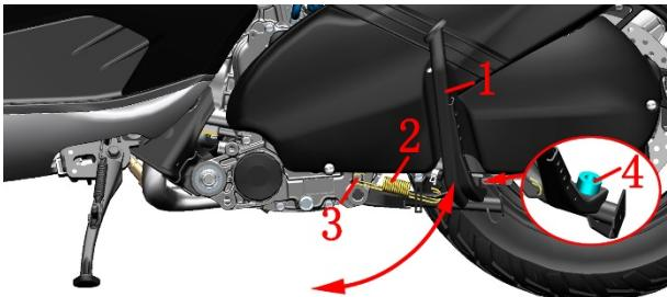
1. Main support 2. Main support spring 3. Main support return spring post 4. Cushioning glue
