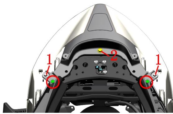
e. Remove the 2 expansion nails on the left and right sides connecting the rear fender and the rear skirt bottom plate.
