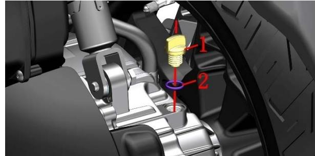
b. Place an oil pan under the rear of the left engine. Use a 14# sleeve to loosen the oil drain bolt(3) counterclockwise.
