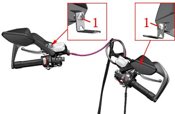
b. Use the 5# Allen to loosen the balance block bolt A 5-8 turns, and remove the left and right hand guards and the balance block assembly.
