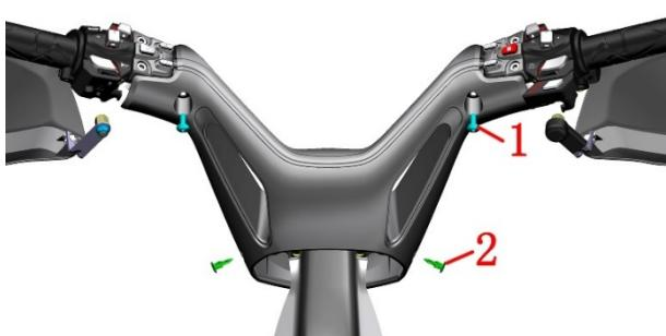
c. Use 6# inner hexagon to remove the left and right handles and switch components.
