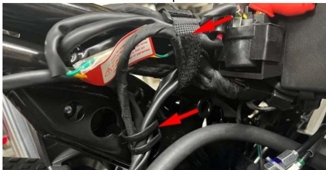
c. Loosen the clamp bolt shown in the figure with a 4# inner hexagon counterclockwise, and pull the air filter outlet pipe toward the rear wheel to pull out the throttle valve body.
