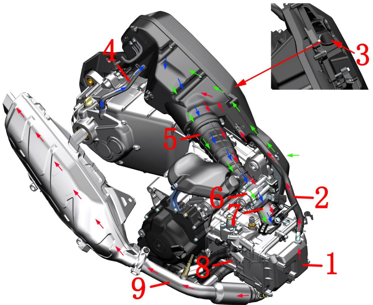
1- Cylinder head 2-Cylinder head exhaust pipe3- Air filter intake inlet 4-Crankshaft Box exhaust pipe5-Air filter outlet pipe6- Throttle valve body assembly 7-Intake manifold8- Cylinder 9- Muffler
