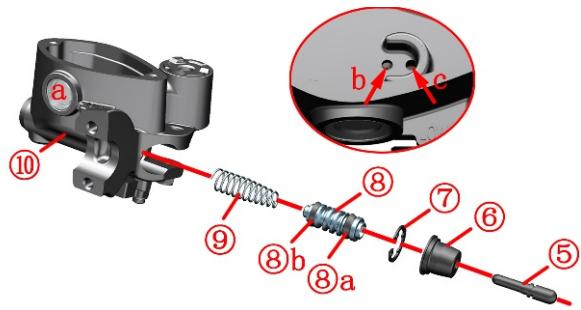
⑤ Piston push rod ⑥ dust cap ⑦ retainer ring ⑧ piston assembly (⑧ a outer seal ring ⑧ b inner seal ring) ⑨ spring ⑩ main pump housing
