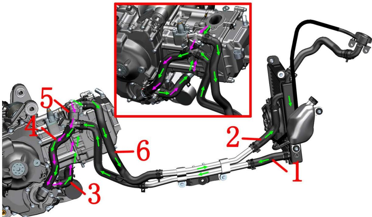
1 - Water inlet pipe 2 - Water outlet pipe of main water tank 3 - Water inlet pipe of main water tank 4 - Connecting pipe of auxiliary water tank 5 - Water inlet pipe of cylinder 6 - Water inlet pipe of water pump cover
