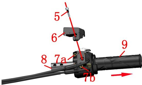
125E: Remove the bolt (5) using the cross lot. Use the 5# Allen to remove the bolts (7a) and (7b) under the right handle bar switch, and open the upper and lower parts of the right handle bar switch. Remove the right handle bar (8) and the right heated handle bar (9) separately.
