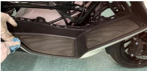
e. Remove 3 M6×16 bolts (2) with 5# inner hexagon, remove 1 M6×14 bolt (3) on the rear side with 4# inner hexagon, and remove 1 expansion nail at the front and rear (1).
