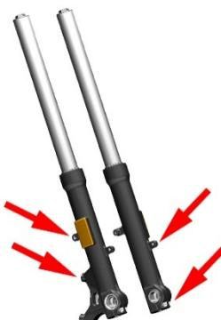
c. If there is a large amount of hydraulic oil attached to the front fork tube, wipe it clean and observe after riding. If there is no oil stain or slight oil stain, it is the hydraulic oil
