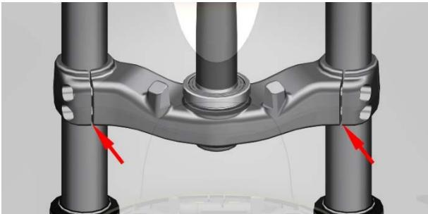
b. Use a batch to pry open a gap on the upper plate, put in the corresponding shock absorber, install the shock absorption in place, and remove the next word batch. Screw in the bolt (6) of M8×35 and tighten using the 6# Allen. Torque: 25N.m (2.6 kgf.m, 18 lbf.ft).
