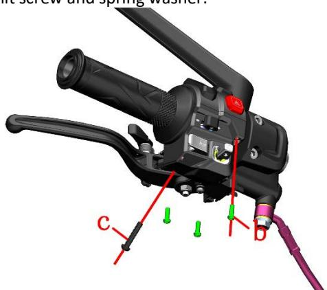
e. After removing the rubber sleeve, use a Phillips screwdriver to remove the M4×30 stop screw and spring washer.
