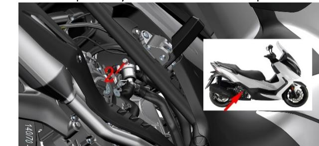
b. Remove the filler cap of the Radiator to accelerate the flow of coolant.
