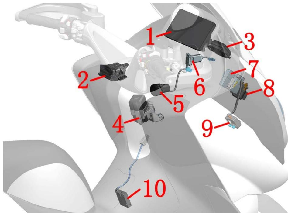
1-TFT Meter 2-Front Left Storage Box Lock Cable 3-Windshield Motor Controller 4-Main lock 5- Double Buckle USB Charging Assembly 6-Single Port Fast Charging Assembly 7-EFI Relay 8 - Starting relay 9 - Charging port holder 10 - Tank electronic lock
