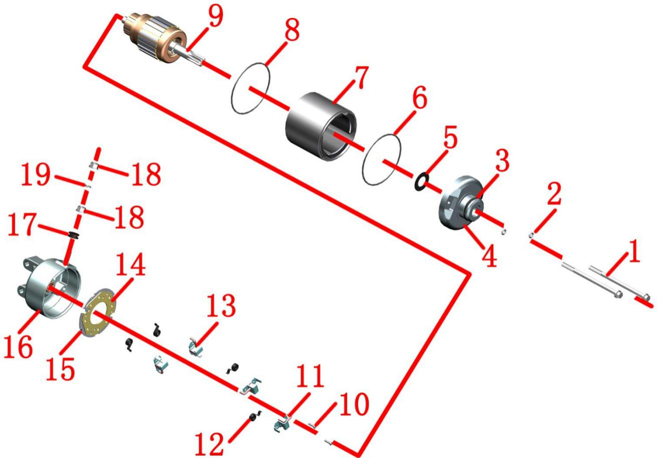
1-M6x90 bolt×2 2-O ring×2 3-O ring 4-starter motor front cover 5-gasket 6-rectangular sealing ring 7-starter motor outer shell 8-rectangular sealing ring 9-electric pole 10-screw ×2 11-Negative brush×2 12-Volute spring×4 13-Positive brush×2 14-Brush frame 15-Brush holder insulation gasket 16-Starter motor back cover 17-Insulation gasket 18-Nut×2 19- Gasket
