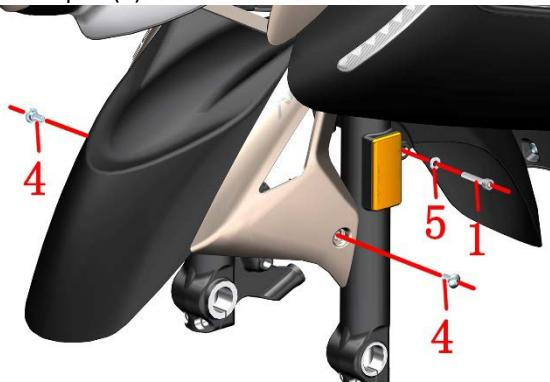
d. First press the sides of the front mud plate according to the small arrow, press the bulge at the arrow of the front mud plate inward, and then move the front mud plate up to the appropriate part and then withdraw it in the direction of the large arrow.
