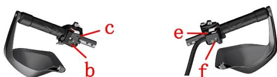
c. When installing the secondary handle bar switch, it is necessary to align the joint surface of the counter-handle bar switch and the main pump of the disc brake with the triangle mark on the handle bar switch, and then use 5# hexagon to tighten 4 M6×30 bolts.
