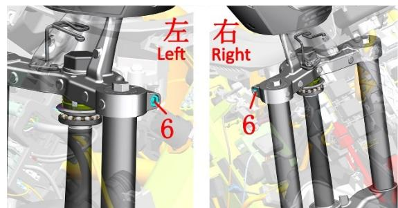
c. Use 6# hexagon to remove the 4 bolts (6) of M8×35, pry open the gap on the lower coupling with a batch of words, and remove the left front shock absorption and right front shock absorption.
