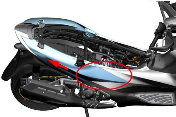
c. Disassemble and assemble the left and right rear skirt components in the same way.
