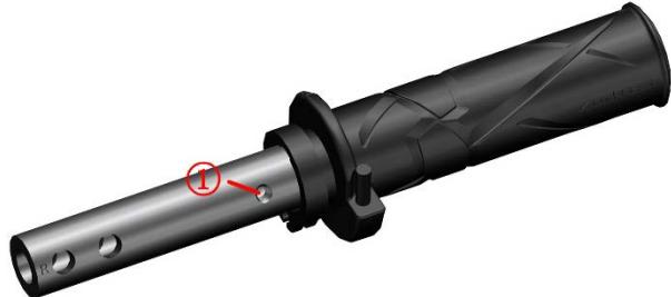
c. When installing the secondary handle bar switch, it is necessary to align the joint surface of the counter-handle bar switch and the main pump of the disc brake with the triangle mark on the handle bar switch, and then use 5# hexagon to tighten 4 M6x30 bolts.
