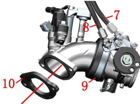
g. Use throttle valve body cleaning agent to clean the carbon deposits on the intake manifold and throttle valve body outlet respectively. It is forbidden to directly soak the throttle valve body assembly and intake manifold assembly with any liquid.
