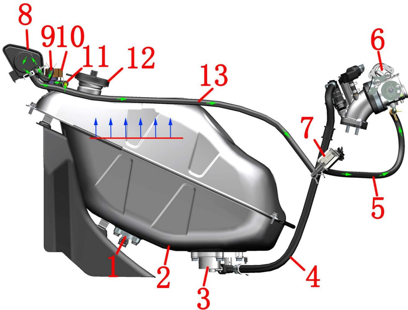
1-Oil level sensor 2-Fuel tanks 3-Fuel pump 4-High-pressure tubing 5-Solenoid valve outlet pipe
