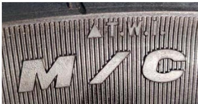
The tread bulge has a wear mark height of 1.6 mm (0.06 in). The sidewall triangle (T.W.I.) markings indicate the position of the wear strips. If it is worn to the marked point, it means that it has been worn to the limit, and it will be a safety hazard to continue driving, and it must be replaced with new tires of the same specification.
