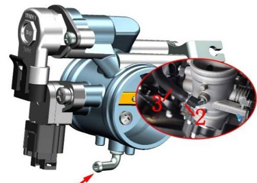
d. After loosening the bolts of the clamp (4) with a 4# hexagon socket wrench, pull out the air outlet pipe (5) of the air cleaner and the clamp (4) from the throttle body in the direction of the arrow.
