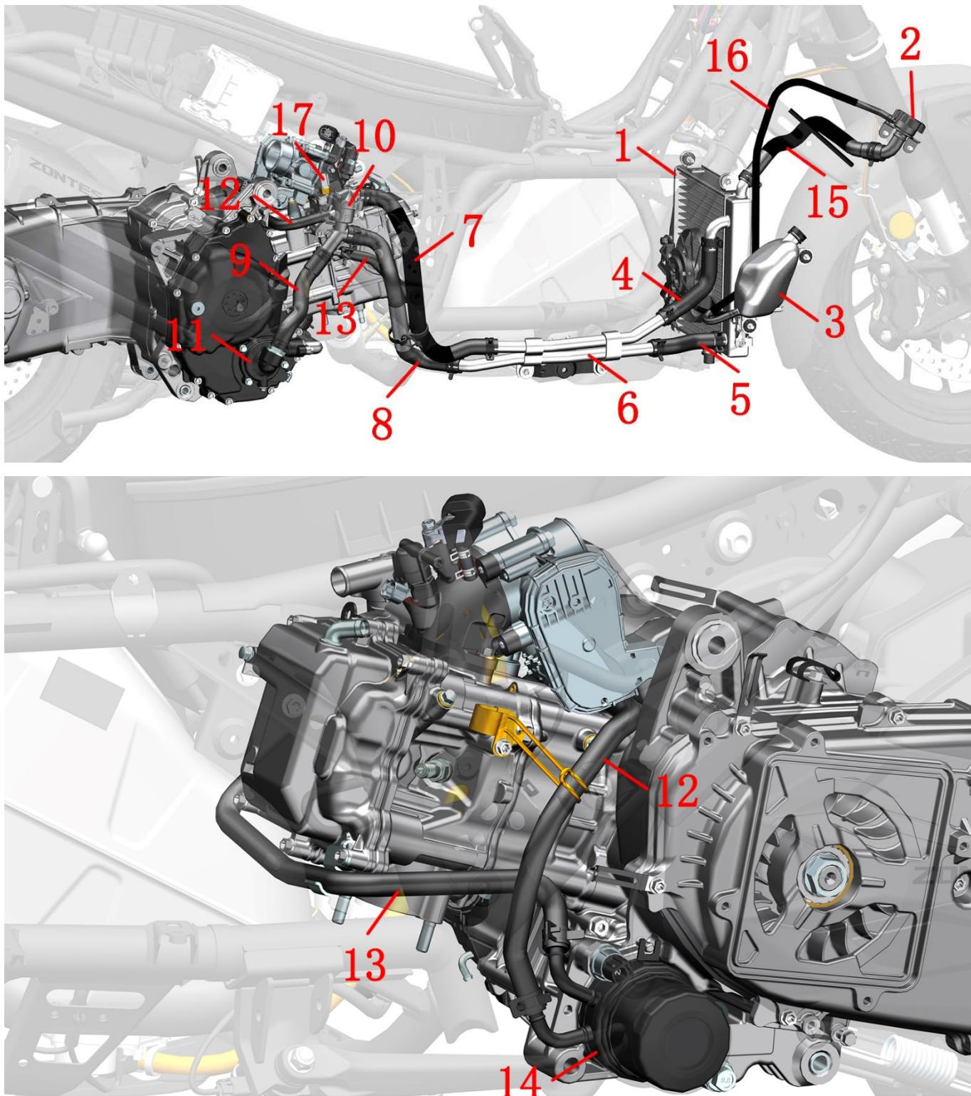
1-Main Water Tank 2-Water tank filler neck 3-Auxiliary Water Tank 4-Main water tank inlet pipe
