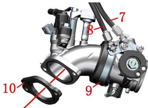
g. Use throttle body cleaner to clean the carbon deposits on the intake manifold and the outlet of the throttle body respectively. Do not directly soak the throttle body assembly and intake manifold assembly with any liquid.
