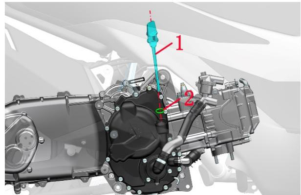
e. Wipe the dipstick clean, then use your hand to rotate clockwise to reinstall the dipstick (1) and O-ring (2) onto the right crankcase cover of the engine.
