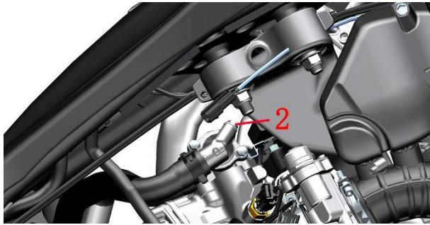
c.Wear waterproof gloves and use the extended funnel to add coolant to the main tank inlet. The coolant level is visible at the water inlet until the coolant is spilled at the stable position of the thermostat bleed bolt.
