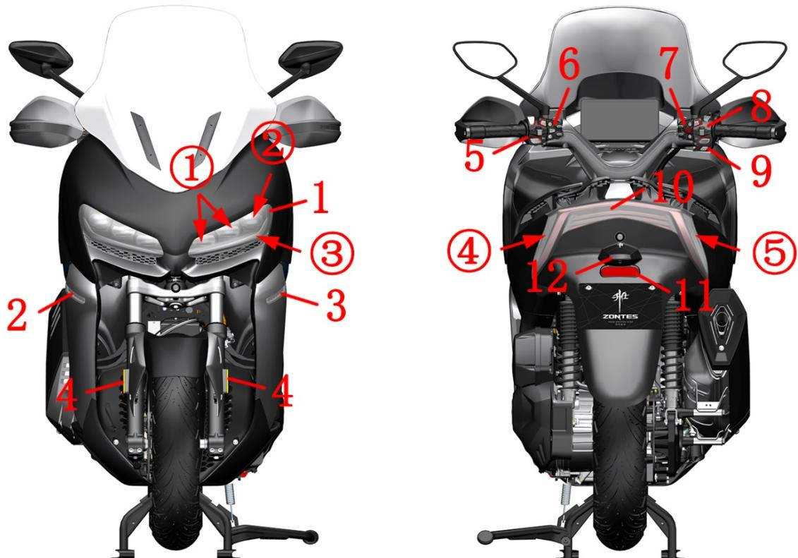
1-headlight (①-low beam position ②-High beam position ③-Position light/daytime running light position) 2-Right turn signal 3-Left turn signal 4-side reflector 5-Left hand handle switch 6-Left hand handle sub switch 7-Right hand handle sub switch 8-Right hand handle switch 9-Handle the heating switch 10-Rear tail light (④-Rear left turn signal ⑤-Rear right turn signal) 11-rear reflector 12-rear license plate lamp
