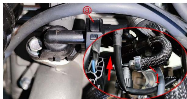
c.Find the circlip (2) at the bottom of the valve body, pinch both ends of the circlip with your hand and move it outwards, then pull out the desorption tube (3).
