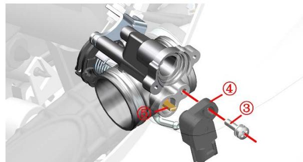
Simple test method: Connect the entire vehicle to the diagnostic instrument, press the ignition switch (no need to start the engine), turn the throttle grip from the initial position to fully open, and check during this process whether the throttle position signal changes from 0 to 100 accordingly.
