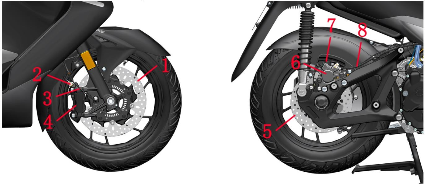
1-Front brake discs 2-FC-HU Brake hoses 3-Wheel speed sensor (front) 4-Front disc brake calipers 5-Rear brake disc
