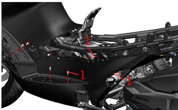
b. Remove the rubber pad on the rear right pedal. Use a T25 Torx wrench to remove 7 M6×14 shoulder bolts (1). Remove the right pedal assembly.
