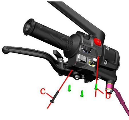
After pulling out the rubber sleeve, use a Phillips screwdriver to remove the M4×30 limit screw and spring washer.
