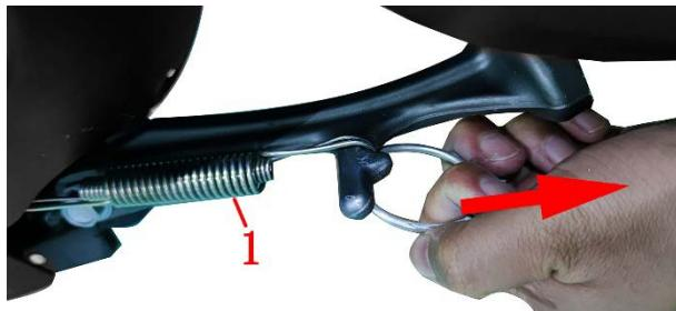
c.First, remove the side bracket spring with a hook or rope, remove the bolt (2) on the inside of the side bracket counterclockwise with an 8# sleeve, and remove the copper gasket (3) and the side bracket flame-out switch. Remove the nut (8) with a 14# socket or torx wrench, then remove the bolt (5) with a 14# socket or torx wrench, take out the bushing (6), and finally remove the side bracket (7).
