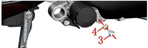
e. Wipe the joint surface clean with non-woven fabric. Check if the joint surface of the oil drain bolt (3) is scratched; if so, replace it with a new one, and if not, wipe it clean.
