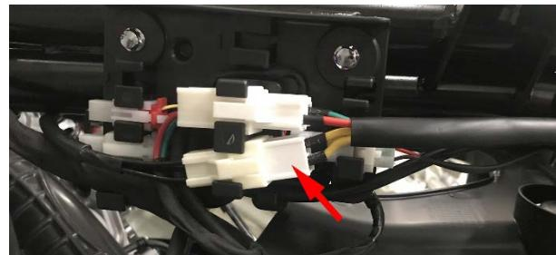
b. Check the connector for looseness or corrosion.
