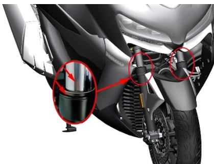
b. Check whether the bottom cylinder is peeling off the paint; Signs of whether the mounting points of the front fenders, front wheel hollow shaft and front brake calipers are broken or cracked. Check the bottom of the bottom barrel for leaks.
