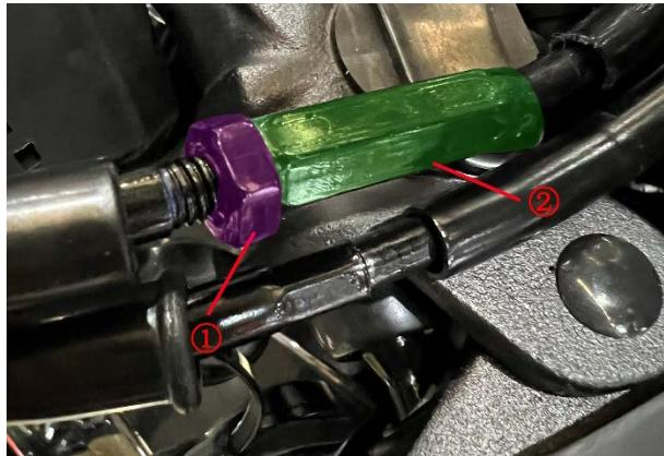
b. If the above adjustment fails to achieve the desired effect, you can refer to the description in "Disassemble the throttle body assembly to clean carbon deposits" to disassemble the throttle body assembly. Use a 10# open-end wrench to loosen the two nuts on the bracket for adjustment.
