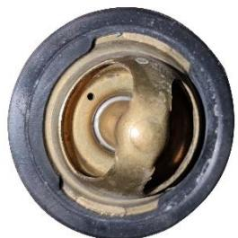
When the water temperature gauge indicates that the indication is high, the engine temperature is overheated, but the coolant temperature in the water tank is not high, it is not hot when touching the radiator with your hands, and the fan of the small water tank rotates normally. It indicates that the general circulation is blocked or blocked, and it can be preliminarily judged to be abnormal thermostat.
