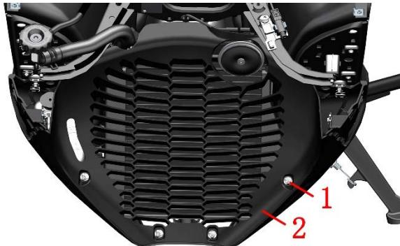
b. Use a T25 torx wrench to remove the shoulder bolts (1) and 4 expansion nails (4) that surround the bottom 4 M6×14 and remove the enveloping bottom (3).
