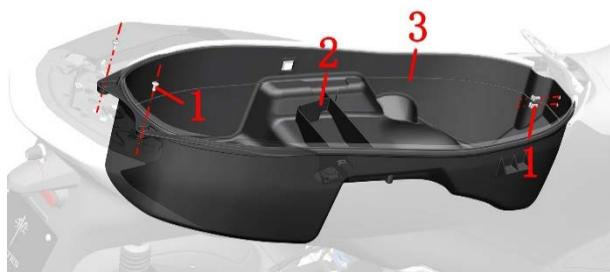
b. Use a T25 Torx wrench to remove the shoulder bolts (1) of the 2 M6×14 fixed in the rear storage compartment. After lifting the storage box slightly, pull out the storage box atmosphere light connector on the left side of the storage box, and then take out the storage box assembly.
