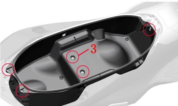
c.Slightly lift the rear of the storage box until the wiring harness connector on the left side of the storage box is exposed. Unplug the ambient light plug located on the left side of the storage box, and then completely remove the storage box after unplugging the plug.
