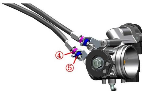
c. If neither of the above two adjustments is effective, a new throttle cable needs to be replaced.
