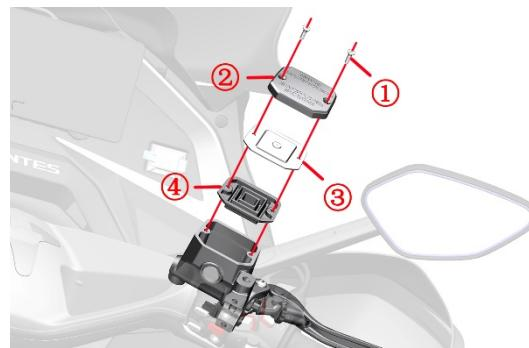
e. Use a brake fluid moisture tester to measure the moisture content. If it is >2%, replace all the brake fluid. If it is ≤2%, add new, unopened DOT 4 brake fluid to the front brake master cylinder, filling up to 3/4 of the transparent observation window. It is recommended that the moisture content be lower than 1.5%. The vehicle is factory-filled with TOTAL HBF 4 (DOT 4) brake fluid.
