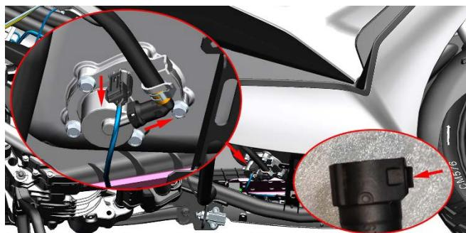
If you need to remove the fuel pump from the vehicle, you can use a siphon pump to drain the fuel from the fuel tank. After lifting the vehicle, press the plug clip as shown in the diagram to disconnect the wiring. Using a 10mm socket, remove the 5 bolts from the bottom, then remove the high-pressure fuel line bracket. Once the bracket is removed, the fuel pump can be taken out.
