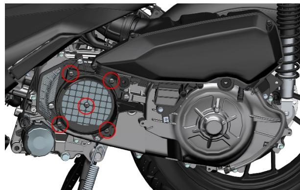
b. Remove the sponge and replace with a new filter, keeping the black side facing the engine and the white side facing outward.
