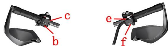
c. When installing the off-hand handlebar switch, you need to align the combination of the off-hand switch with the disc brake main cylinder to align the triangle logo on the handlebar switch, and then use the 5# hexagon socket to tighten 4 M6×30 bolts.
