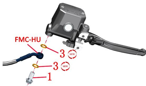
e. Remove the upper cover according to the steps of adding brake fluid, and remove the brake switch and brake handle according to the steps of removing the brake switch and brake handle.
