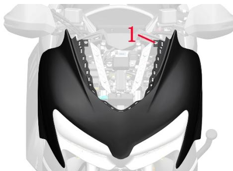
b. Use a cross batch to remove the 2 expansion nails (2) on the lid in the front panel.
