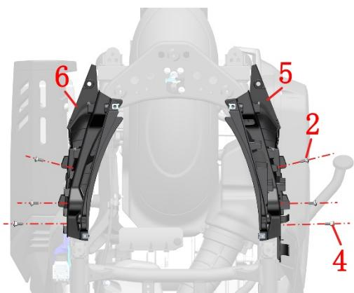
d. Use a T25 torx wrench to remove 2 expansion nails (7). Take out the left rear tail skirt liner (5) and the right rear tail skirt liner (6).
