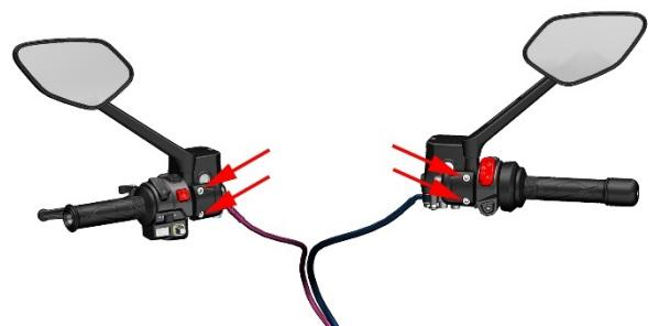
d. Use a Phillips screwdriver to remove the three M4×12 screws b that come with the left handle switch, and remove the M5×25 left handle switch limit screw c. Separate the upper and lower part of the left handle switch. After pulling out the rubber sleeve, use a Phillips screwdriver to remove the M4×30 limit screw and spring washer.
