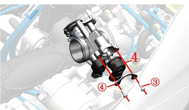
f.Use throttle body cleaner to clean the carbon deposits on the head of the stepper motor. Spray a small amount of cleaner into the valve body hole. Do not soak the stepper motor in any liquid.
