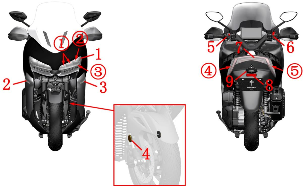
1-headlight (①-low beam position ②-High beam position ③-Position light/daytime running light position) 2-Right turn signal 3-Left turn signal 4-side Reflector 5-left hand holds the switch 6-right hand switch 7-rear taillight (④-rear Left Turn Signal ⑤-rear Right Turn Signal) 8-rear Reflector 9-rear license plate light
