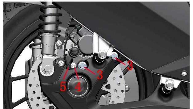
c. Remove the brake pads first.
