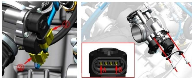
Simple test method: After turning off the power, remove the stepper motor without unplugging the cable plug. When turning on the power, press the flameout switch without ignition, check if the motor plug can contract and retract back and forth, and finally turn off the flameout switch to check if the plug returns to its original position.
