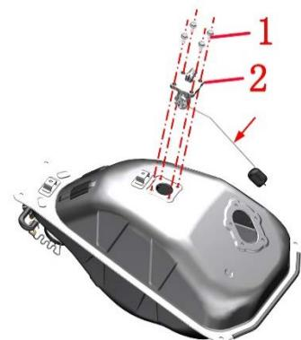
When reassembling, it is necessary to pre-tighten diagonally and then tighten 4 bolts, otherwise the sealing rubber ring of the oil level sensor is compressed unevenly, which will easily lead to leakage and cause potential safety hazards.
