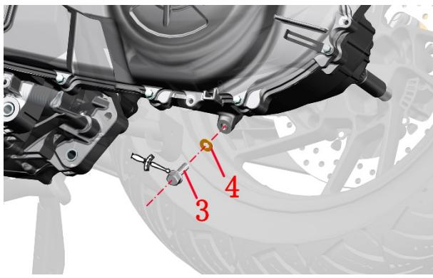
c. Remove the M8×25 oil drain bolt (3) and the 8.3×16×1.5 copper gasket (4).
