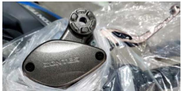
d. After wearing waterproof gloves, remove the bolt (1) with a Phillips screwdriver, and remove the upper cover (2), cover plate (3), and sealant gasket (4).
