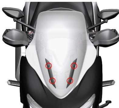
b. Use a T25 Allen Torx wrench to loosen the 4 M6×16 bolts on the left and right decorative covers of the windshield. Take out the left and right trim covers, windshields, and windshield bracket rubber pads from the windshield in turn.
