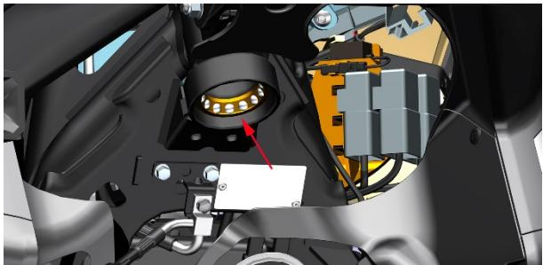
b. Put the steering column dust cover (1) and the steering column adjustment nut (2) in sequence . Then use the adjustment nut tool to tighten the torque. First tighten to 50N.m ( 5.1 kgf.m, 37 lbf.ft ) , then loosen 1/4 turn , and then tighten to 15 N.m ( 1.2 kgf.m, 11 lbf.ft ).
