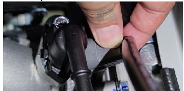
If you need to replace the injector, wait until the engine and muffler are cooled before you proceed. After placing the oil container at the bottom, refer to the steps for removing the high-pressure oil pipe to pull out the high-pressure oil pipe at the fuel pump end and release the remaining fuel. Use a 10 # sleeve to remove the bolt (1), remove the nozzle holder (2), and then remove the injector (3).
