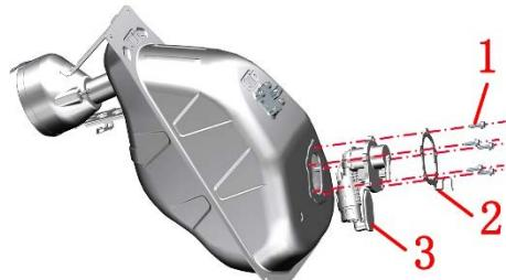
When reassembling, pre-tighten diagonally first and then tighten the five bolts (1), otherwise the sealing rubber ring of the fuel pump (3) will be compressed unevenly and easily cause leakage, resulting in safety hazards .
