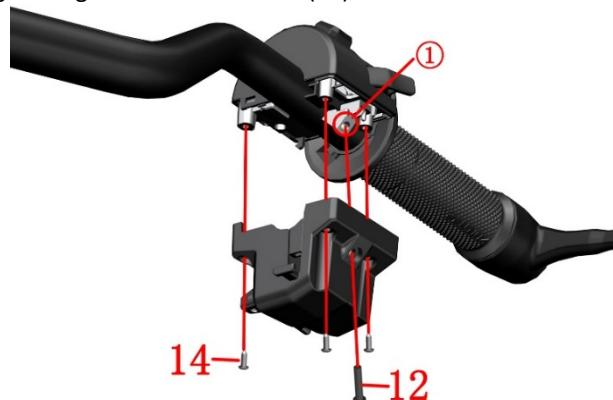
c. Use a Phillips screwdriver to install the positioning bolt (13) back into the handlebar.
