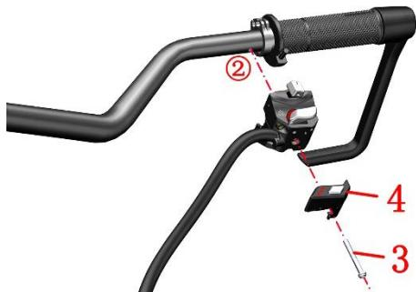
d. When installing the auxiliary handlebar switch , align the joint surface of the auxiliary handlebar switch and the disc brake master cylinder with the triangle mark on the handlebar switch , and then use 5 # hexagon socket to tighten the four M6×30 bolts .
