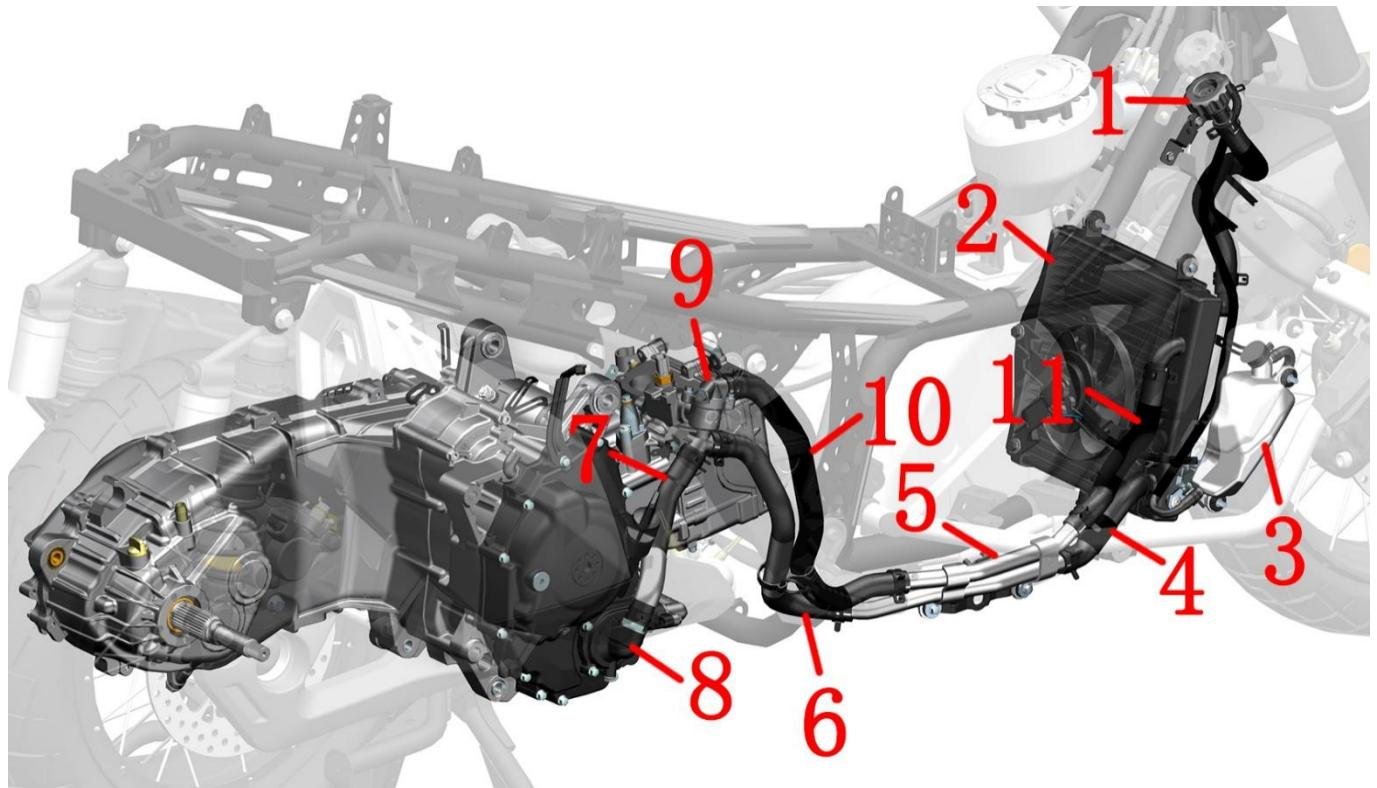
1 - Main water tank filling port 2 - Main water tank 3 - Auxiliary water tank
