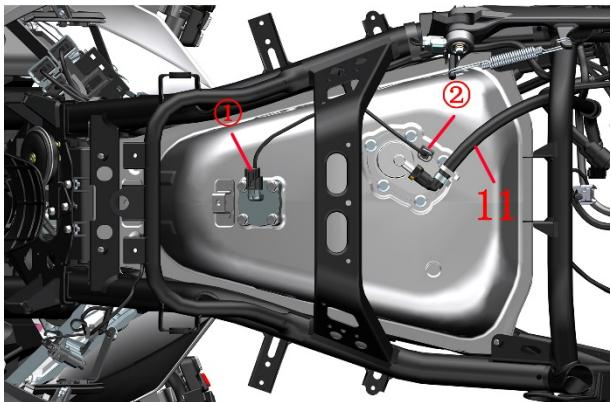
i. Use a ratchet wrench + 10# socket to remove the four M6 × 16 bolts and remove washers (13) and (14).
