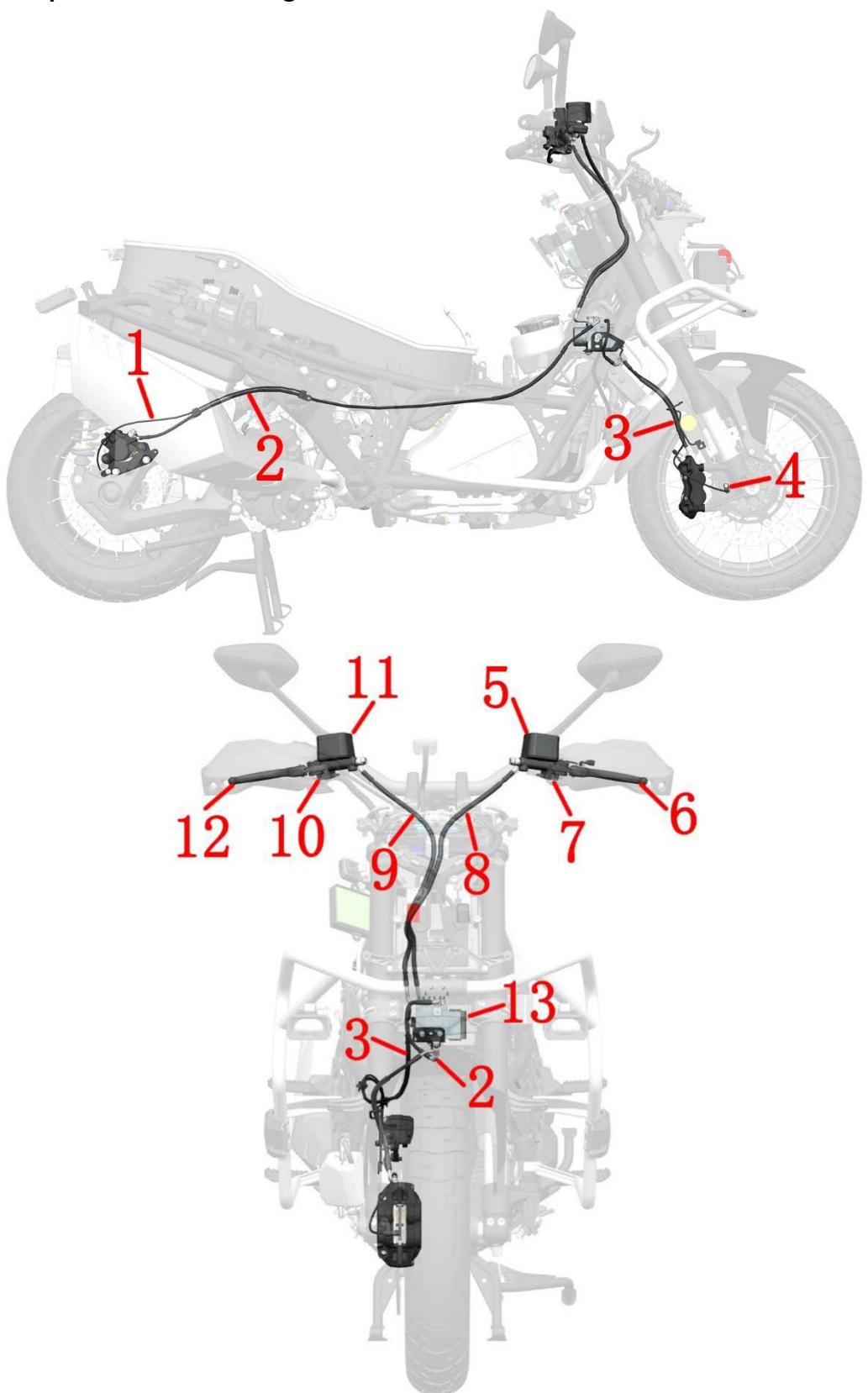
1- Wheel speed sensor ( rear wheel ) 2-FC-HU brake hose 3-RC-HU brake hose 4-Wheel speed sensor ( front wheel ) 5- Rear disc brake master cylinder 6 -Rear brake handle 7 -Rear brake switch 8-RMC-HU brake hose 9-FMC-HU brake hose 10 -Front brake switch 11 -Front disc brake master cylinder 12 -Front brake handle 13 - Hydraulic control unit
