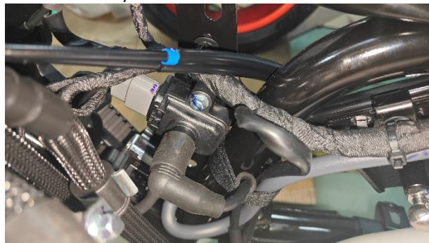
Remove the cable tie and pull out the high-voltage wire near the ignition coil.
