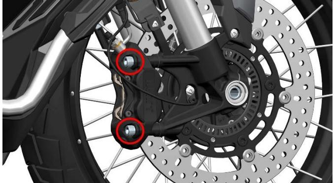
b. Place the oil pan under the front disc brake caliper.
