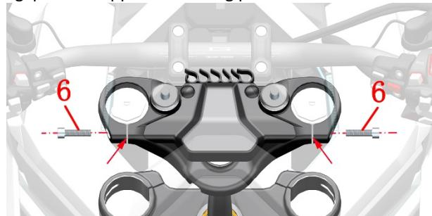
b . Use a 6# hexagon socket to remove the four M8 ×30 bolts ( 6), use a flathead screwdriver to pry open the gap on the lower connecting plate , and remove the left front shock absorber and the right front shock absorber.
