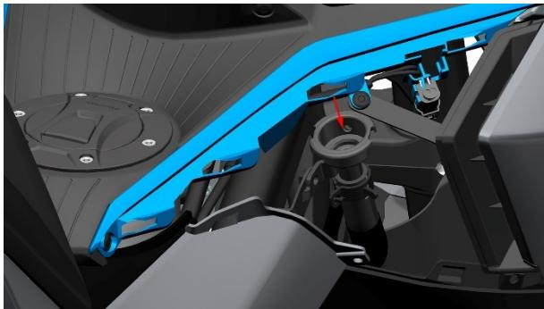
d. Tighten the main water tank water inlet cover. Tighten the exhaust bolt (2) ; torque: 8 ~ 10N. m (0.8 ~ 1 kgf.m, 6 ~ 7 lbf.ft) .
