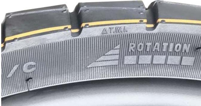
of the raised wear mark on the tread is 1.6mm ( 0.06 in ). The triangle mark (  $\triangle$  TWI ) on the sidewall indicates the position of the wear strip . If the wear reaches the mark point, it means that the wear has reached the limit. Continuing to drive will be a safety hazard and you must replace the tire with a new one of the same specification.
