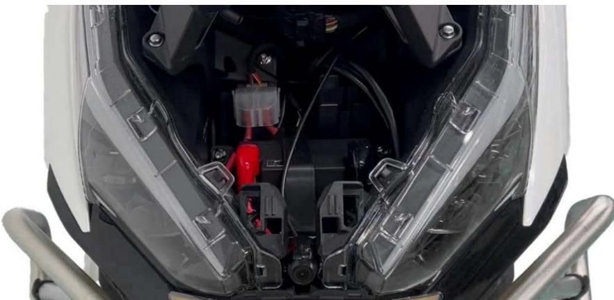
b. Unlock the vehicle, turn the engine off switch to "  $\Omega$  ", retract the side stand, hold the brake handle and press the start button. You should be able to hear the start relay closing. Otherwise, check the starting circuit.
