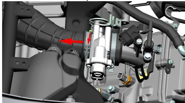
e. Use a 5# hexagon socket to remove the two bolts and remove the valve body assembly from the engine.
