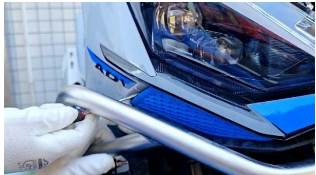
b . Use a 4 # hexagon socket or a crochet hook to remove the four expansion screws and take off the decorative piece on the head.
