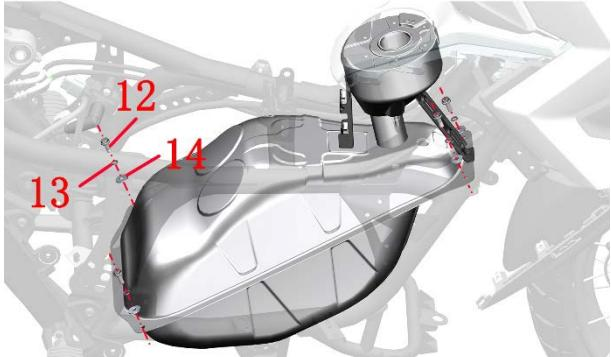
j. Slightly lift the fuel tank assembly from the rear end, move it backward until the fuel tank filling port safely passes under the frame, and then remove the fuel tank assembly upwards.
