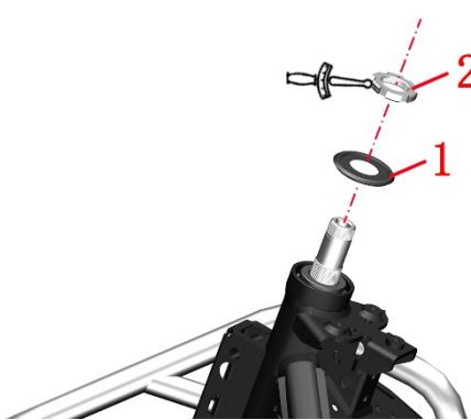
c . Ensure that the lower connecting plate rotates without getting stuck or loose, and then put in the adjusting
