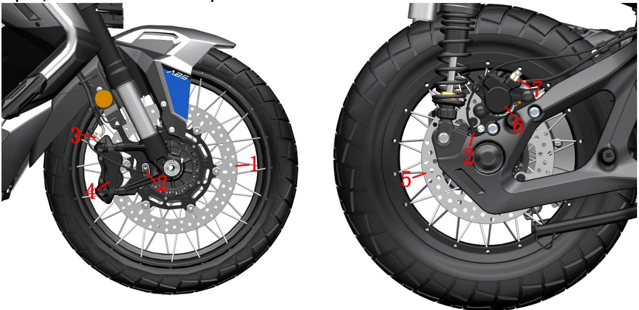
1 - Front brake disc 2 - Wheel speed sensor 3 -FC-HU brake hose 4 - Front disc brake calipers 5 - Rear brake disc 6 - Rear disc brake caliper 7 - RC-HU brake hose
