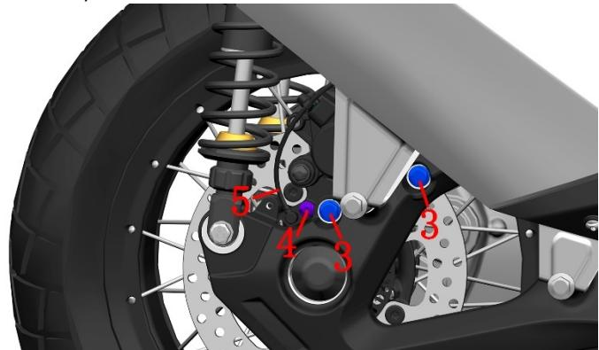
c. Remove the brake pads first.
