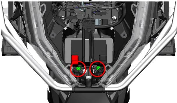
f. Unplug the left and right headlight plugs and remove the headlights.
