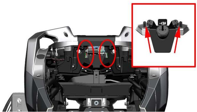
B. Remove the camera assembly from the rear of the vehicle.
