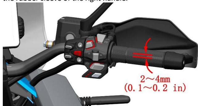
d. After starting the engine, turn the steering handle left and right to ensure that the idle speed remains unchanged during the steering process, and then turn off the engine.
