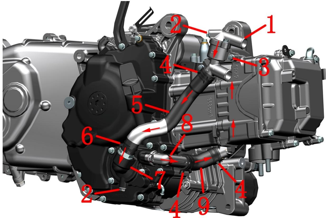
1 - Thermostat assembly 2 - M6×12 bolt\* 2 3 - M6×22 bolt \* 2
