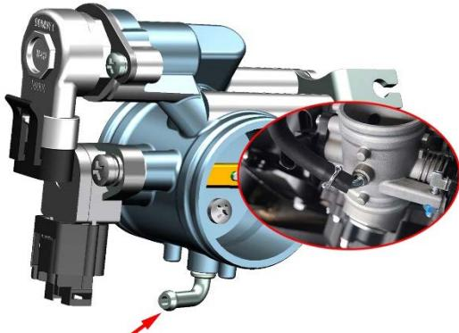
d. Use a 4# hexagon socket to loosen the bolts of the clamp and then pull the air filter outlet pipe and the clamp out of the throttle valve body in the direction of the arrow.
