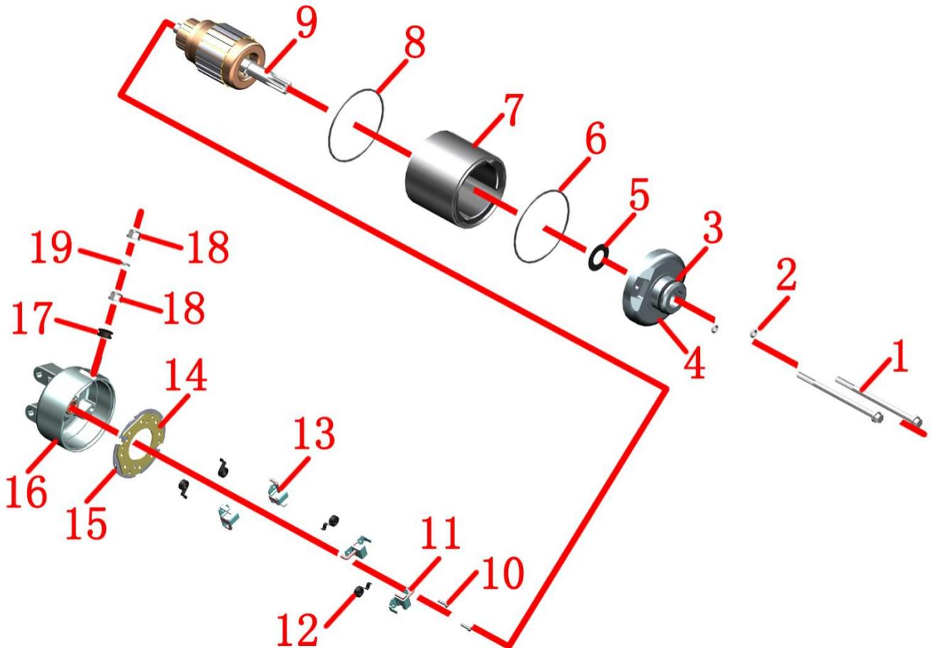
1-M 6 x 90 bolt x 2 2-O ring x 2 3-O ring 4-Starter motor front cover 5-gasket 6-rectangular seal 7-Starter motor outer shell 8-rectangular seal 9-electrode 10- screw x 2 11- Negative brush x 2 12-Coil spring x 4 13-Positive brush x 2 14-Brush rack 15-Brush rack insulation gasket 16-Starter motor rear cover 17-Insulation pad 18-Nut x 2 19-Gasket
