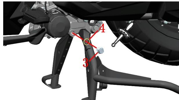
e. Wipe the joint surface clean with non-woven cloth. Check whether the joint surface of the drain bolt (3) is scratched; if so, replace it with a new one, otherwise wipe it clean.
