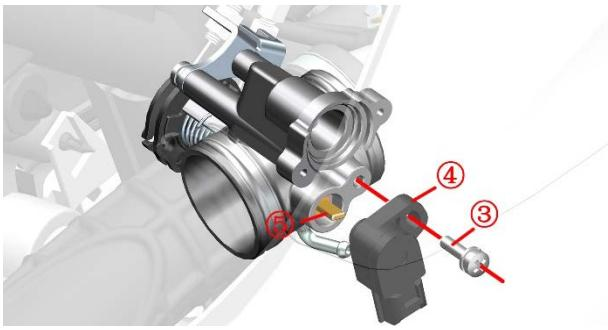
Simple test method: Connect the vehicle to the diagnostic instrument, press the ignition switch (no need to start the ignition), turn the throttle handle from the initial position to full open, and check whether the throttle position signal changes from 0 to 100.
