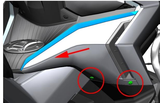
c. Use a # 4 hexagon socket or hook to remove the expansion screw that secures the right side plate assembly of the head.
