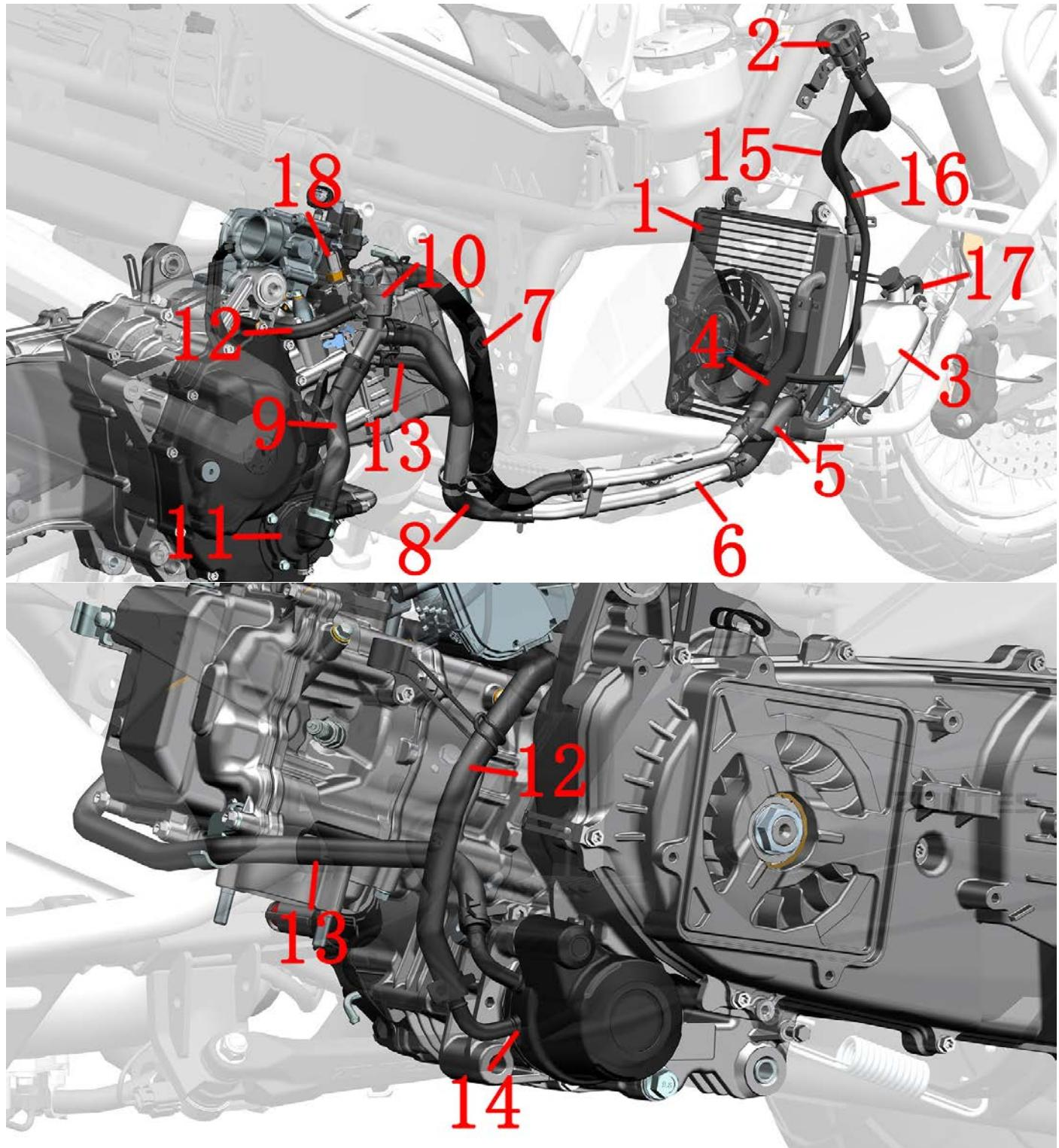
1- Main water tank 2- Main water tank filling port 3- Auxiliary water tank
