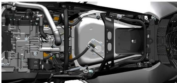
If you need to remove the fuel pump from the vehicle, use the fuel pump to drain the fuel in the fuel tank. Lift the vehicle and press the plug buckle shown in the figure to pull out the cable. Remove the 5 bolts from the bottom with a 10 # socket, and remove the high-pressure oil pipe bracket to remove the fuel pump.
