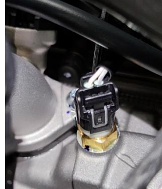
First, refer to the steps for removing the storage box to remove the storage box, and refer to the steps for removing the throttle body to remove the throttle body to facilitate the removal of the water-oil common sensor. Located on the right side of the intake manifold. First, pinch the top of the plug, press the anti-drop card, and then pull out the plug.
