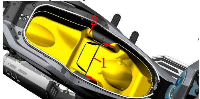
b. Use a T25 hexagonal wrench to remove the eight M6 bolts securing the rear storage box .
