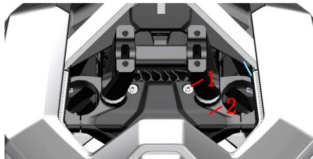
b. Use a ratchet wrench + extension rod + 30 # sleeve to remove the cap nut (8) of the upper connecting plate, and remove the gasket (9). Take out the gasket and the upper connecting plate together .
