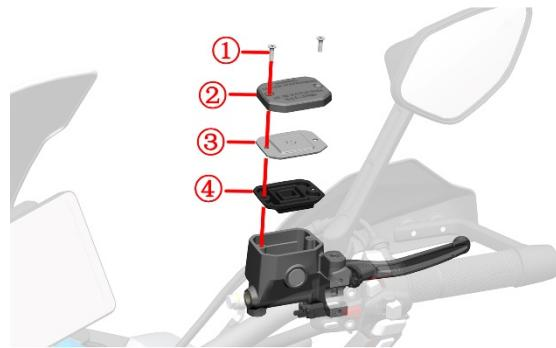
e. Use a brake fluid water content tester to measure the water content. If it is > 2%, replace all brake fluid ; if it is ≤ 2 %, add newly opened DOT 4 brake fluid to 3/4 of the transparent observation window of the front disc brake master cylinder. The recommended water content should be less than 1.5 %. This vehicle is factory-added with TOTAL Total HBF 4 (DOT 4) Brake fluid.
