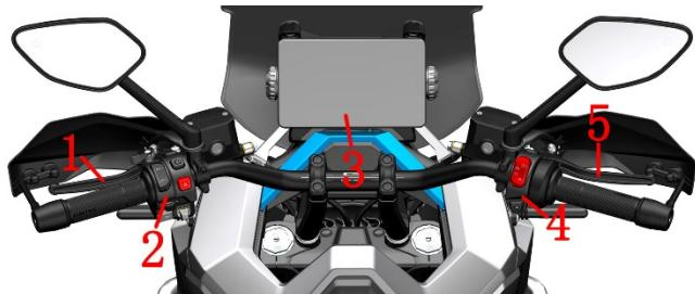
1.Rear Brake Lever 2.Left Handlebar Switch 3.Meter 4.Right Handlebar Switch 5.Front Brake Lever
