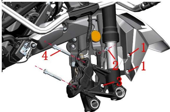
c. Use a T45 hexagon wrench to remove the two M6× 14 shoulder bolts . Use a 10 # socket to remove the M6× 20 bolt (2) .
