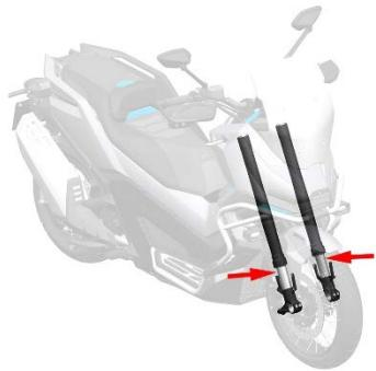
b. Check the bottom of the drum for paint peeling; check the front fender, front wheel hollow shaft and front brake caliper mounting points for signs of breakage or cracking. Check the bottom of the drum for leakage.
