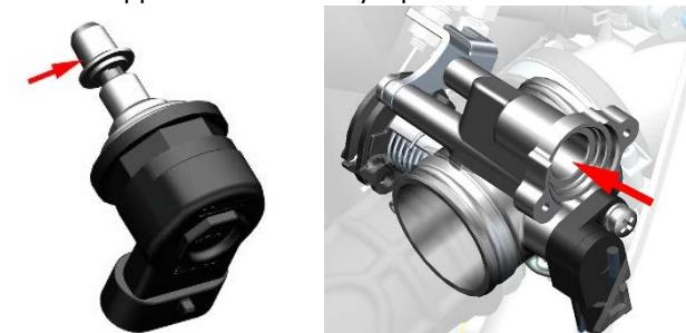
e. Install the stepper motor back onto the valve body, making sure the sealing ring is not missing. Plug the plug back in.
