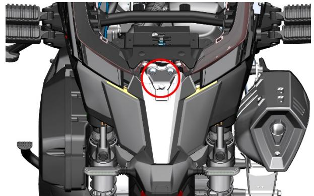
c. Unplug the connectors of the rear license plate light, left and right rear turn signals and rectifier, and remove the rear fender assembly.
