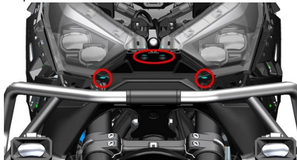
c . Remove the left and right head linings.
