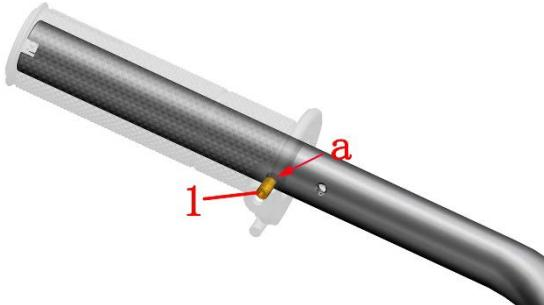
b . When installing the left-hand switch, align the cross head bolt (2) with the positioning hole ① on the handlebar and the direction handle, and then tighten it with a cross screwdriver . Align the upper and lower parts of the left-hand switch, and use a 5 # hexagon socket to tighten the two bolts that come with the left-hand switch .
