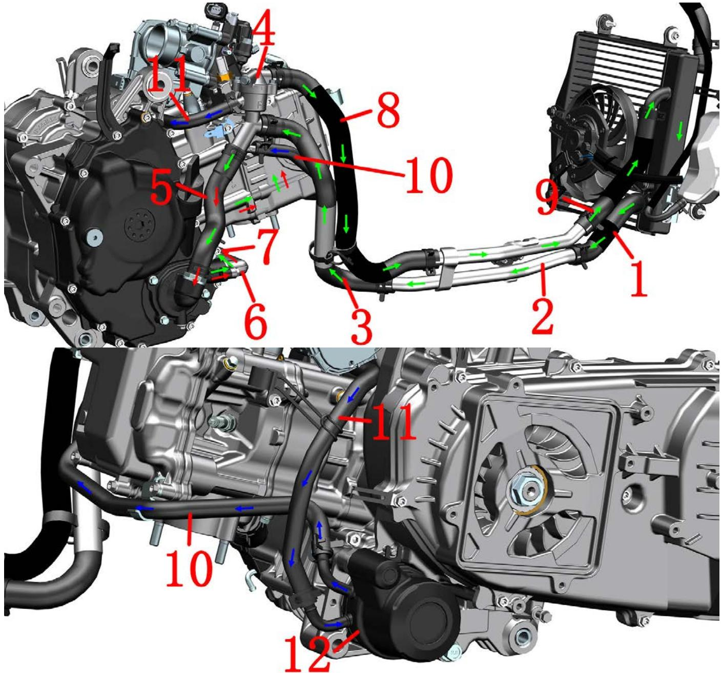
1- Main water tank outlet pipe 2- Aluminum water pipe 3- Engine water pipe
