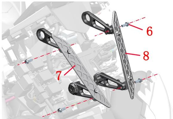
c. Use the 8# sleeve to remove 4 M6×16 bolts (6), and remove the motor pressing plate (9).
