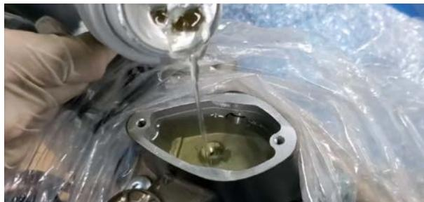
f.Observe whether the liquid level of the main pump is at 3/4 of the transparent inspection place, if not, it needs to be added or pumped out or discharged with a syringe.
