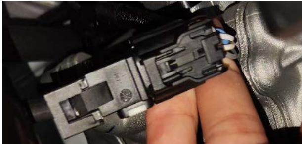
The resistance value of the heating element measuring the two white wires with a multimeter is  $9\pm2\text{k}\Omega$ ; or measure its current should be  $\leq 2.1\text{A}$ . Otherwise, it can be judged that the oxygen sensor is faulty. The ceramic inside the oxygen sensor
