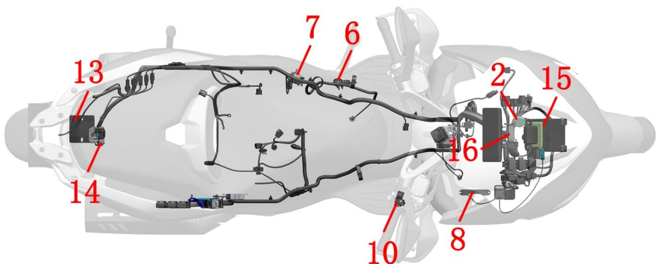
1-TFT meter 2-Flasher 3-Windshield motor controller 4-accumulator 5-horn 6-Side bracket kill switch 7-Canister solenoid valve 8-No electrical inductive antenna 9-Steering lock 10-Electric handbar switch 11-Tire pressure receiver 12-Engine controller (ECU) 13-rectifier 14-Cushion lock 15-PKE 16-Tilt switch
