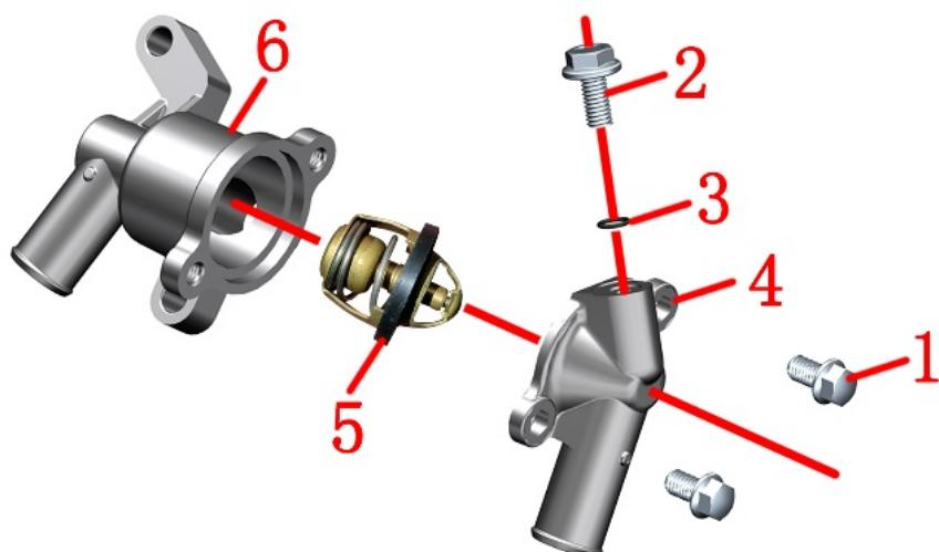
1-M6×10bolt\*2 2-M6×12bolt 3-φ5.6×φ1 O-ring 4-upper housing of thermostat 5-thermostat core 6-thermostat lower housing
