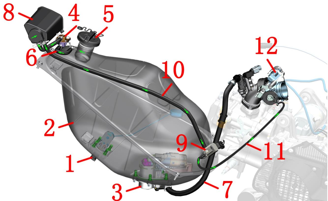
1-Oil level sensor 2-Fuel tanks 3-Fuel pump 4-Air-oil separator (welded inside the tank) 5-Fuel tank cap 6-Adsorption/ventilation tubes 7-High-pressure tubing 8-Carbon canisters 9-Canister solenoid valve 10-Solenoid valve intake pipe 11-Solenoid valve outlet pipe 12-Throttle body assembly
