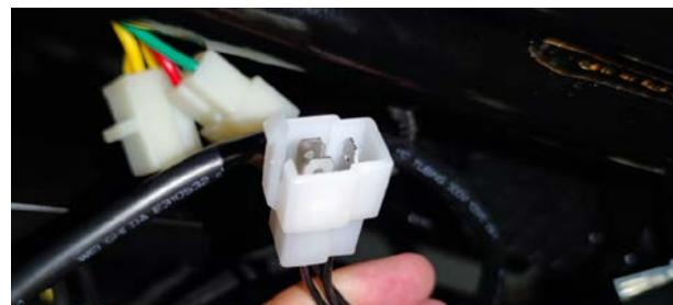
d. After disconnecting the yellow 3P connector, use the multimeter to measure the voltage between the red positive wire and the green negative wire. It should match the battery voltage. Use the multimeter's buzzer mode to check if the green negative wire is continuously connected to the ground (the ground wire can be any stud directly connected to the frame).
