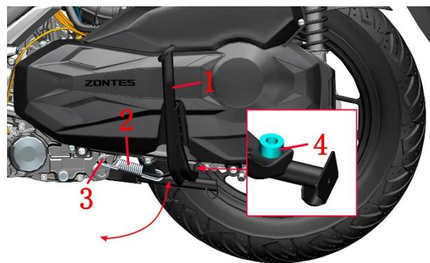
1.Main bracket 2.Main bracket spring 3.Main bracket return spring column 4.Buffer glue
