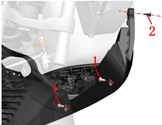
c. After taking out the left pedal rubber pad (3), use a T25 torx wrench to remove the shoulder bolt (1) of 1 M6×14 on the left pedal.
