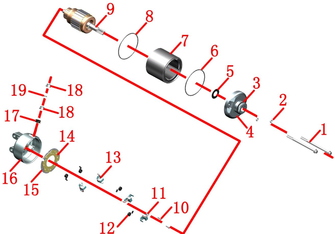
1-M6×90 bolt×2 2-O ring×2 3-O ring 4-starter motor front cover 5-gasket 6-rectangular sealing ring 7-starter motor outer shell 8-rectangular sealing ring 9-electric pestle 10-screw ×2 11-negative brush ×2 12-worm spring ×4 13-positive brush ×2 14-brush rack 15-brush holder insulating gasket 16-starting motor back cover 17-insulating pad 18-nut×2 19-gasket
