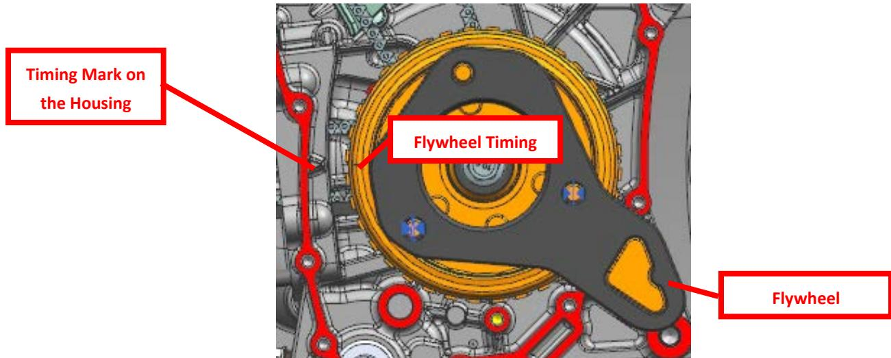
b.Tighten the timing chain again, and check that the "T" mark on the flywheel aligns with the adjacent line and the triangle mark on the housing.
