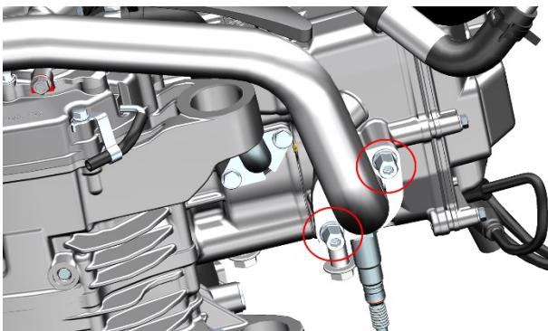
a.If there is a slight air leak, you can first try to tighten the exhaust port nut with a 6# hexagon socket wrench; if the problem persists, you will need to remove the muffler and replace the engine exhaust port gasket with a new one.
