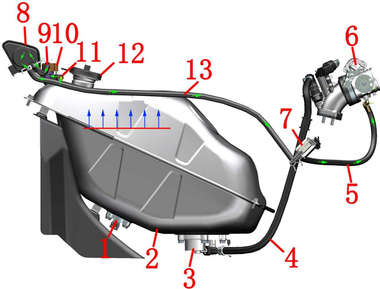
1-Oil level sensor 2-Fuel tanks 3-Fuel pump 4-High-pressure tubing 5-Solenoid valve outlet pipe
