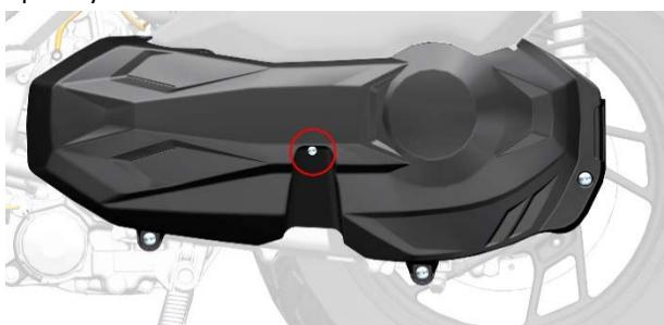
c. Use a T30 torx wrench or 8# socket to remove the 3 M6×16 hexagonal small flange torx bolts, flanging bushings and buffer glue as shown in the figure, and be careful not to lose the bushing and buffer glue. Or use 4# hexagon to remove 3 M6×14 shaft shoulder bolts. Press the center pin of the expansion nail of the air filter decoration cover with a 4# hexagon socket to remove the expansion nail. Then remove the trim cover.
