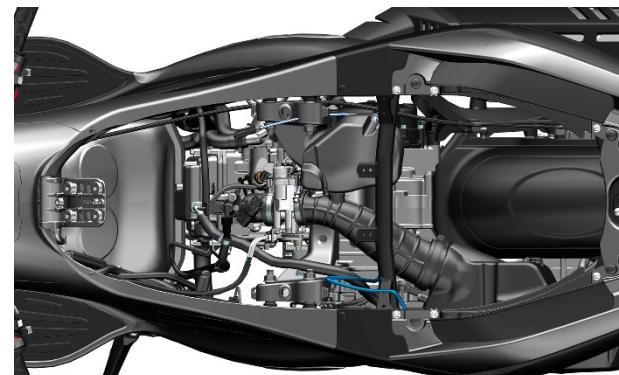
b. Use a T25 torx wrench to remove the 4 shoulder bolts (1) of M6×14 on both sides and the 4 expansion nails (2) in the middle. Remove the bottom of the lower bracket (3).
