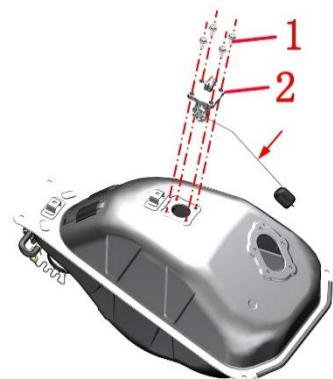
When reassembling, it is necessary to pre-tighten diagonally and then tighten 4 bolts, otherwise the sealing rubber ring of the oil level sensor is compressed unevenly, which will easily lead to leakage and cause potential safety hazards.
