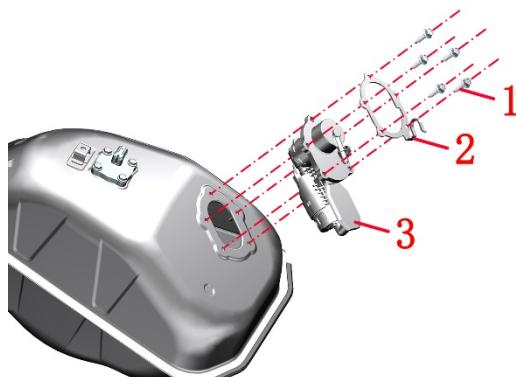
When reassembling, it is necessary to pre-tighten diagonally and then tighten 5 bolts (1), otherwise the sealing ring of the fuel pump (3) is compressed unevenly, which is easy to lead to leakage and cause potential safety hazards.
