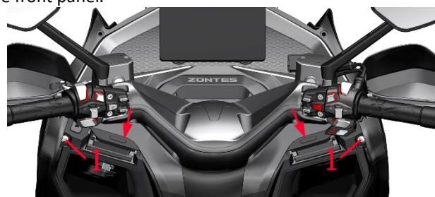
**Disassembly of windshield motor components**
