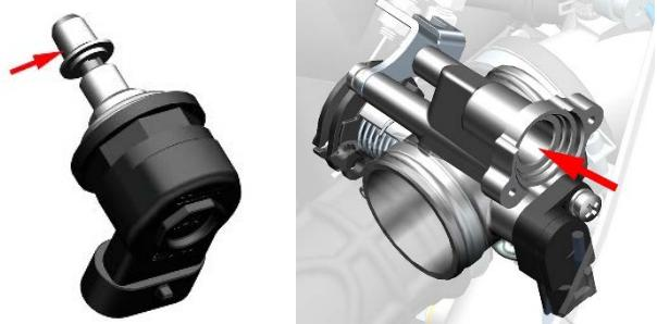
g.Install the stepper motor back onto the valve body, ensuring that the sealing ring is not omitted. Plug the connector back in.
