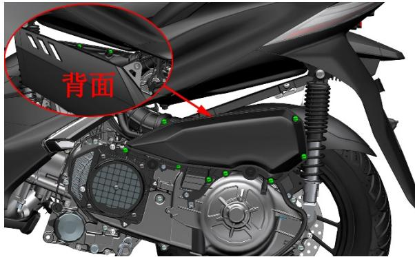
b. Remove the air filter housing.
