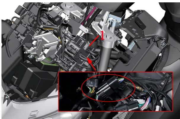
b. Find the front camera harness plug, press the buckle to remove the plug, use the 8# sleeve to remove 4 M6×22 hexagonal flange bolts (2), and then remove the headlight assembly.
