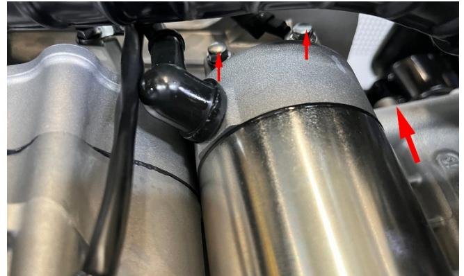
e. When reinstalling, pay attention not to omit the O ring of the starting motor, and align the teeth of the electric starting reduction gear. Note that the O-ring needs to be properly fitted into the box, as cutting edges can cause leakage. The torque of the two bolts that hold the starter motor in place:  $12\pm1.5\text{ N.m}$  ( $1.2\pm0.2\text{ kgf.m}$ ,  $9\pm1\text{ lbf.ft}$ ). and mark with a marker.
