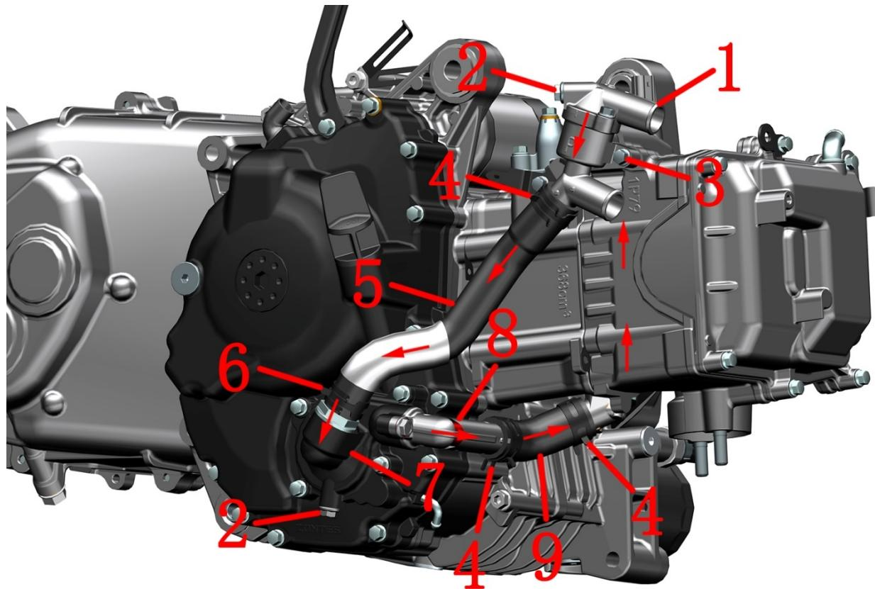
1-Thermostat assembly-M6×12 bolt\*2 3- M6×22bolt\*2 4-Water pipe hoop( $\phi$ 26)\*3 5-Water pump cover inlet pipe 6-Water pipe clamp( $\phi$ 24) 7-Water pump cover assembly 8-Water pump cover outlet pipe joint 9-Water pump cover outlet pipe
