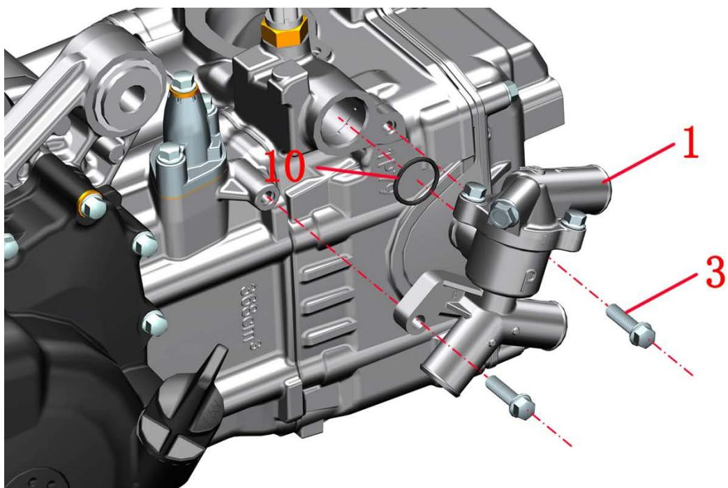
The joint surface should be cleaned before reassembly, and it should be noted that the O-ring should not be missed and
