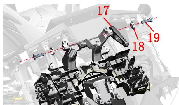
**The front of the front compartment panel is removed**
