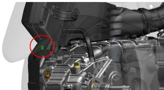
b. Use a T30 torx wrench to remove the torx bolt in the M6×16 hexagonal small flange shown in the figure or remove the M6×14 shaft shoulder bolt with a 4# hexagon socket, the bolt here cannot be removed temporarily, and it can be completely loosened.
