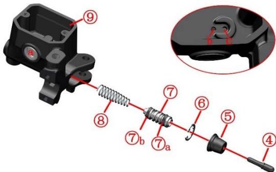
④Piston pushrods ⑤Dust cap ⑥Retaining rings ⑦Piston assembly (⑦a Outer seal ⑦b Inner seals) ⑧spring ⑨Main pump housing
