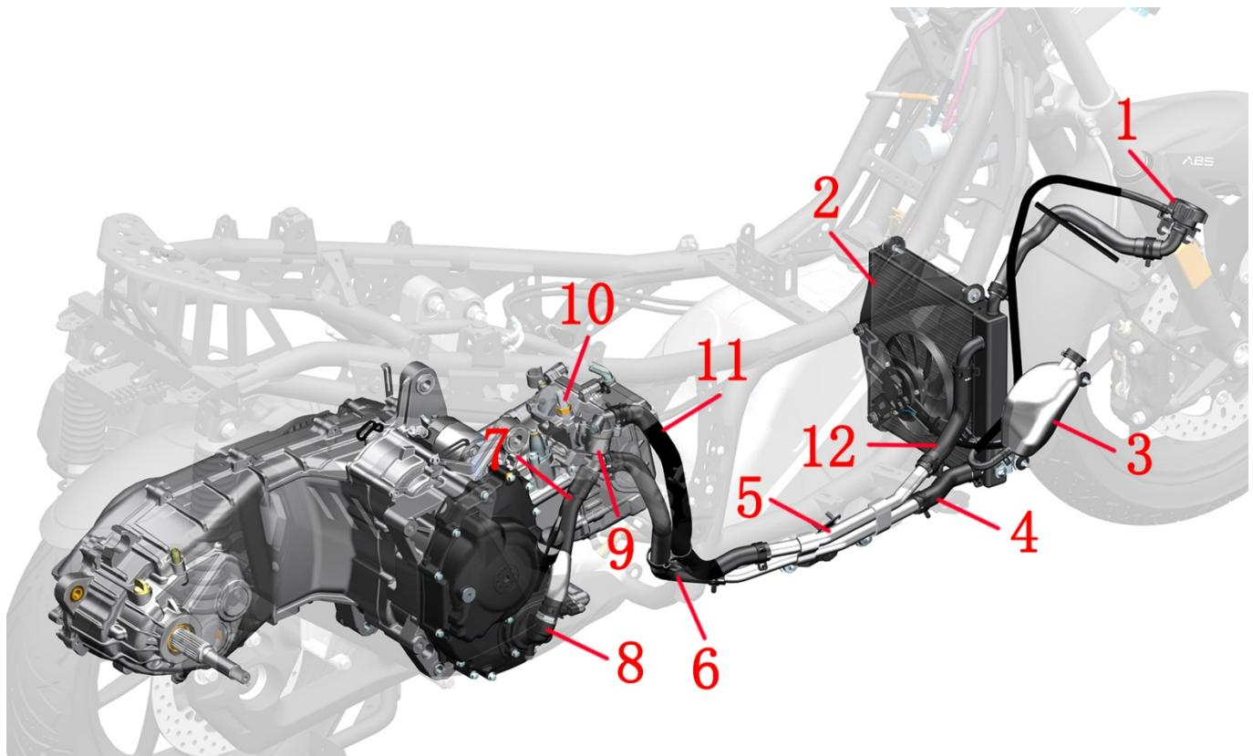
1-Main tank filler 2-Main water tank 3-Auxiliary tank 4-Main tank outlet pipe 5-Aluminum water pipes 6-Engine water pipes
