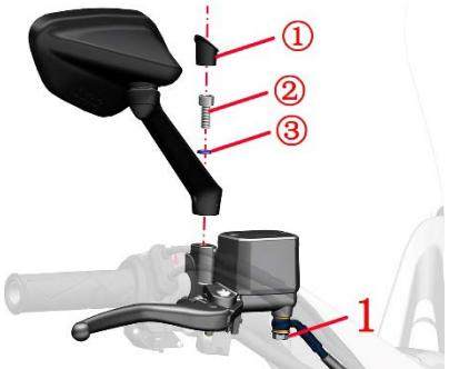
c. After grasping the front brake main pump, remove the 2 bolts (2) with 5# hexagon and remove the right switch.
