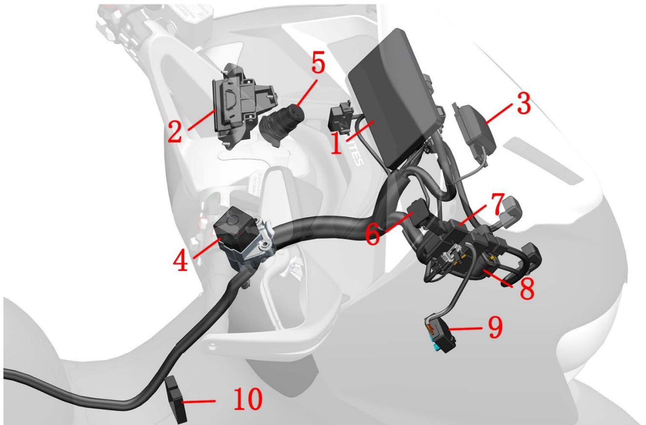
1-TFT appearance 2-Front left storage compartment lock 3-Windshield motor controller 4-Steering lock
