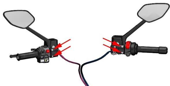
d. Use a Phillips screwdriver to remove the three M4×12 screws b that come with the left handle switch, and remove the M5×25 left handle switch limit screw c. Separate the upper and of the left handle switch. After pulling out the rubber sleeve, use a Phillips screwdriver to remove the M4×30 limit screw and spring washer.
