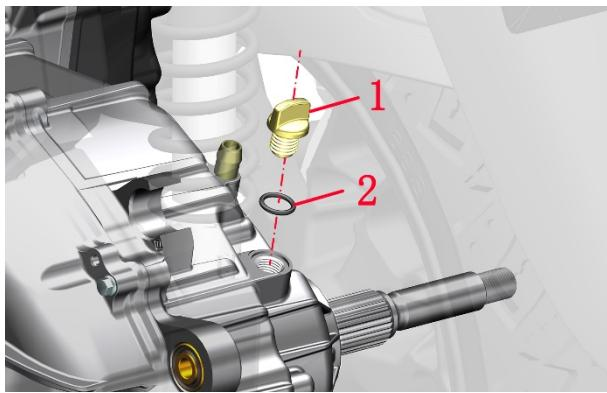
b. Place an oil drain pan under the rear of the left engine. For the ETC model, use a 10# socket; for the early 24 model, use a 14# socket, and the currently produced models use a 10# socket; loosen the oil drain bolt (3) counterclockwise.
