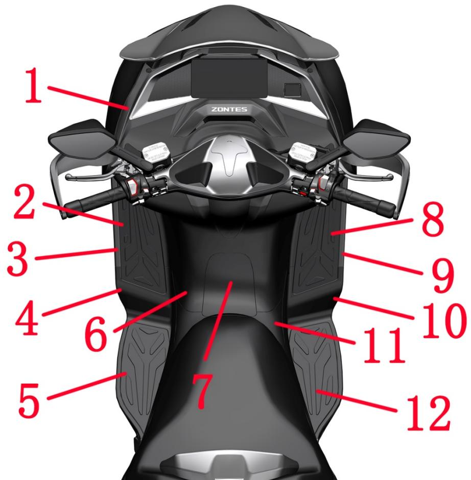
1.Front compartment panel front 2.Front left pedal pad 3.Left pedal decorative cover lining 4.Left pedal upper
