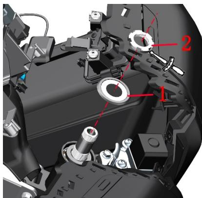
c. Ensure that the lower plate does not rotate and does not jam or loosen, and then put in the adjusting nut washer (3), the direction post adjusting nut (2), and the adjusting nut anti-loose washer (4) in turn. The nut only needs to be tightened and aligned with the first nut.
