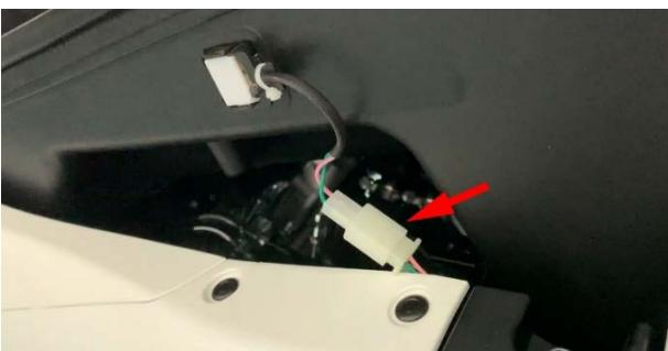
d.Unplug the plugs of stepper motor ① and sensor ②.
