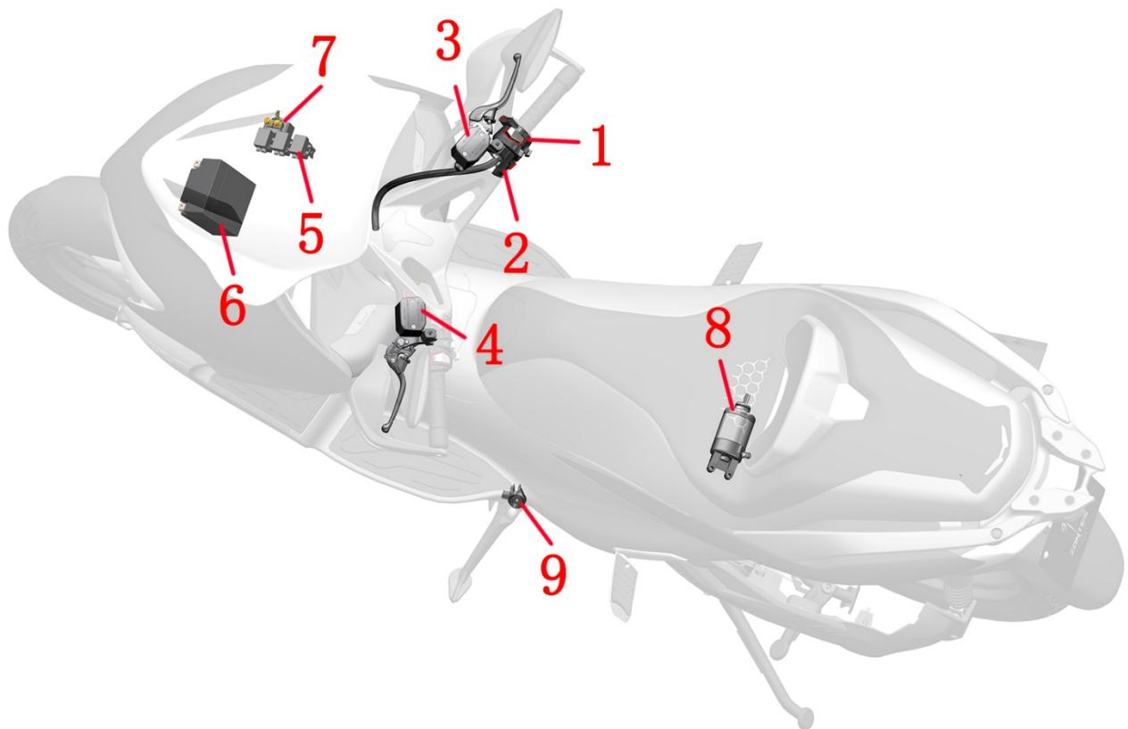
1- Right-hand handle switch (kill switch, start button) 2- Right hand handle sub switch (unlock vehicle)
