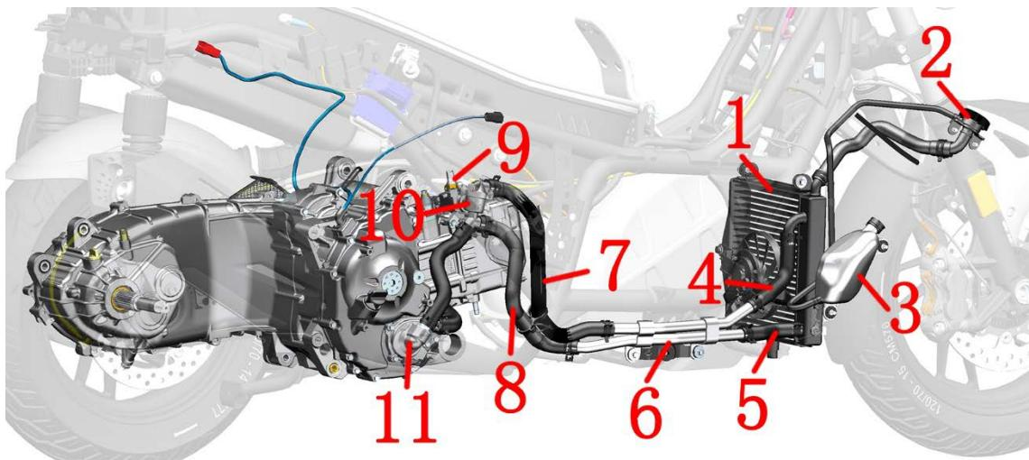
1-Main water tank 2-Water tank filling port 3-Auxiliary tank 4-Main tank inlet pipe 5-Main tank outlet pipe
