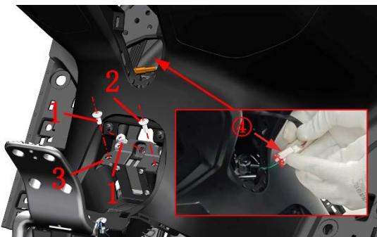
e.Use a T25 torx wrench to remove the 4 M6x14 shoulder bolts (1) of the box panel assembly, and then take out the box panel assembly.
