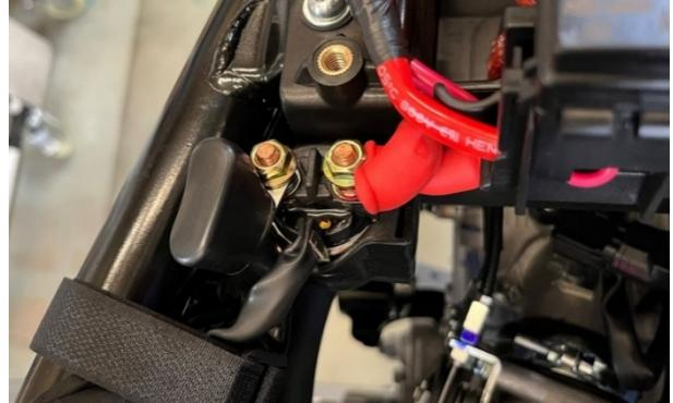
When reinstalling, ensure that the yellow/red and green/red wires of the relay correspond to the main wiring color codes. The nuts do not need to be differentiated. After tightening the nuts, make sure to cover the protective cap securely.
