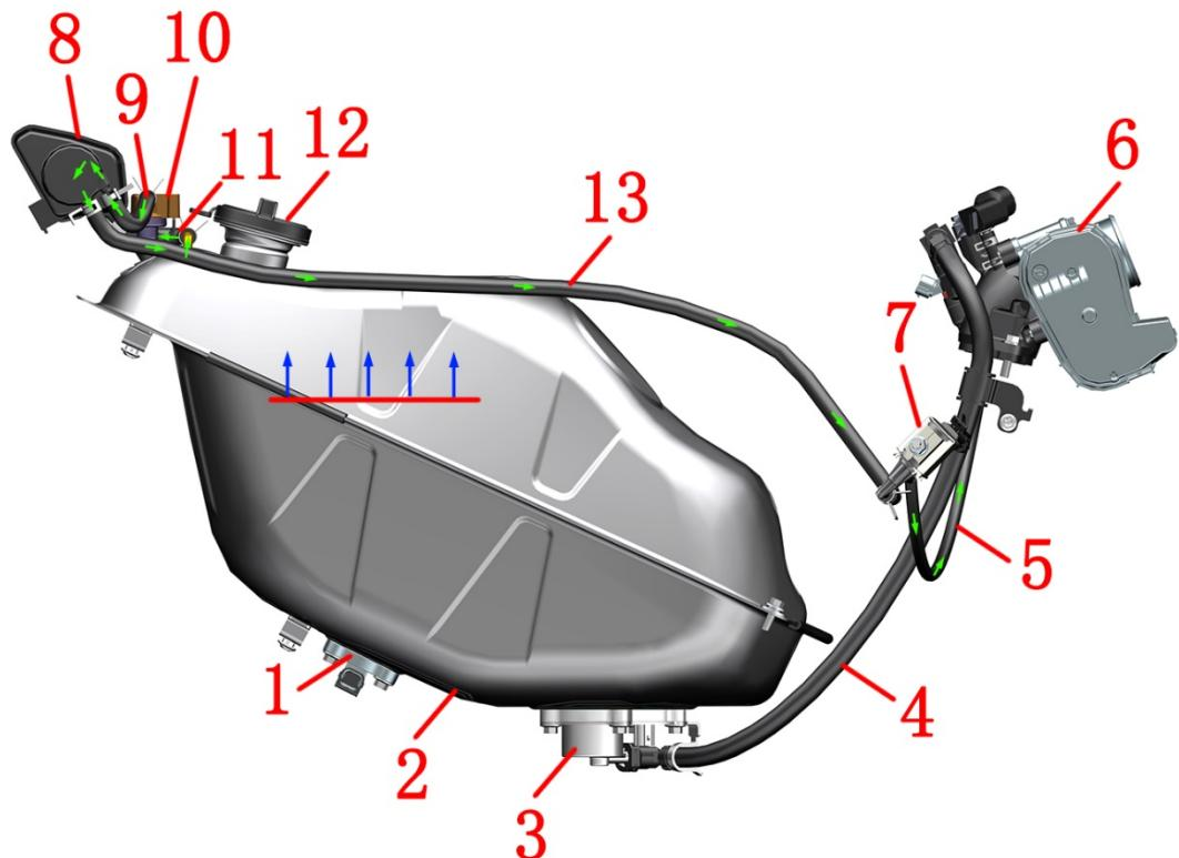
1-Oil level sensor 2-Fuel Tank 3-Fuel Pump 4-High-pressure oil pipe 5-Solenoid Valve Outlet Pipe
