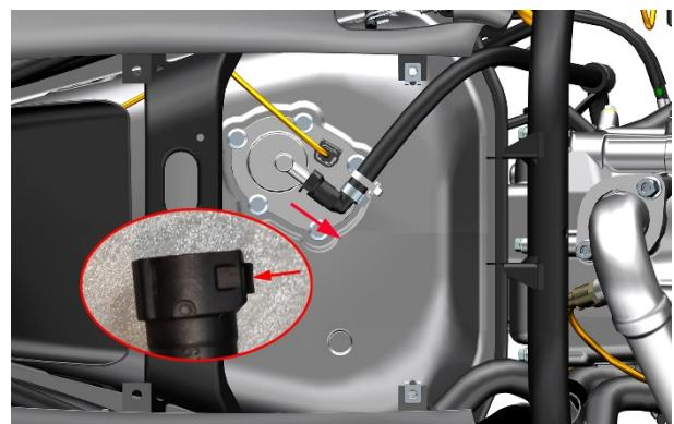
d. After pressing the anti-release lock at the fuel injector, pull out the high-pressure oil pipe in the direction of the arrow.
