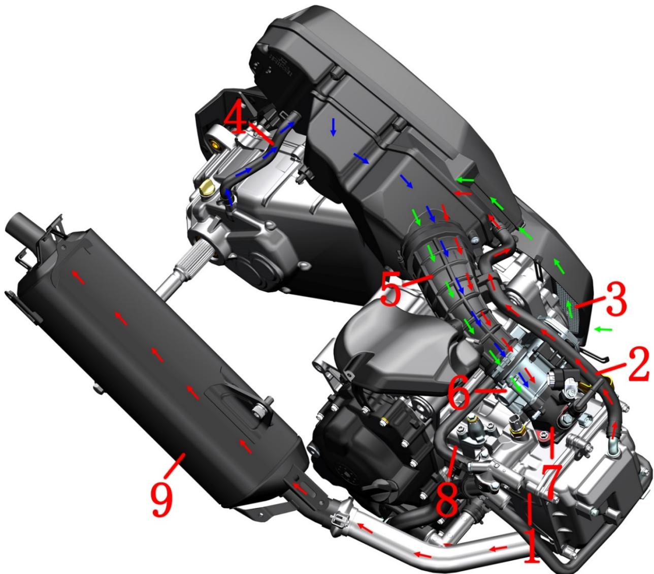
1-Cylinder Head 2-Cylinder Head Breather Pipe 3-Air Filter Inlet 4-Gearbox Breather Pipe 5-Air Filter Outlet Pipe
