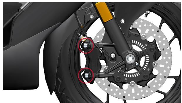
b. Place the oil pan under the front disc brake caliper. First uncover the rubber cap of the screw (1), put on waterproof gloves and remove the bolt (2) with an 8# torx wrench, remove the bolt (3) with a 14# torx wrench, and remove the two copper washers (4).
