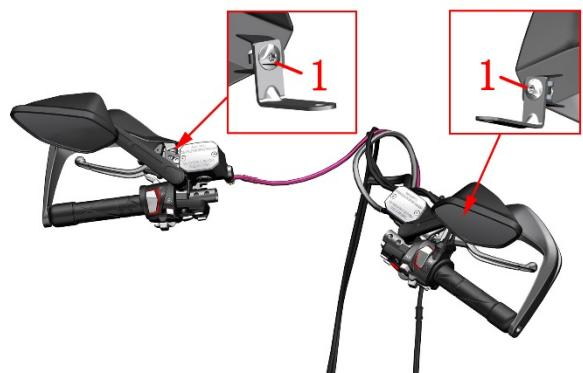
b. Use the 5# hexagon socket to loosen the balance weight bolt A for 5-8 turns, and remove the left and right hand guards and the balance weight assembly.
