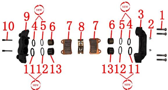
1-Bolt 2-Circlip 3-Caliper inner housing 4-φ30 oil seal 5-φ30 dust seal 6-φ30 piston 7-brake pad 8-brake pad spring 9-caliper outer housing 10-pin 11-φ34 oil seal 12-φ34 dust seal 13-φ34 piston
