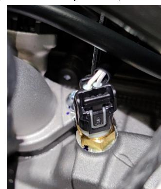
The resistance value of the two-pin room temperature of the multimeter is:  $1.5\sim4.0\text{k}\Omega$ .
