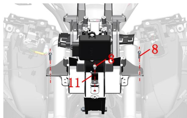
e. Use a T25 socket torx wrench to remove 3 M6×14 shaft shoulder bolts (2) and remove the wire box (12).
