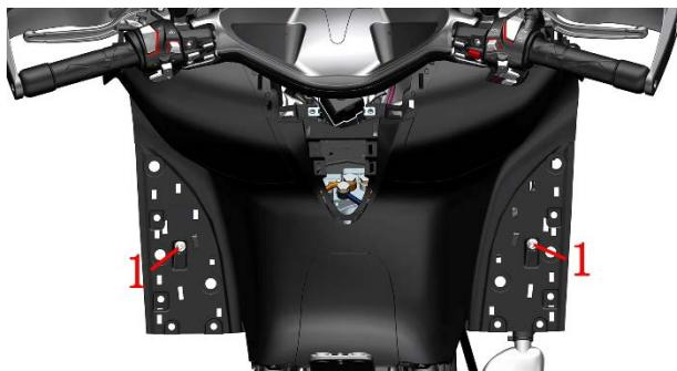
d.Turn on the battery, unlock the fuel tank cover lock and remove the fuel tank cover. Then use a T25 Torx wrench to remove the two M6x14 shoulder bolts (1) and M6x14 shoulder bolts (2) that hold the tank lock. Locate and unplug the tank lock harness connector (4), then remove the tank lock (3).
