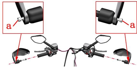
c. Use a 5# hexagon wrench to remove the four M6×30 bolts, then remove the left handlebar half cover, rear disc brake master cylinder, right handlebar half cover, and front disc brake master cylinder.
