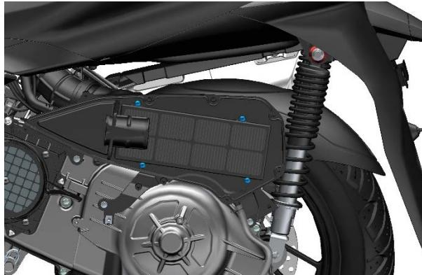
b. Remove the old air filter cartridge. Use a dust gun to blow the dust on the inside of the air intake pipe, and then wipe the inner wall clean with a clean non-woven fabric.
