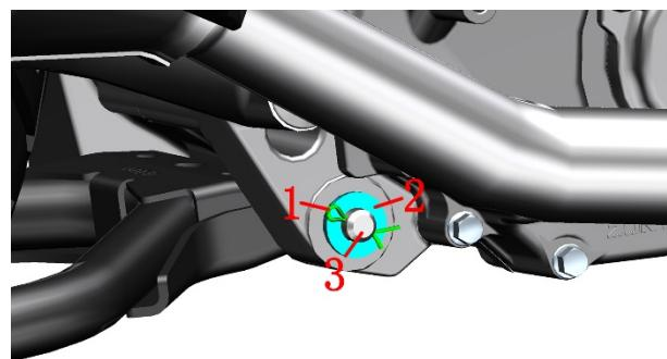
b.Remove the spring from the main bracket.
