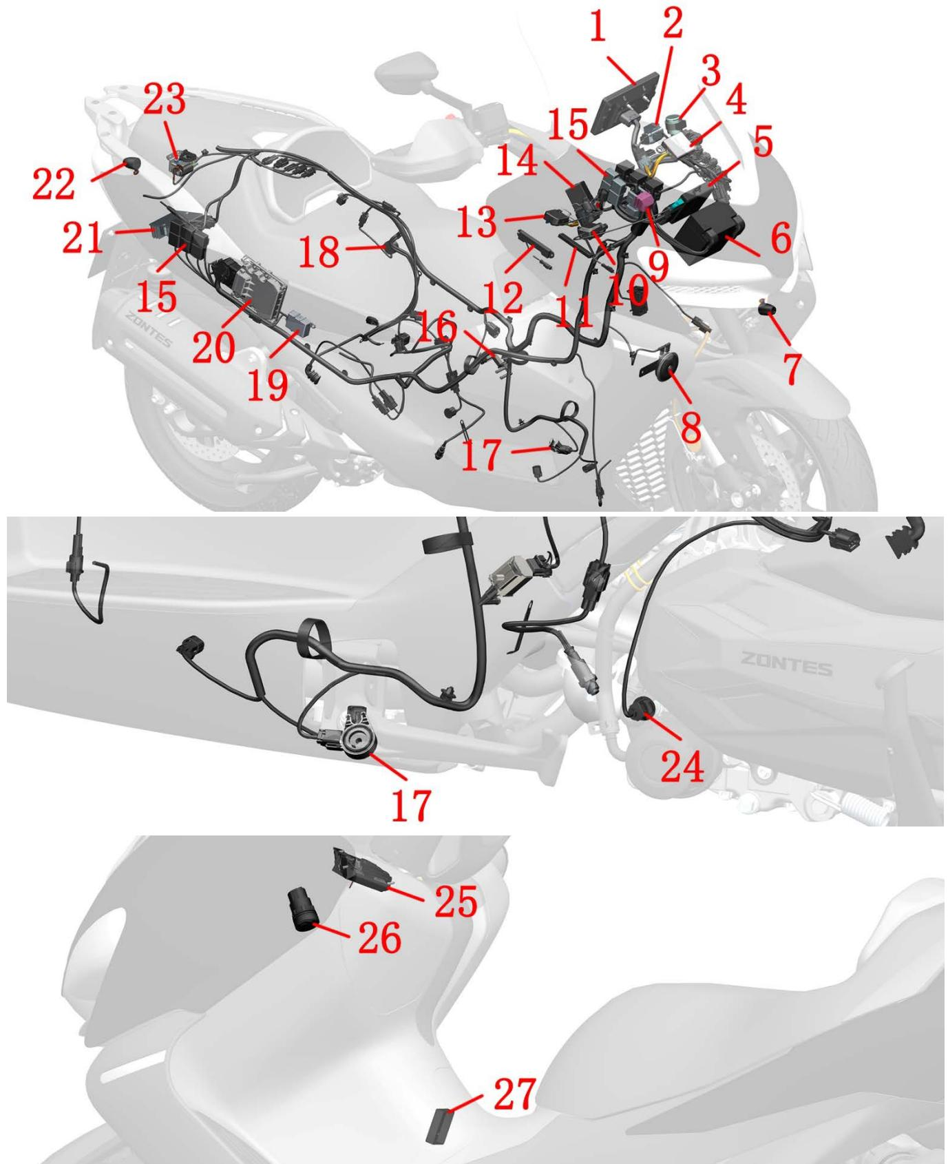
1-TFT Instrument 2-Tilt Switch 3-Flasher 4-Intelligent Control Box 5-PKE Main Unit 6-Lithium Battery 7-Front Camera
