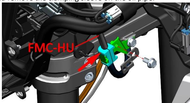
c. Remove the bolts that fix the tubing with a 10# sleeve, and remove the FMC-HU tubing and FC-HU tubing.
