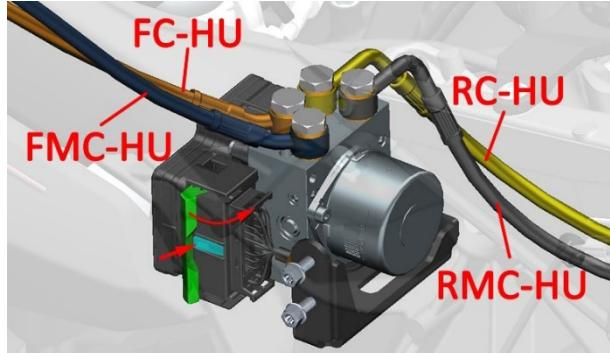
c. Use the 8# sleeve to remove the 2 bolts on the left side of the main frame, and remove the hydraulic control unit and bracket assembly from the motorcycle.
