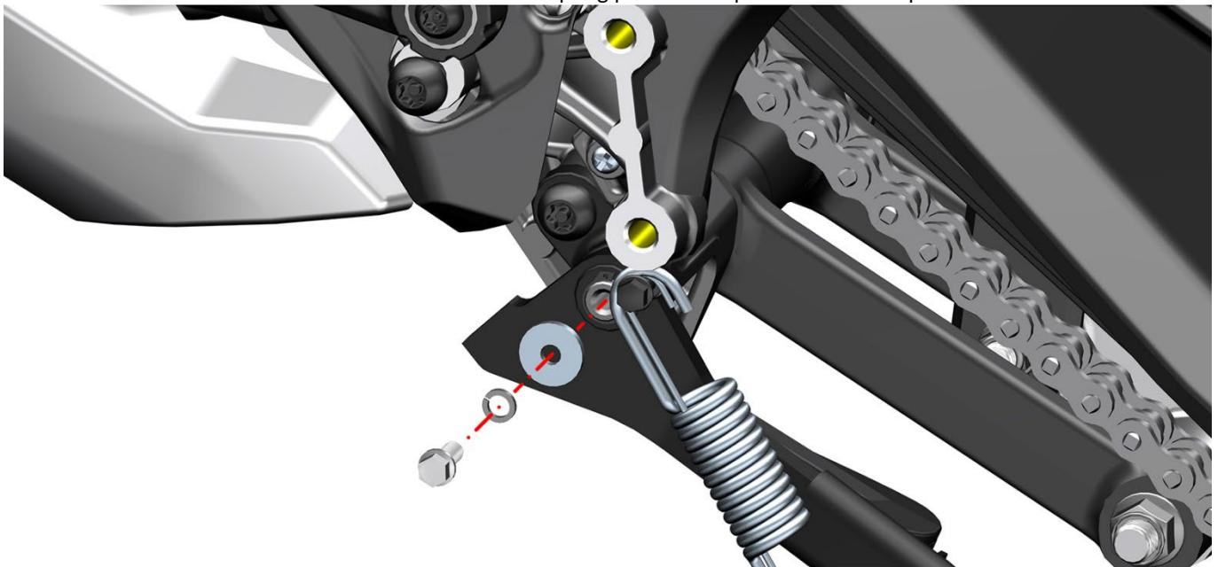
c. Refer to the method of removing the side bracket spring to remove the main bracket spring. After removing the bolt on the front of the main bracket (a) in a counterclockwise direction with a T50 plum blossom socket with holes, rotate the main bracket down until the other bolt is exposed (b in the figure). Standard torque:  $65\pm5$  N.m.
