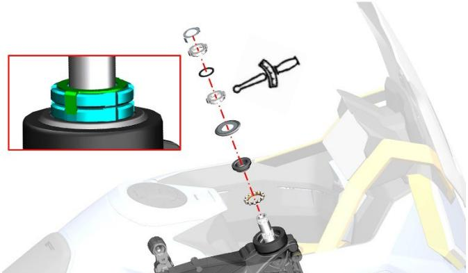
d. Install the cushion block and upper connecting plate, insert the gasket, and finally screw in the cap nut with a torque of 100N. m (10.2 kgf. m, 74 lbf. ft).
