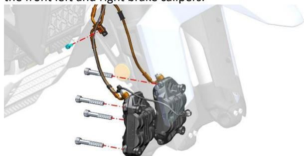
c. Use a T25 torx wrench to remove the 4 bolts on the left and right sides of the front fender (1); Then use the 5# hexagon to remove the 2 bolts (2) on both sides. Detach the tubing from the retaining clip in the rear left side of the fender.
