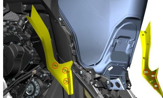
e. Use a 4# hexagon tool to remove 2 hexagon shoulder bolts (1). Standard torque for bolt (1): 6~8 N.m.
