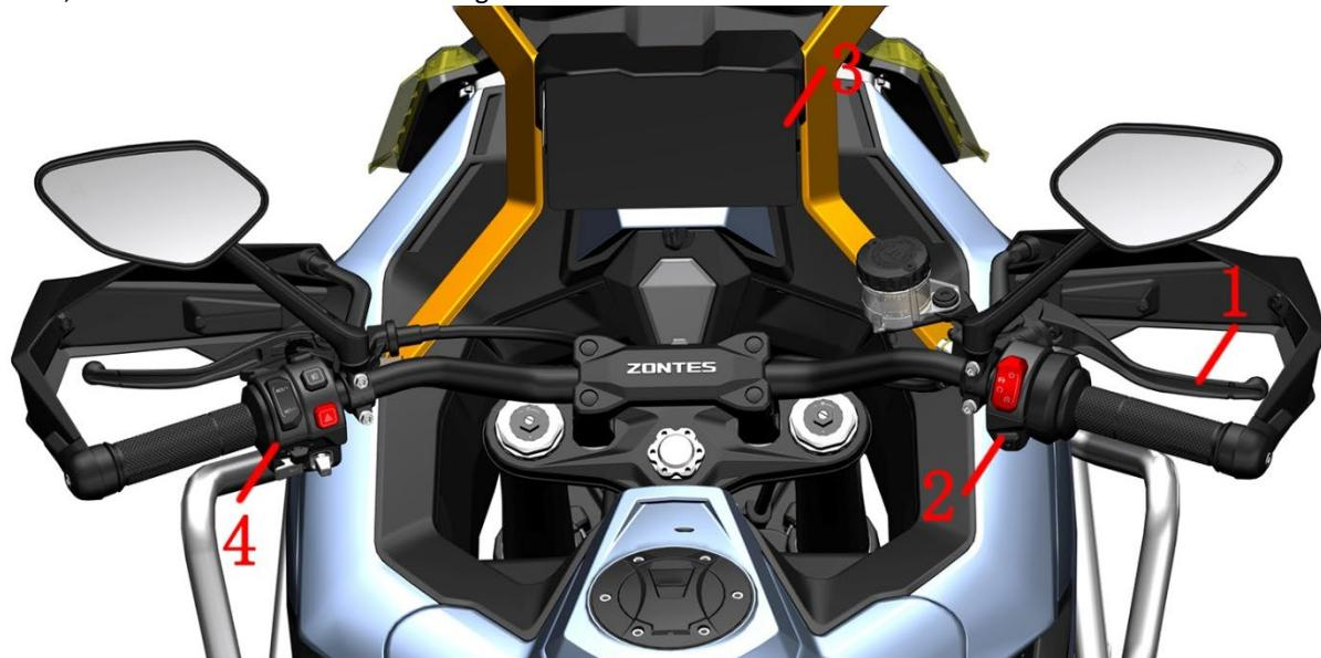
1. Front brake handle 2. Right hand handle switch 3. Meter 4. Left hand handle switch
