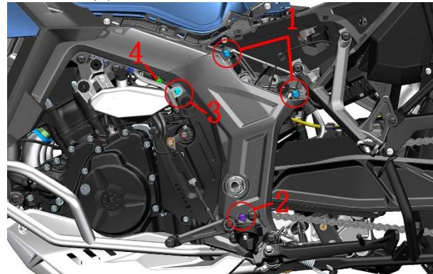
d. Use a T50 Torx socket with a mid-hole to remove the 3 M10×30 bolts. Lower the gear lever and front pedal stand.
