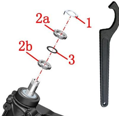
c. If the steering is heavy, loosen the adjusting nut (2b) anticlockwise. Tighten clockwise to 35 N.m (3.6 kgf.m, 26 lbf.ft), then 1/4 turn anticlockwise, then 13 N.m (1.3 kgf.m, 10 lbf.ft).
