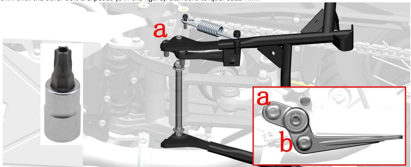
d. Use the external circlip pliers to remove the circlips on both sides.
