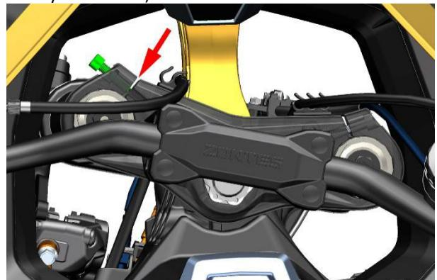
b. Use the 6# hexagon socket to loosen the bolts of 4 M8×35 for 5-8 turns, pry open the gap on the lower plate with a flathead screwdriver (as shown in the arrow), and remove the left front shock absorber and right front shock absorber.
