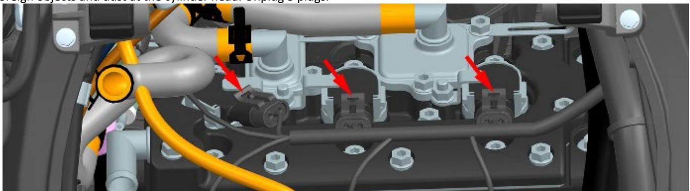
Remove the nut with a 10# sleeve and remove the ignition coil pressing plate. Remove the ignition coil. Use the 14# sleeve to remove the spark plug. If the fit is tight, you can shake it slightly from side to side to take out the ignition coil.
