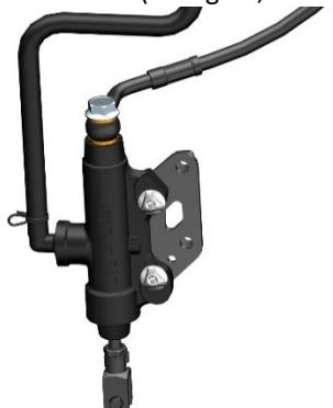
c. Use a Phillips screwdriver to remove the expansion pegs that hold the rear brake oil cup in place.
