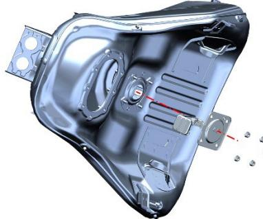
When reassembling, it is necessary to pre-tighten diagonally and then tighten 4 bolts, otherwise the sealing rubber ring of the fuel level sensor is compressed unevenly, which will easily lead to leakage and cause potential safety hazards.
