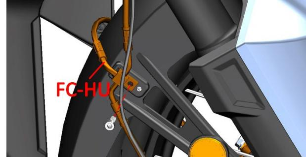
e. Untie the two oil pipes on the inside of the left frame and pull the two oil pipes out of the front.
