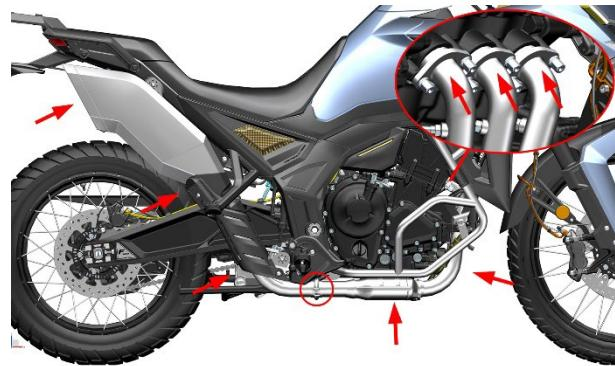
b. If there is a slight air leakage at the connection between the engine and the muffler, you can first try to tighten the exhaust nut (3) with 6# hexagon socket; standard torque:  $25\pm1.5$ . If the problem is not resolved, the muffler needs to be removed and replaced with a new engine exhaust gasket (4). The specific disassembly method can refer to the disassembly of the muffler.
