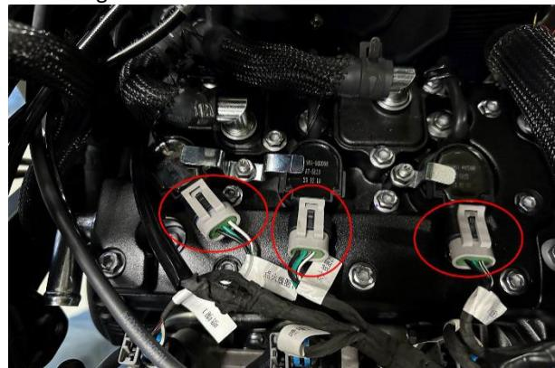
d. Use a 10# sleeve to remove 2 ignition coil pressure plates, and take out 3 ignition coils. The standard torque for the nut is 12 N.m.
