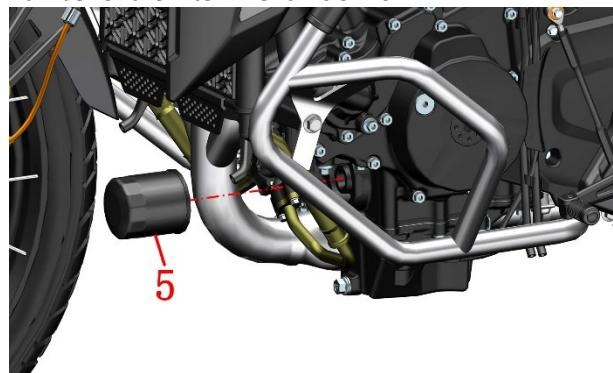
b. Drain the oil from the filter.
