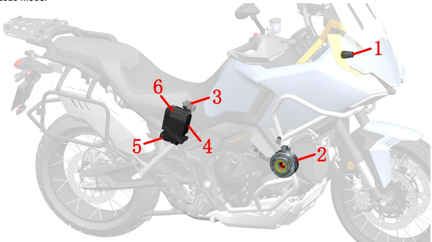
1 - USB Charger (Type-C) 2 - Magneto 3 - Starter Relay (40A) 4 - Battery 5 - Rectifier 6 - Fuse Box
