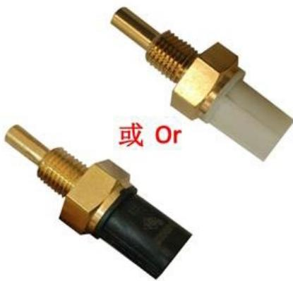
The water and oil share sensor is located in the middle cylinder position of the engine, and the two-pin resistance of the sensor is detected after the plug is removed. The auxiliary tank needs to be removed and then remove the water and oil share sensor. Pinch the top of the plug first, press the anti-disconnection card, and then pull the plug outward.
