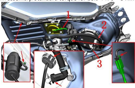
i. Refer to the steps of removing the air filter, remove the air filter first, press the anti-release lock in the direction of the arrow, and then pull out the high-pressure fuel pipe. After replacing the high-pressure fuel pipe with a new one, follow the disassembly steps to restore.
