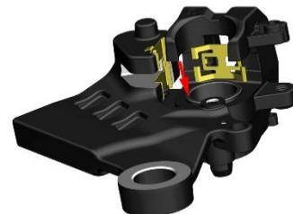
c. Grasp the outer brake pad with the left hand, insert the pin ② with the right hand, and be careful not to insert it to the end. After the inner brake pad is put in place, insert the pin shaft to the end and lock the pin ② with a T25 torx wrench, and replace the circlip ① with needle-nose pliers. Note that the side with grooves is facing the brake disc; The black metal back panel faces the calipers. Standard torque is 17 N.m.
