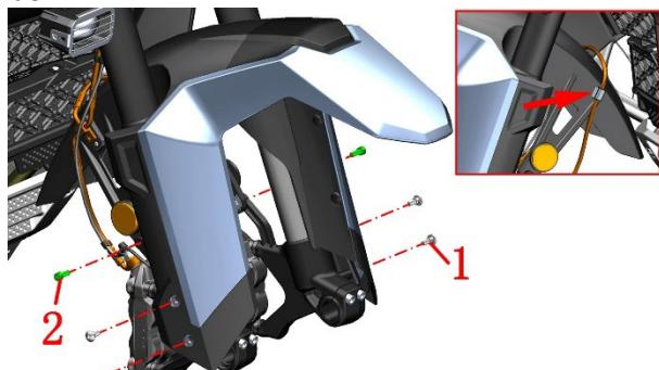
d. After moving the front mud board up to the appropriate part, pull it out in the direction of the big arrow. Remove the bolt on the wheel speed sensor with a T25 Torx wrench and remove the sensor. Remove the front right brake caliper.
