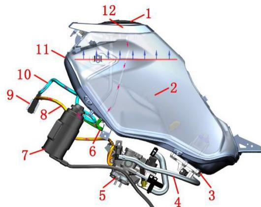
1-Fuel Tank Lock 2-Fuel Level Sensor 3-Fuel Pump 4-High Pressure Fuel Hose 5-Throttle Valve Body Assembly 6-Adsorption/Snorkel 7-Carbon Canister 8-Solenoid Valve Outlet Pipe 9-Carbon Canister Solenoid Valve 10-Solenoid Valve Intake Pipe 11-Fuel Tank 12-Air- Fuel Separator (Inside Tank Lock)
