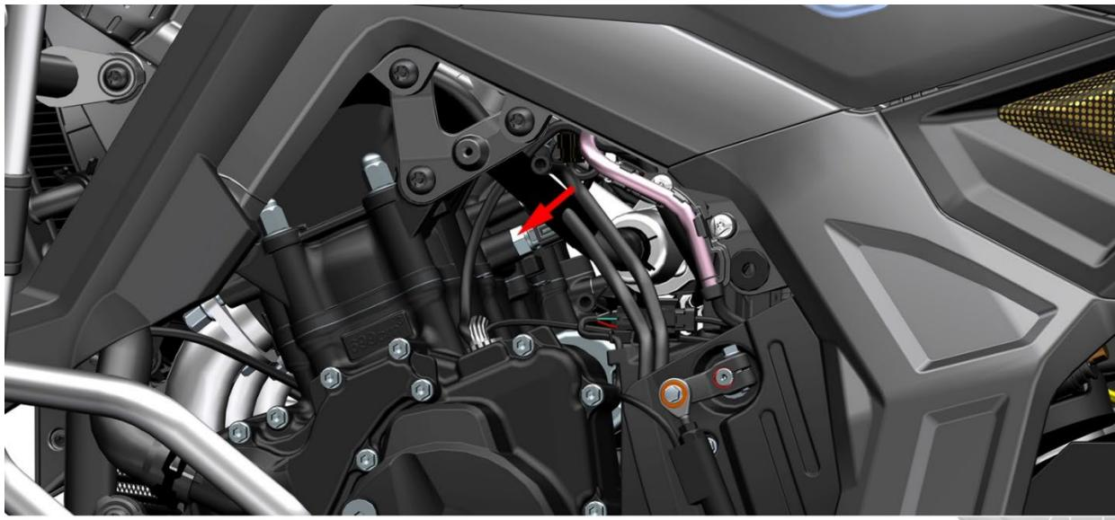
Use a multimeter with two pins of room temperature resistance values:  $3.74 \sim 1.22\text{k}\Omega$  ( $10 \sim 40^\circ\text{C}$ ) ;  $1.22 \sim 0.27\text{k}\Omega$  ( $40 \sim 90^\circ\text{C}$ ) .
