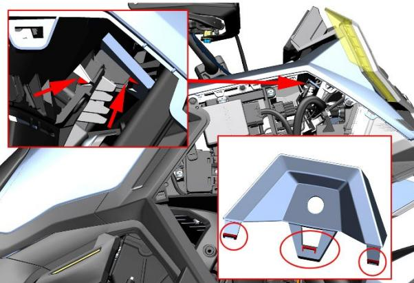
c. Remove the meter assembly
