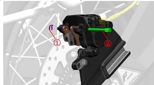
b. With the help of a tool, push the piston in the direction of the arrow to the end. If the resistance is very large, you can refer to the method of adding brake fluid to the front brake main cylinder, remove the upper cover and then push it. If the spring blade on the caliper falls off, it needs to be replaced in the direction shown.
