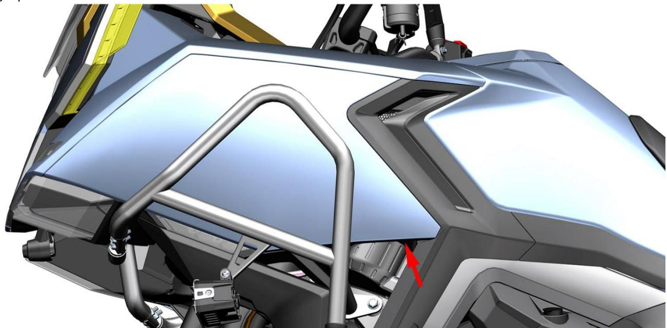
Use a Phillips screwdriver with a diameter of 6mm and a length of 150~200mm to align the sawtooth of the dimming bolt, rotate it counterclockwise to turn it down, and turn it clockwise to turn it up.
