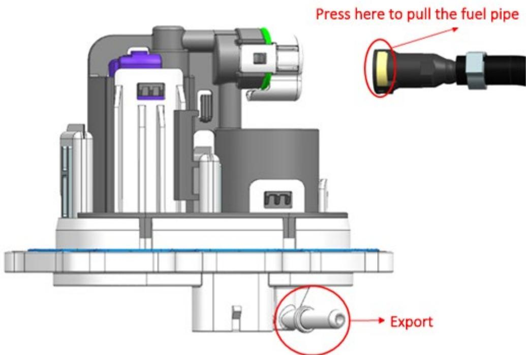
If the fuel pump needs to be removed from the vehicle, the fuel tank can be emptied with a suction pump. Flip the fuel tank assembly to the back and remove the 9 bolts with the 10# or 8# (some vehicles produced from the end of June to the end of August 2025) sleeve to remove the fuel pump.
