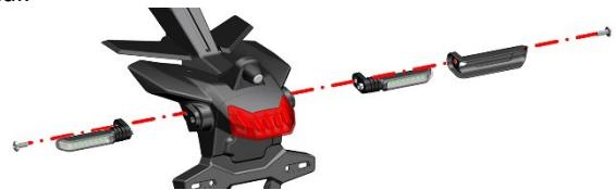
e. First, use the 4# hexagon to remove 2 M6×14 inner torx shoulder screws and 1 M6×17.5 inner torx shoulder screw, then slowly pull out the rear fender bracket cover, and remove the splint M6×11.
