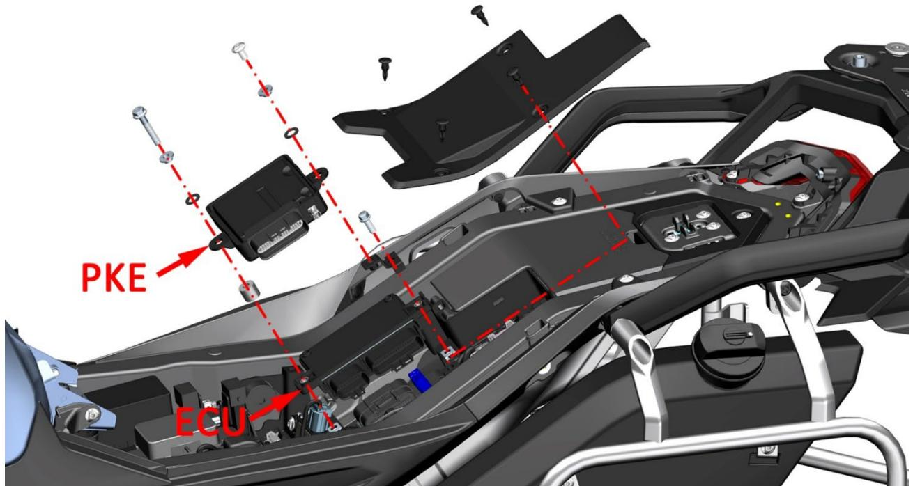
Note: To replace the ECU, you need to shut down the whole vehicle and wait for 10 seconds before operating to avoid the abnormality of the EFI system.
