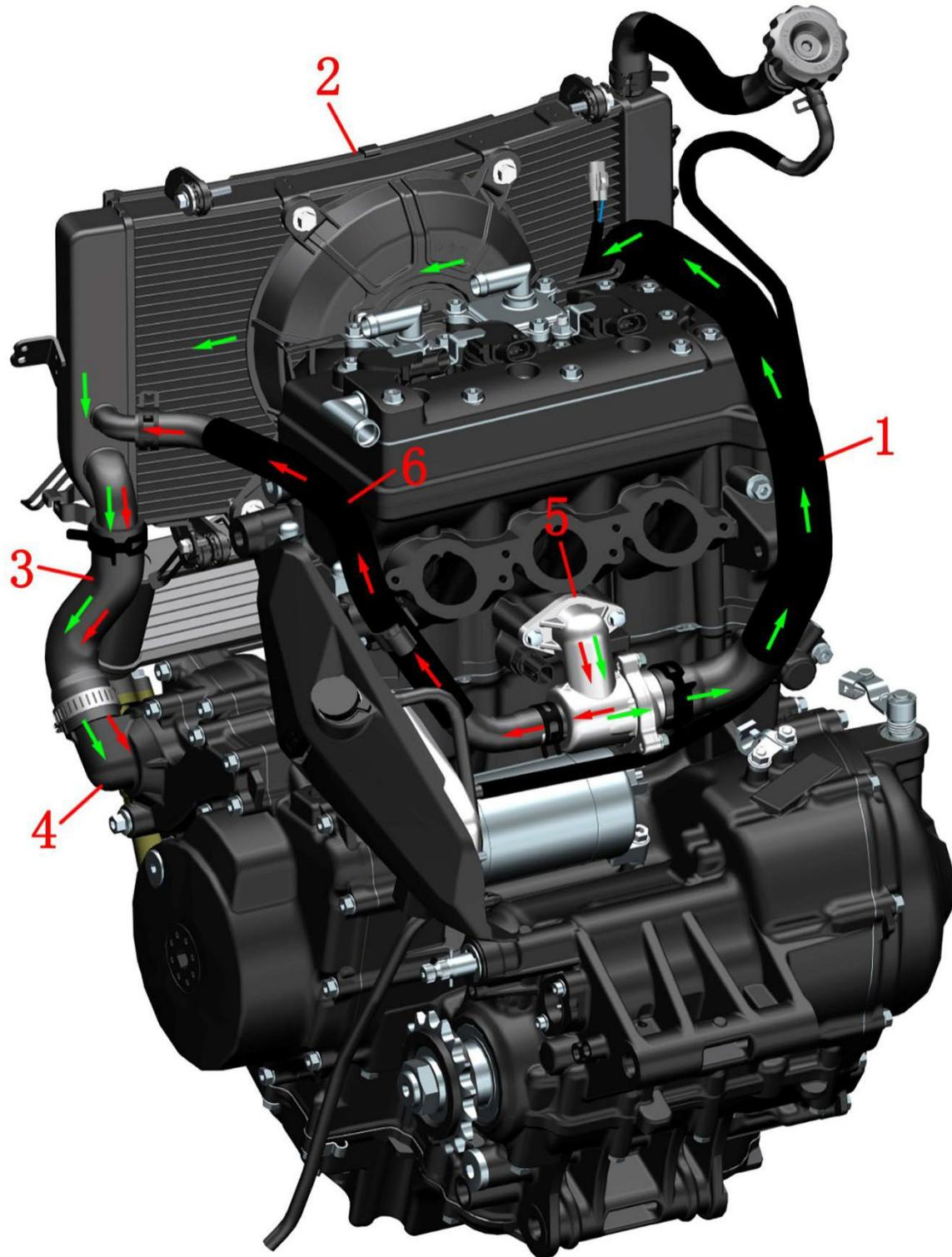
1-Main water tank inlet pipe 2-Main water tank 3-Engine water inlet pipe 4-Water pump assembly 5-Thermostat assembly 6-Small circulation water pipe
