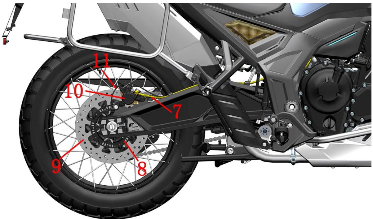
1- Brake disc assembly (front right) 2-Disc brake caliper (front right) 3-FC-HU brake hose 4-Wheel speed sensor ( front wheel ) 5-Disc brake caliper (front left) 6-Brake disc assembly (front left) 7-RC-HU brake hose 8 - Rear wheel A BS induction coil 9 -Brake disc (rear) 10-Rear disc brake caliper 11-Wheel speed sensor (rear wheel)
