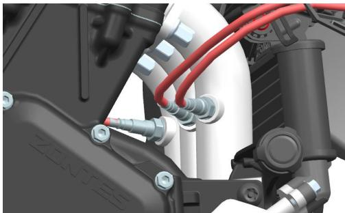
The new sensor threads are coated with a special paste thread anti-sintering agent to prevent air leakage and facilitate subsequent re-disassembly. If the old inspection is fine, it is necessary to apply an appropriate amount of anti-sintering agent to the thread before installation.
