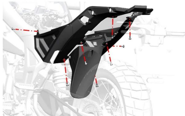
b. Use the 4# hexagon to remove the 3 M6×14 inner torx shaft shoulder screws fixed on the inner mud board, and then remove the inner mud board.
