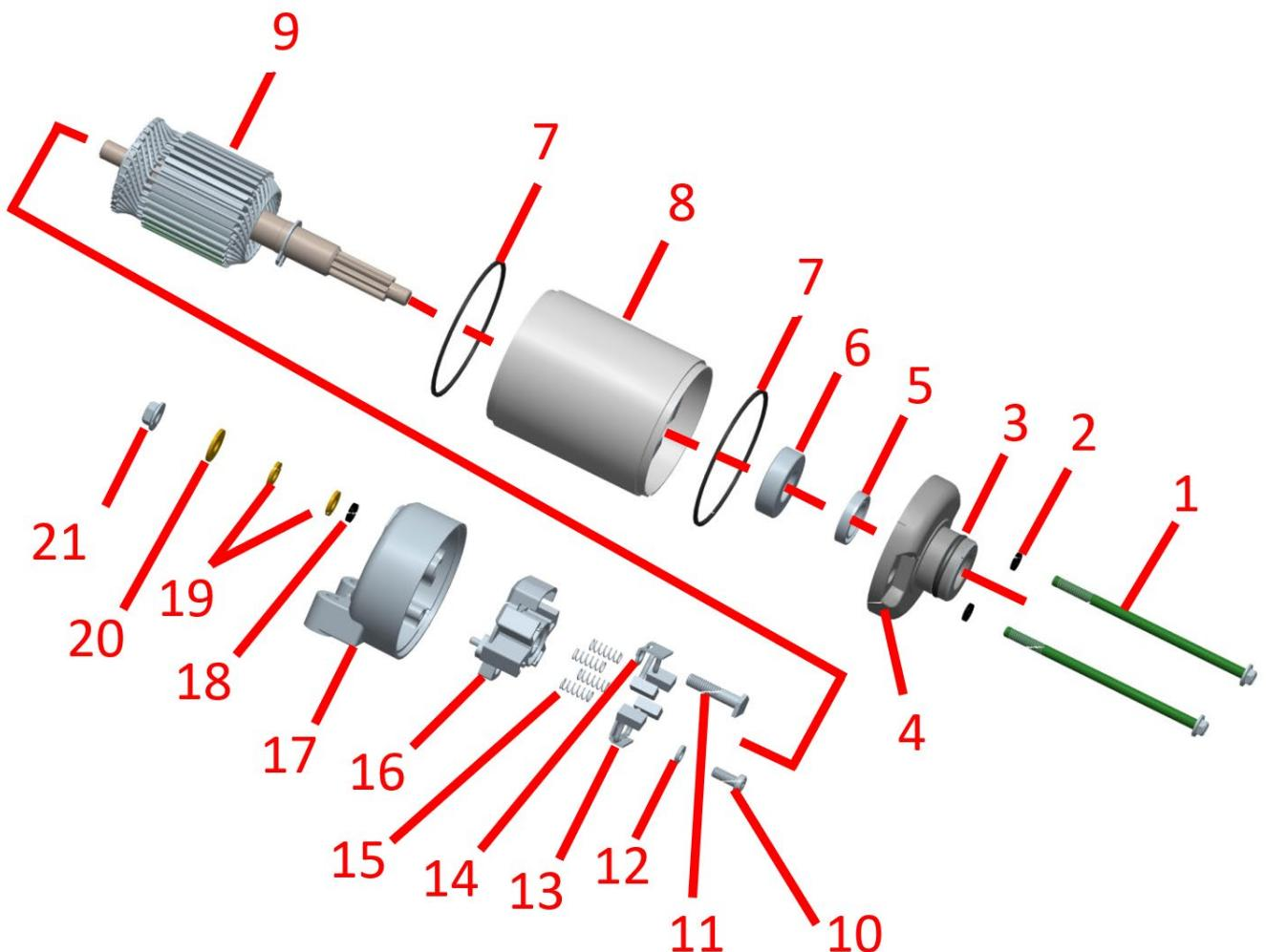
1-M5×98 bolt×2 2-O ring×2 3-O ring 4-starter motor front cover 5-oil seal 6-bearing 7-rectangular sealing ring 8-starter motor outer shell 7-rectangular sealing ring 9-electric pestle 10-screw ×2 11-head screw with limit 12-washer 13-negative brush×2 14-positive brush×2 15-worm spring ×4 16-insulating brush frame 17-starter motor back cover 18-sealing rubber ring 19-insulating gasket 20 anti-loosening gasket 21 nut
