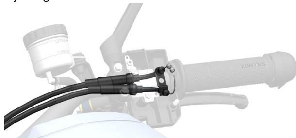
c. If the fault of high resistance cannot be solved after lubrication, the throttle cable needs to be replaced.
