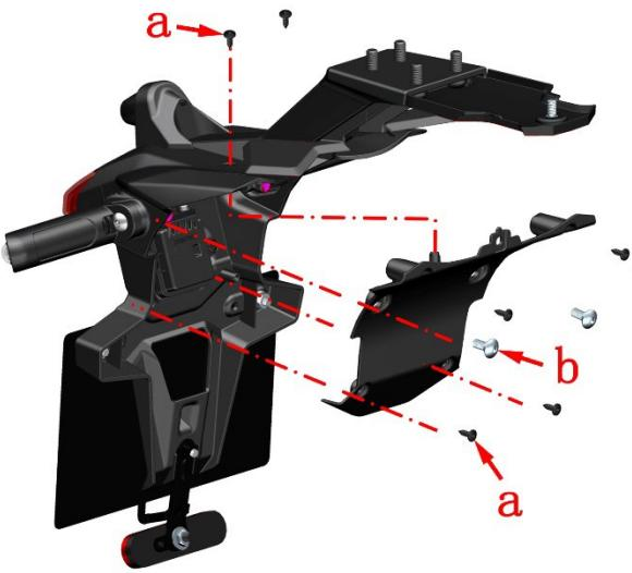
b. Use a Phillips screwdriver to remove the two self-tapping screws that fix the blind zone radar, loosen the blind zone radar and the plug interface, and pull out the blind zone radar.
