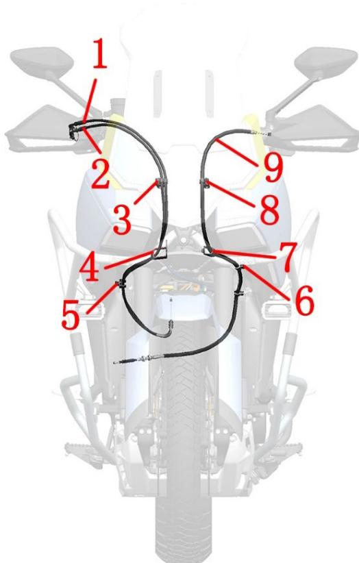
1- Refueling line 2- Oil return line 3-Right handlebar wiring bracket 4- Throttle cable limit bracket 5 - Throttle cable clamp 6 - Clutch cable clamp 7-Clutch cable limit bracket 8-Left handlebar wiring bracket 9-Clutch cable
