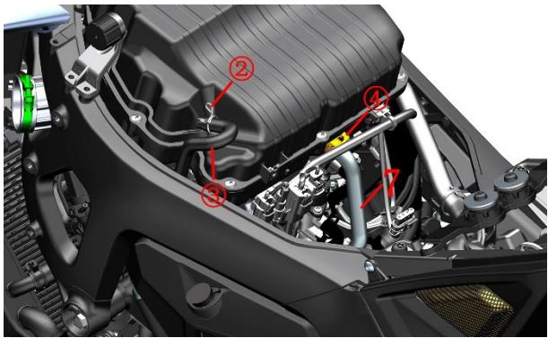
c. Lift the air filter slightly, use the hoop clamp to remove the hoop (5) on the rubber pipe (8) of the air supply valve, and the air filter housing can be taken out after removing the rubber pipe of the air supply valve.
