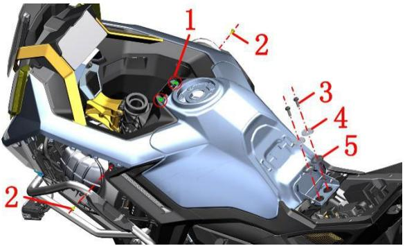
d. After pulling out the three buckles of the left and right fuel tank decorative covers, remove the left and right fuel tank decorative covers respectively.
