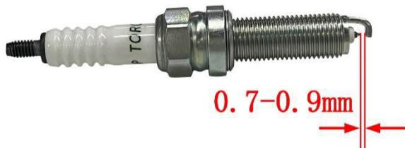
d. If necessary, the gap can be adjusted by bending the side electrode, and pay attention to the strength when adjusting.
