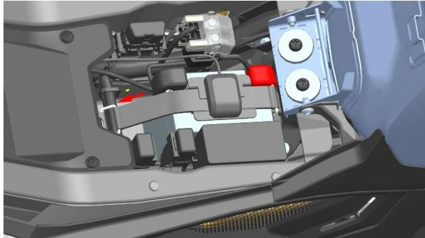
b. Pull out the black protective cap of the negative electrode first, and remove the negative electrode first. Then disassemble the positive electrode. Remove the battery.
