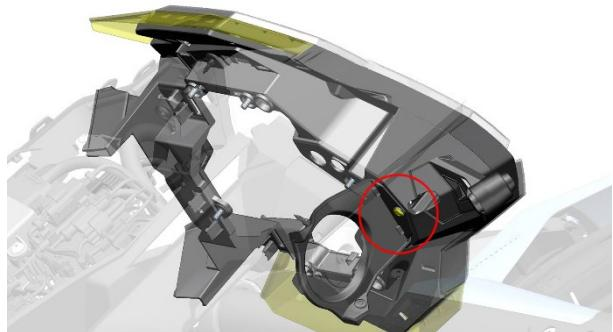
c. Remove all switch connectors from the head lining, unplug the connectors of all position lights and cameras, and remove the head liner assembly.
