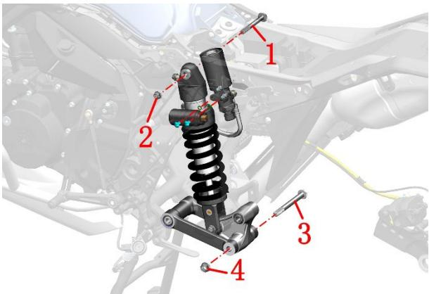
b. One person fixes the head of the bolt with a 14# sleeve, and one person uses a 14# sleeve to remove the nut, remove the bolt, and remove the rear shock absorber and triangle bar assembly. Nut torque:  $65\pm5\text{N.m}$  ( $6.6\pm0.5\text{ kgf.m}$ ,  $48\pm4\text{ lbf.ft}$ ).
