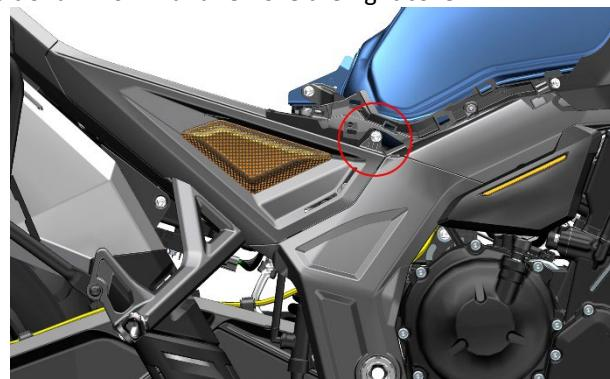
c. Unplug the decorative cover of the charging port seat, use the T25 plum blossom hexagon to remove 1 M6×12 bolt (1), 1 M6×14 shoulder bolt (2), 2 M6×16 bolts (3), remove the right side cover of the frame, and pay attention to bumping the engine guard plate when removing.
