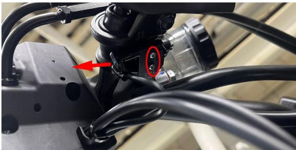
a. Pull out the two plugs of the front brake switch in the direction of the arrow, without distinguishing between the positive and negative poles.
