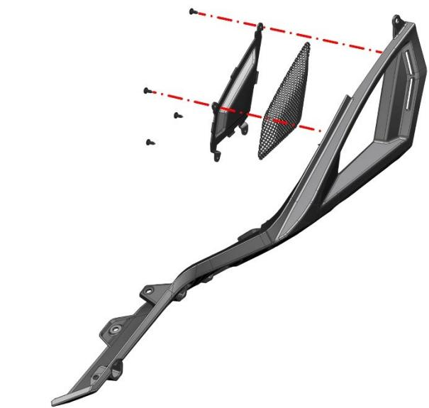
f. Remove the expansion nail fixed on the right tail skirt and the right cover, and then remove the right cover.
