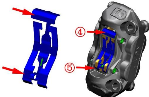
J. hold down the piece at the point of the arrow ④ to the direction of the arrow with the hand, and insert the pin ② into the hole position to fix the brake pad (1). Tighten the pin ② with a T25 hexagon torx wrench. Standard torque is 17 N.m.
