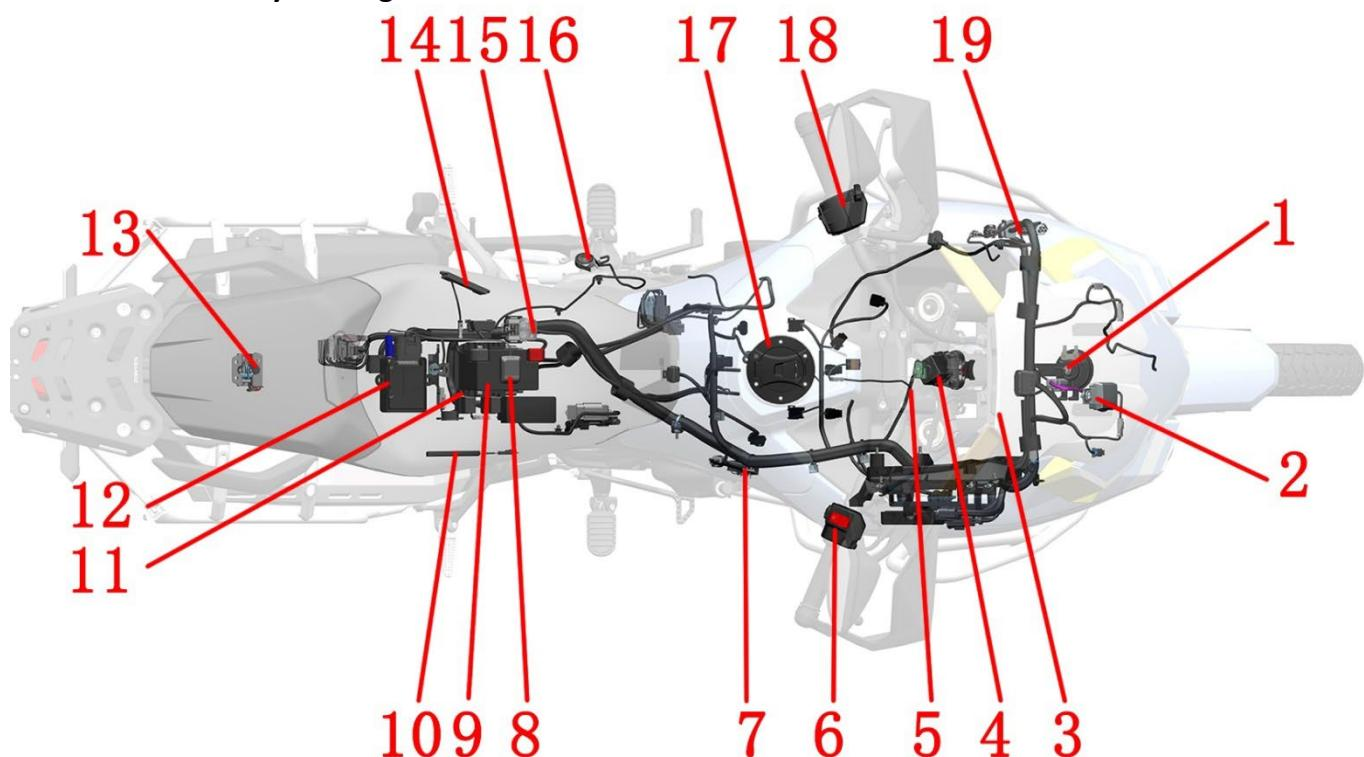
1-Horn 2-Windshield motor controller 3-TFT meter, 4-Faucet lock, 5-Canister solenoid valve, 6-Right hand handle switch, 7-Charging port base, 8-GPS antenna, 9-Lithium battery, 10- PKE antenna, 11-Rectifier, 12-PKE host, 13-Cushion lock, 14-Non-electric induction antenna, 15-Starting relay, 16-Side bracket flame-out switch, 17-Fuel tank lock, 18-Left handle switch, 19-Main cable
