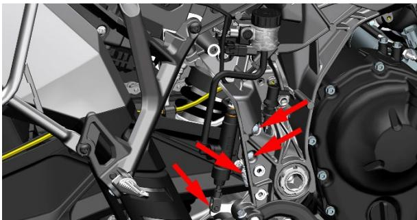
b. Use a T25 torx wrench to remove the two bolts on the rear brake switch bracket, wear waterproof gloves and use a 12# sleeve to remove the disc brake oil pipe bolts, remove the copper pad and remove the RMC-HU oil pipe, and pour out the brake fluid in the main cylinder. Standard torque of disc brake hose bolts: 32 N.m (3.3 kgf.m, 24 lbf.ft).
