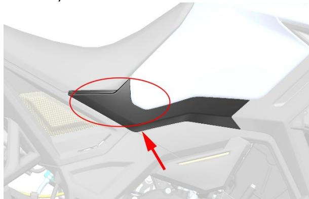
b. Use T25 plum blossom hexagon left and right surrounds to remove two M6×14 shaft shoulder bolts, bolts, and 1 expansion nail.
