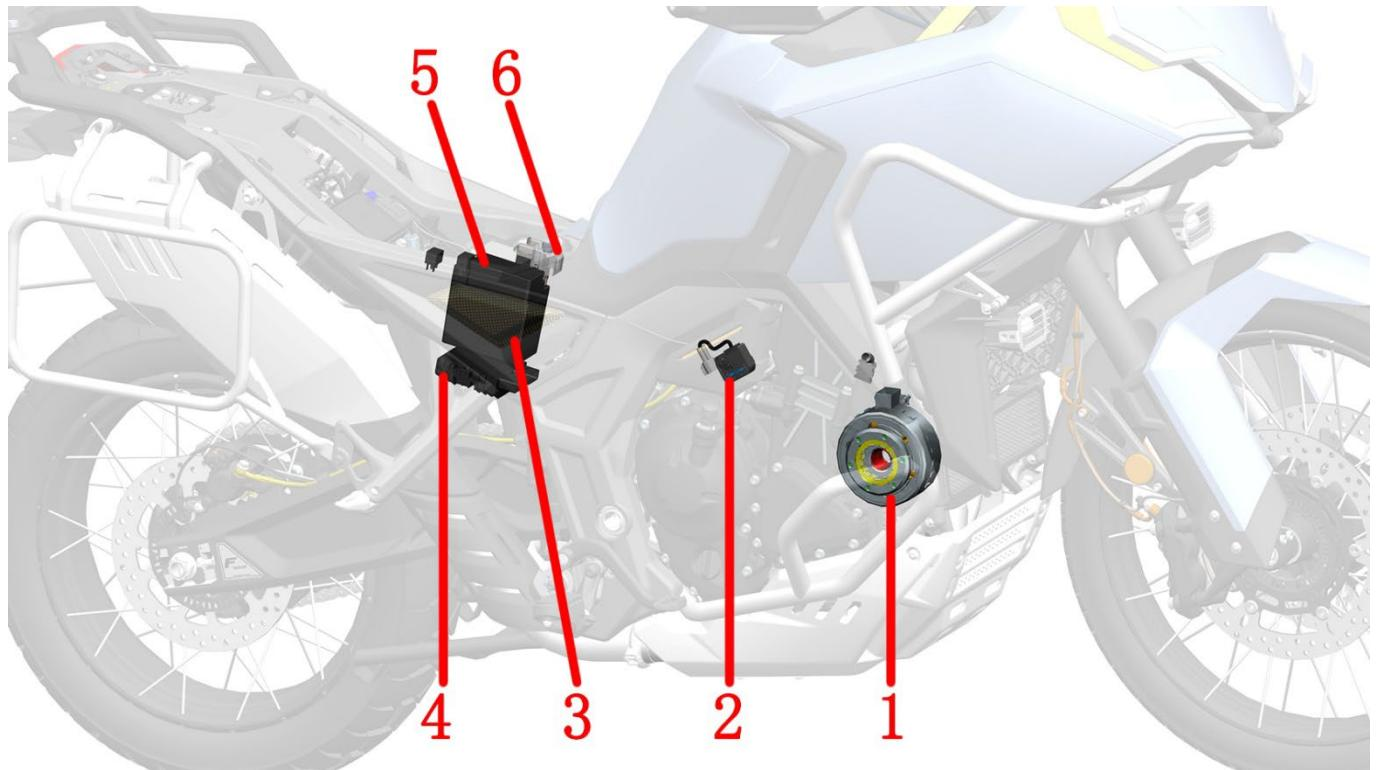
1-Magneto 2-Charging port base 3-accumulator 4-rectifier 5-Fuse box 6-Starting relay (40A)
