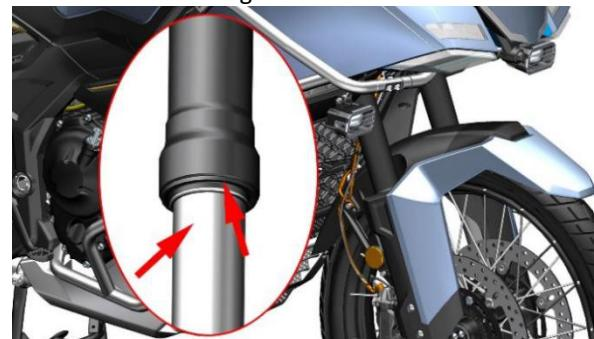
b. Check whether the bottom barrel is peeling off the paint, and whether the mounting points of the front fender, front wheel hollow shaft and front brake caliper are broken or cracked. Check the bottom of the bottom barrel for leaks.
