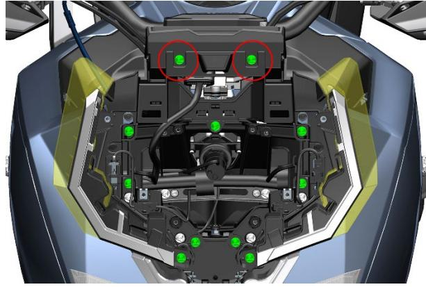
b. After removing the left and right sides of the surrounding, push the buckle of the bottom trim of the instrument from the gap.
