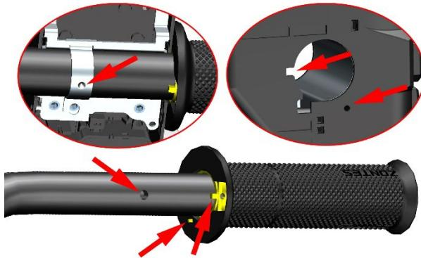
c. When installing the front disc brake half cover or clutch rocker arm half cover, align the joint surface of the half cover and the disc brake master cylinder or the half cover and the clutch rocker arm with the round hole on the handlebar, and then use an 8# sleeve to tighten the bolts. Note that you need to tighten the top bolts first, then tighten the bottom.
