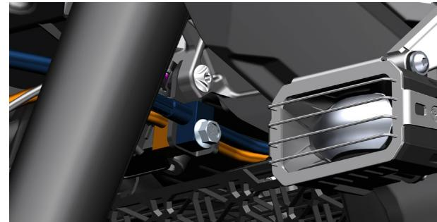
d. Remove the bolts that hold the tubing with 5# hexagon socket and loosen the FC-HU tubing.
