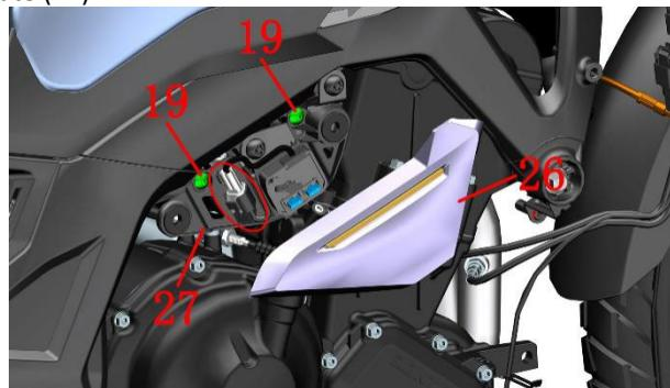
e. After tidying up the wiring harness, use the hoop pliers to remove the  $\phi 36$  hoop (28) connecting the thermostat (25) from the gap removed from the charging port base, and then grab one end of the main water tank water inlet pipe (15) to pull out the main water tank water inlet pipe (15).
