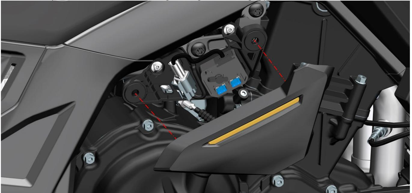
Remove the rubber plug and insert the DC plug of the charger that comes standard with the original factory. Then plug the AC socket into a 110-220V power supply. If the battery is damaged by using an inferior charger, it is not within the scope of the three guarantees.
