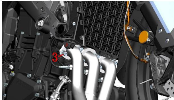
g. Use a T50 wrench with a center hole (for some early-produced vehicles) or a 14# socket to remove bolt (7), and a T45 wrench to remove bolt (8). Remove the muffler. Note: When removing bolts (7) and (8), support the front of the muffler; when completely removing them, ensure that the engine exhaust port gasket (4) at the connection between the muffler and the engine is not left behind. The standard torque for bolt (7):  $65 \pm 5$  N.m. The standard torque for bolt (8):  $25 \pm 3$  N.m.
