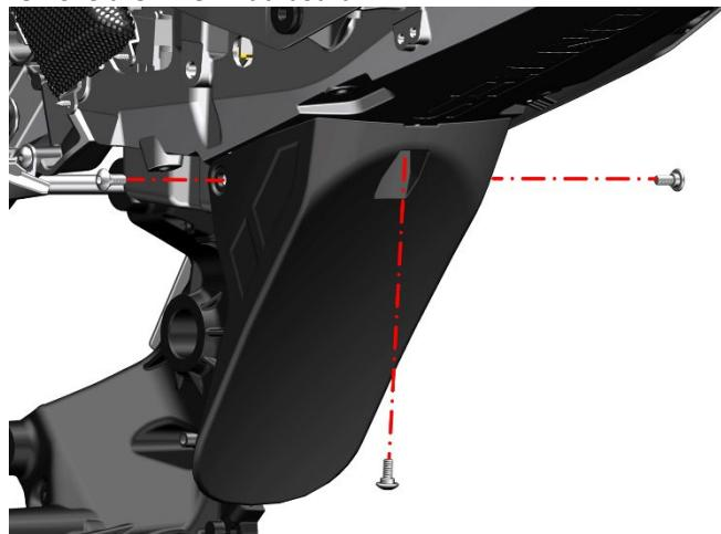
c. First, use the 4# hexagon to remove the 2 M6×14 inner torx shaft shoulder screws fixed on the upper part of the tail group. Then grasp the A and B parts of the right tail group components and gradually pull out the components along the
