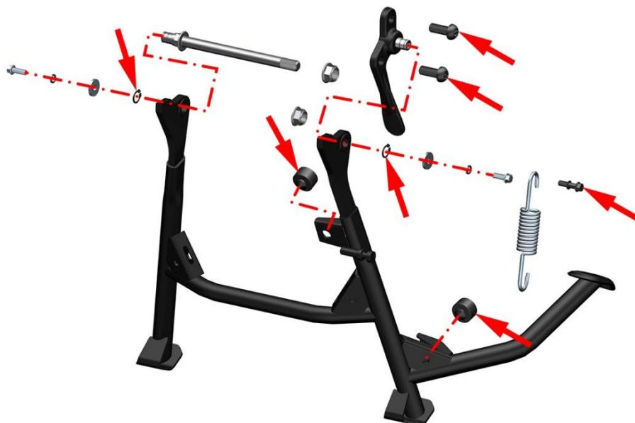
Inspect the parts indicated by the arrows in the picture above, and the disassembly method is detailed below.
