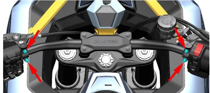
b. Buckle down the 4 decorative buckles on the pressure block, use 6# hexagon socket to remove the 4 bolts, remove the pressure block, and pick up the handlebar.
