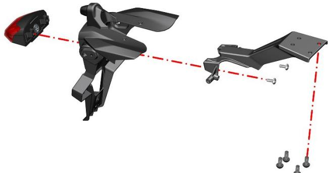
g. First, use a Phillips screwdriver to remove the bottom 2 self-tapping screws, pull out the upper part of the rear camera decorative cover from the buckle, use a Phillips screwdriver to remove the camera clamp matching bolts and its spacers, then pull out the camera interface and arrange the wiring harness, and then take out the rear camera and the lower part of the rear camera decorative cover.
