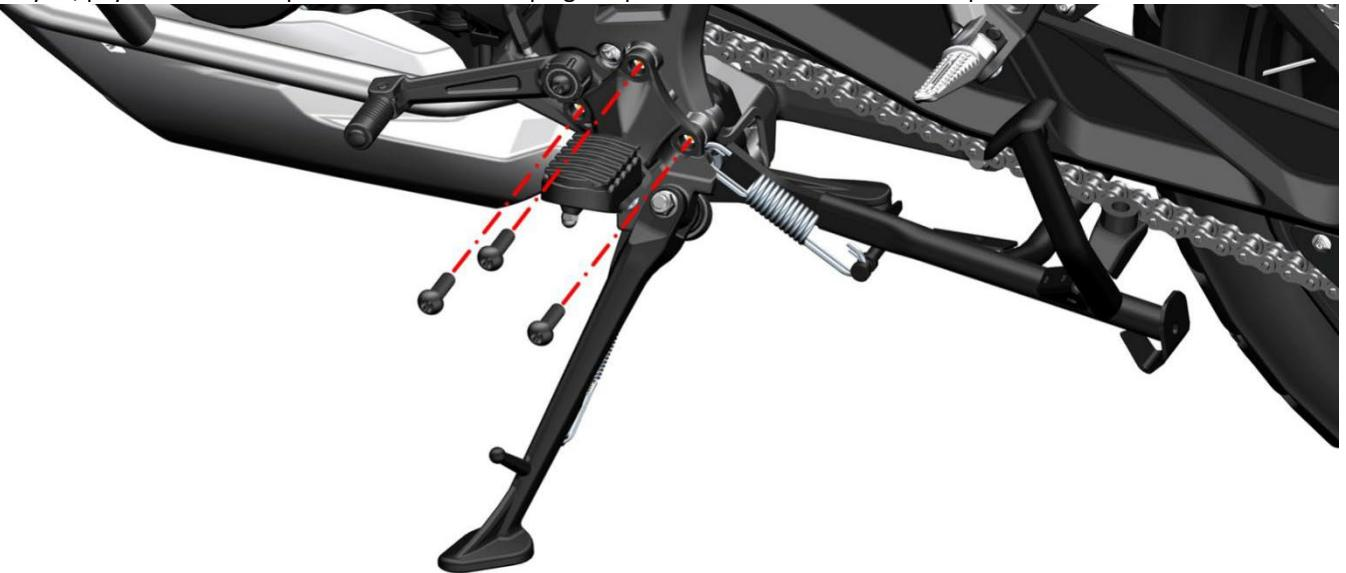
b. Remove the bolt with the 8# sleeve and remove the spring pad and flat pad. Standard torque:  $12\pm1.5$  N.m.
