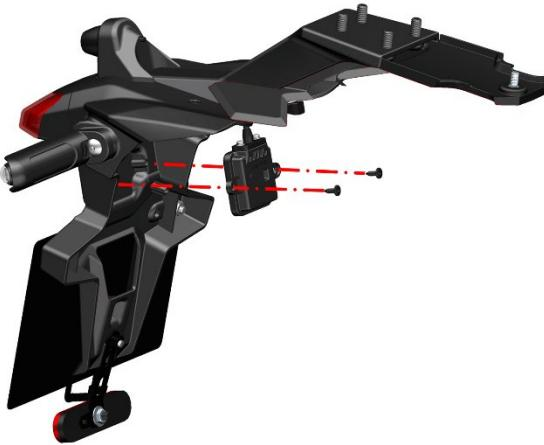
c. Use the 4# hexagon to remove the two M6×16 non-standard inner plum bolts in front of the billboard, and unscrew out the two GB6177 nuts that fix the bolts, take out the rear billboard obliquely, and use the 4# hexagon to unscrew out an M6×14 inner plum shaft shoulder screw, remove the rear reflector bracket and the rear reflector.
