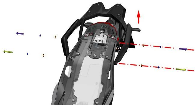
b. Flip the rear armrest to the back, use the 4# hexagon to remove the bolts of the left 4 non-standard inner plum blossoms M6×12, remove the left buffer glue of the rear armrest (shown L), and remove the right buffer glue (shown R) in the same way.
