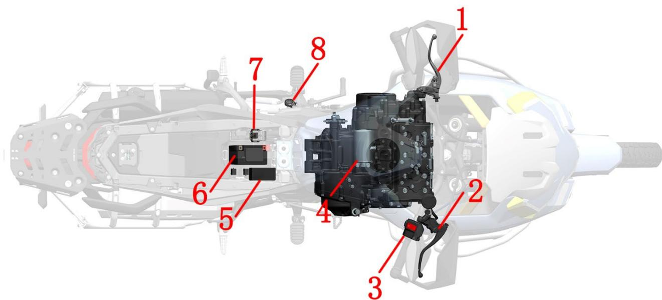
1-Clutch rocker arm (clutch switch) 2-Front disc brake main cylinder (front brake switch) 3-Right handle switch 4-Starter motor 5-Fuse box 6-Battery 7-Starter relay 8-Side bracket power out switch
