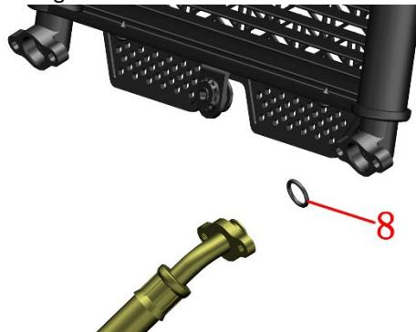
d. If the oil leakage phenomenon cannot be solved by replacing the O-ring (8) on the oil pipe, the corresponding oil leakage oil pipe needs to be replaced.
