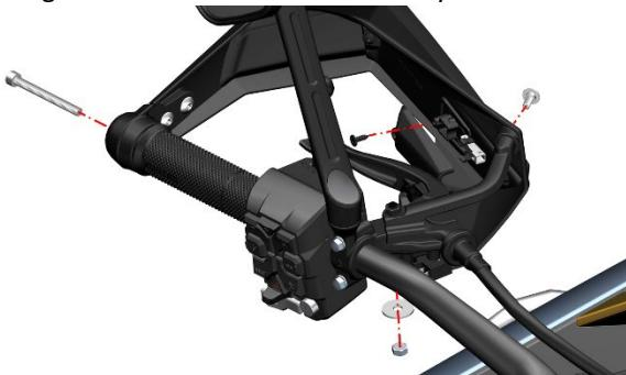
b. Use a cross screwdriver to remove the two self-tapping screws on the handlebar guard and remove the turn signal. Use a T25 plum wrench to remove the two bolts and separate the balance weight and the hand guard.
