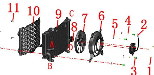
1-Fan motor bolt\*3 2-Fan motor 3-Fan passport bolt\*4 4-Spring pad\*4 5-Gasket\*4 6-Fan guard 7-Fan 8-Fan nut 9-Water tank 10-Water tank front guard 11-Shoulder bolt\*4
