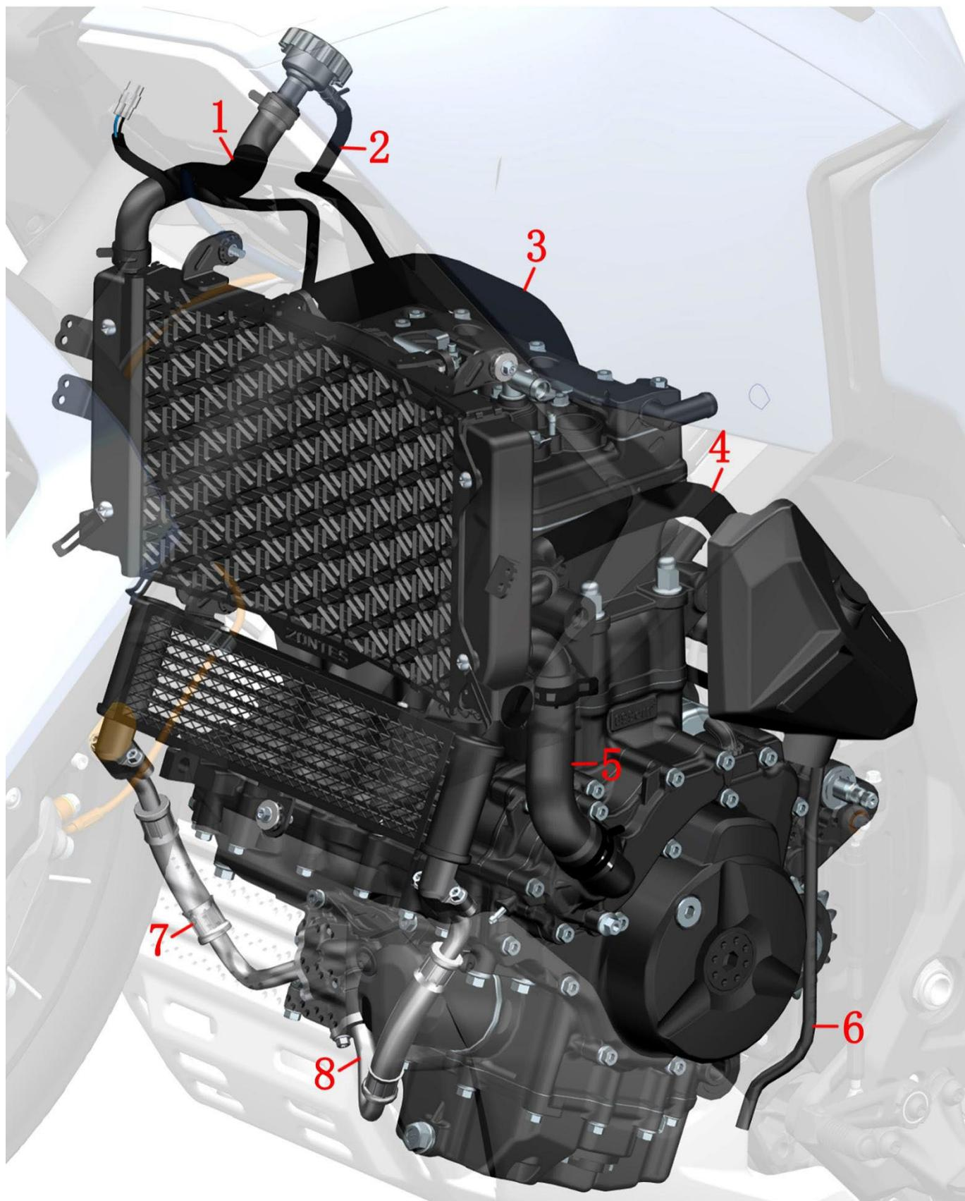
1-ZT703—F The connecting water pipe of the water tank filling port
