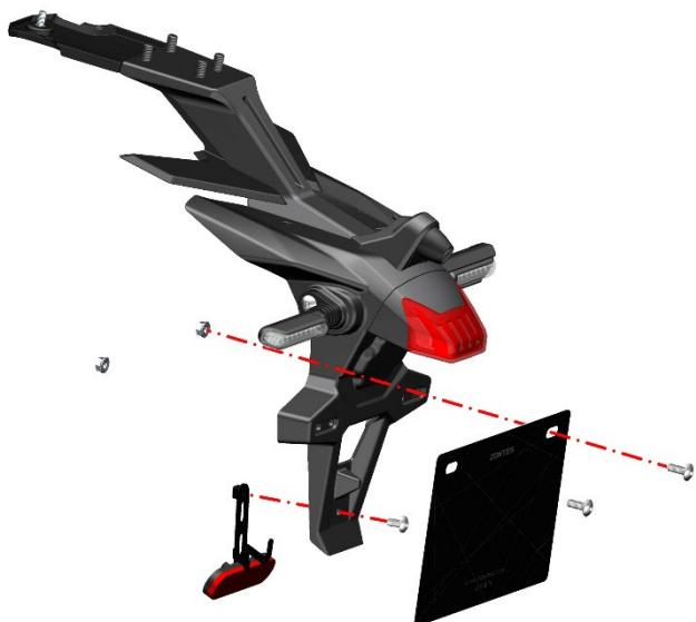
d. Use the 4# hexagon to remove the left 1 M6×25 non-standard bolt, remove the left turn signal, and use the 4# hexagon to remove the right 1 M6×25 non-standard bolt, remove the rear turn signal anti-scald cover and right turn signal.
