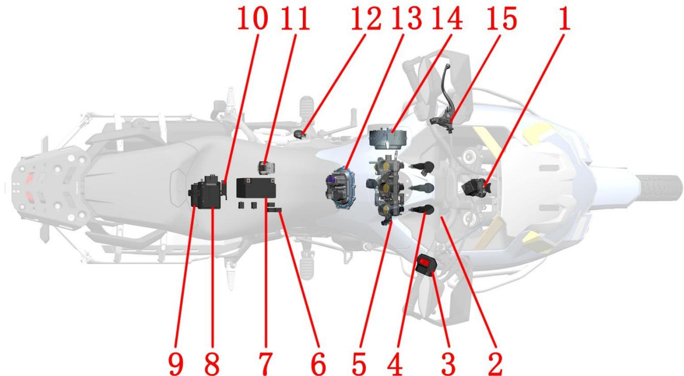
1-Faucet locks 2-Oxygen sensor 3-Right-hand handle switch 4-Ignition coil 5-Throttle assembly 6-Relays (There are 3 pieces inside the main harness fuse box and 2 pieces on the outside of the fuse) 7-accumulator 8-PKE host 9-ECU 10-Tilt switch 11-Start the relay 12-Side bracket flameout switch 13-oil pump 14-Magneto 15-Clutch rocker
