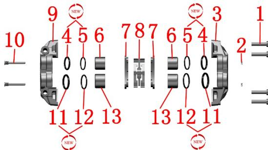
1-bolt 2-Circlip 3-Caliper inner housing 4-φ30 Oil seals 5-φ30 Dust-sealed 6-φ30 piston 7-Brake pads 8-Brake pad spring pads 9-Caliper outer housing 10-Pin shaft 11-φ34 Oil seals 12-φ34Dust-sealed 13-φ34 piston
