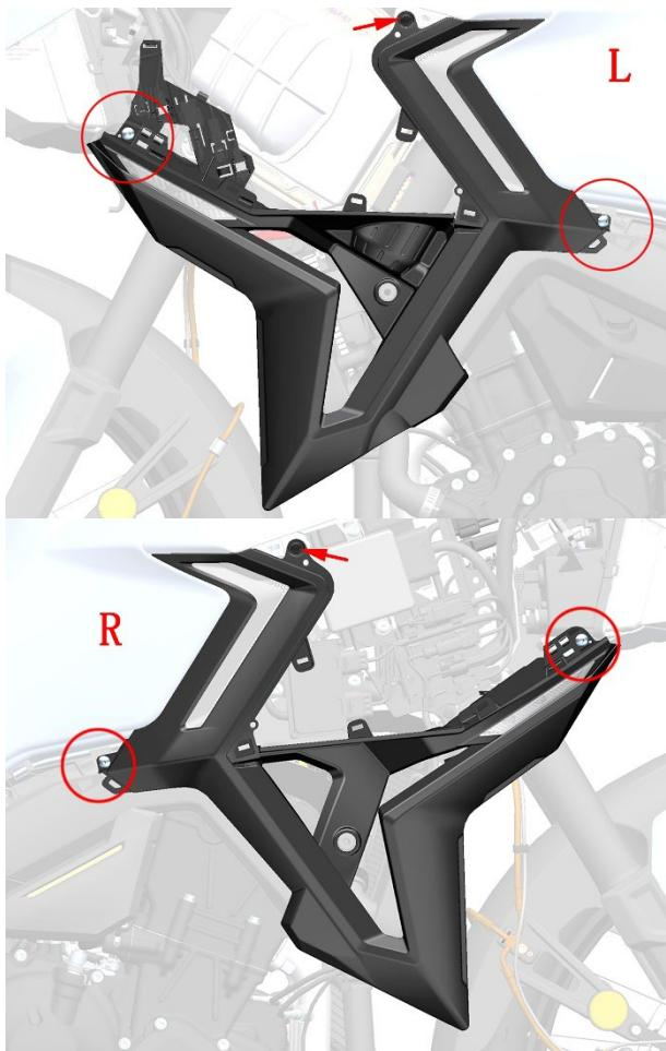
c. Use T25 plum blossom hexagon to remove a M6×16 shaft shoulder bolt bolt, 1 expansion nail, unplug the right enveloping corner lamp, you can remove the enveloping lower assembly, the left enveloping lower component disassembly method is the same.
