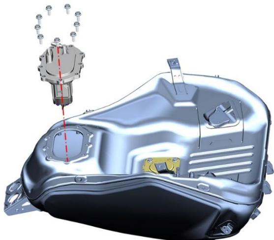
Note that you should not press the fuel outlet pipe shown in the red circle, and once damaged, you can only replace the entire fuel pump assembly.
