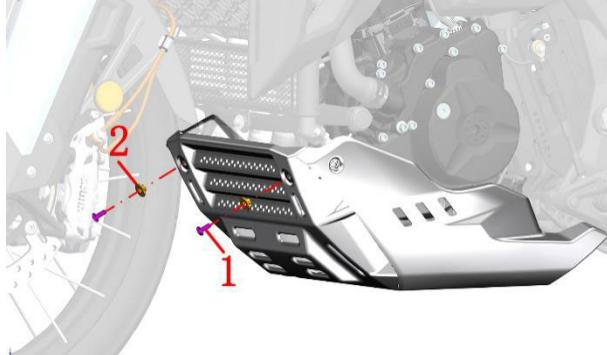
c. Use the plum T25 hexagon inside hex to remove the 3 bolts (1) and flanging bushing (2) of the engine guard, and remove the engine guard. Standard torque: 6 - 8 N.m
