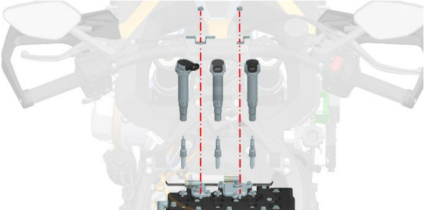
When installing the ignition coil back, first insert the ignition coil back into the bottom, and turn the ignition coil plug towards the position shown in the figure above, then put it back into the pressure plate, and put the nut back tight, and the torque standard is  $11.5\pm1\text{N.m}$ .
