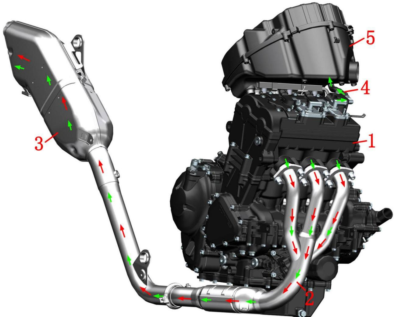
1-cylinder head 2-front muffler 3-rear muffler 4-exhaust gas snorkel 5-air filter assembly
