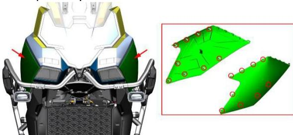
c. Remove the 2 torx groove plate head bolts (3) with a hole torx wrench, and remove the 2 fuel tank flat pads (4) and glue pressing (5). Remove 2 inner torx shoulder bolts (1) with T25 torx socket sockets. Remove 2 expansion nails (2) with a cross batch. Standard torque for bolt (1): 6~8 N.m. Standard torque for bolt (3): 25 ± 3 N.m.
