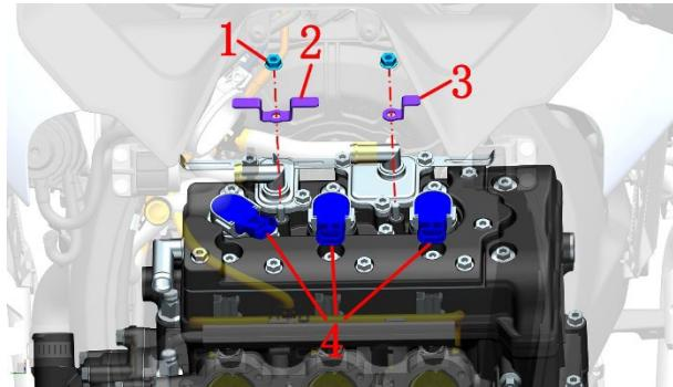
e. Use a blow gun to blow off dust, debris, etc. near the spark plug.
