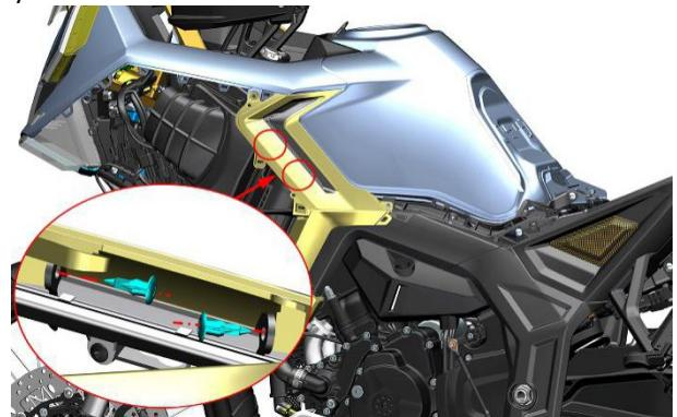
g. Gently pull the lower part of the left envelope in the direction pointed by the arrow with your hand, and remove the self-tapping screws behind the envelope with a cross batch. Lift it up slightly and remove the lower part of the envelope. The right side is removed in the same way.
