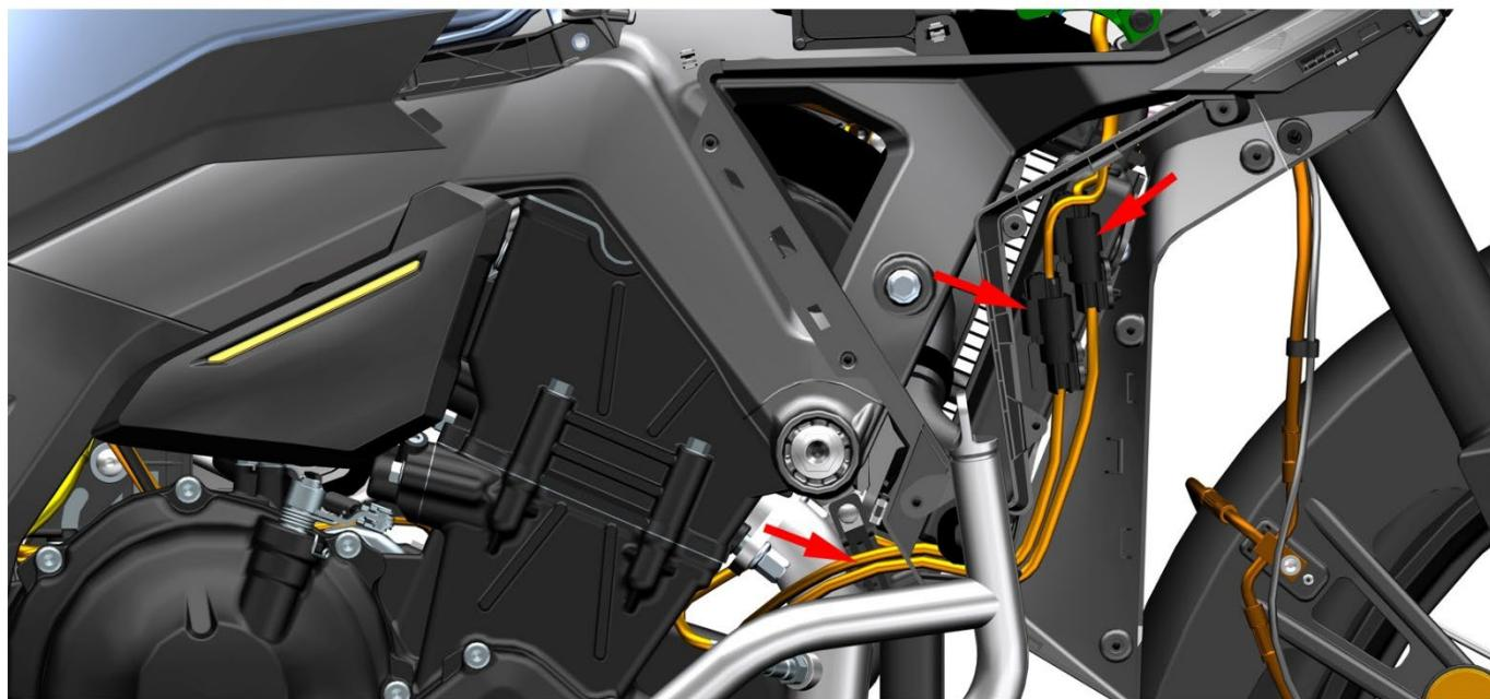
After removing the cover, you can see that the oxygen sensor is fixed as shown in the figure above, squeeze the mushroom head out of the fixing hole.
