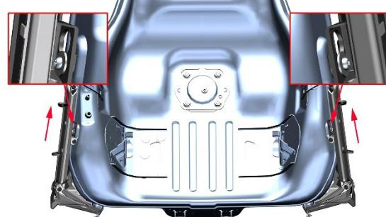
e. Remove the 2 bolts with a cross batch and remove the spacer.
