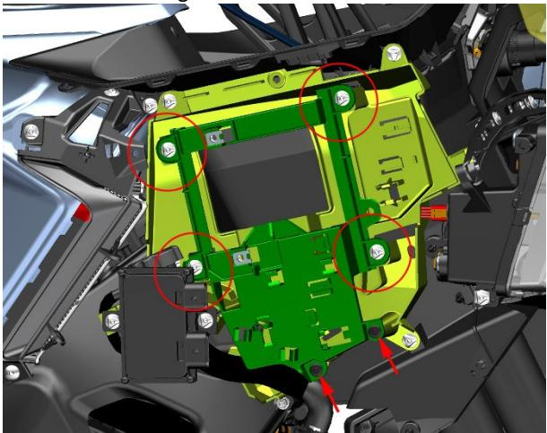
c. Use a T25 Allen Torx wrench to remove the shoulder bolts and bolts of the two M6×14 socket sockets, and remove the fog lamp drive box.
