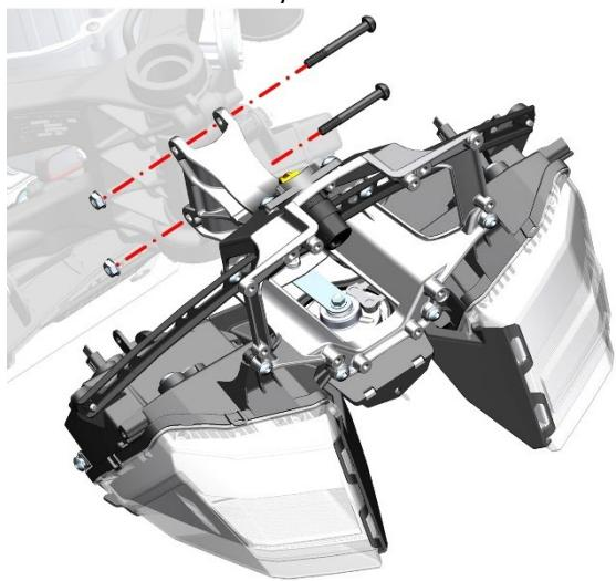
c. The disassembly and disassembly of the head bracket is shown in the figure below.
