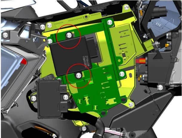
b. Use a T25 socket torx wrench to remove the four shoulder bolts and bolts of M6×14, two expansion nails, and remove the ECU fixing bracket.
