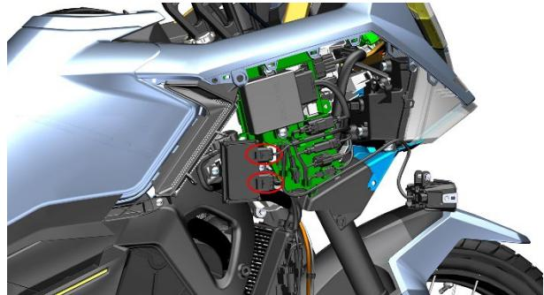
c. Arrange the wiring harness next to it, use the plum T25 hexagon to remove the 2 shoulder bolts (1) that fix the fog lamp drive box and remove the fog lamp drive box (2). standard torque is 2~3N.m.
