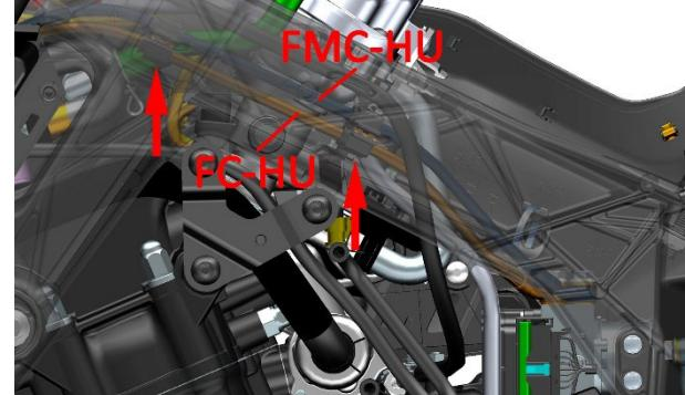
f. Find the plug of the wheel speed sensor on the right side of the vehicle (near the upper right guard), press the anti-disengagement card and pull out the plug.
