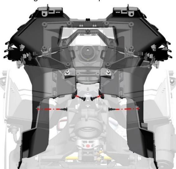
b. Use the T25 plum blossom hexagon to remove an M6×14 axle shoulder bolt on the left side of the vehicle, note: the right M6×14 bolt has been removed when disassembling the wiring version.
