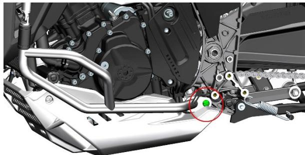
f. Use the T50 torx hexagon with the middle hole to remove 1 M10×25 bolt and remove the right guard bar.
