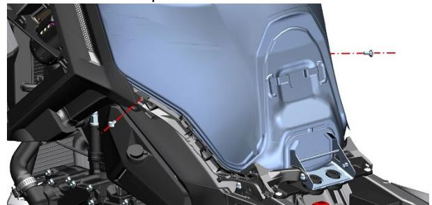
f. Use the hexagon tool to remove the 2 expansion nails in the direction pointed by the arrow pointing to the lower part of the left surround, and remove the right side in the same way.
