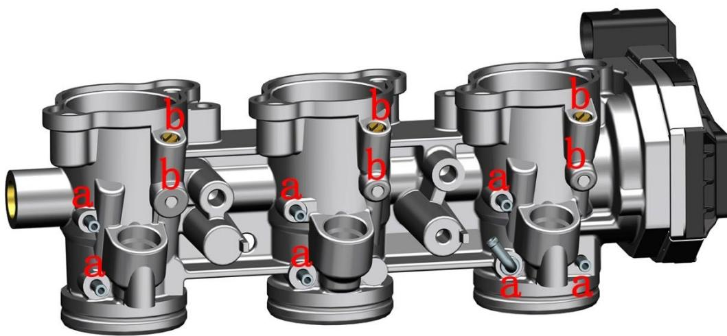
2. Idling is unstable, with the engine speed fluctuating up and down. At this time, connect the diagnostic tool and check that the throttle signal voltage fluctuation must not exceed  $0.08\text{V}$ , and the throttle opening fluctuation must not exceed  $0.5\%$ . If any of the above is abnormal, the throttle body needs to be replaced.
