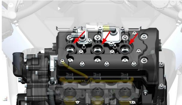
f. Remove the spark plug by rotating counterclockwise with the vehicle's own on-board tool or the special 14# spark plug sleeve.
