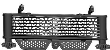
Plug any end of the oil cooler connector and pass compressed air with a pressure of 200 kPa from the other side of the connector to ensure that there is no air leakage at the nozzle position.
