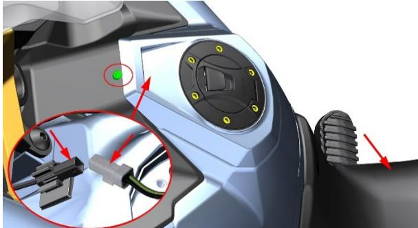
b. After pulling out the 9 buckles of the left and right surrounding panels, remove the left and right surrounding panels respectively.
