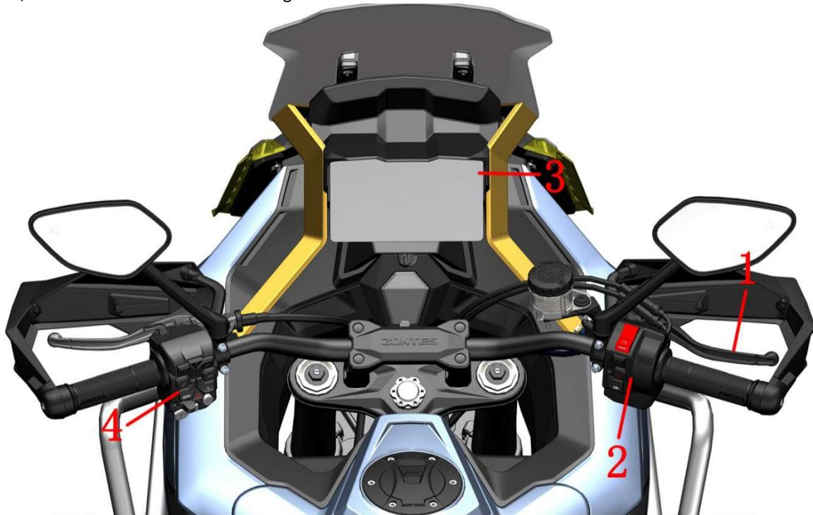
1. Front brake handle 2. Right hand handle switch 3. Meter 4. Left hand handle switch
