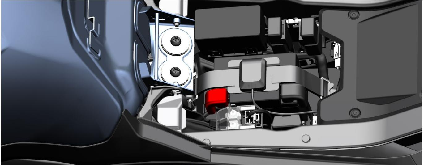
The charging voltage of the charger shall not be higher than 15V. When you do not use the motorcycle for a long time, you should charge it regularly according to the requirements of the driving manual. If the battery loss effect is properly handled by a professional recycling agency, do not discard it at will to avoid pollution to the environment.
