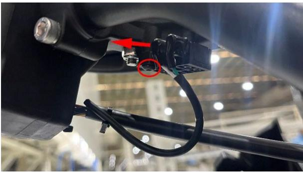
d. Remove the stud with a 10# socket or torx wrench to replace the clutch handle. Standard torque is 8~10 N.m.
