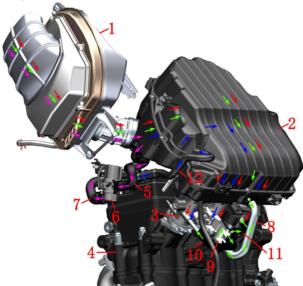
1-Left intake chamber assembly 2-Air filter assembly 3-Throttle valve body assembly 4-Cylinder head 5-Make-up valve rubber hose-4 6-Make-up valve 7-Make-up valve rubber hose-3 8-Stepper motor rubber hose-2 9-Throttle make-up valve 10-Stepper motor rubber hose-1 11-Stepper motor rubber hose-3 12-Exhaust gas snorkel
