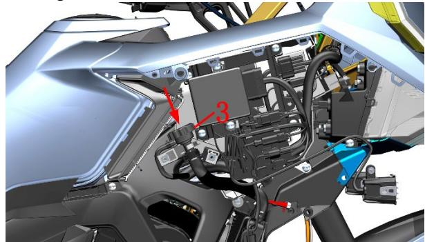
e. Wear waterproof gloves and use the extended funnel to add coolant to the main tank inlet. Until the level of the water filler no longer drops.
