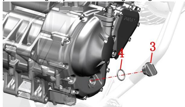
g. After waiting for the oil to flow out completely, use a clean non-woven fabric to wipe the oil drain bolts; Check whether there are scratches on the joint surface of the oil drain bolt, and replace it if so. Then use a clean non-woven fabric to wipe the joint surface of the engine and oil drain bolts.
