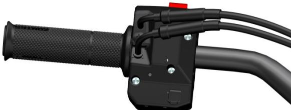
d. Use a Phillips screwdriver to remove the two bolts on the back cover of the left-hand switch, remove the back of the left-hand switch, and then remove the bolts that secure the front. Remove the front of the switch.
