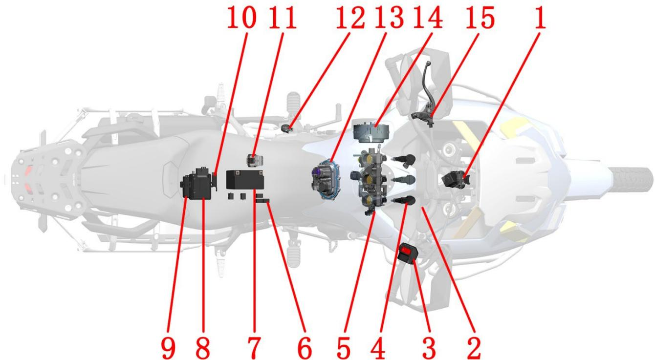
1-Faucet locks 2-Oxygen sensor 3-Right-hand handle switch 4-Ignition coil 5-Throttle assembly 6-Relays 7-accumulator8-PKE host 9-ECU 10-Tilt switch 11-Starting relay 12-Side bracket flameout switch 13-fuel pump 14-Magneto 15-Clutch rocker
