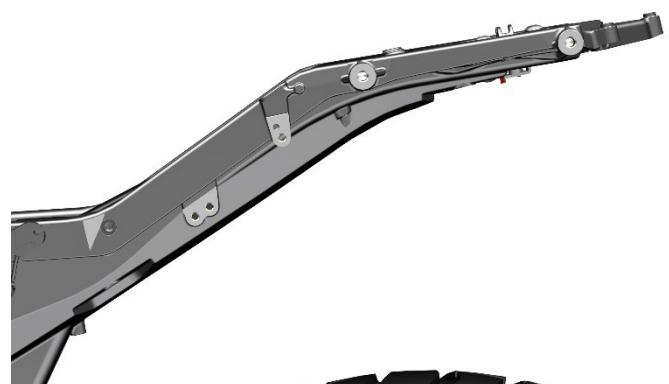
e. Use a Phillips screwdriver to remove the 4 self-tapping screws, remove the right cover mesh liner and the right cover mesh trim, and use the same method to remove the left cover mesh lining.
