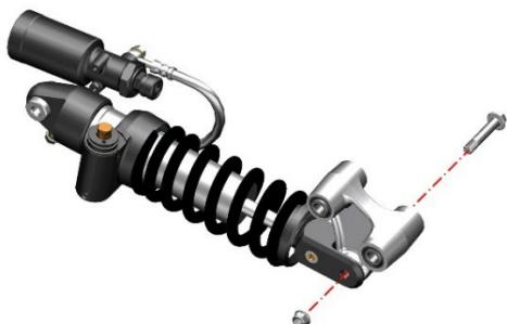
c. If you need to replace the rear shock-absorbing straight connecting rod, you can remove the straight connecting rod according to "Maintenance - Main Bracket". Note: A jack or support is required to support the vehicle.
