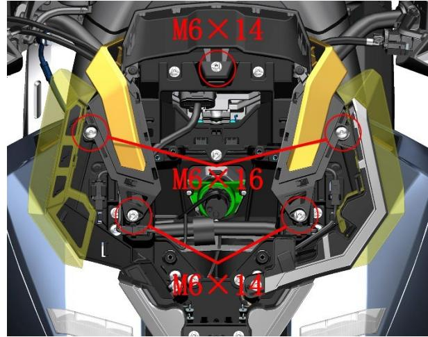
b. After removing the enclosing panel, use a Phillips screwdriver to remove the self-tapping screws as shown. Remove the left and right sides in the same way.
