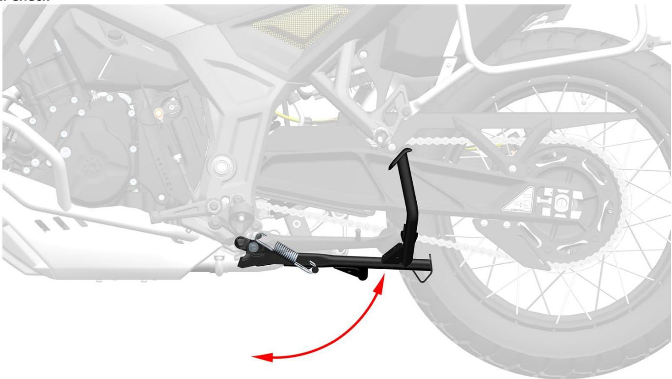
a. Straighten the vehicle, step on the main bracket labor-saving lever with your feet, and check whether the spring elasticity is normal. The main bracket should be able to quickly return to the driving position under the action of the spring's own elastic force.
