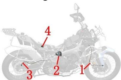
1-Front wheel speed sensor 2-ABS Hydraulic control unit 3-Rear wheel speed sensor 4-OBD Diagnostic interface
