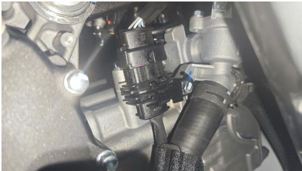
Use a multimeter to measure the resistance of the heating element of the two white wires to be  $9 \pm 2k\Omega$ ; or measure the current to be  $\leq 2.1A$ . Otherwise, it can be judged that the oxygen sensor is faulty. The ceramic inside the oxygen sensor is hard and brittle. Do not use hard objects to knock or blow with strong gas, otherwise it will easily cause damage.
