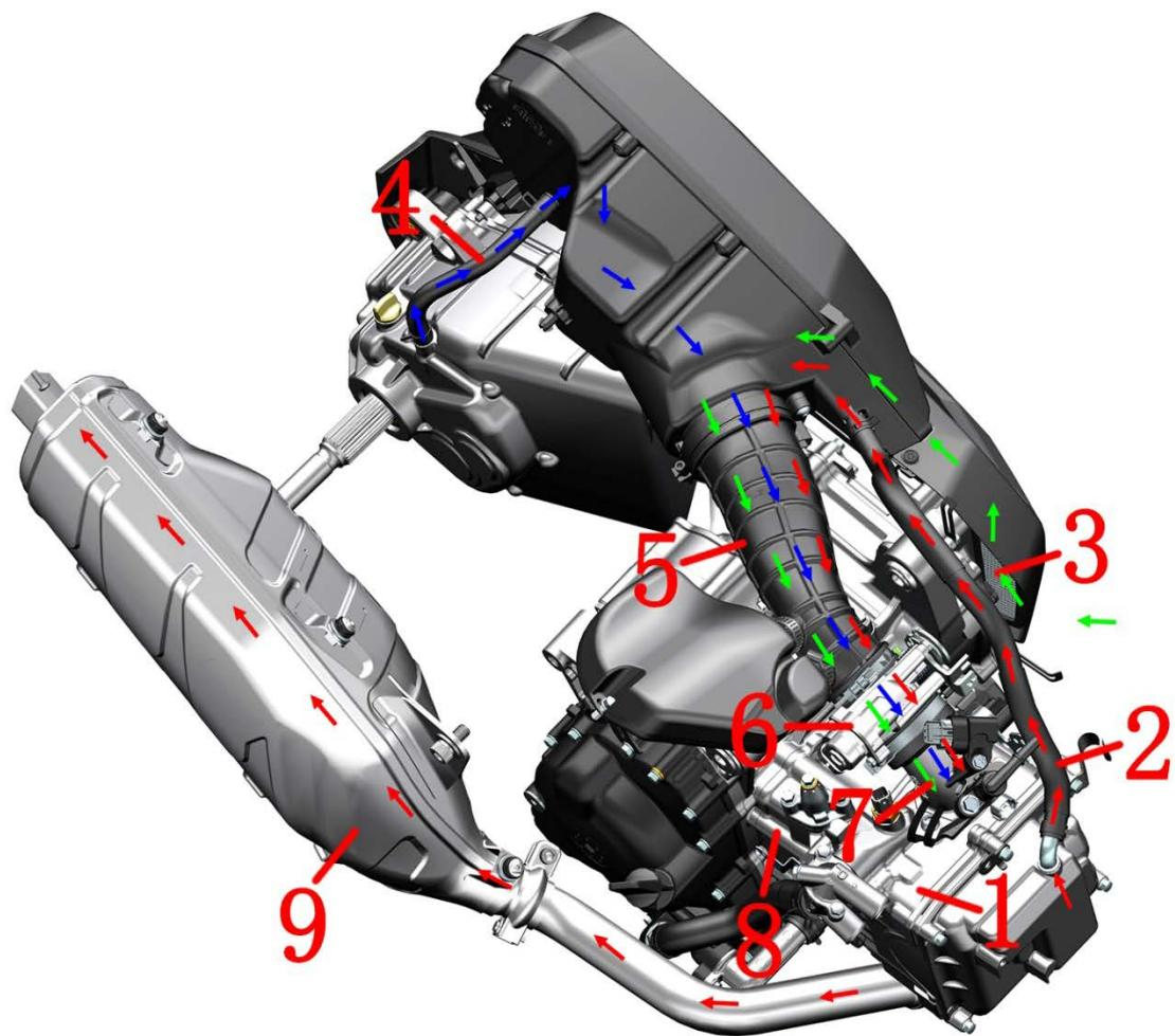
1 - cylinder head 2 - cylinder head exhaust pipe 3 - air filter inlet 4- Gearbox exhaust pipe
