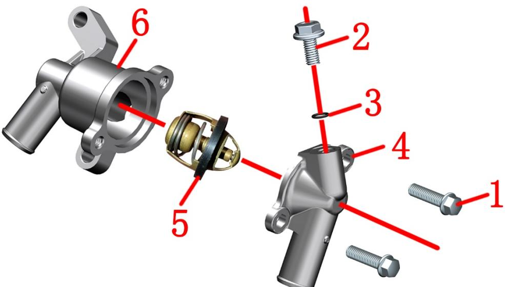
1- M6×22 bolts\*2 2-M6×12 bolts 3-Φ 5.6×Φ1 O-ring 4-Thermostat upper housing 5-Thermostat core 6- Thermostat lower housing
