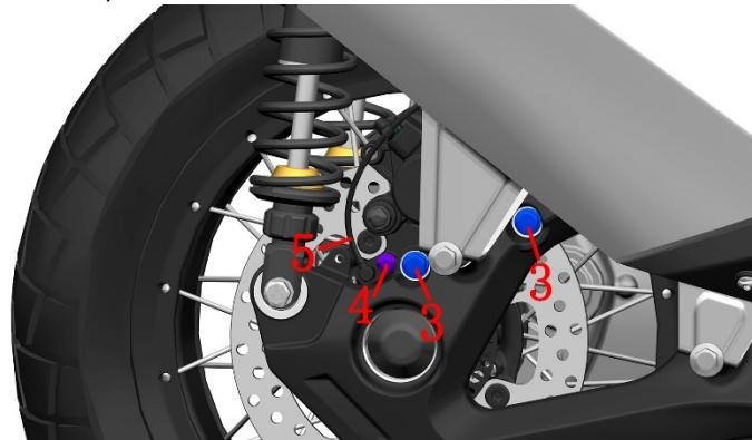
c. Remove the brake pads first.
