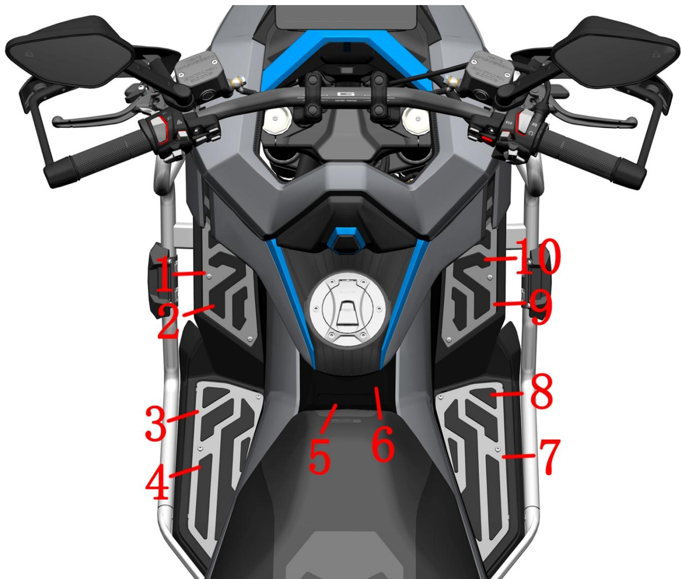
1. Front left pedal rubber pad pressure plate 2. Front left pedal rubber pad 3. Rear left pedal rubber pad pressure plate 4. Rear left pedal rubber pad 5. Fuel tank movable cover 6. Fuel tank cover middle 7. Rear right pedal rubber pad pressure plate 8. Rear right pedal rubber pad 9. Front right pedal rubber pad pressure plate 10. Front right pedal rubber pad
