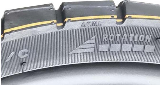
of the raised wear mark on the tread is 1.6mm ( 0.06 in ). The triangle mark (ΔTWL) on the sidewall indicates the position of the wear strip . If the wear reaches the mark point, it means that the wear has reached the limit. Continuing to drive will be a safety hazard and you must replace the tire with a new one of the same specification.
