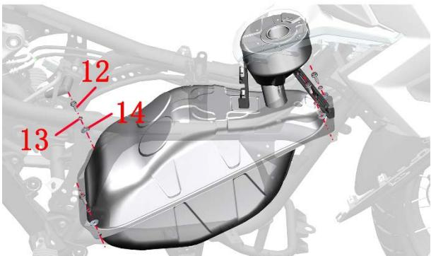
j. Slightly lift the fuel tank assembly from the rear end, move it backward until the fuel tank filling port safely passes under the frame, and then remove the fuel tank assembly upwards.
