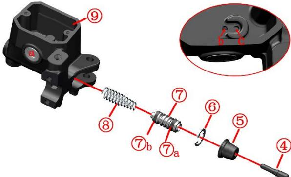
④Piston push rod ⑤Dust cap ⑥ retaining ring ⑦ piston assembly ( ⑦a outer sealing ring ⑦b inner seal ring ) ⑧ spring ⑨ main pump housing
