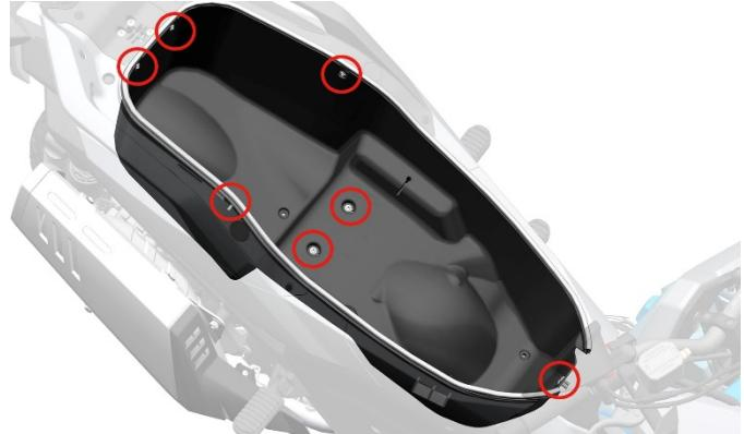
c . Lift the back of the storage box slightly until the wiring harness connector on the left side of the storage box is exposed. Find the ambient light plug and USB cable on the left side of the storage box , unplug the plug and take out the storage box completely .
