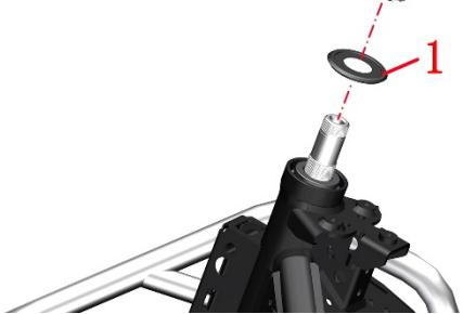
c . Ensure that the lower connecting plate rotates without getting stuck or loose, and then put in the adjusting
