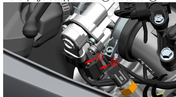
b. Place a small container under the high-pressure fuel pipe and untie the cable tie. Press the green buckle indicated by the arrow and pull out the high-pressure fuel pipe at the same time. A small amount of fuel will flow out when pulling it out, and it is forbidden to drip onto the surface of the parts.
