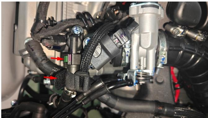
c. Find the retaining ring at the bottom of the valve body, pinch both ends of the retaining ring and move it out, then pull out the desorption tube.
