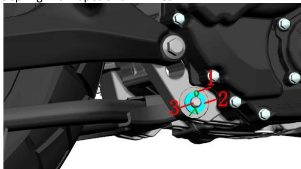
b. Remove the spring from the main bracket .
