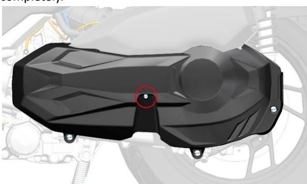
c . Use a 8 # sleeve or T30 plum wrench with hole to remove the three small flange bolt M6×16+flaning bushing+buffer rubber,be careful not lose flanging bushing and buffer rubber. or use 4# hexagon socket remove the three M6×14 shoulder bolts shown in the figure . Use a 4 # hexagon socket to press down the center cylindrical pin of the expansion screw of the air filter decorative cover , and then remove the expansion screw . Remove the decorative cover.
