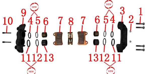
1- Bolt 2- Circlip 3- Inner housing of caliper 4-  $\phi 3$  0 oil seal 5-  $\phi 3$  0 dust seal 6-  $\phi 3$  0 piston 7- Brake pad seal 8- Brake pad spring 9- Outer housing of caliper 10- Pin 11-  $\phi 3$  4 oil seal 12-  $\phi 3$  4 dust seal 13-  $\phi 3$  4 piston
