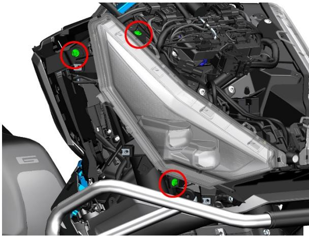
e. Use a T2 5 -inch box end wrench to remove the two middle bolts as shown in the figure.
