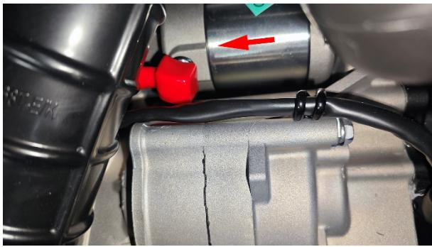
When reassembling, be careful not to miss the O-ring that comes with the starter motor, and align it with the teeth of the electric starter reduction gear. Note that the O-ring must be correctly assembled into the box. If the edge is cut, it
