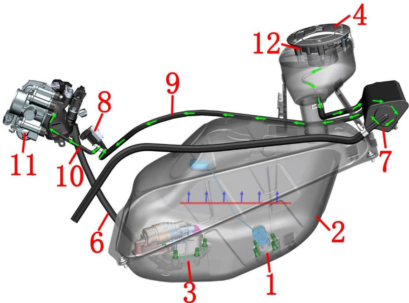
1 - Fuel level sensor 2 - Fuel tank 3 - Fuel pump 4 - Fuel tank cap 5 - Adsorption /vent pipe
