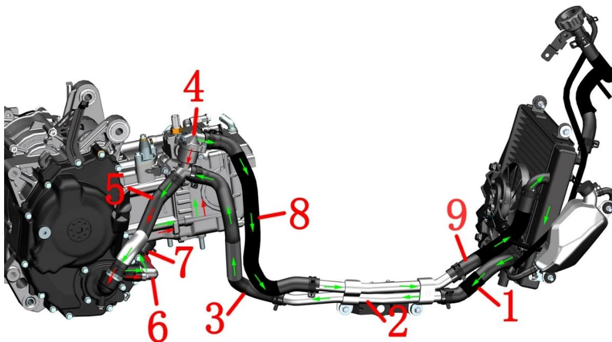
1- Main water tank outlet pipe 2- Aluminum water pipe 3- Engine water pipe
