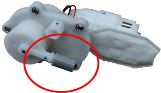
When reassembling, you need to pre-tighten the bolts diagonally first and then tighten the 5 bolts. Otherwise, the uneven compression of the fuel pump's sealing rubber ring may easily lead to leakage and cause safety hazards.
