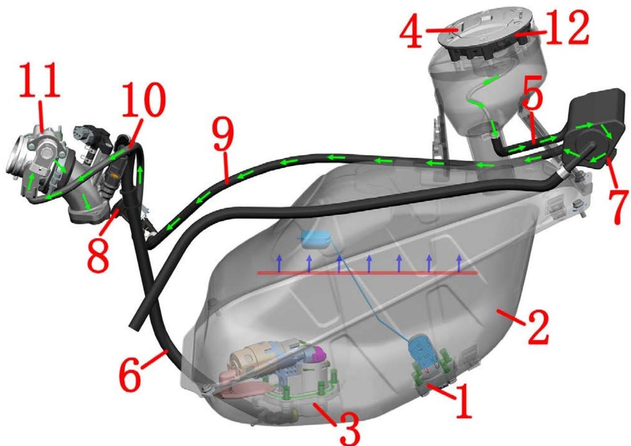
1 - Fuel level sensor 2 - Fuel tank 3 - Fuel pump 4 - Fuel tank cap 5 - Adsorption /vent pipe
