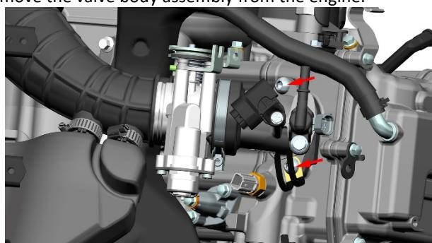
f. Remove the insulation pad and O-ring assembly, and remove the O-ring. Use a 4# hexagon socket to loosen the clamp and separate the intake manifold from the valve body assembly. Use two 10# open-end wrenches to loosen the two nuts on the fuel line and pull it out to remove it from the bracket; remove the cylindrical head of the throttle line from the turntable. After loosening the two nuts of the return oil line, completely loosen the bottom nut from the threaded
