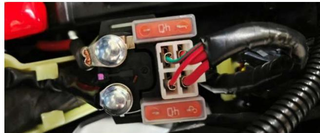
When reinstalling the relay, the red wire is installed in the threaded hole marked "B" on the relay, and the black wire is installed in the threaded hole marked "M" on the relay. Make sure the screws are tightened and the protective cap is put on, then plug in the relay connector.
