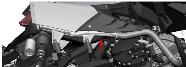
• Oil, dirt and other stains on the surface of the muffler should be cleaned promptly .
