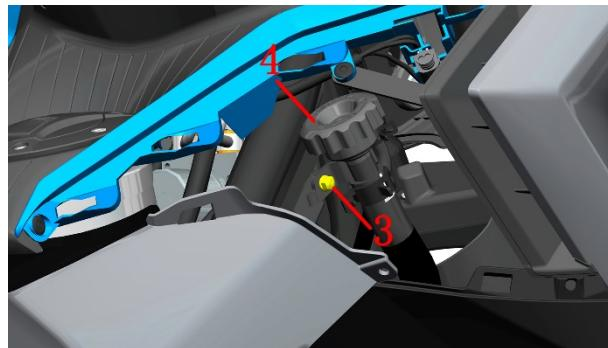
c. Use a 10# sleeve to loosen the thermostat's M6×12 bleed bolt (5) counterclockwise for 4 to 5 turns. Do not remove it completely. Note that a small container should be used to collect the coolant overflowing from the bleed bolt. Do not allow the coolant to drip directly onto the surface of the part. The O-ring at the bleed bolt is  $\phi 5.6 \times \phi 1$  .
