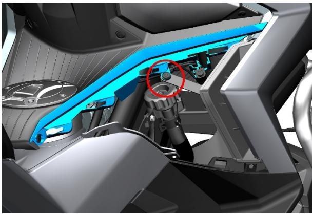
d . Find the plug of the turn signal and unplug the connector of the right turn signal.
