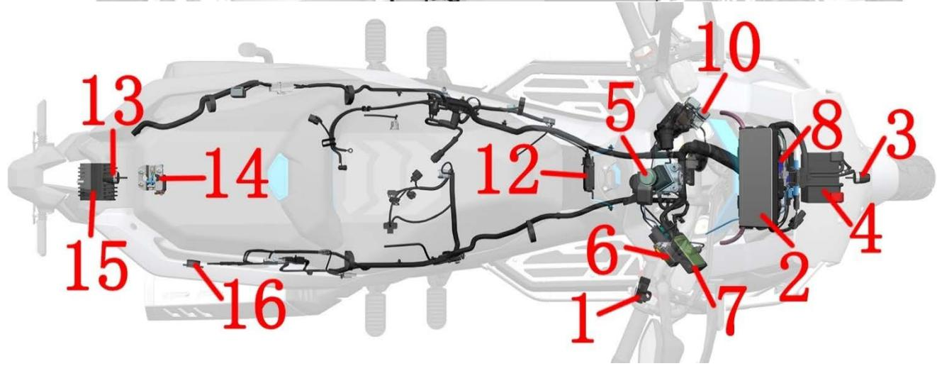
1- Electric heating handle switch 2 - TFT instrument 3 - Front camera 4 - Battery 5 - Flasher 6 - Charging port 7 - PKE host 8 - Engine controller (ECU) 9 - Start relay 10 - EFI relay 11 - Speaker 12 - Fog lamp drive box 13 - Rear camera 14 - Electronic seat lock 15 - Rectifier 16 - Buzzer
