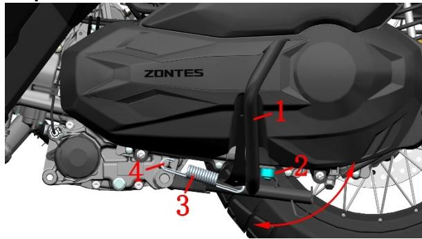
1. Main bracket 2. Buffer rubber 3. Main bracket spring 4. Main bracket reset spring column
