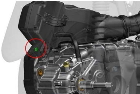
b . Use T30 plum wrench with hole to remove the small flange bolt M6×16 or use 4# hexagon socket remove the M6×14 shoulder bolts shown in the figure . The bolt here cannot be removed for the time being, so just loosen it completely.
