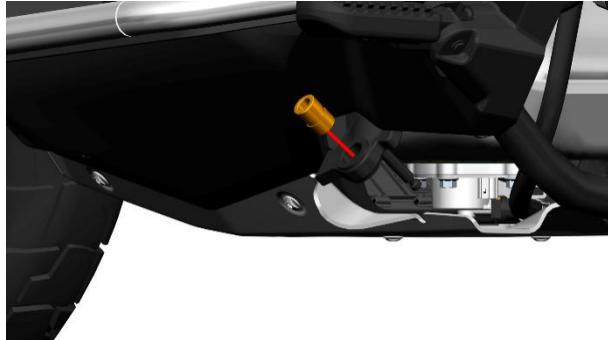
g. Use diesel or kerosene, or a clean rag to wipe off the remaining grease. Apply a proper amount of grease to the two mounting surfaces inside the side bracket and the outer surface of the bushing , and try not to apply it to the threaded holes.
