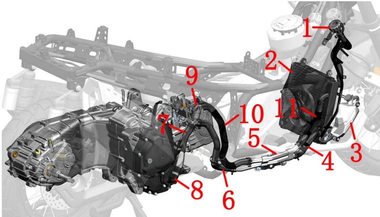
1 - Main water tank filling port 2 - Main water tank 3 - Auxiliary water tank 4 - Main water tank outlet pipe 5 - Aluminum water pipe 6 - Engine water pipe 7 - Water pump cover water inlet pipe 8 - Water pump cover assembly 9- Thermostat assembly 10- Thermostat water outlet pipe 11- Main water tank water inlet pipe
