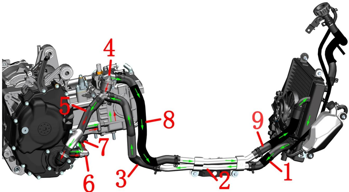
1- Main water tank outlet pipe 2- Aluminum water pipe 3- Engine water pipe 4 - Thermostat
