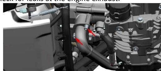
a. If there is a slight air leak, try to tighten the exhaust port nut with a 6 # hexagon socket; if the problem is not solved, remove the muffler and replace the engine exhaust port gasket with a new one.
