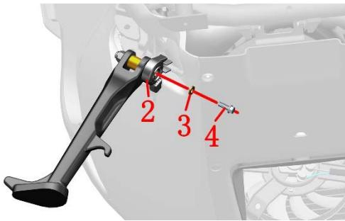
e. Use a 14 # sleeve to secure the bolts on the inside and a 14 # sleeve to remove the nuts on the outside.
