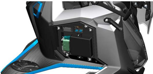
Open the rubber plug and insert the original standard charger DC plug. Then plug the AC socket into a 110-220V power source. If the battery is damaged by using a low-quality charger, it is not covered by the warranty.
