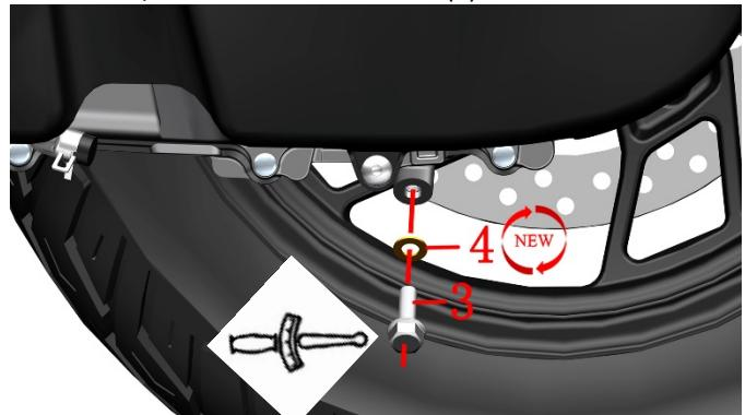
c. Remove the M8x25 drain bolt (3) and 8.3x16x1.5 copper gasket (4).
