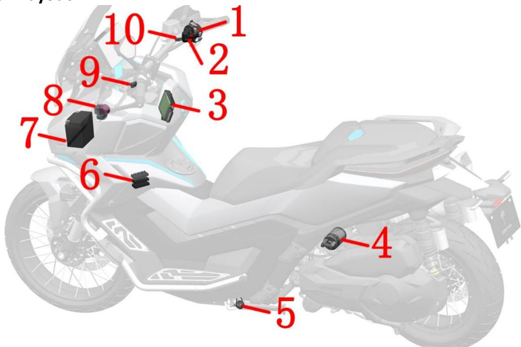
1- Right handlebar switch (ignition off switch, start button ) 2- Right handlebar auxiliary switch (unlock vehicle ) 3- PKE 4-Starter motor 5-Side stand ignition off switch 6- fuse box 7-battery 8-starter relay 9-rear brake switch 10- front brake switch )
