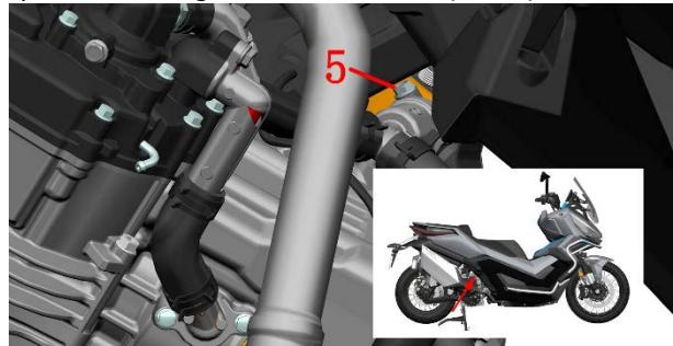
d. Wear waterproof gloves and use an extended funnel to add coolant to the main water tank water inlet. Wait until the thermostat bleed bolt position is stable and the coolant overflows, and the coolant level can be seen at the water inlet.
