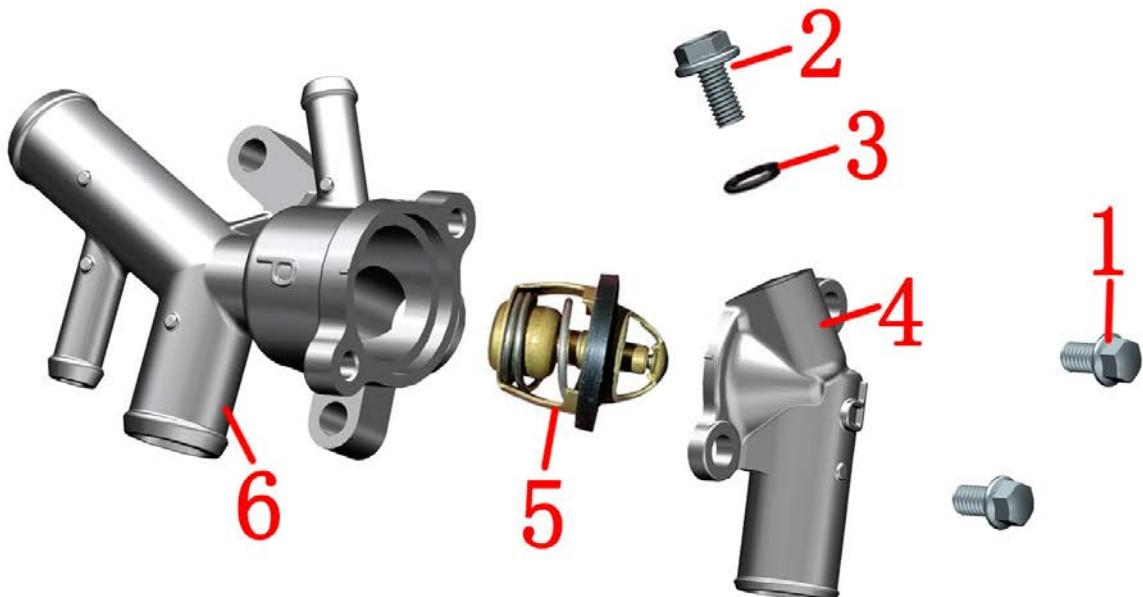
1-M6 ×22 bolts\*2 2-M6 ×12 bolts 3-φ 5.6×φ1 O-ring 4-Thermostat upper housing 5-Thermostat core 6- Thermostat lower housing
