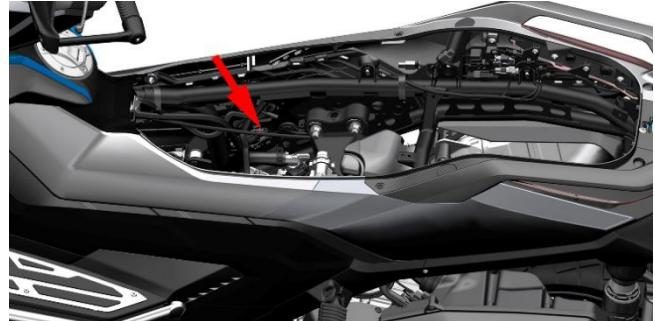
Find the plug on the inside of the left tail cover of the motorcycle body. In addition, use a multimeter to measure the phase-to-phase resistance of any two terminals of the three -pin plug of the magneto stator. It should be  $0.7\pm0.15\Omega$  at 25 °C (77F) .
