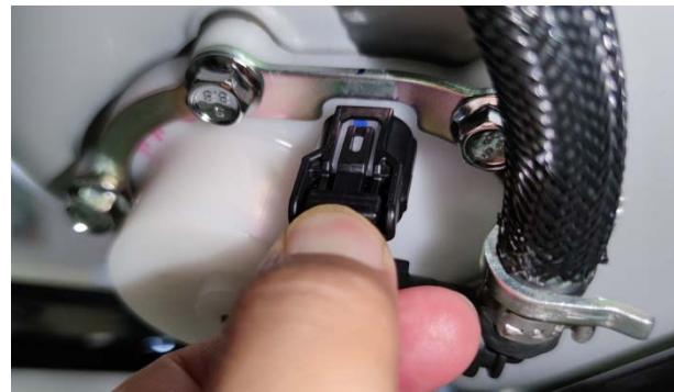
Be careful not to press the oil outlet pipe circled in red. Once damaged, the entire fuel pump assembly can only be replaced.
