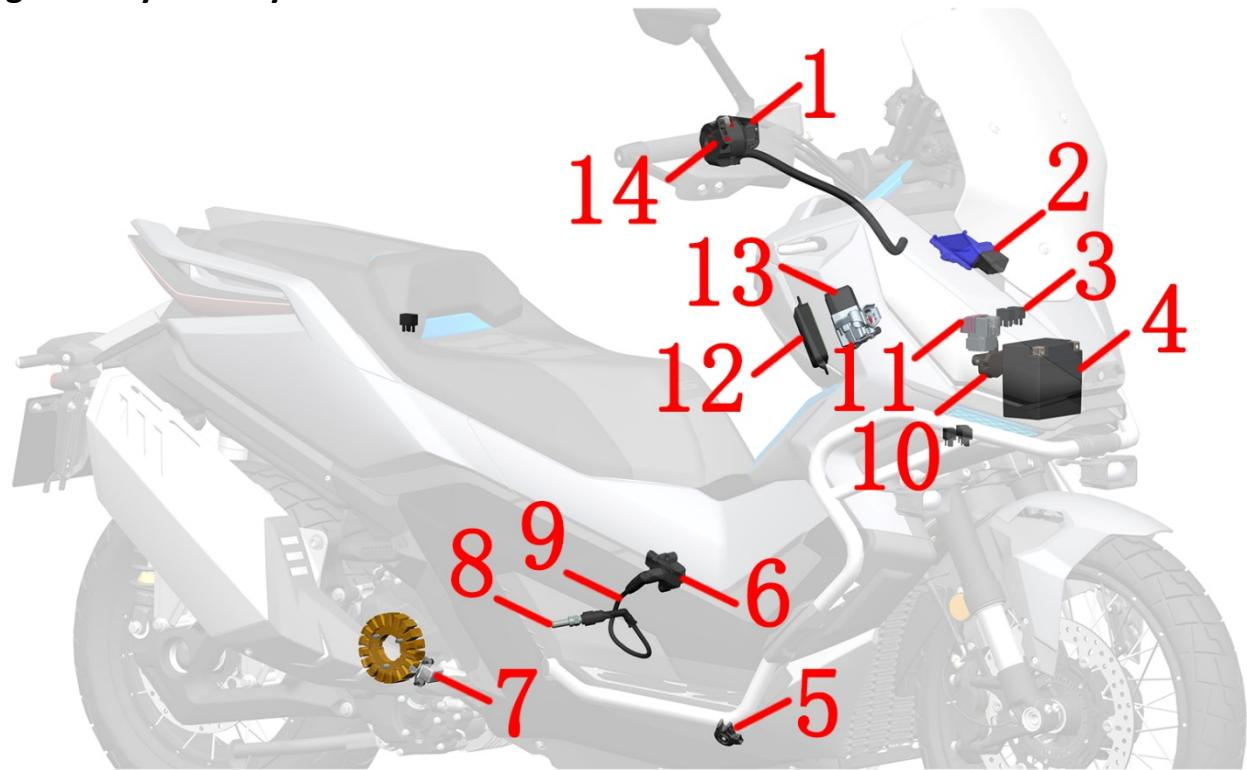
1- Right Handlebar Auxiliary Switch 2-Engine controller (ECU ) 3- Relay 4-Battery
