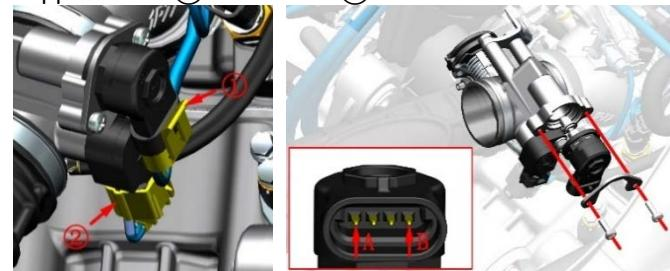
Simple test method: After turning off the power, take out the stepper motor, do not loosen the cable plug, press the flameout switch when turning on the machine, do not ignite, check whether the motor plug can shrink back and forth, and finally turn off the flameout switch to check whether the plug returns to its original position.
