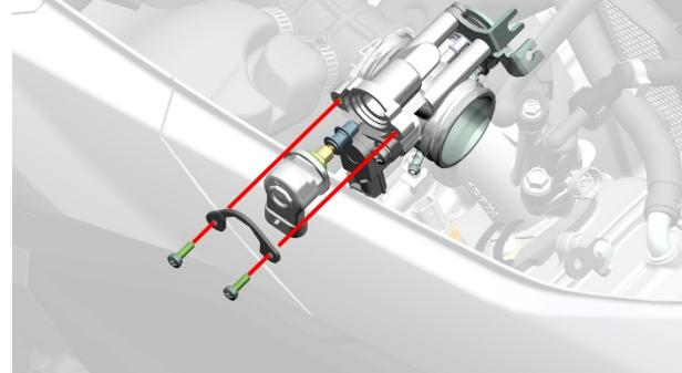
d. Use throttle cleaning agent to clean the carbon deposits on the head of the stepper motor. Spray a small amount of cleaning agent into the valve body hole. Do not soak the stepper motor with any liquid.
