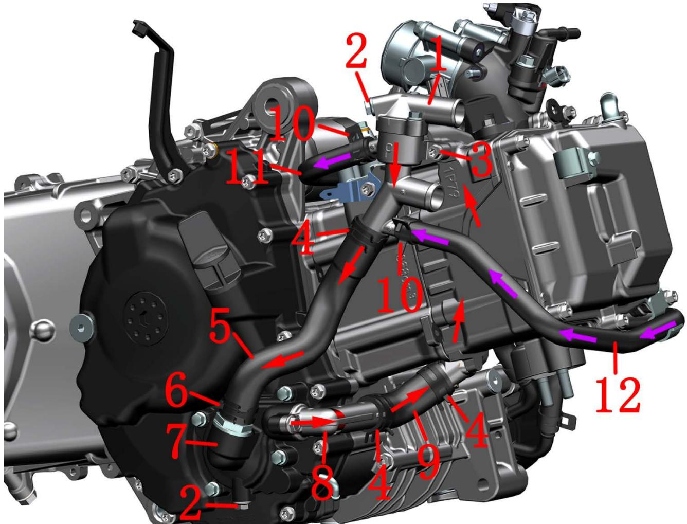
1-Thermostat assembly 2-M6×12 bolt\* 23 - M6×22 bolt \* 24 - Water pipe clamp (φ 26) \* 35 - Water pump cover water inlet pipe 6 - Water pipe clamp (φ 24) 7 - Water pump cover assembly 8 - Water pump cover outlet pipe joint 9 - Water pump cover outlet pipe
