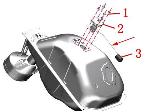
When reassembling, you need to pre-tighten the 4 bolts diagonally first and then tighten them . Otherwise, the uneven compression of the sealing rubber ring of the oil level sensor may easily lead to leakage and cause safety hazards .
