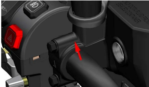
e . Place the handlebar on the pad, and use bolts and pressure blocks to pre-fix the handlebar on the pad. It is necessary to leave adjustment positions for the handlebar, and there is no need to tighten the bolts for the time being. As shown in Figures ③ and ④, place the handlebar according to the scale position until it coincides with the positioning point of the pressure block, and then use a 6 # hexagonal tool to tighten the four bolts.
