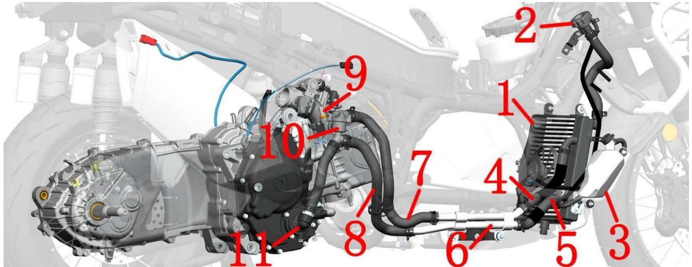
1 - Main water tank 2 - Water tank filling port 3 - Auxiliary water tank 4 - Main water tank inlet pipe 5 - Main water tank outlet pipe 6 - Aluminum water pipe 7 - Thermostat water outlet pipe 8 - Engine water inlet pipe 9 - Water and oil common sensor 10- Thermostat 11- Water pump cover assembly
