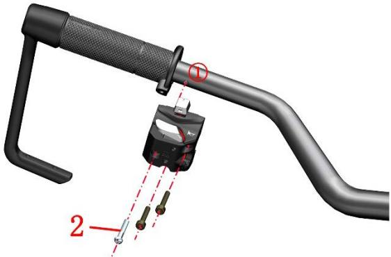
c. When installing the right-hand switch, align the cross-head bolts (3) with the positioning holes ② on the handlebar switch and the direction handle, and then pre-tighten them with a cross-head screwdriver . Align the upper and lower parts of the right-hand switch and combine them, and use a 5 # hexagon socket to tighten the two bolts that come with the right-hand switch . Remove the pre-tightened
