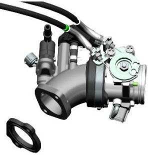
g. Use throttle body cleaning agent to clean the carbon deposits on the intake manifold and throttle body outlet. Do not soak the throttle body assembly and intake manifold assembly directly with any liquid.
