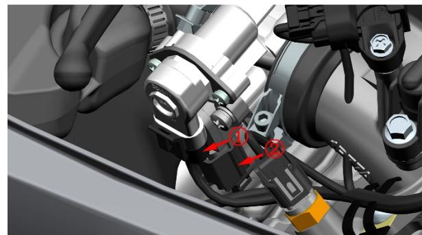
c. Use a short Phillips screwdriver to remove the two bolts and anti-drop card that come with the throttle valve body assembly, and then remove the stepper motor.
