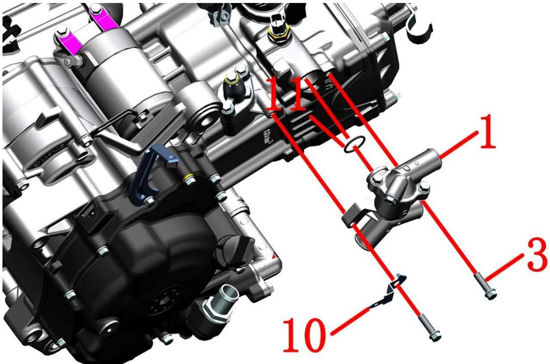
reassembly , clean the joint surface and make sure that the O-ring is not missing and is properly assembled . The clamp should be stuck inside the boss to prevent it from loosening. Bolt (3) Torque:  $12\pm1.5$  Nm ( $1.2\pm0.2$  kgf.m,  $9\pm1$  lbf.ft) .
