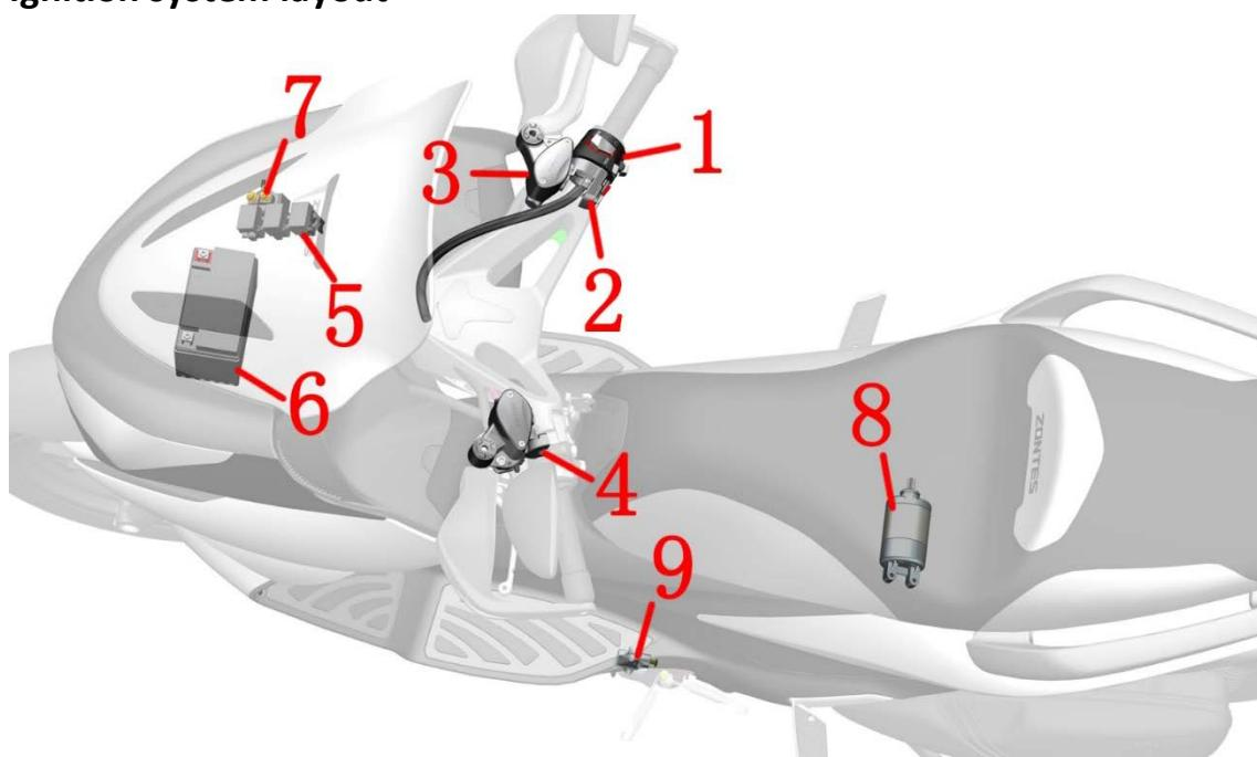
1-Right-handle switch (stop switch, start button) 2-Right-handle secondary switch (to unlock the motorcycle) 3-Front disc brake main pump (front brake switch) 4-Rear disc brake main pump (rear brake switch) 5-Fuse box 6-Battery 7-Starting relay 8-Starting motor 9-Side bracket flameout switch
