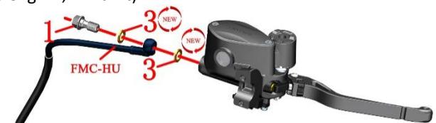
e. Refer to the steps of adding brake fluid to remove the upper cover; refer to the steps of removing the brake switch and brake handle to remove.
