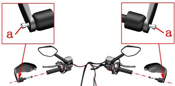
c. Remove 4 M6×30 bolts (2) with 5# Allen, remove the left deputy handle switch (3), rear disc brake main pump assembly b, right deputy handle switch (4), front disc brake main pump assembly c.
