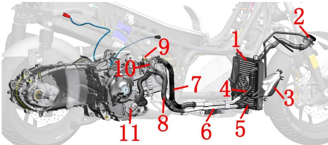
1-Main water tank 2-Water tank filling port 3-Auxiliary water tank 4-Main water tank inlet pipe 5-Main water tank outlet pipe 6-Aluminum water pipe 7-Thermostat outlet pipe 8-Engine inlet pipe 9-Water and oil common sensor
