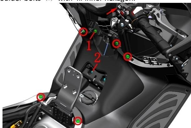
b. Unplug the fuel tank lock connector and take off the fuel tank trim cover assembly.
