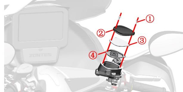
e. Use the brake fluid water content tester to measure the water content, if it is more than 2%, all brake fluid needs to be replaced; if it is less than or equal to 2%, add newly opened DOT 4 brake fluid to the transparent observation window of the front disc brake main pump 3/4 places. It is recommended that the water content should be less than 1.5%. Total 0.23L (0.24 US qt, 0.2 Imp qt, 0.06 US gal, 0.05 Imp gal) TOTAL HBF 4 (DOT 4) brake fluid is added to this vehicle from the factory.
