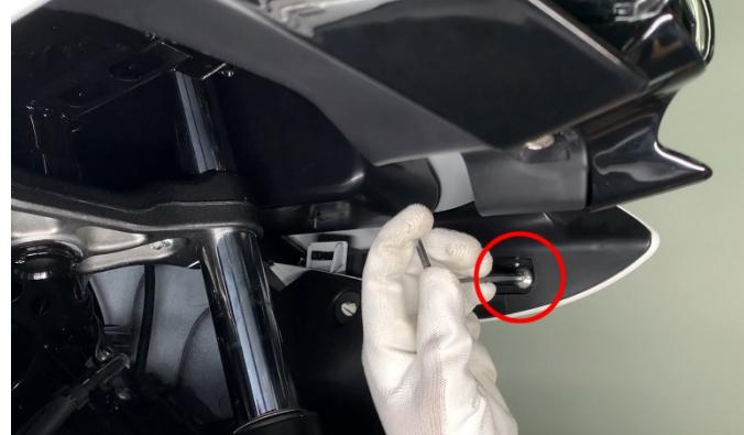
b. Start the motorcycle, open the left glove box, and use a 4# inner hexagon to remove one M6×14 shoulder bolt and one expansion nail as shown in the picture
