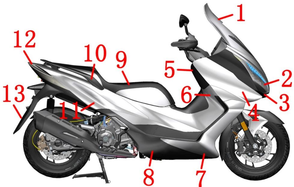
1. Windshield 2. Headlights 3. Lower part of the hood 4. Right panel of the hood 5. Front right panel 6. Right side cover
