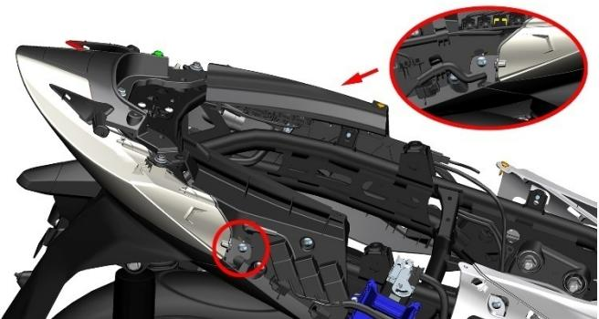
d. Buckle down the two expansion nails as shown in the picture, use a 10# sleeve to remove the two M6x16 bolts on the left and right sides of the fixed taillight(1), and use a 10# sleeve to remove one M8x bolt that fixes the rear light 30 bolts (2).
