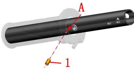
b. When installing the left hand handle switch, it is necessary to align the bolt (a) with the positioning hole (1) on the directional handle, and then tighten it with a cross batch. When installing the right-hand handle bar, align the mounting hole of the heating switch with the positioning hole (1) on the directional handle, and then tighten the bolt (2) with a cross batch. Use the 5# Allen to tighten the bolts (b), (c), (e), and (f) that hold the left and right handle switches in turn.
