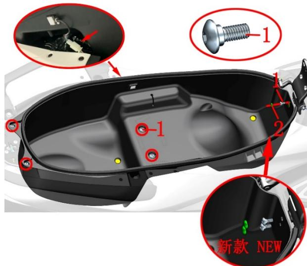
c. Slightly lift the back of the glove box until the harness connector on the left side of the glove box is exposed, unplug the ambient light plug on the left side of the glove box, unplug the plug, and take out the glove box completely.
