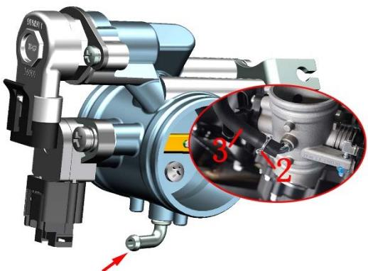
d. Loosen the bolt of the clamp(4) with a 4# inner hexagon and pull out the air filter outlet pipe(5) and clamp(4) in the direction of the arrow to pull out the throttle valve body.
