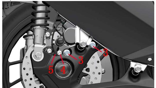
c. Refer to the procedure for replacing the brake pads to remove the brake pads first.
