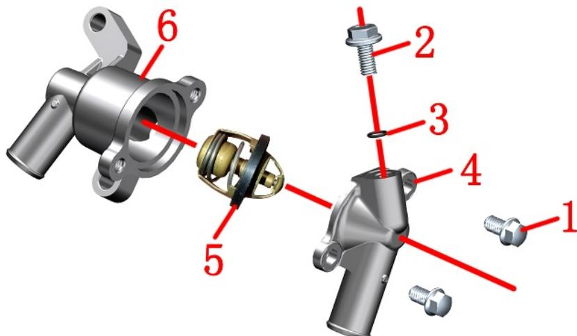
1-M6×10 bolt\*2 2-M6×12 bolt 3-φ5.6×φ10 ring 4-thermostat upper shell 5-thermostat core 6-thermostat lower shell
