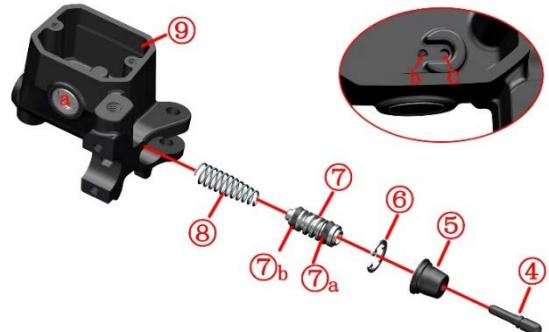
④ Piston pushrods ⑤ Dust cap ⑥ Retaining rings
