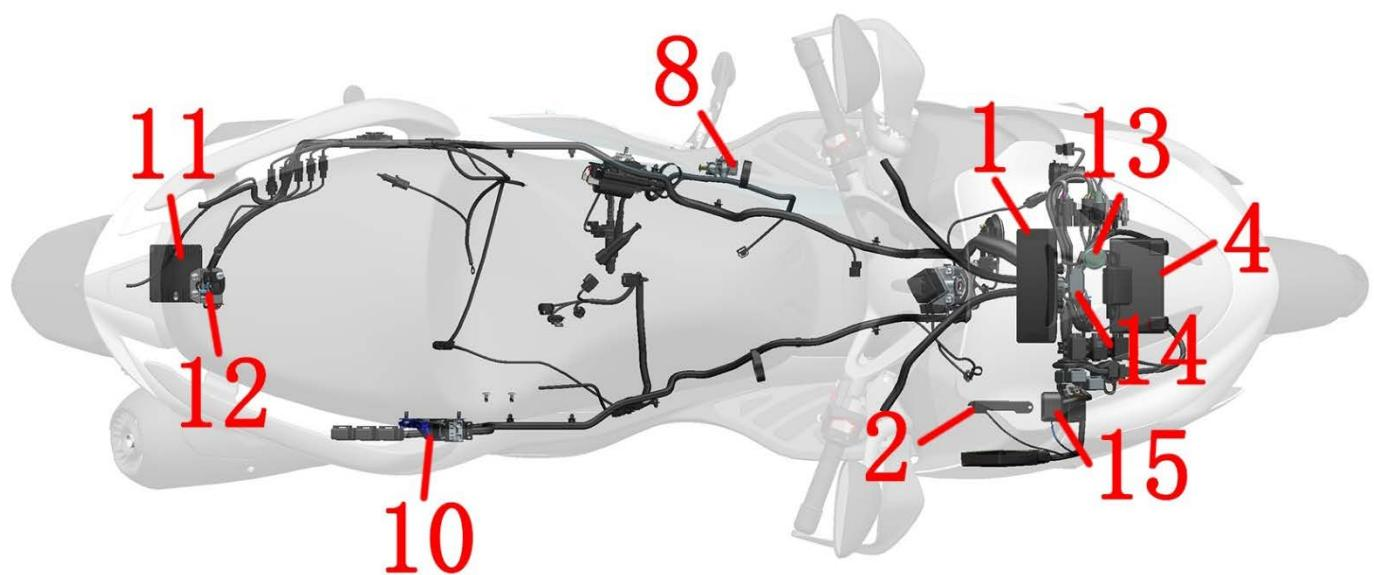
1-TFT Meter 2-Non-inductive antenna 3-Windshield motor controller 4-Battery 5-Main lock 6-PKE 7-Horn
