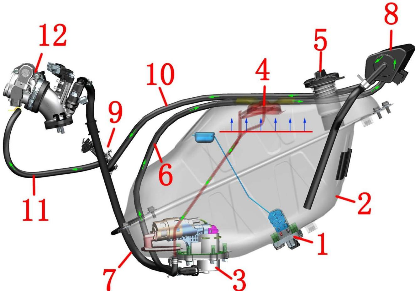
1- Fuel level sensor 2- Fuel tank 3- Fuel pump 4- Oil-air separator (welded inside the fuel tank) 5- Fuel tank cap 6- Adsorption/vent pipe 7-High pressure fuel pipe 8-Carbon tank 9-Carbon tank solenoid valve 10- Solenoid valve intake pipe 11-solenoid valve outlet pipe 12-throttle valve body assembly
