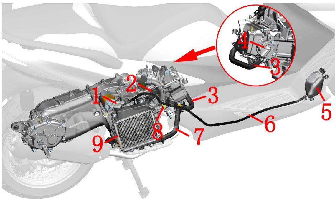
1- water tank water inlet 2-main water tank inlet pipe 3-engine inlet pipe.4-Water pump cover inlet pipe
