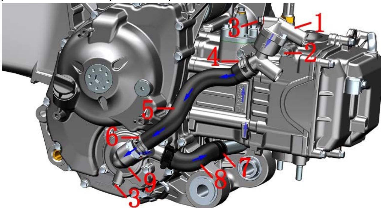
1-Thermostat assembly 2-M6 x 22 Bolt \* 2 3-M6 x 12 bolts \* 2 4-water pipe hoop (φ 25) 5 - Water pump cover inlet pipe 6 -
