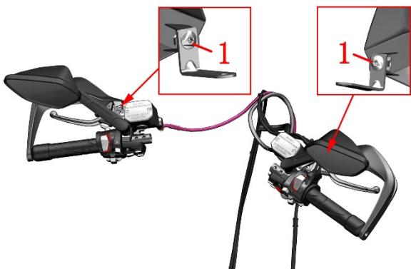
b. Use the 5# Allen to loosen the balance block bolt A 5-8 turns, and remove the left and right hand guards and the balance block assembly.
