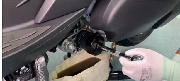
c. Drain the oil inside the fine filter.
