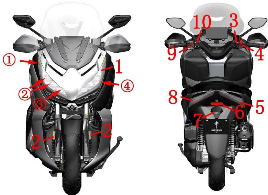
1- Headlights (①-Front turning light position ②-Low beam position ③-High beam position ④-Position light/daytime running light position) 2-Side reflector 3- Right Handlebar Half 4-Right handbar switch 5-Right tail light (right turning light / brake light / position light) 6- Rear reflector 7- License plate light 8-Left rear turning light (left turning light / brake light / position light) 9-Left handle switch 10- Left handlebar half cover
