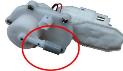
When reassembling, you need to pre-tighten diagonally and then tighten the 5 bolts. Otherwise, the uneven
