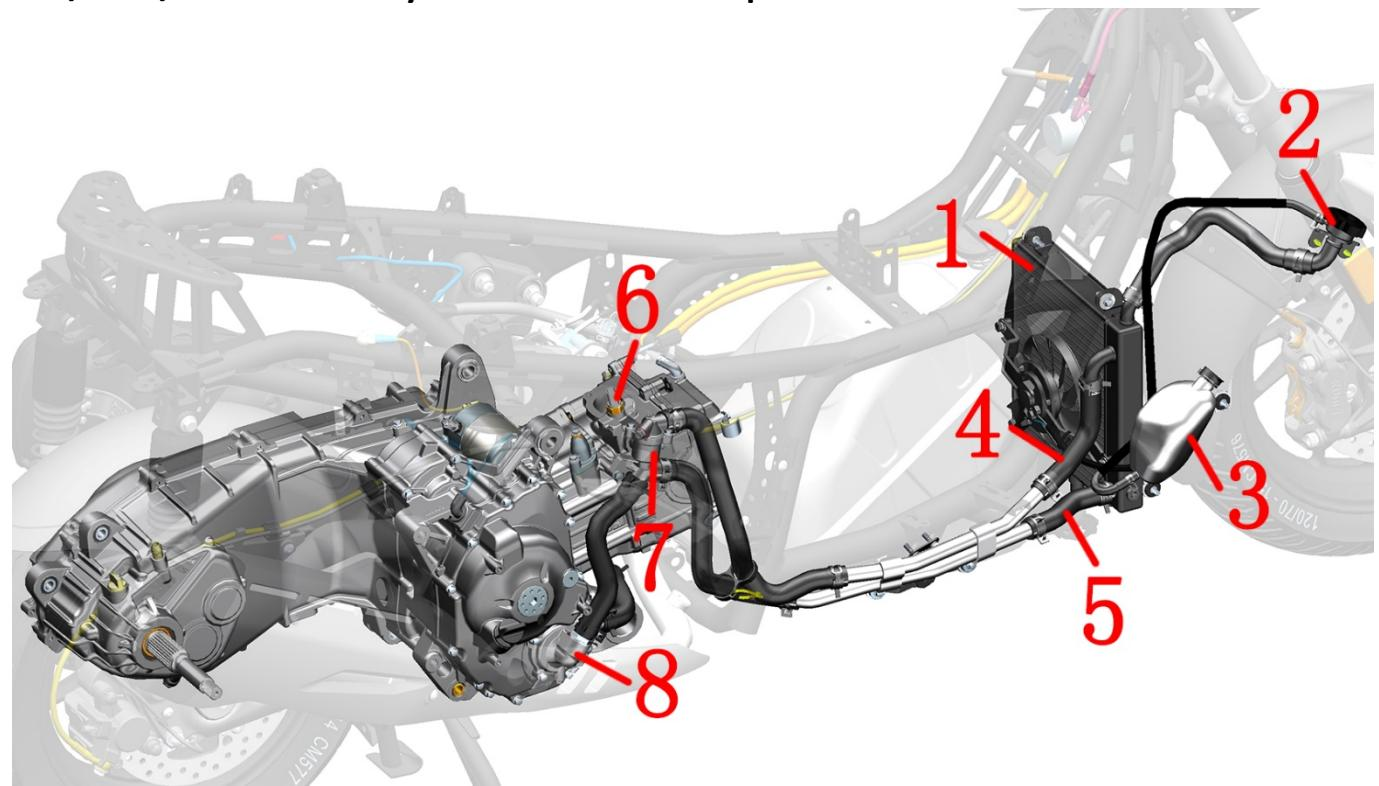
1 - Main water tank 2 - Water tank filler 3 - Auxiliary water tank 4 - Water inlet pipe of main water tank 5 - Water outlet pipe of main water tank 6 - Water oil shared sensor 7 - Thermostat 8 - Water pump cover assembly
