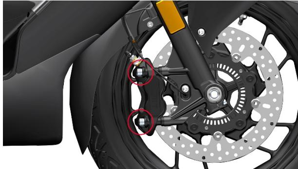
b. Place the oil drain pan under the front disc brake caliper. First remove the screw rubber cap (1), wear waterproof gloves, and then remove the bolt (2) with 8 # box wrench, remove the bolt (3) with 14 # box wrench, and remove two copper washers (4).
