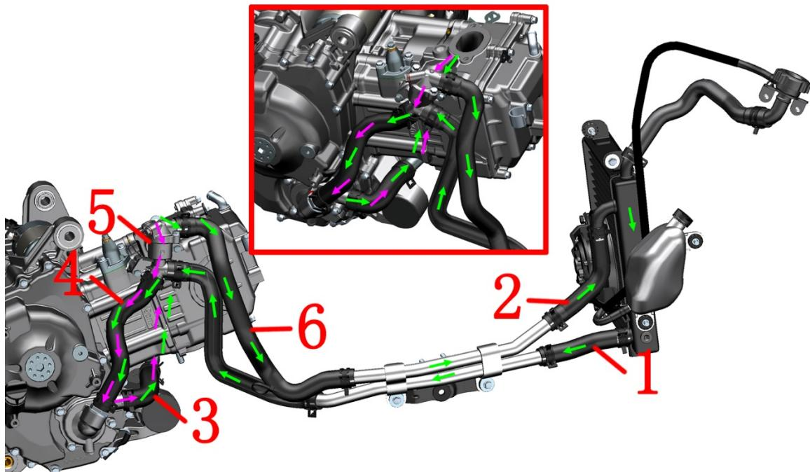
1- Main water tank outlet pipe 2- Main water tank inlet pipe 3- Water pump cover outlet pipe
