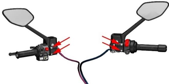
d. Use a Phillips screwdriver to remove the three M4×12 screws b on the left handle switch, then remove the M5×25 limit screw c on the left handle switch. Separate the upper and lower parts of the left handle switch. After pulling off the rubber sleeve, use a Phillips screwdriver to remove the M4×30 limit screw and spring washer.
