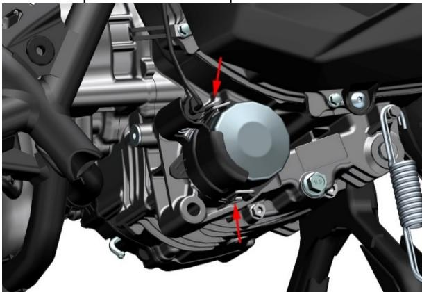
E368 (ETC): Use a T25 Torx wrench to remove an M6 shoulder bolt as shown in the diagram to take off the oil filter guard (ETC).
