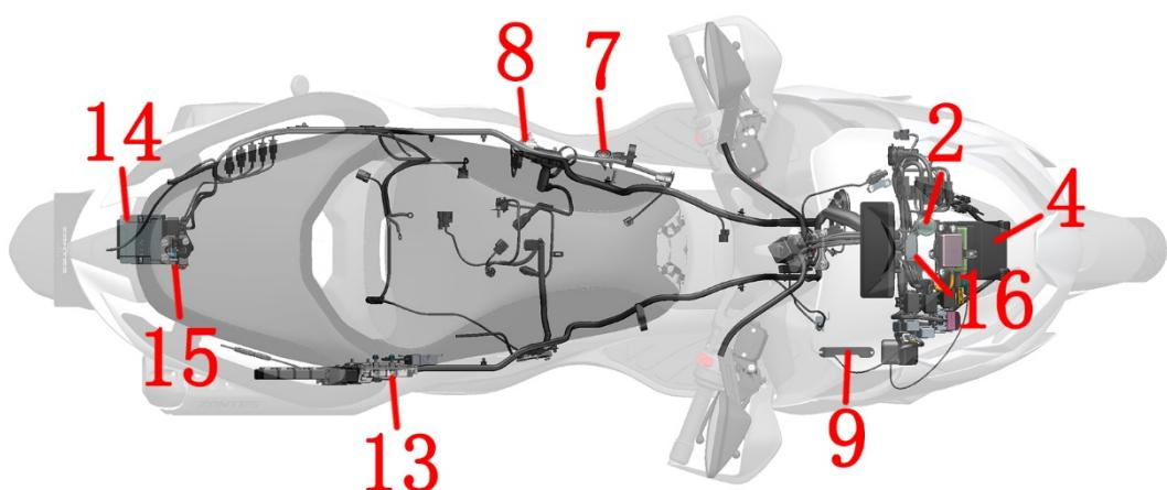
1-TFT instrument 2-Flasher 3-Smart Control Box 4-Battery 5-PKE 6-Horn 7-Side bracket flame-out switch
