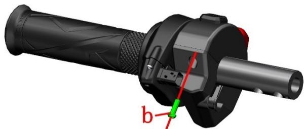
g. Use a Phillips screwdriver to remove two ST2.6×9.5 self-tapping screws (d), one M4×30 screw (e), and a spring washer. Remove the right-hand handle switch. Note: The screws and self-tapping screws are small, so handle them carefully to avoid losing them.
