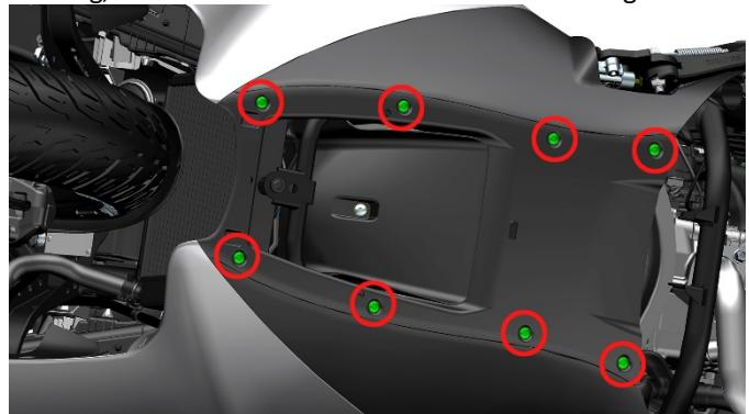
d. Lift out the pedal rubber pad and the pedal rubber pad pressure plate using a one-word batch, press and pull up the pedal rubber pad and the pedal rubber pad pressure plate until the pedal rubber pad and the rear pedal rubber pad pressure plate are taken out. Disassemble the left and right sides in the same way.
