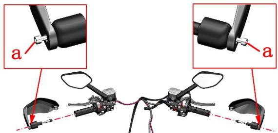
c. Use a #5 Allen wrench to remove the four M6×30 bolts, then take off the left handlebar half cover and rear disc brake master cylinder, and the right handlebar half cover and front disc brake master cylinder.
