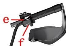
c. When installing the secondary handle bar switch, it is necessary to align the joint surface of the counter-handle bar switch and the main pump of the disc brake with the triangle mark on the handle bar switch, and then use 5# hexagon to tighten 4 M6×30 bolts.
