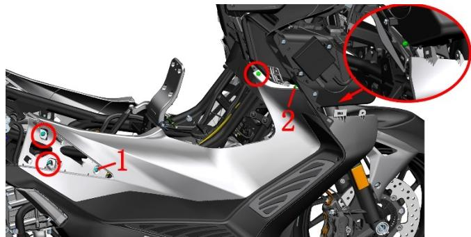
a. To remove the left and right side covers of the fuel tank, first remove the head assembly and tail skirt assembly.
