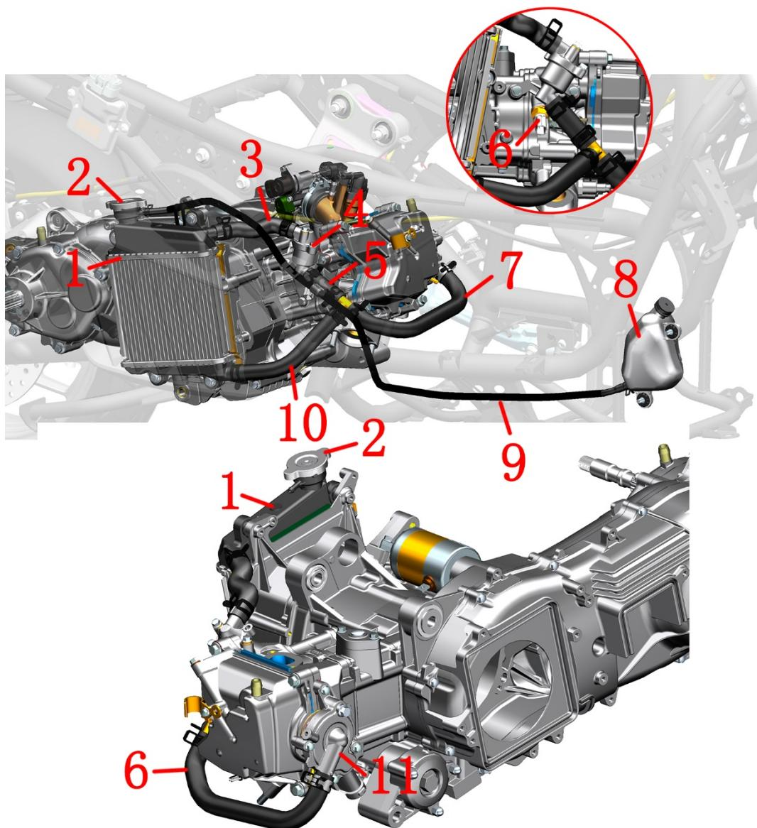
1-Main water tank 2-Water tank filling port 3- Main water tank inlet pipe 4- Thermostat 5- Thermostat outlet pipe
