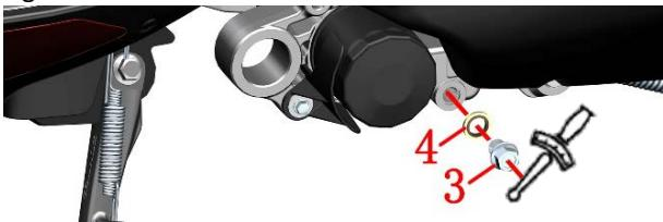
e.Wipe clean the joint surface with a non-woven fabric. Inspect the oil drain bolt(3) whether the joint surface is scratched; if there is any, replace it with a new one, if not, wipe it clean.
