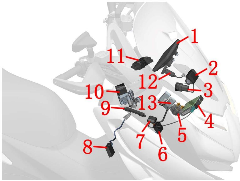
1- TFT instrument 2-Windshield motor controller 3-Dual Port Universal USB Charging Cable 4-PKE 5-Starting relay
