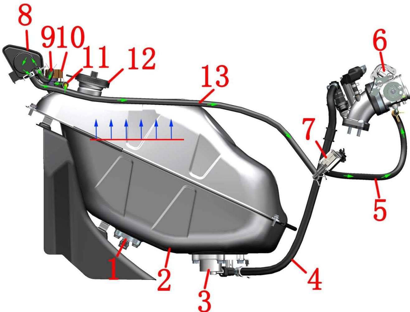
1-Oil level sensor 2-Fuel tank 3-Built-in fuel pump 4-High pressure oil pipe 5-Carbon canister solenoid valve outlet pipe
