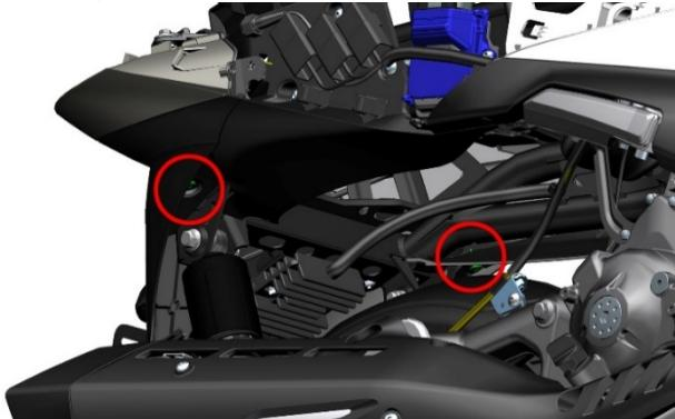
f. Unplug the wire harness connector on the left side of the rear of the motorcycle, arrange the wire harness and remove
