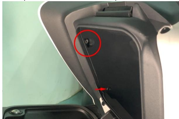
c. Gently pat the left head side panel forward with your hand to remove it, and use the same method to remove the right side panel.
