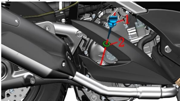
e. Wipe clean the oil dipstick, and turn the oil dipstick(1) and O-ring(2) clockwise by hand to replace the right crankcase cover of the engine.
