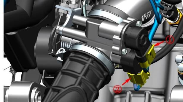
e. Use a short Phillips screwdriver to remove the 2 bolts (3) and the anti-off card (4) that come with the throttle valve body assembly, and then remove the stepping motor (4).
