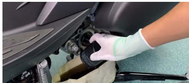
d.Use a clean non-woven fabric to wipe off the remaining oil and impurities on the engine.
