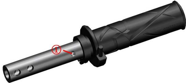
c. When installing the secondary handle bar switch, it is necessary to align the joint surface of the counter-handle bar switch and the main pump of the disc brake with the triangle mark on the handle bar switch, and then use 5# hexagon to tighten 4 M6×30 bolts.
