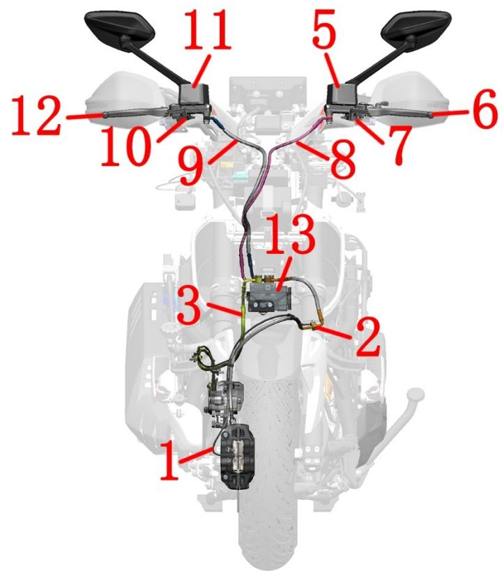
1-Wheel speed sensor (front wheel) 2-FC-HU brake hosepipe 3-RC-HU brake hosepipe 4-Wheel speed sensor (rear wheel)
