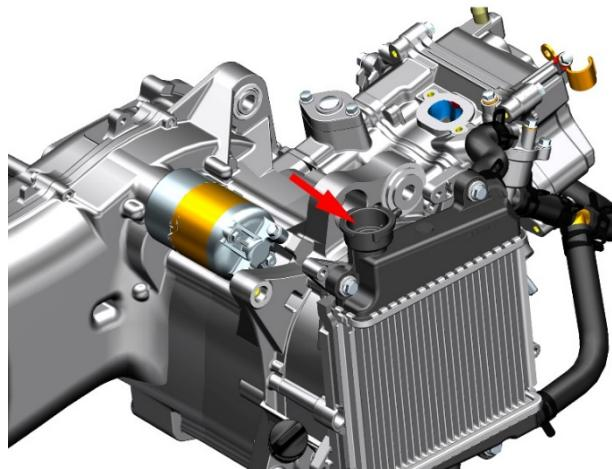
e. Tighten the filler cap of the Radiator. Tighten the exhaust bolt; torque: 8~10N.m (0.8~1 kgf.m, 6~7 lbf.ft).
