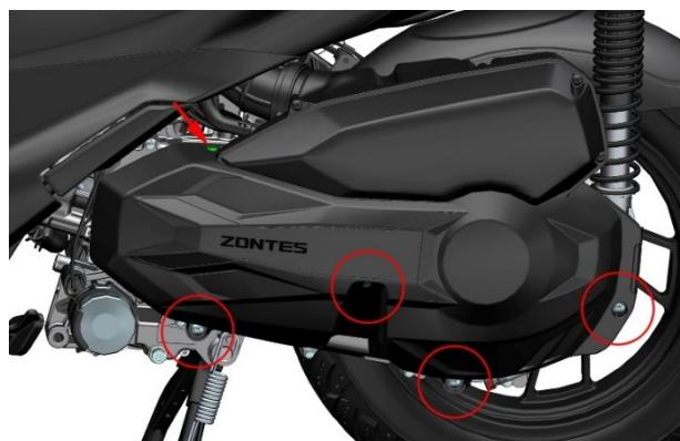
c. Pull out the 2 mushroom buckles on the air filter decoration cover and remove the air filter decoration cover.
