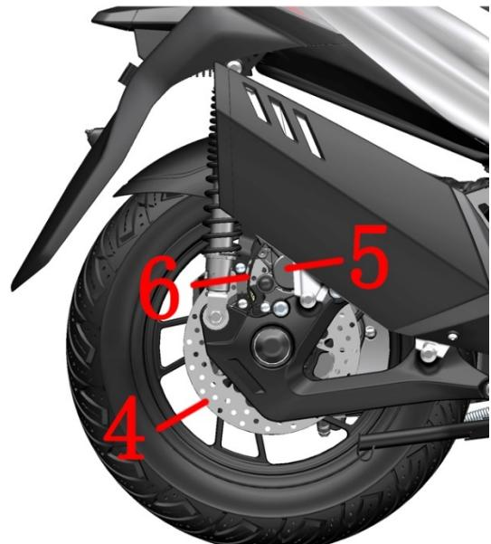
1-Front brake disc components 2-Wheel speed sensor (Font Wheel) 3-front disc brake caliper
