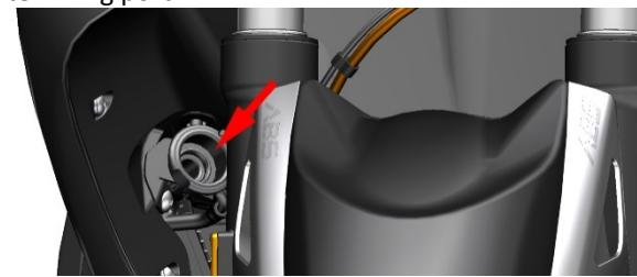
d. Tighten the filler cap of the Radiator. Tighten the exhaust bolt; torque: 8~10N.m (0.8~1 kgf.m, 6~7 lbf.ft).
