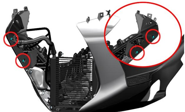
c. Press and pull out the 8 expansion nails at the bottom of the fairing, and remove the bottom of the lower fairing.
