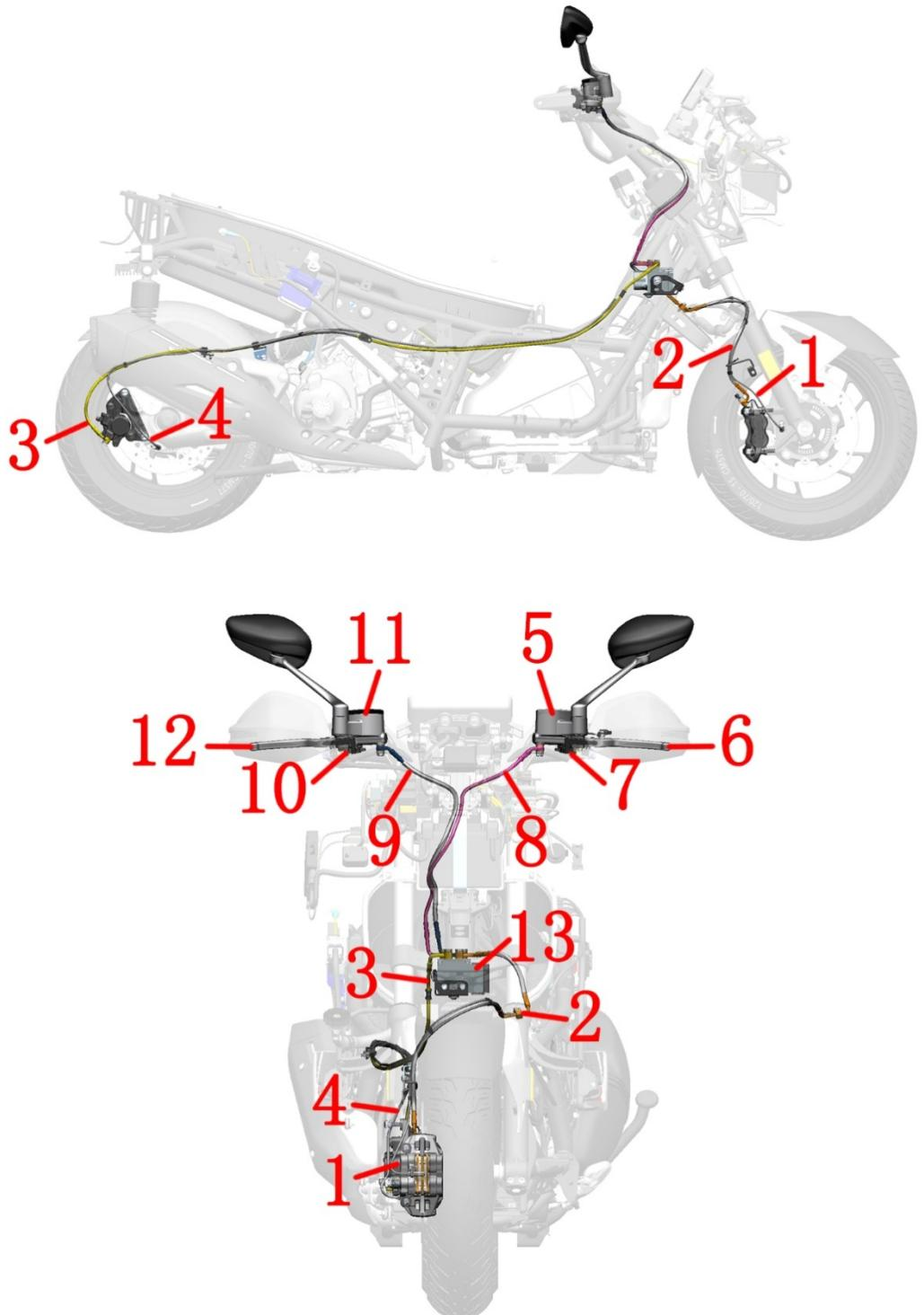
1-Wheel speed sensor (front wheel) 2-FC-HU brake hose 3-RC-HU brake hose 4-Wheel speed sensor (rear wheel)
