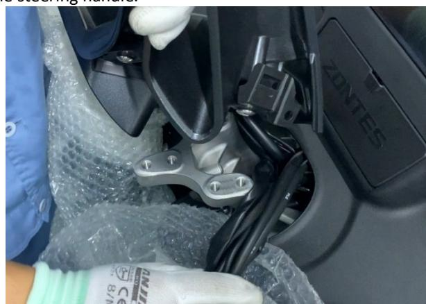
g. Use the 4# inner hexagon to remove the bolts on the left and right storage box brackets.
