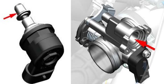
g. Install the stepper motor back to the valve body, paying attention not to miss the sealing ring. Plug the plug back in.
