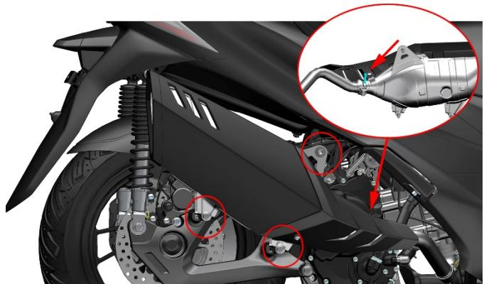
2. Check for nut and bolts at the muffler
