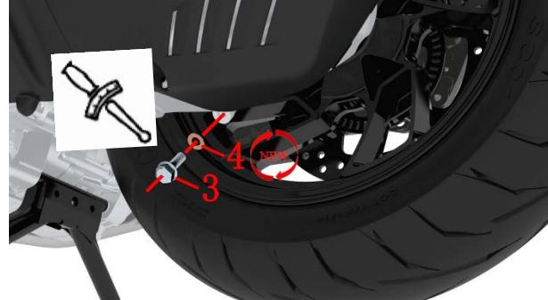
c. Remove the oil drain bolt(3) and the copper pad(4).
