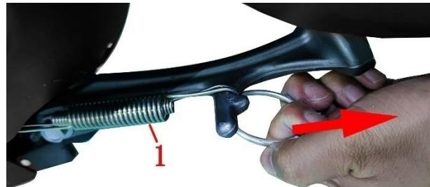
c. Grasp the side bracket with one hand, and pull it in the direction of the arrow with the other hand to remove the spring.
