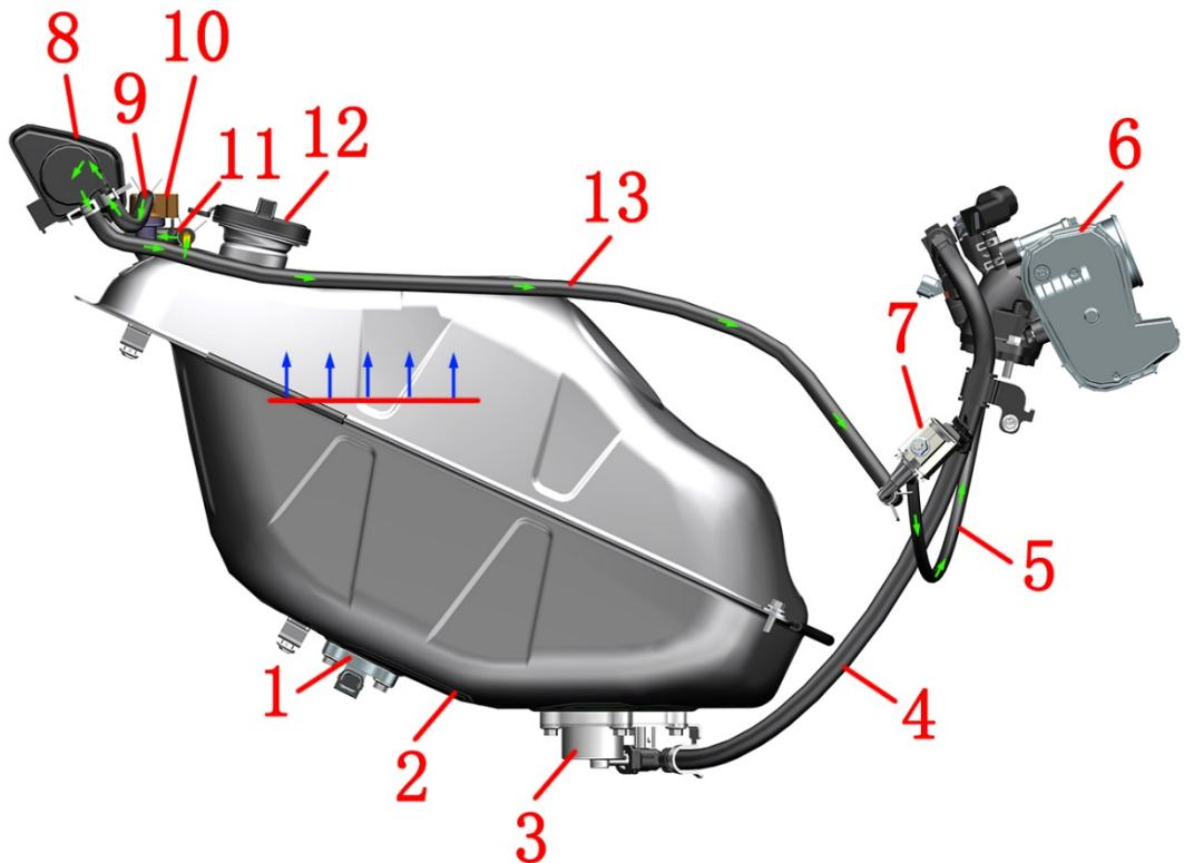
1-Oil level sensor 2-Fuel tank 3-Built-in fuel pump 4-High pressure oil pipe 5-Carbon canister solenoid valve outlet pipe
