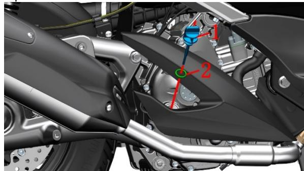
e. Apply a layer of oil to the new fine filter seal and install it on the engine. Torque: 20 N.m (2 kgf.m, 15 lbf.ft).
