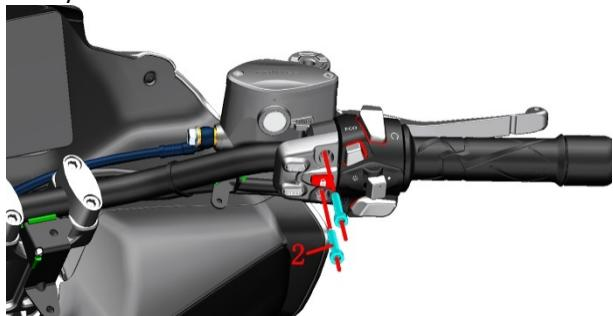
d. Tilt the front brake main pump so that the bolt(1) faces upward, wear waterproof gloves and use a 12# sleeve to remove the bolt(1), remove the copper pad(3), remove the FMC-HU oil pipe, and remove the brake fluid in the main pump. Pour out. Bolt(1) Standard torque: 32N.m (3.3kgf.m, 24 lbf.ft).
