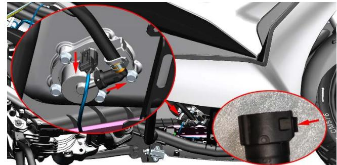
If the fuel pump needs to be removed from the vehicle, the fuel pump can be used to drain the fuel in the fuel tank. After lifting the vehicle, press the plug buckle as shown in the figure to pull out the cable. Remove 5 bolts from the bottom with a 10# sleeve, and then remove the fuel pump after removing the high-pressure fuel pipe bracket.
