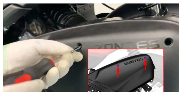
c. Use a Phillips screwdriver to remove the 4 screws that fix the housing of the air filter.
