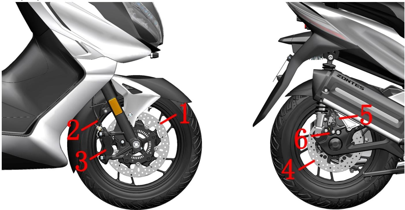
1-Front brake disc components 2-Wheel speed sensor (Front Wheel) 3-front disc brake caliper
