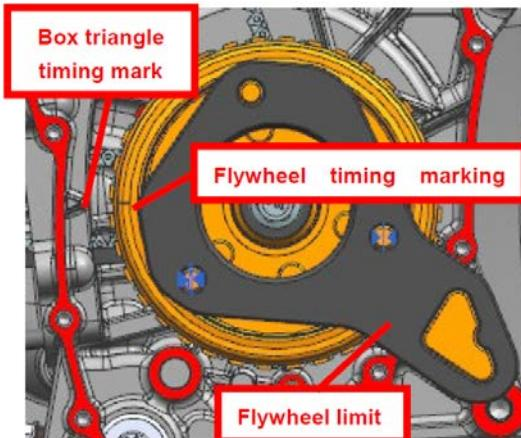
b. Tighten the timing chain, check again and align the line immediately after the "T" mark on the flywheel with the triangle mark on the box.
