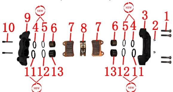
1- Bolt 2- Circlip 3- Inner side caliper housing 4-φ30 oil seal 5-φ30 dust seal 6-φ30 piston 7- Disc brake pad 8- brake spring 9- Out side caliper housing 10-Pin 11-φ34 oil seal 12-φ34 dust seal 13-φ34 piston
