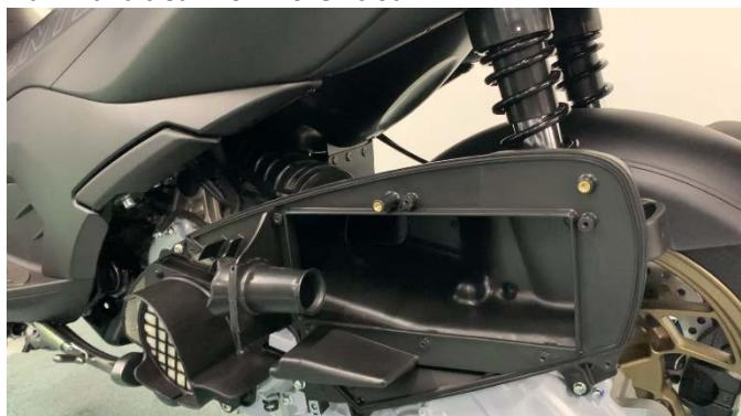
c. Replace the new filter element and sealing strip.
