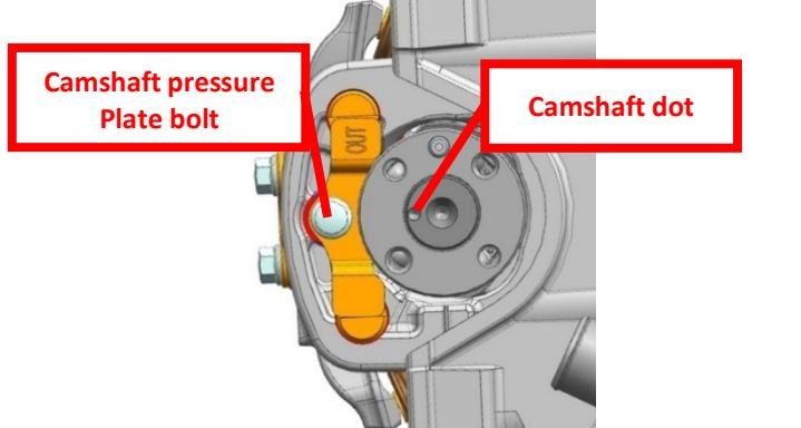
The bolt center is aligned with the dot center
