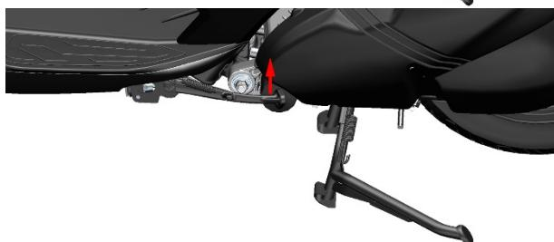
c. Check whether the flameout switch function is normal.
