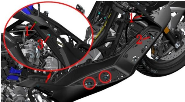
f. Pull apart the right pedal assembly, and use an 8# sleeve to remove the auxiliary water tank. Place the auxiliary water tank well, the left pedal assembly can be removed by referring to the right pedal assembly.
