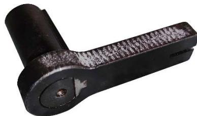
Remove the rotor from the engine, install the flywheel gauge as shown in Figure 1, and check whether the marking line on the side of the rotor is in the slot (Figure 2).
