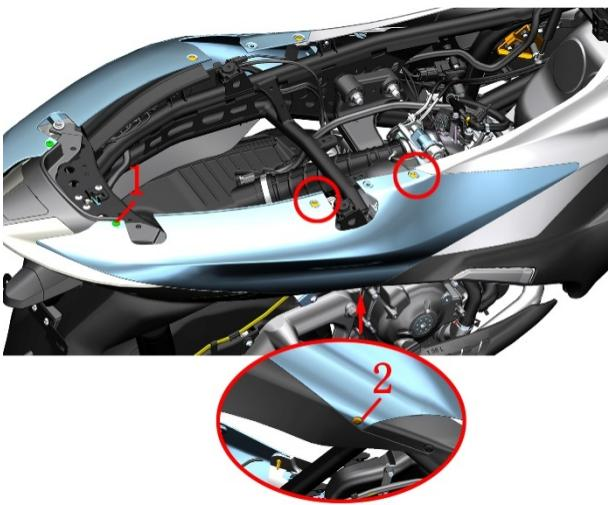
b. Gently tap the tail skirt back with your hand to remove the right rear tail skirt assembly. Pay attention to the buckle in the circle as shown in the picture when installing.
