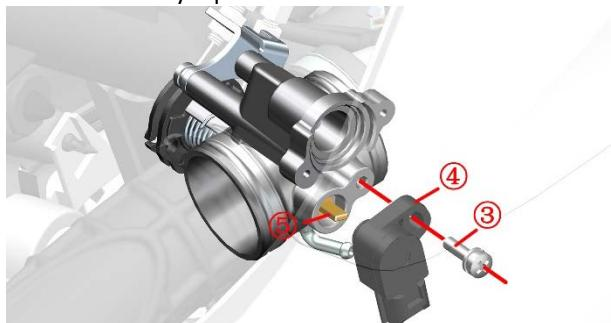
Simple test method: connect the whole vehicle to the diagnostic instrument, press the flameout switch (no need to ignite), turn the throttle handlebar from the initial position to full open, this process to see if the throttle position signal follows the change from 0 to 100.
