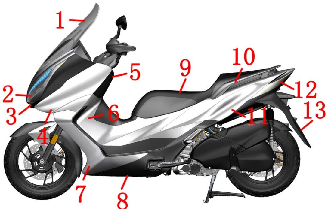
1. Windshield 2. Headlights 3. Lower part of the hood 4. Left plate of the hood 5. Front left panel 6. Left side cover 7. Left pedal decorative cover 8. Lower fairing left 9. Seat 10. Left rear armrest 11. Left part of the tail skirt
