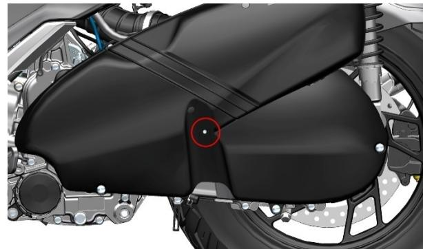
c. Use a #4 inner hexagon or T30 Torx wrench to remove the 3 M6×14 bolts as shown in the figure. Press down the center pin of the expansion nail on the air filter decorative cover with a #4 inner hexagon, then remove the expansion nail. Remove the decorative cover.
