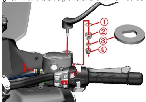
c. After grasping the front brake main pump, remove the 2 bolts (2) with a 5# inner hexagon, and remove the right auxiliary switch.
