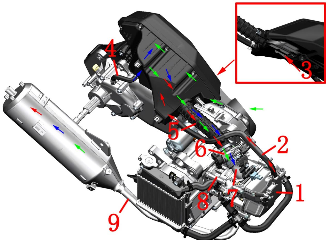
1- Cylinder head 2-Cylinder head exhaust pipe3- Air filter intake inlet 4-Crankshaft Box exhaust pipe5-Air filter outlet pipe6- Throttle valve body assembly 7-Intake manifold8- Cylinder 9- Muffler
