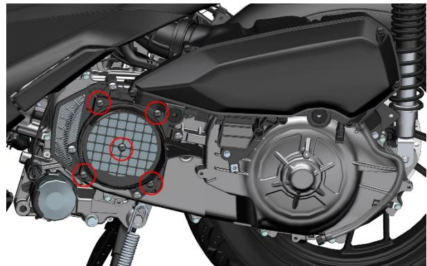
b. Remove the sponge and replace it with a new filter element. Note that the black side faces the engine and the white side faces outward.
