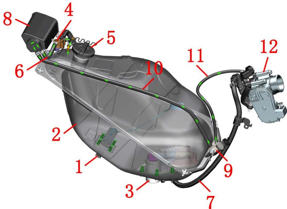
1- Fuel level sensor 2- Fuel tank 3- Fuel pump 4- External oil and gas separator 5- Fuel tank cap 6-Adsorption/vent pipe 7-High pressure fuel pipe 8-Carbon tank 9-Carbon tank solenoid valve 10- Solenoid valve intake pipe
