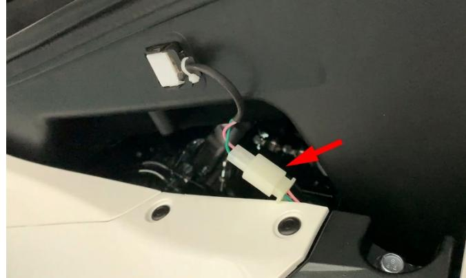
d. Unplug the plug of the stepping motor (1) and the sensor (2)
