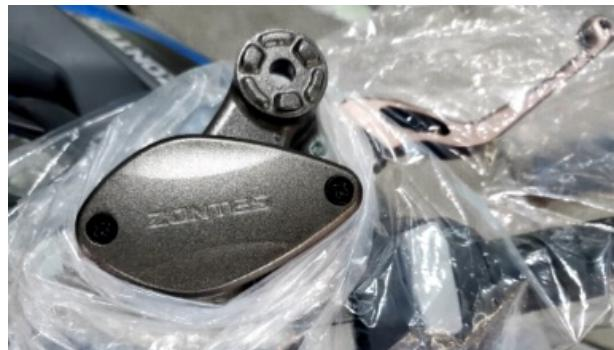
d. After wearing waterproof gloves, use a Phillips screwdriver to remove the bolt①, and remove the upper cover②, the cover③, and the sealing rubber gasket④.
