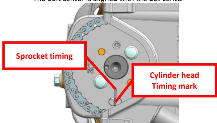
The timing of the sprocket is aligned with the timing of the cylinder head
