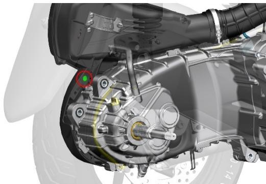
b. Use 4# inner hexagon or T30 Torx wrench to remove the M6×14 bolt as shown in the figure. The bolt here cannot be removed temporarily, just loosen it completely.
