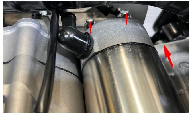
e. When reassembling, make sure not to omit the O ring that comes with the starter motor, and align the teeth of the electric starter reduction gear. Note that the O-ring needs to be correctly assembled into the box, as it will cause leakage if cut edges occur. Torque of the two bolts for fixing the starter motor:  $12\pm1.5\text{ N.m}$  ( $1.2\pm0.2\text{ kgf.m}$ ,  $9\pm1\text{ lbf.ft}$ ). And mark with a marker.
