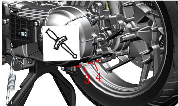
d. Remove the oil drain bolt(3) and the copper pad(4).
