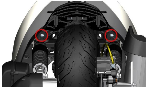
c. Use a 4# inner hexagon to remove the two M6x14 bolts on the left and right sides of the motorcycle that fix the taillights.
