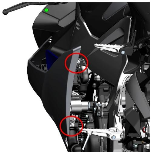
h. On the left side of the vehicle, carefully pull the buckle or mushroom peg indicated by the arrow from top to bottom, and remove the left bracket panel assembly.
