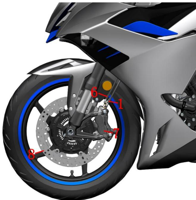
1-Brake hose left and right caliper interchange section 2-Disc brake caliper (front right) 3-Wheel speed sensor (front wheel)
