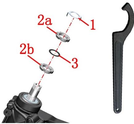
c. If the steering is heavy, loosen the adjusting nut (2b) counterclockwise. Tighten clockwise to 35 N.m (3.6 kgf.m, 26 lbf.ft), then 1/4 turn counterclockwise, then 13 N.m (1.3 kgf.m, 10 lbf.ft).
