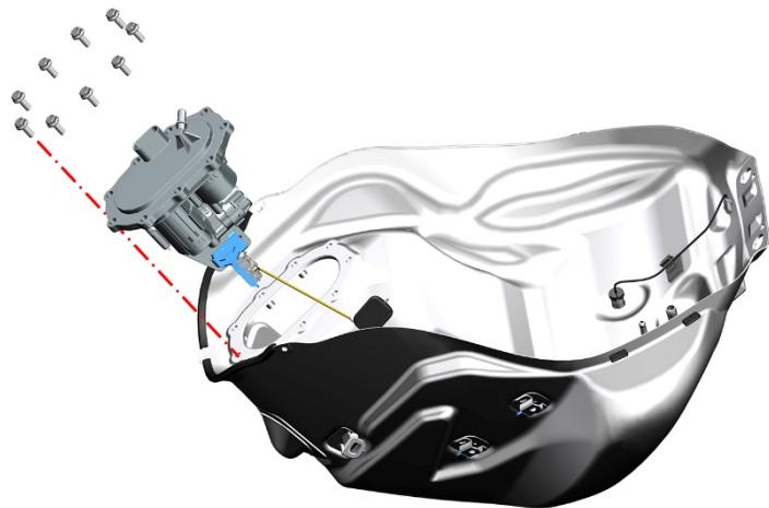
When reassembling, it is necessary to pre-tighten diagonally and then tighten 9 bolts, otherwise the uneven compression of the sealing rubber ring of the fuel pump will easily lead to leakage and potential safety hazards.
