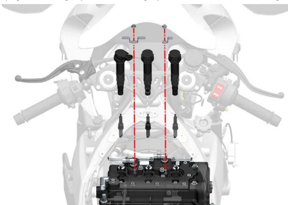
When installing the ignition coil back, first insert the ignition coil back into the bottom, and turn the ignition coil plug towards the position shown in the figure above, then put it back into the pressure plate, and put the nut back tight, and the torque standard is  $11.5\pm1\text{N.m}$ .
