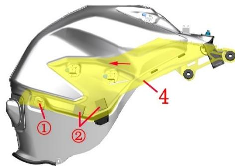
e. Remove the rubber wire buckle (8) first. Use a 10# open-end wrench to remove 2 M6×35 bolts, and remove 2 nuts (5), 2 flat washers (6), 2 laminating glues (7), 2 bushings (11), 1 bracket (10) and 2 pads (9) respectively.
