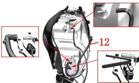
f. Refer to the steps in "Replacing the Spark Plug" to remove the entire air filter. Press and hold the tubing buckle to pull out the high-pressure tubing (12).
