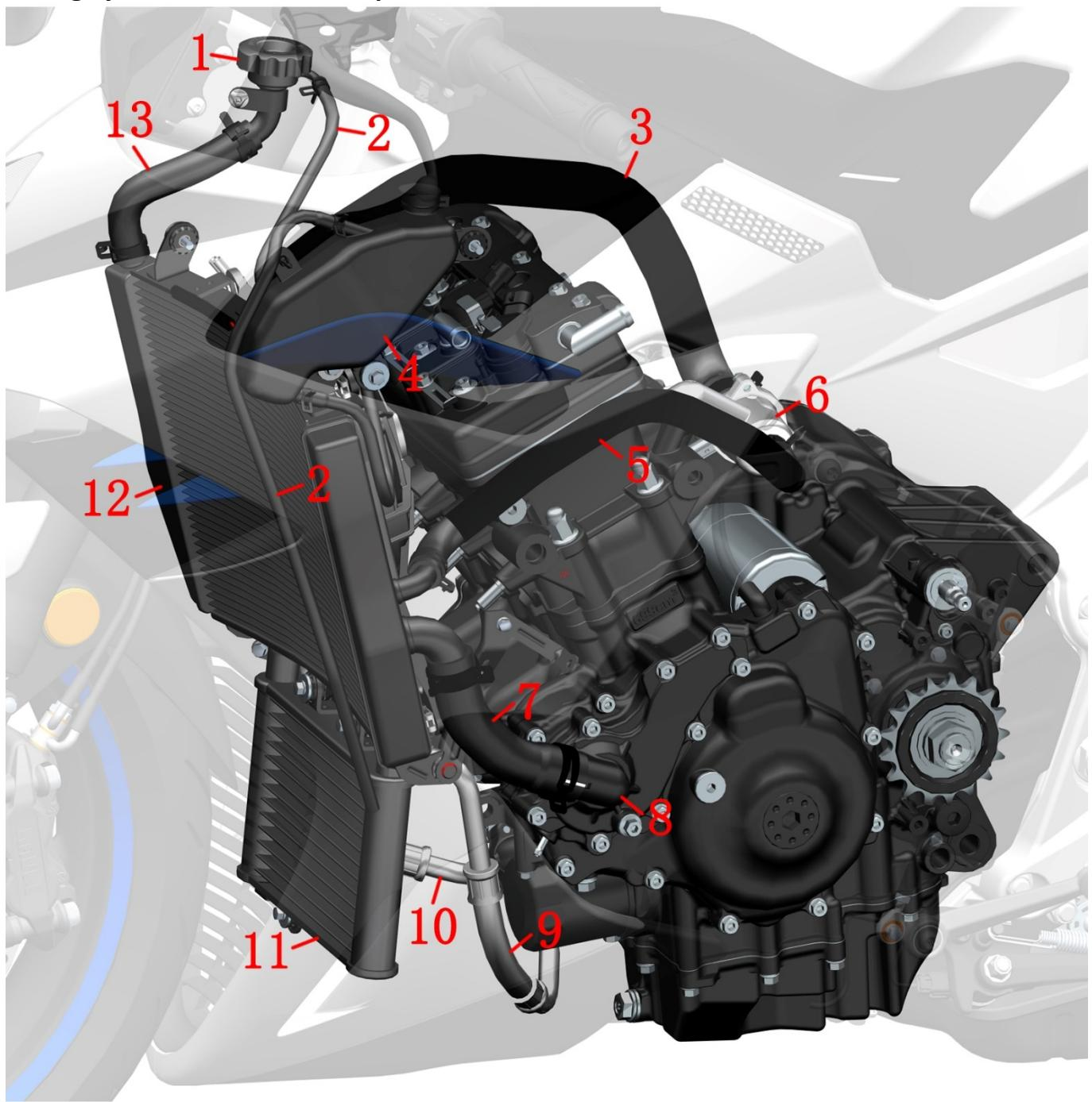
1- ZT703-RR Water Tank Refill 2- ZT310-R Auxiliary Water Tank Leaking Pipe 3-ZT703-F Main Water Tank Inlet Pipe 4- ZT703-RR Auxiliary Water Tank 5- ZT703-F Small Circulation Water Pipe 6- ZT703 Thermostat 7- ZT703-RR Engine Water Inlet Pipe 8- Water Pump Cover Assembly 9- ZT703-RR Engine Outlet Pipe (TFL) 10- ZT703-RR Engine Inlet Pipe (TFL) 11- ZT703-RR Oil Cooler (13 Tubes) 12- ZT703-RR Main Water Tank (38 Tubes) 13- ZT703-RR Water Tank Water Filling Port Connected Water Pipe
