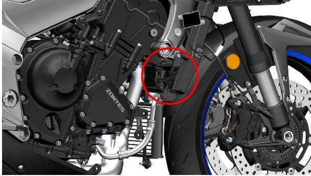
c. Use the 8# sleeve to remove 2 pieces of M6×22 bolts (9) and 1 piece of M6×30 bolt (10) that fix the oil cooler.
