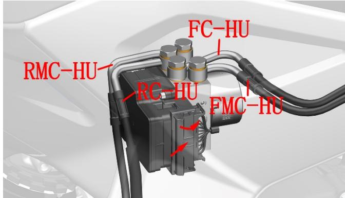
FMC-HU: Front disc brake main pump - hydraulic control unit
