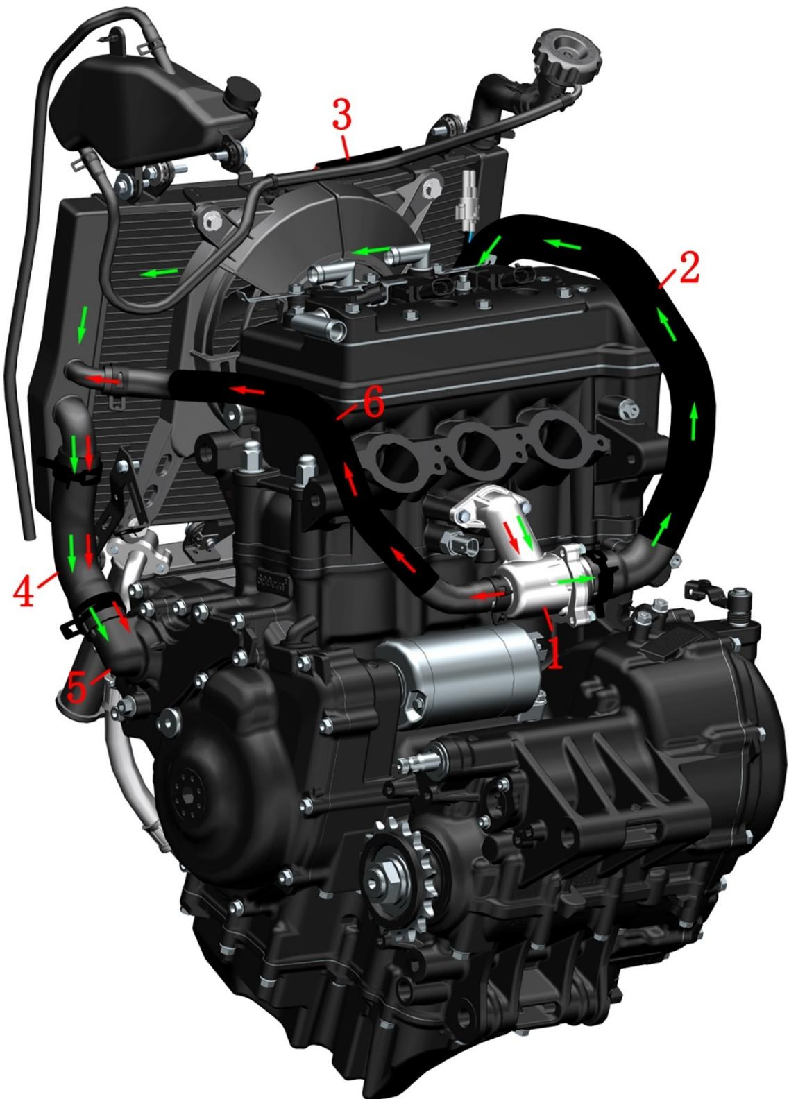
1-Thermostat assembly 2-Main water tank inlet pipe 3-Main water tank 4-Engine water inlet pipe 5-Water pump cover assembly
