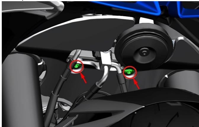
b. Remove the two M6 bolts with the 8# sleeve, loosen the FMC-HU hose, the forward brake duplex joint fixing bracket, and the FC-HU hose, and take out the hose along the frame after removing the hose connection of the hydraulic control unit.
