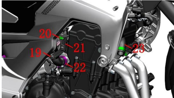
c. Use a T50 torx wrench with a middle hole to remove the bolts (19) of 1 M10×20 and 2 bolts (20) of M10×35 that fix the left hanging piece (24) of the main frame, and remove the left hanging piece (24) of the main frame; Then use the 8# sleeve to remove the bolts (1) of the two M6×22 fixing the thermostat (25), and take out the thermostat assembly (25).
