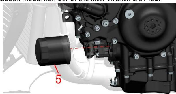
b. Drain the oil from the filter.
