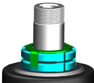
f. Assemble the orientation assembly back.
