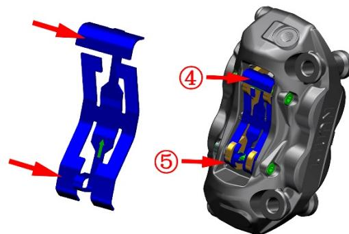
j. hold down the piece at the point of the arrow (4) to the direction of the arrow with the hand, and insert the pin (2) into the hole position to fix the brake pad (1). Tighten the pin (2) with a T25 hexagon torx wrench.
