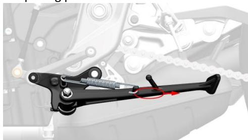
c. Grab the side bracket with one hand and pull the other hand in the direction of the arrow to remove the spring.
