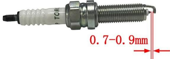
d. If necessary, the gap can be adjusted by bending the side electrode, and pay attention to the strength when adjusting.
