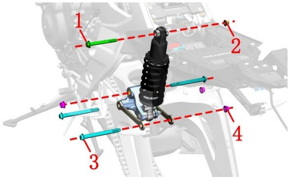
b. One person uses a 14# sleeve to fix the head of the bolt, and one person uses a 14# sleeve to remove the nut, remove the bolt, and remove the rear shock absorber and triangle bar assembly. Nut torque:  $65\pm5\text{N.m}$  ( $6.6\pm0.5\text{ kgf.m}$ ,  $48\pm4\text{ lbf.ft}$ )
