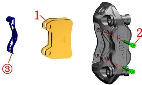
c. Remove the shrapnel (3), remove the brake pad (1).
