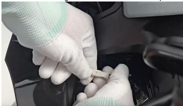
f. Use an 8# torx wrench to remove the two M6×12 hexagonal bolts (1) to remove the rearview mirror, pay attention to the rearview mirror before removing the bolt to stabilize the rearview mirror to prevent it from falling. The method of removing the left and right mirrors is the same.
