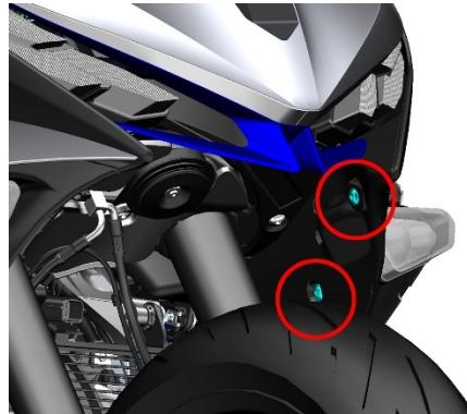
d. Carefully pull the buckle or mushroom peg at the arrow indication and remove the upper component of the left surround.
