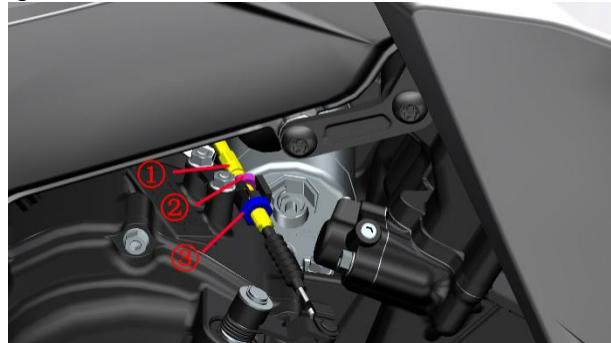
c. If the above two adjustments are invalid, a new clutch cable needs to be replaced.
