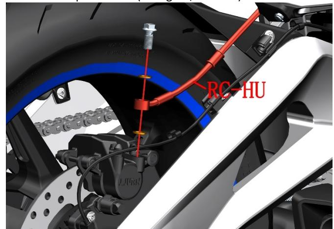
b. Remove the rear caliper and brake pads first by following the steps for removing the rear wheel and replacing the brake plate.
