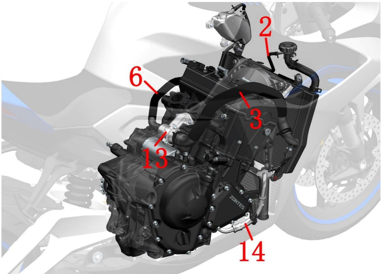
1-Main water tank water inlet 2-Sub water tank connecting water pipe 3-Main water tank water inlet pipe 4-Water tank water inlet connecting water pipe 5-Auxiliary water tank 6-Small circulating water pipe 7-Main water tank 8-Auxiliary water tank leaking pipe 9-Engine water inlet pipe 10-Water pump cover assembly 11-Oil cooler 12-Engine oil outlet pipe 13-Thermostat 14-Engine oil inlet pipe.
