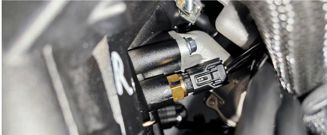
The two-pin resistance value of the multimeter at room temperature is:  $3.74\sim1.22\text{k}\Omega(10\sim40^\circ\text{C})$ ;  $1.22\sim0.27\text{k}\Omega(40\sim90^\circ\text{C})$ .
