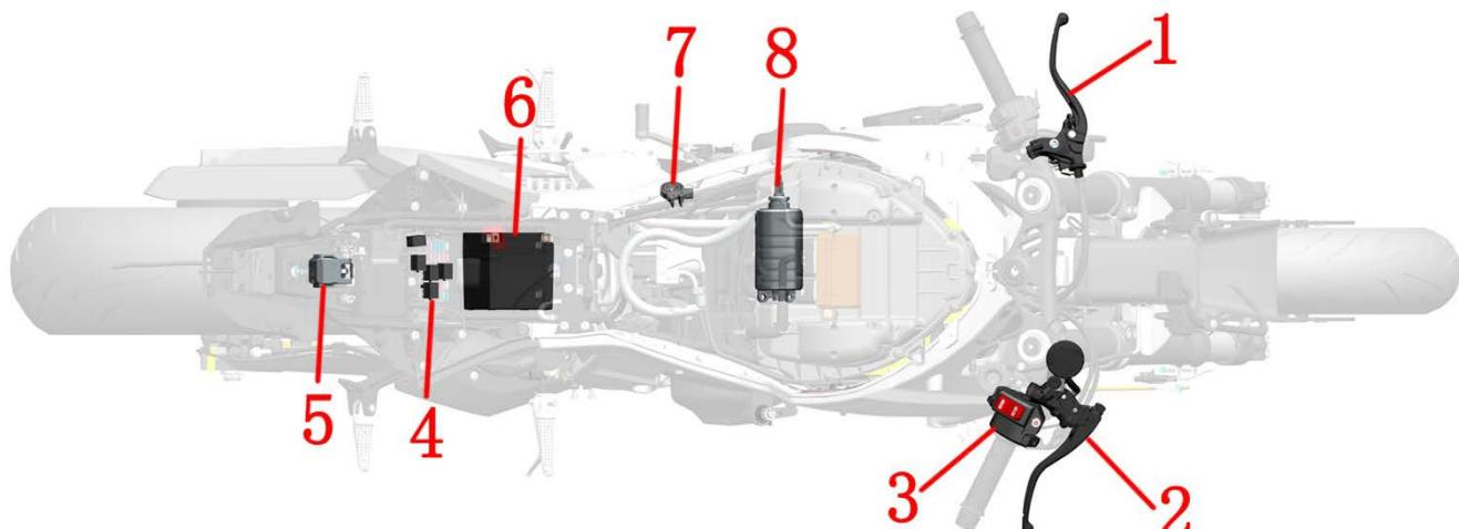
1-Clutch rocker arm (clutch switch) 2-Front disc brake main cylinder (front brake switch) 3-Right hand handle switch 4- Fuse box 5- Starter relay 6-Battery 7- Side bracket power out switch 8- Starter motor
