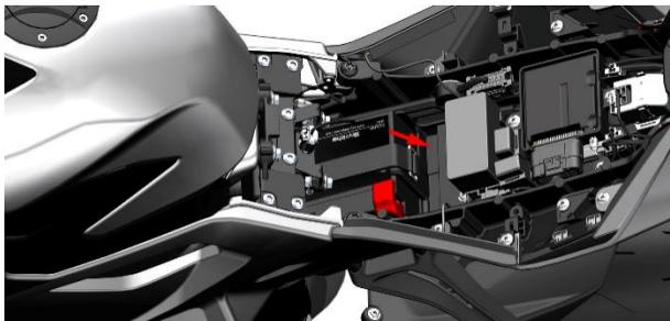
b. After pulling out the battery, first disconnect the negative terminal by removing the black protective cap, followed by the positive terminal. Then, remove the battery.
