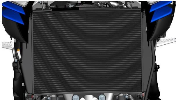
b. Use a flat carving knife or a small flathead screwdriver to straighten the deformed fins. If the fins are deformed by more than 20%, a new radiator will need to be replaced.
