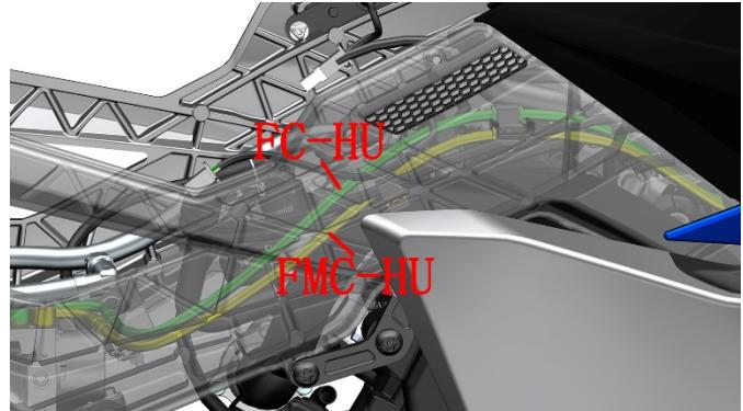
e. Check whether the cable is damaged, if there is wear and tear on the cable sheath, it needs to be wrapped with electrical tape to avoid short circuit and motorcycle failure. Wrap it with electrical tape to avoid short circuits and motorcycle breakdowns.
