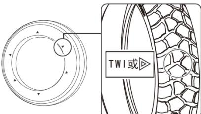
The sidewall triangle ( $\Delta$ T.W.I.) markings indicate the position of the wear strips. If it is worn to the marked point, it means that it has been worn to the limit, and it will be a safety hazard to continue driving, and it must be replaced with new tires of the same specification.
