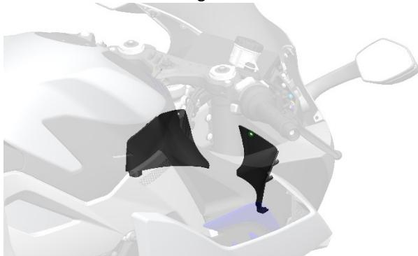
e. After removing the interior surrounding, remove the joints of the left and right mirrors from the interior panels.
