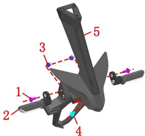
e. First, use a Phillips screwdriver to remove one non-standard Phillips screw (1) that fixes the license plate light, then remove the license plate light (2), remove the rear reflector (3) from the rear fender assembly, and then take out two splint nuts (4); For more information, please watch the video of the rear fender assembly disassembly.
