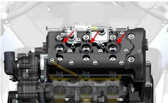
g. Remove the spark plug by rotating it counterclockwise with the vehicle-mounted tool or the special 14# spark plug sleeve.
