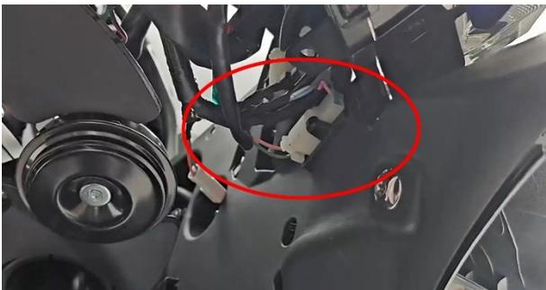
i. Use an 8# torx wrench to remove the two M6×12 hex bolts (1) that fix the windshield assembly on the left and right sides, and use a T25 torx wrench to remove the two M6×12 bolts. Note: Hold the panel assembly steady when disassembling to prevent it from falling directly to the ground.
