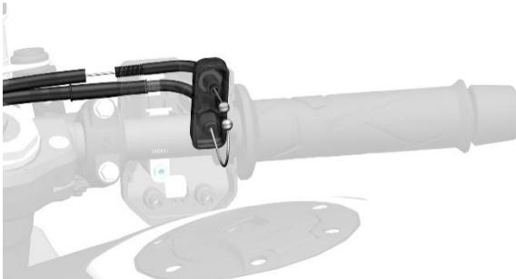
c. If the fault of high resistance cannot be solved after lubrication, the throttle cable needs to be replaced.
