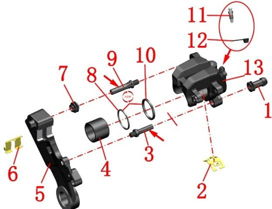
1-Caliper mounting plate pin cap 2-elastic card 3-lower sliding shaft 4-piston 5-caliper mounting plate 6-card 7-caliper pin cap 8-dust seal 9-upper sliding shaft 10-oil seal 11-air nozzle 12-air nozzle rubber cap 13-caliper housing
