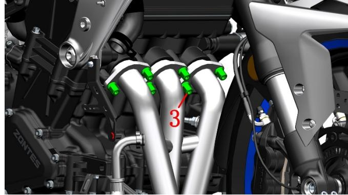
h. Use the 6# hexagon to remove the 2 bolts (8) that fix the tail ends of the mufflers on both sides, and take out the bushing (12). Remove the muffler assembly. Note: When removing the bolt (8), the front part of the muffler needs to be supported, and when completely removed, it is necessary to pay attention to the engine exhaust port gasket (4) where the muffler is connected to the engine.
