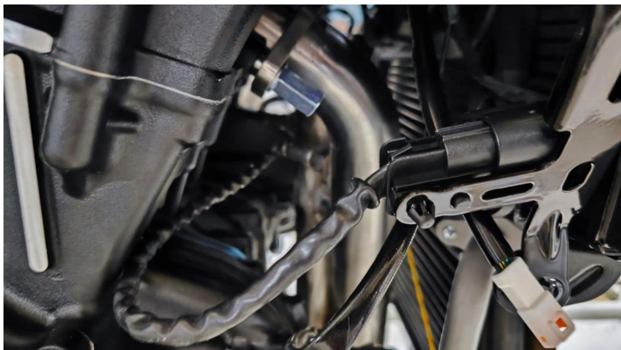
After removing the cover, you can see that the oxygen sensor is fixed as shown in the figure above, the mushroom head is extruded from the fixing hole, the oxygen sensor connection plug can be unplugged, and the pin resistance corresponding to the purple line and the white wire of the oxygen sensor can be measured with a multimeter, and the standard value is  $12.5\pm1.7\Omega$ ; If the resistor is small or infinite, it needs to be replaced.
