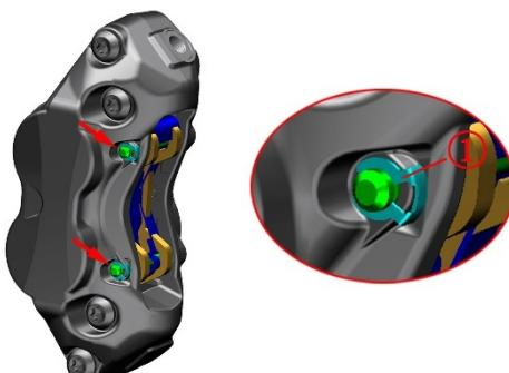
b. Use a T25 socket torx wrench to remove the upper pin (2) and then the lower pin in turn.
