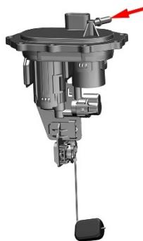
If the fuel pump needs to be removed from the vehicle, the fuel tank can be emptied with the suction pump. Flip the fuel tank assembly to the back and remove the 9 bolts with the 8# or 10# sleeve to remove the fuel pump.
