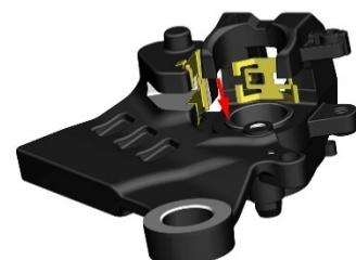
c. Grasp the outer brake pad with the left hand, insert the pin (2) with the right hand, and be careful not to insert it to the end. After the inner brake pad is put in place, insert the pin shaft to the end and lock the pin (2) with a T25 torx wrench, and replace the circlip (1) with needle-nose pliers.
