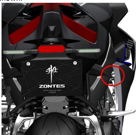
e. On the right side of the vehicle, carefully pull the buckle or mushroom staple indicated by the arrow from top to bottom, and remove the right bracket panel assembly.
