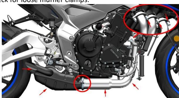
b. If there is a slight air leakage at the connection between the engine and the muffler, you can first try to tighten the exhaust nut (3) with 6# hexagon socket; If the problem is not resolved, the muffler needs to be removed and replaced with a new engine exhaust gasket (4). The specific disassembly method can refer to the disassembly of the muffler.
