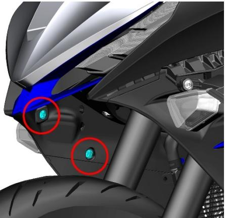
b. Carefully pull the buckle or mushroom staple at the point indicated by the arrow and remove the upper assembly of the right surround.
