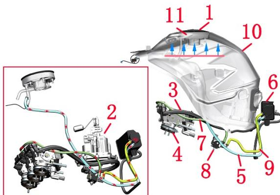
1-Fuel Tank Lock 2-Fuel Pump 3-High Pressure Oil Hose 4-Throttle Valve Body Assembly 5-Adsorption/Snorkel 6-Carbon Canister 7-Solenoid Valve Out 8-Air Hose 9-Carbon Canister Solenoid Valve 10-Fuel Tank 11-Air-Oil Separator (Inside Tank Lock)
