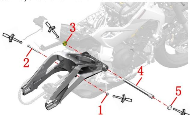
c. Use a 13# open-end wrench to remove the two bolts and nuts in the grooves of the rear flat fork.
