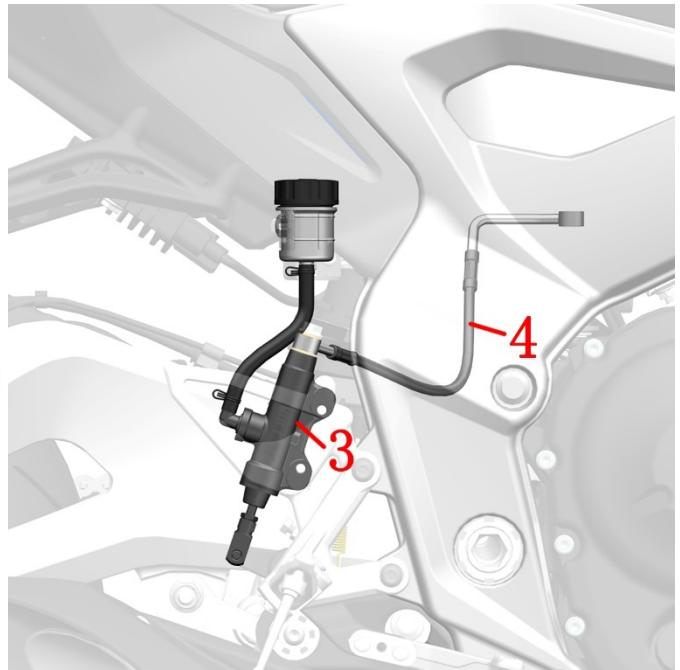
1-Front disc brake main cylinder 2-FMC-HU brake hose 3-RMC-HU brake hose 4-Rear disc brake main cylinder
