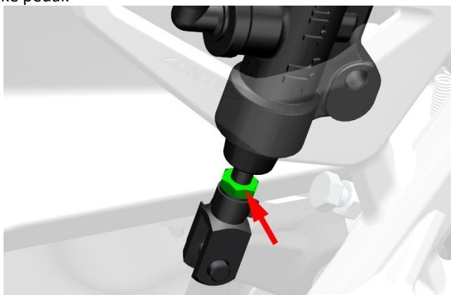
Big adjustment: Loosen the bolt on the brake pedal, adjust the brake pedal to the angle that the driver is comfortable with, and then tighten the bolt.
