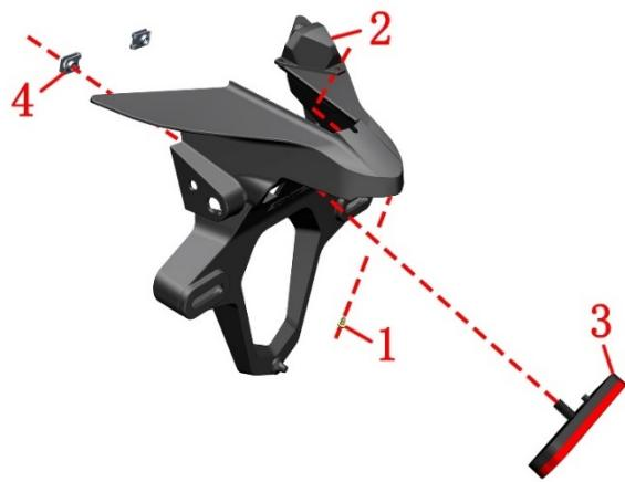
c. Use a T25 Torx wrench to remove 2 M6 bolts (1), then remove 2 M6 nuts (2), and then separate the rear license plate (3) from the rear fender assembly (4).
