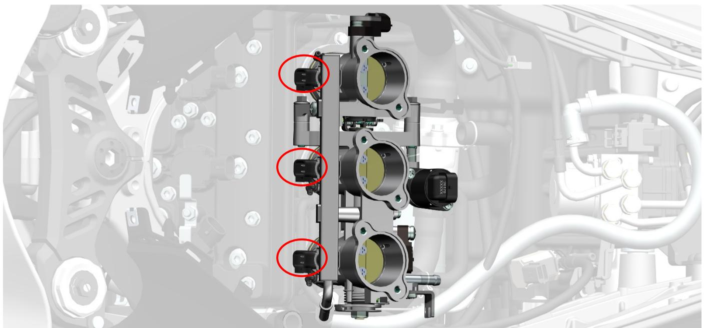
If you need to replace the injectors, wait until the engine and muffler have cooled down. Use a Phillips screwdriver to remove the two screws that hold the slide rail in place and remove the rail and injector together. Use a flathead screwdriver to pry open the clip of the injector to remove the injector.
