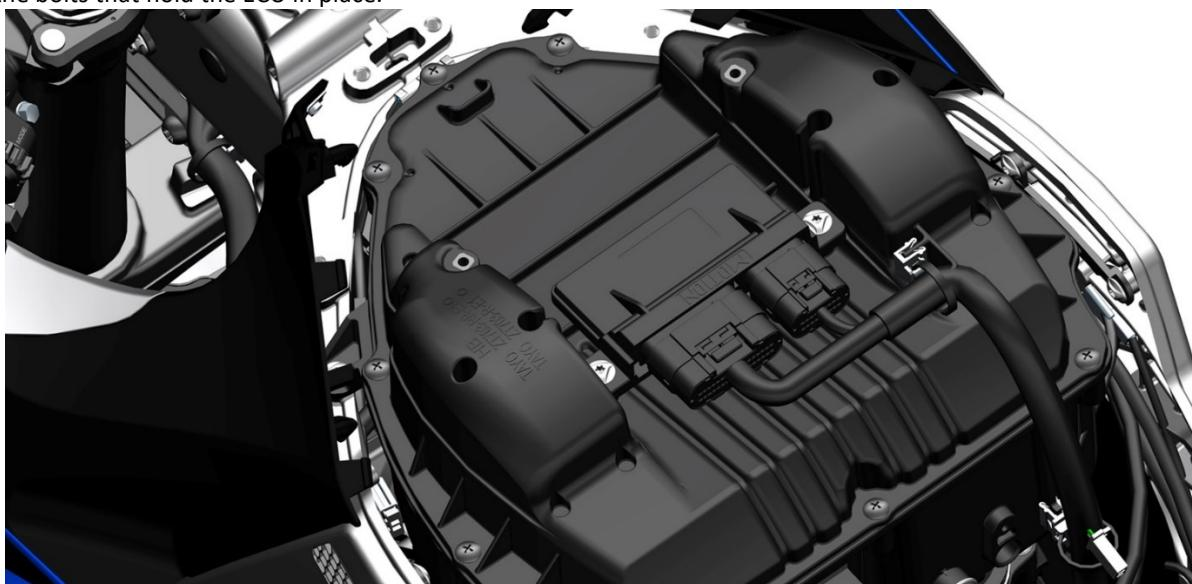
Note: To replace the ECU, you need to shut down the whole motorcycle and wait for 10 seconds before operating to avoid the abnormality of the EFI system.
