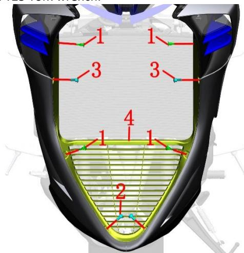
b. Remove the middle of the bracket (4).
