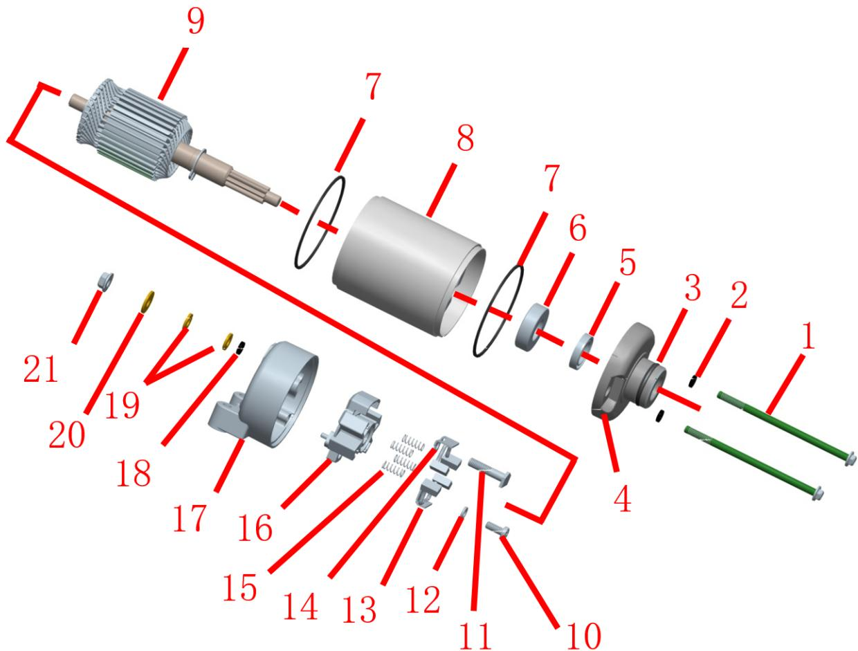
1-M5×98 bolt x 2 2-O ring x 2 3-O ring 4-starter motor front cover 5-oil seal 6-bearing 7-rectangular sealing ring 8-starter motor outer shell 7-rectangular sealing ring 9-electric pestle 10-screw x 2 11-head screw with limit 12-washer 13-negative brush x 2 14-positive brush x 2 15-worm spring x 4 16-insulating brush frame 17-starter motor back cover 18-sealing rubber ring 19-insulating gasket 20 anti-loosening gasket 21 nut
