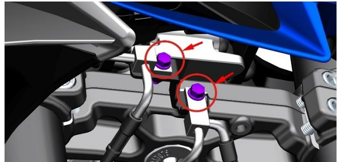
c. Use a T25 torx wrench and an 8# open-end wrench, remove the following two bolts, remove the front brake hose directional upper bracket, and pull out the front wheel speed sensor socket in the frame. For details, please refer to the air filter assembly removal procedure, and the air filter can be removed before finding the socket fixed on the right frame. Press the anti-loosening socket to pull it out.
