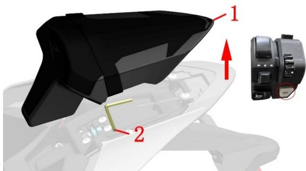
b. and use the 5# hexagon that has just been taken out to remove the 2 fixing screws (1), 2 flanging bushings (2) and 2 flanging bushing buffer glues (3) that fix the main cushion, gently push back the main cushion (4) with your hand, and remove the main cushion (4); For more information, please watch the saddle removal video.
