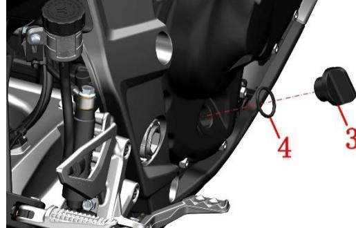
g. After waiting for the oil to flow out completely, wipe the oil drain bolts with a clean non-woven fabric, check whether there are scratches on the joint surface of the oil drain bolts, and replace them. Then use a clean non-woven fabric to wipe the joint surface of the engine and oil drain bolts.
