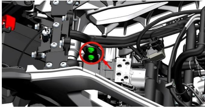
d. After grasping the hydraulic control unit, remove the two M6×16 bolts with a T25 torx wrench, and then remove the hydraulic control unit. If you need to replace the bracket, you will need to remove the flanging bushing and cushioning glue.
