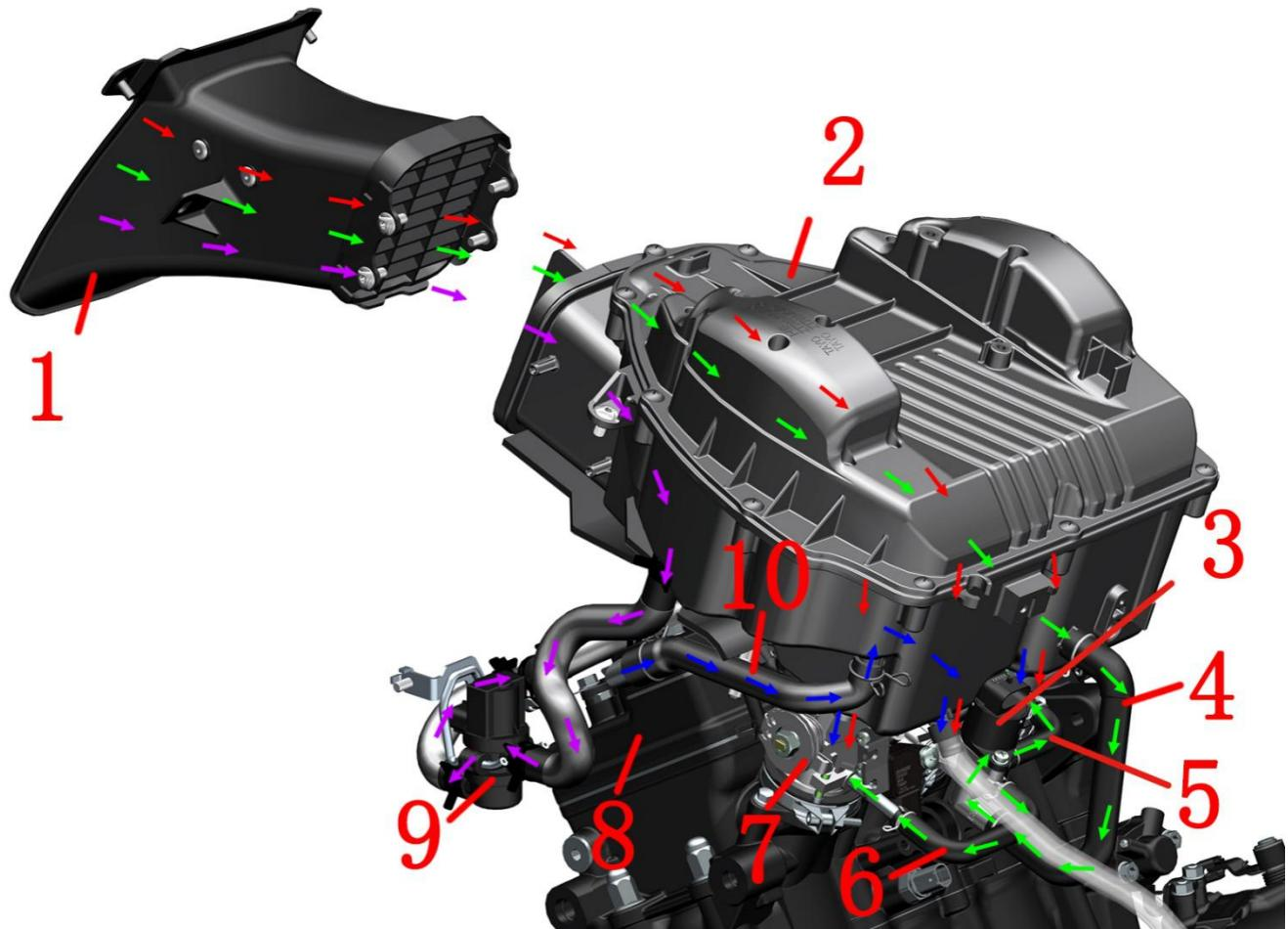
1-Stamping intake pipe assembly 2-Air filter assembly 3-Throttle fill valve 4-Stepper motor rubber hose (2) 5-Stepper motor rubber hose (3) 6-Stepper motor rubber tube (1) 7-Throttle valve body 8-Cylinder head 9-Secondary make-up valve 10-Exhaust gas snorkel
