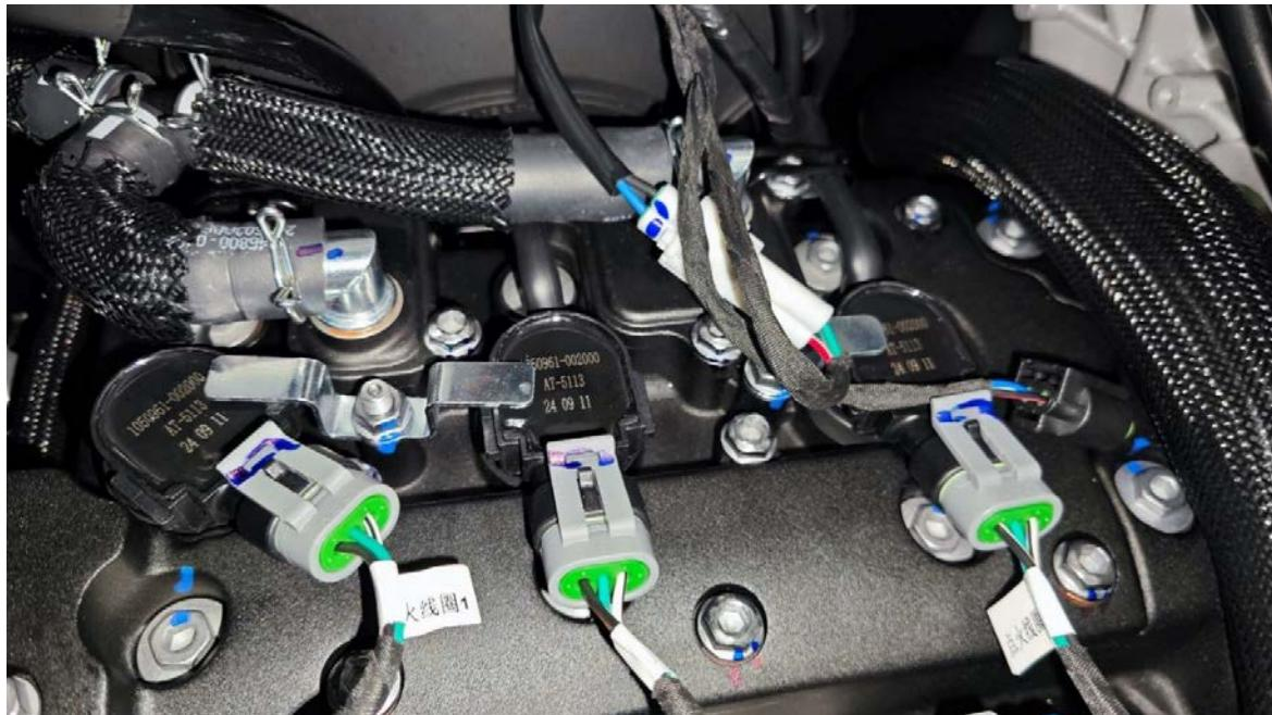
Remove the nut with the 10# sleeve and remove the ignition coil pressure plate. Remove the ignition coil. Use the 14# sleeve to remove the spark plug. If the fit is tight, you can shake it slightly from side to side to take out the ignition coil.
