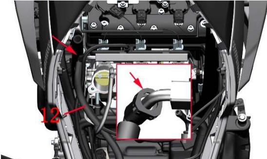
g. Install the high-pressure tubing (12) back according to the above steps.
