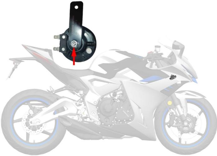
If you need to remove the horn, use the T25 Torx wrench to remove the 2 bolts. Pull the horn out and remove it after pulling the plug.
