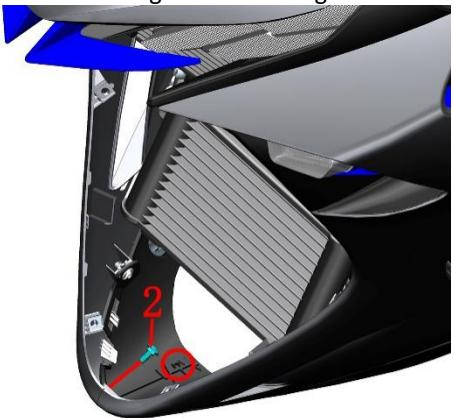
d. Use a T25 Allen Torx wrench to remove 1 M6×12 bolt as shown.
