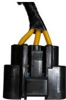
d. Check whether the yellow wire color 3P plug on the stator side of the magneto is not conductive with the ground. If the resistance value or the conduction with the ground, the magneto stator needs to be replaced.
