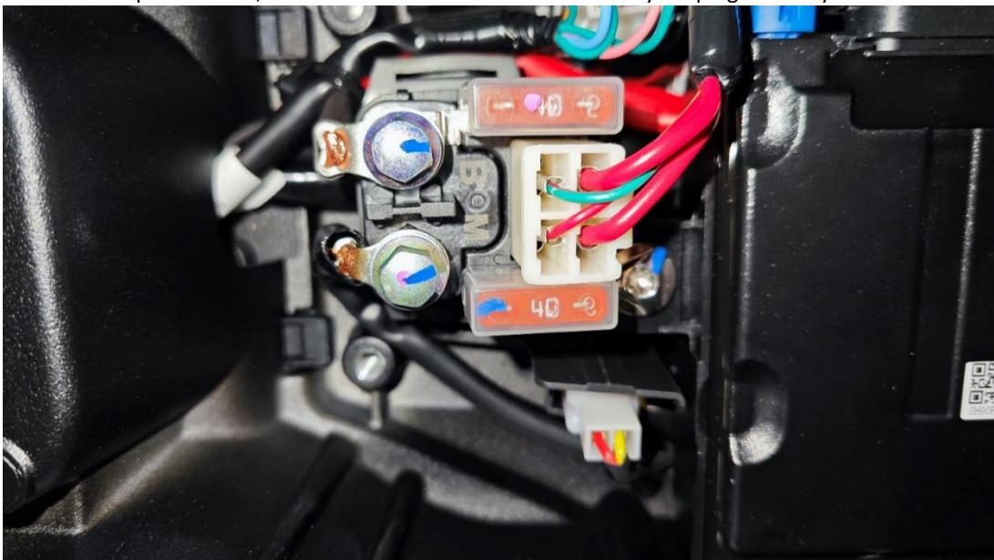
When reinstalling the relay, the red wire is installed on the threaded hole of the relay marked "B", and the black wire is installed on the threaded hole of the relay marked "M". Make sure the protective cap is closed after the screws are tightened, and then plug in the relay connector.
