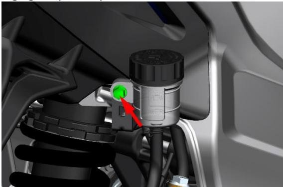
b. Unscrew the upper cover of the main pump counterclockwise and take out the rubber sleeve inside. Add
