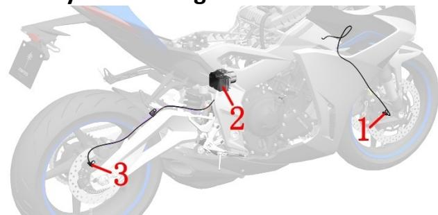
1-Front wheel speed sensor 2-ABS hydraulic control unit 3-Rear wheel speed sensor
