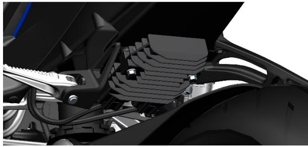
b. Unplug the 3 wires. Check the plug for looseness or corrosion.
