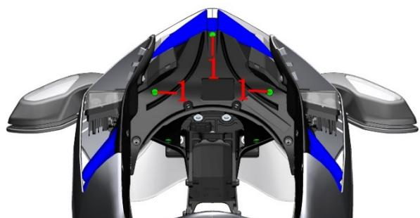
h. After removing the head lower liner, find the wiring harness connector of the left and right position lights and unplug them.
