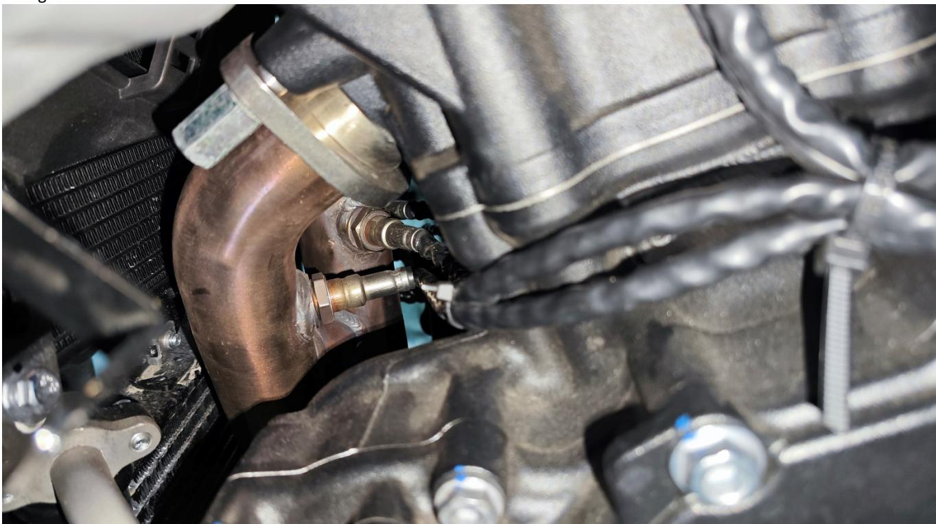
The new sensor threads are coated with a special paste thread anti-sintering agent to prevent air leakage and facilitate subsequent re-disassembly. If the old inspection is fine, it is necessary to apply an appropriate amount of anti-sintering agent to the thread before installation. Torque standard:  $18\pm1.5N.m$ .
