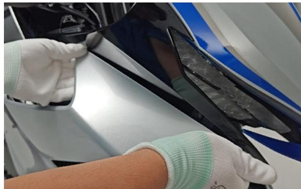
c. Use a crochet hook to remove the 2 expansion pegs on the right side of the front panel.
