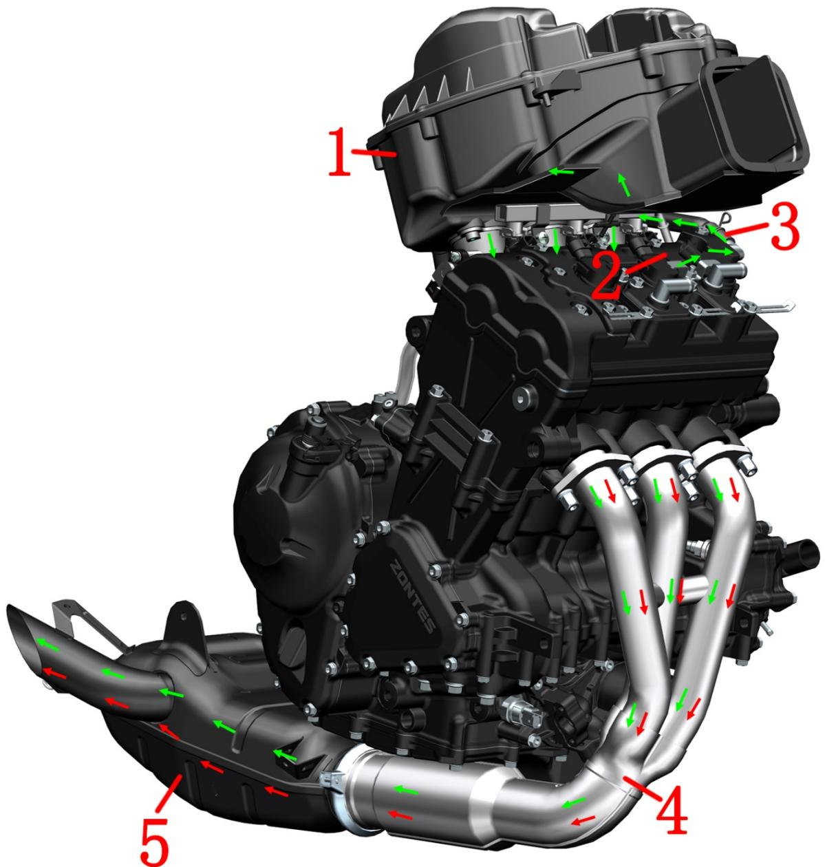
1-Air filter assembly 2-Cylinder head 3-Exhaust gas snorkel 4-Front muffler 5-Rear muffler
