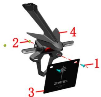
d. Use a T25 torx wrench to remove the two M6×16 inner torx shaft shoulder bolts (1) on the left and right sides, remove the left and right turn signals (2), then remove the two M6 nuts (3), and use the T25 torx wrench to remove one M6 bolt (4) that fixes the rear fender bracket (5), and then take out the rear fender bracket (5).
