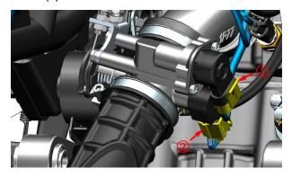
b.Place a small container underneath the high-pressure fuel line. Press down on the latch indicated by (3) and pull out the high-pressure fuel line (1) in the direction of the arrow. A small amount of fuel may leak out during removal, so avoid allowing it to drip onto any part surfaces.
