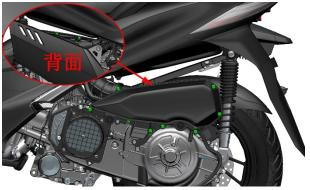
b.Remove the air filter housing.
