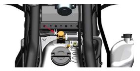
h.Use a ratchet wrench + 10# socket to remove 4 M6×16 bolts (6), and remove the springpad (7) and washer (8).
