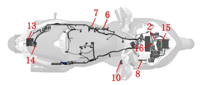
1-TFT meter 2-Flasher 3-Windshield motor controller 4-accumulator 5-horn 6-Side bracket kill switch 7-Canister solenoid valve 8-No electrical inductive antenna 9-Steering lock 10-Electric handbar switch 11-Tire pressure receiver 12-Engine controller (ECU) 13-rectifier 14-Cushion lock 15-PKE 16-Tilt switch
