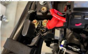
When reinstalling, ensure that the yellow/red and green/red wires of the relay correspond to the main wiring color codes. The nuts do not need to be differentiated. After tightening the nuts, make sure to cover the protective cap securely.
