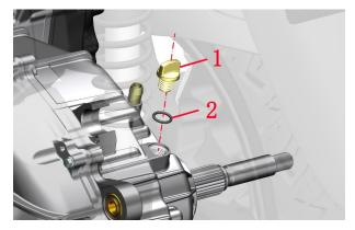
b.Place the oil pan under the rear of the engine on the left side.Use a 14# sleeve to loosen the oil drain bolt (3) counterclockwise.
