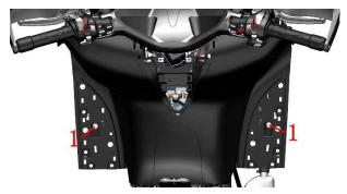
d.Turn on the battery, unlock the fuel tank cover lock and remove the fuel tank cover. Then use a T25 Torx wrench to remove the two M6×14 shoulder bolts (1) and M6×14 shoulder bolts (2) that hold the tank lock. Locate and unplug the tank lock harness connector (4), then remove the tank lock (3).
