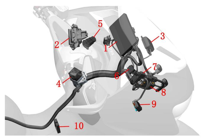
1-TFTappearance 2-Front left storage compartment lock 3-Windshield motor controller 4-Steering lock 5-Dual-port USB charging cable 6-Single-port charging cable 7-EFI relays 8-Start the relay 9-Charging port base 10-Electronic lock of the fuel tank
