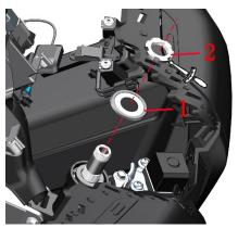
c.Ensure that the lower plate does not rotate and does not jam or loosen, and then put in the adjusting nut washer (3), the direction post adjusting nut (2), and the adjusting nut anti-loose washer (4) in turn. The nut only needs to be tightened and aligned with the first nut.
