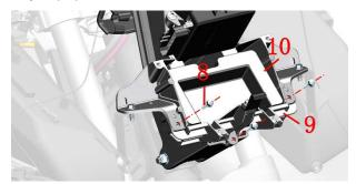
d.Use the 8# sleeve to remove 3 M6×16 bolts (8) and remove the bracket (11).
