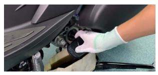
d. Use a clean non-woven fabric to wipe off the remaining oil and impurities on the engine.
