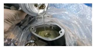
f.Observe whether the liquid level of the main pump is at 3/4 of the transparent inspection place, if not, it needs to be added or pumped out or discharged with a syringe.
