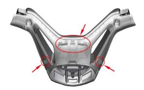
f.Replace the left and right 2 expansion nails. Use a T25 Allen Torx wrench to replace the 2 bolts on the left and right sides. (Check whether the direction handle is pressed or not) g.Replace the upper cover of the direction handle.
