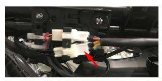
b.Check the connector for looseness or corrosion.
