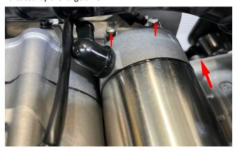
e.When reinstalling, pay attention not to omit the O ring of the starting motor, and align the teeth of the electric starting reduction gear. Note that the O-ring needs to be properly fitted into the box, as cutting edges can cause leakage. The torque of the two bolts that hold the starter motor in place: 12±1.5 N.m (1.2±0.2 kgf.m, 9±1 lbf.ft). and mark with a marker.
