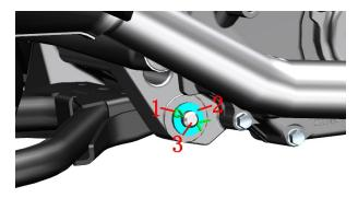
b.Remove the spring from the main bracket.
