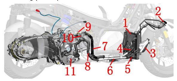
1-Main water tank 2-Water tank filling port 3-Auxiliary tank 4-Main tank inlet pipe 5-Main tank outlet pipe 6-Aluminum water pipes 7-Thermostat outlet pipe 8-Engine water inlet pipe 9-Water and oil share sensors 10-Thermostats
