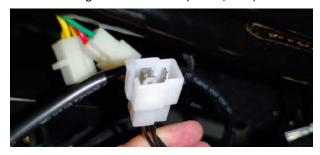
d.After disconnecting the yellow 3P connector, use the multimeter to measure the voltage between the red positive wire and the green negative wire. It should match the battery voltage. Use the multimeter's buzzer mode to check if the green negative wire is continuously connected to the ground (the ground wire can be any stud directly connected to the frame).
