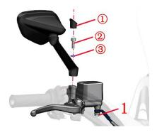
c.After grasping the front brake main pump, remove the 2 bolts (2) with 5# hexagon and remove the right switch.
