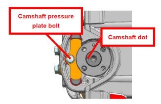
The bolt center is aligned with the dot center
