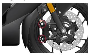
b.Place the oil pan under the front disc brake caliper. First uncover the rubber cap of the screw (1), put on waterproof gloves and remove the bolt (2) with an 8# torx wrench, remove the bolt (3) with a 14# torx wrench, and remove the two copper washers (4).
