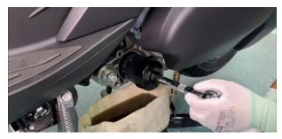
c.Drain the oil inside the fine filter.
