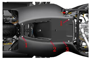
c.Unplug the fuel pump and start the engine to idle until the engine stalls. Turn the engine off switch to "\(\overline{\mathcal{A}}\)", and lock the motorcycle after powering off.
