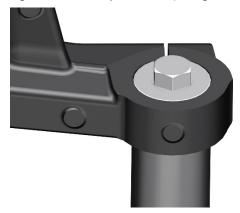
c.Install the two M8×30 bolts on the lower link plate, and use the same method to install the other shock absorber.
