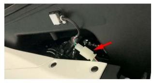
d.Unplug the stepper motor (1) and sensor (2).
