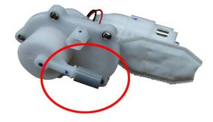
When reassembling, it is necessary to pre-tighten diagonally and then tighten 5 bolts, otherwise the uneven compression of the sealing rubber ring of the fuel pump will easily lead to leakage and cause potential safety hazards.
