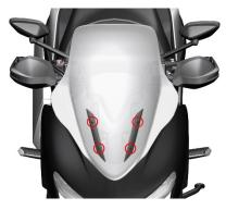
b.Use a T25 Allen Torx wrench to loosen the 4 M6×16 bolts on the left and right decorative covers of the windshield. Take out the left and right trim covers, windshields, and windshield bracket rubber pads from the windshield in turn.
