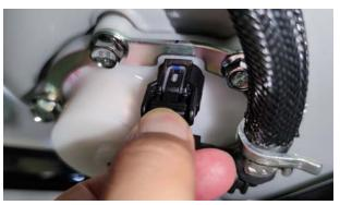
Note that you should not press the outlet pipe shown in red, and once damaged, you can only replace the entire fuel pump assembly.
