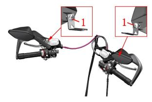
b.Use the 5# hexagon socket to loosen the balance weight bolt A for 5-8 turns, and remove the left and right hand guards and the balance weight assembly.
