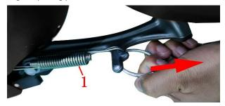
c.First, remove the side bracket spring with a hook or rope, remove the bolt (2) on the inside of the side bracket counterclockwise with an 8# sleeve, and remove the copper gasket (3) and the side bracket flame-out switch. Remove the nut (8) with a 14# socket or torx wrench, then remove the bolt (5) with a 14# socket or torx wrench, take out the bushing (6), and finally remove the side bracket (7).
