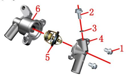
1-M6×10bolt\*2 2-M6×12bolt 3-φ5.6×φ1 O-ring 4-upper housing of thermostat 5-thermostat core 6-thermostat lower housing
