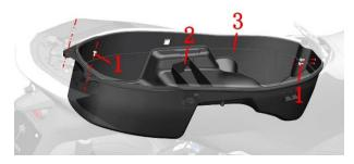
b.Use a T25 Torx wrench to remove the shoulder bolts (1) of the 2 M6×14 fixed in the rear storage compartment. After lifting the storage box slightly, pull out the storage box atmosphere light connector on the left side of the storage box, and then take out the storage box assembly.
