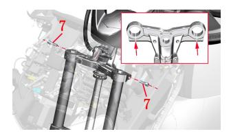
c.Use the 6# hexagon to remove 4 M8×30 bolts (7), pry open the gap on the lower plate with a lot, and remove the left front shock absorber and right front shock absorber.
