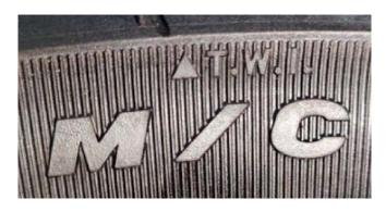
The tread bulge has a wear mark height of 1.6 mm (0.06 in). The sidewall triangle (PT.W.I.) markings indicate the position of the wear strips. If it is worn to the marked point, it means that it has been worn to the limit, and it will be a safety hazard to continue driving, and it must be replaced with new tires of the same specification.
