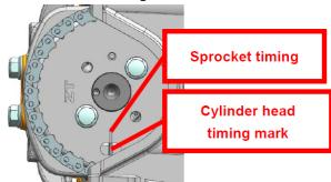
The timing of the sprocket is aligned with the timing of the cylinder head
