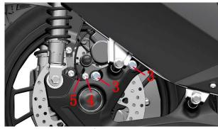
c.Remove the brake pads first.
