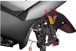
c.Use the 5# hexagon socket to remove 1 M6×30 bolt (1) and remove the spacer (2). Use a T45 Torx Allen wrench to remove the shoulder bolt (4) of one M6×14.
