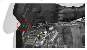
b.Use a T30 torx wrench to remove the torx bolt in the M6×16 hexagonal small flange shown in the figure or remove the M6×14 shaft shoulder bolt with a 4# hexagon socket, the bolt here cannot be removed temporarily, and it can be completely loosened.
