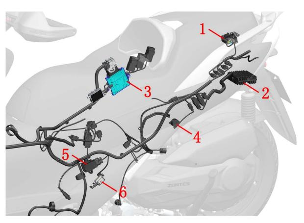
1-Cushion lock 2-rectifier 3-Engine controller (ECU) 4-buzzer 5-Ignition coil body 6-Canister solenoid valve
