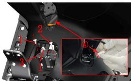
e.Use a T25 torx wrench to remove the 4 M6 $\times$ 14 shoulder bolts (1) of the box panel assembly, and then take out the box panel assembly.
