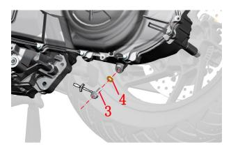
c.Remove the M8×25 oil drain bolt (3) and the  $8.3\times16\times1.5$  copper pad (4).
