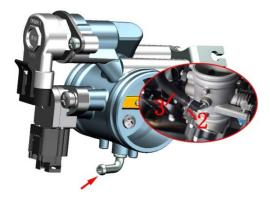
d.Loosen the bolt of the clamp (4) with a 4# hexagon socket and pull out the throttle valve body according to the direction of the arrow after the air filter outlet pipe (5) and clamp (4).
