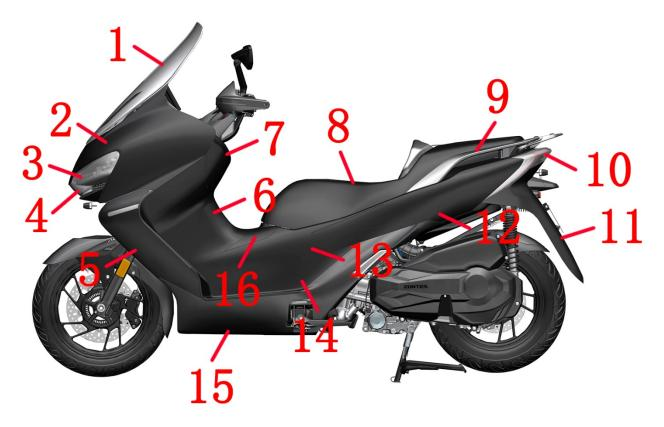
1.Windshield 2.Front panel 3.Headlight 4.Headlight cover 5.Left pedal decorative cover 6.Front compartment panel rear 7.Left front compartment lid 8.Cushion assembly 9.Left rear armrest 10.Left tail light 11.Rear fender 12.Left tail skirt 13.Left cover 14.Left pedal upper 15.Left pedal lower 16.Fuel tank cover rear decorative cover
