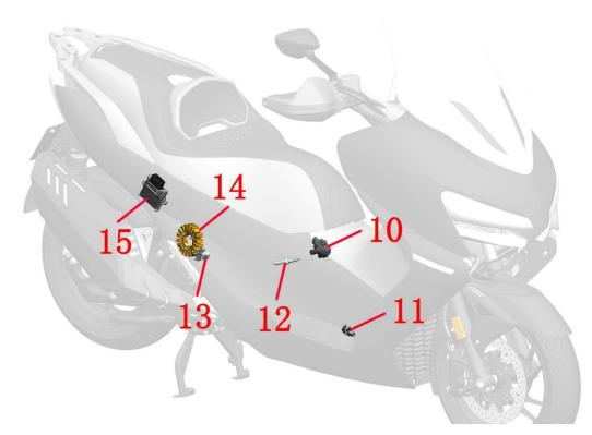
1-Tilt switch 2-PKE 3-Relays 4-Steering lock 5-The right hand handles the secondary switch 6-Right-hand handle switch 7-accumulator 8-Fuse box 9-Start the relay 10-Ignition coil 11-Side bracket kill switch 12-spark plug 13-Crankshaft position sensor 14-Magneto stator 15-ECU Note:
