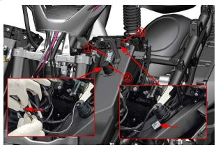
b.Remove the harness connector next to the relay that connects to the storage box panel.
