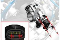
Simple test method: take out the stepper motor after turning off the power, do not loosen the cable plug, press the power-out switch at start-up, do not ignit, check whether the motor plug can shrink back and forth, and finally turn off the power-out switch to see if the plug returns to its original position. To check whether the stepper motor is abnormal, measure whether the resistance at both ends A and B is  $53\pm5.3\Omega$ .
