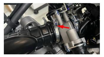
D.Pull the outlet pipe to the right side of the motorcycle to expose the two M6×30 bolts that fix the starting motor, and remove them with an 8# sleeve. After removing the bolts, remove the starter motor from the engine in the direction indicated by the large arrow.
