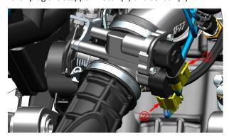
e.Use a short Phillips screwdriver to remove the 2 bolts (3) and the anti-release card (4) that come with the throttle body assembly, and then remove the stepper motor (4).
