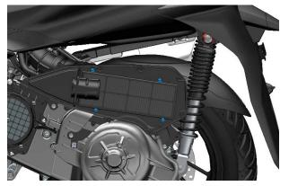
b.Remove the old air filter cartridge. Use a dust gun to blow
