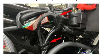
c.Loosen the clamp bolt shown in the figure countercl ockwise with 4# hexagon socket, and pull the air filter outlet pipe out of the throttle valve body in the directi on of the rear wheel.
