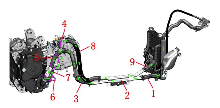
1-Main tank outlet pipe 2-Aluminum water pipes 3-Engine water pipes 4-Thermostats 5-The water pump covers the inlet pipe 6-Water pump cover outlet pipe joint 7-The water pump covers the outlet pipe 8-Thermostat outlet pipe 9-Main tank inlet pipe 48 / 137
