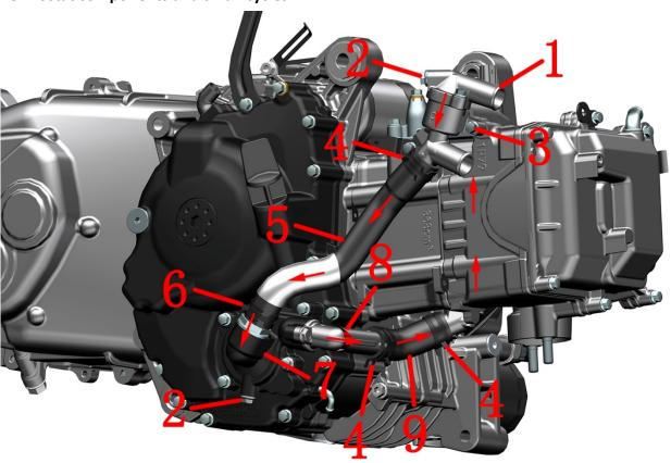
1-Thermostat assembly-M6×12 bolt\*2 3- M6×22bolt\*2 4-Water pipe hoop(φ26)\*3 5-Water pump cover inlet pipe 6-Water pipe clamp(φ24) 7-Water pump cover assembly 8-Water pump cover outlet pipe joint 9-Water pump cover outlet pipe
