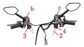
d.Refer to the "Throttle Clue" step and loosen the throttle
