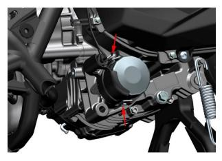
b. Place an oil pan underneath the fine filter cover. Use a 14-sided 65mm cap-style filter wrench (with a Shida model number of 97401) combined with a 1/2" (12.5mm) ratchet wrench to rotate counterclockwise and remove the fine filter.
