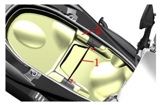
b.Refer to the steps of "Removal of the Rear Handrail" to remove the rear handrail assembly. Remove 6
