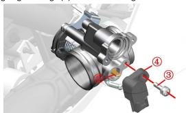
Simple test method: connect the whole motorcycle to the diagnostic instrument, press the ignition switch (no need to ignite), turn the throttle handle from the initial position to full open, this process to see if the throttle position signal follows the change from 0 to 100.
