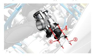
f.Use a throttle cleaner to clean up carbon deposits from the stepper motor head. Spray a small amount of cleaning agent into the valve body bore. It is forbidden to soak the stepper motor with any liquid.
