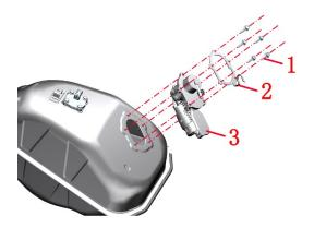
When reassembling, it is necessary to pre-tighten diagonally and then tighten 5 bolts (1), otherwise the sealing ring of the fuel pump (3) is compressed unevenly, which is easy to lead to leakage and cause potential safety hazards. Remark:
