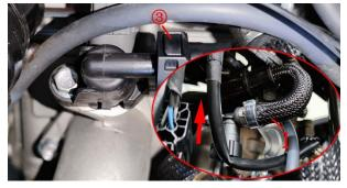
c.Find the circlip (2) at the bottom of the valve body, pinch both ends of the circlip with your hand and move it outward, and then pull out the desorption tube (3).
