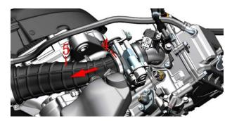
e.Remove the valve body assembly from the engine after removing the 2 bolts (6) with 5# hexagon sockets.
