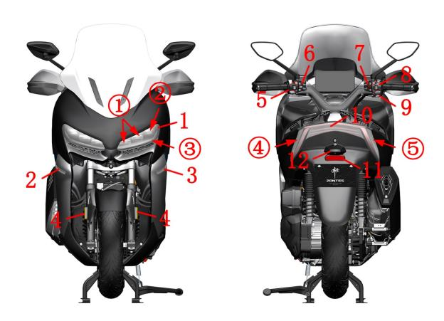
1-headlight (1)-low beam position 2-High beam position 3)-Position light/daytime running light position) 2-Right turn signal 3-Left turn signal 4-side reflector 5-Left hand handle switch 6-Left hand handle sub switch 7-Right hand handle sub switch 8-Right hand handle switch 9-Handle the heating switch 10-Rear tail light (4)-Rear left turn signal 5)-Rear right turn signal) 11-rear reflector 12-rear license plate lamp
