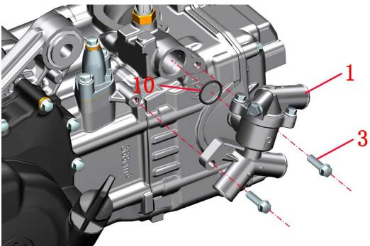
The joint surface should be cleaned before reassembly, and it should be noted that the O-ring should not be missed and 96 / 137
