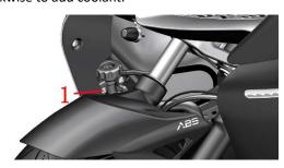
b.Remove the storage box according to the steps for removing the throttle body. Use a 10# sleeve to loosen the M6×12 deflation bolt (2) of the thermostat counterclockwise for 4 $^{\sim}5$  turns, and do not remove it completely. Note that a small container is used to absorb the coolant that has spilled from the exhaust bolts. Do not allow coolant to drip directly onto the surface of the part. The O-ring at the vent bolt is  $\phi5.6\times\phi1$ .
