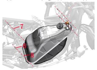
i.Lift the tank assembly slightly from the tail end, move it back until the tank filler passes safely under the frame, and remove the tank assembly upwards.
