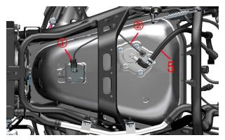
g.Use pliers to remove the clamp on the canister that connects to the oil and gas sensor and remove the hose.
