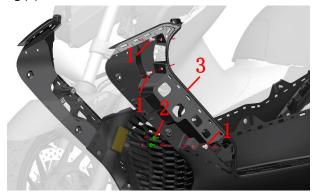
b.Use a T25 Torx wrench to remove the shoulder bolts (1) of the two M6×14 fixed to the lining (3) of the left decorative cover, and remove the inner lining (3) of the left decorative cover.
