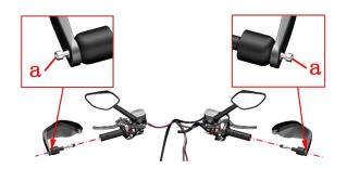
c.Remove 4 M6×30 bolts (2) with 5# hexagon socket, remove the left deputy handle switch (3), rear disc brake main pump assembly b, right deputy handle switch (4), front disc brake main pump assembly c.
