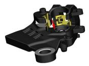
c. Grasp the outer brake pad with the left hand, insert the pin ② with the right hand, and be careful not to insert it to the end. After the inner brake pad is put in place, insert the pin shaft to the end and lock the pin ② with a T25 torx wrench, and replace the circlip ① with needle-nose pliers. Note that the side with grooves is facing the brake disc; The black metal back panel faces the calipers.
