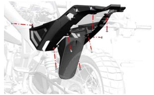
b. Use the 4# hexagon to remove the 3 M6×14 inner torx shaft shoulder screws fixed on the inner mud board, and then remove the inner mud board.
