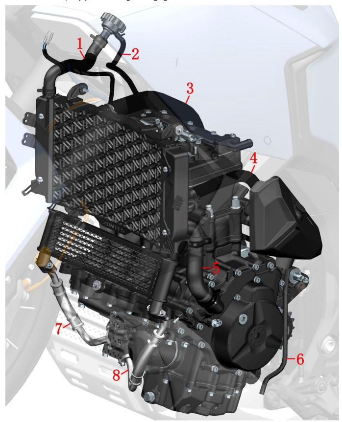
1-ZT703—F The connecting water pipe of the water tank filling port2-ZT703—F Connecting water pipe for the auxiliary tank3-ZT703—F Main tank inlet pipe4-ZT703—F Small circulating water pipes5-ZT703—F Engine water inlet pipe6-ZT310—R Leaky pipe in the auxiliary tank7-ZT703—F Engine inlet pipe8-ZT703—F Engine outlet pipes
