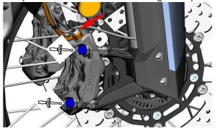
Front disc brake calipers disassembled
