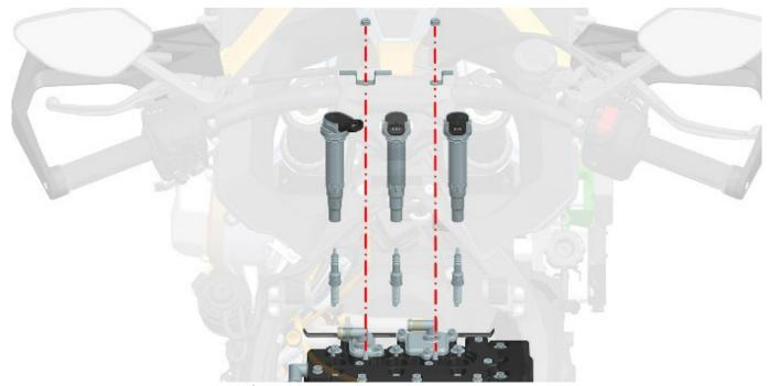
When installing the ignition coil back, first insert the ignition coil back into the bottom, and turn the ignition coil plug towards the position shown in the figure above, then put it back into the pressure plate, and put the nut back tight, and the torque standard is 11.5±1N.m.
