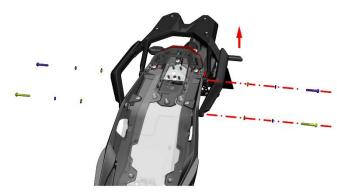
b. Flip the rear armrest to the back, use the 4# hexagon to remove the bolts of the left 4 non-standard inner plum blossoms M6×12, remove the left buffer glue of the rear armrest (shown L), and remove the right buffer glue (shown R) in the same way.
