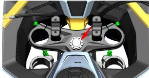
b. Remove the two bolts (1) of the upper plate with 6#
