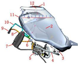
1-Fuel Tank Lock 2-Oil Level Sensor 3-Fuel Pump 4-High Pressure Oil Hose 5-Throttle Valve Body Assembly 6-Adsorption/Snorkel 7-Carbon Canister 8-Solenoid Valve Outlet Pipe 9-Carbon Canister Solenoid Valve 10-Solenoid Valve Intake Pipe 11-Fuel Tank 12-Air-Oil Separator (Inside Tank Lock)
