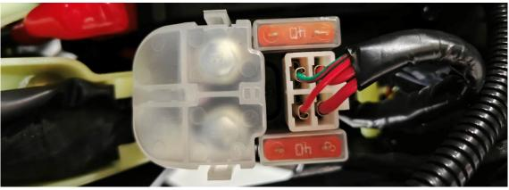
b. Unlock the vehicle, hit the engine shutdown switch to " , put away the side bracket, pinch the brake handle and press the start button, then you should be able to hear the sound of the starter relay sucking, otherwise the starting line should be checked.
