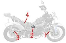
1-Front wheel speed sensor 2-ABS Hydraulic control unit 3-Rear wheel speed sensor 4-OBD Diagnostic interface
