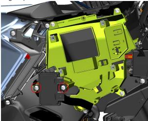
d. Remove the tank refill from the wiring board and pull open the tank refill
