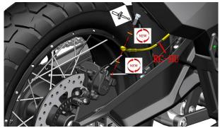
b. Remove the rear caliper and brake pads first by following the steps for removing the rear wheel and replacing the brake plate.
