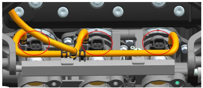
If you need to replace the injectors, wait until the engine and muffler have cooled down. Use a Phillips screwdriver to remove the two screws that hold the slide rails in place, and remove the rails and injectors together. Use a flathead screwdriver to pry open the clip of the injector to remove the injector.
