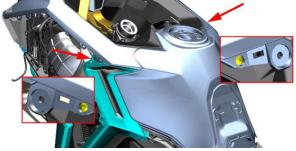
h. Gently support the tail of the fuel tank with your hand, pull out the fuel pump plug (3), start the engine and idle until the engine turns off. Turn the engine off switch to " , and lock the car after powering off. Press the anti-disengagement latch in the direction of the arrow and pull out the high-pressure oil pipe (2). Press the anti-disengagement latch in the direction of the arrow, pull out the plug of the oil level
