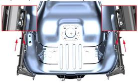
e. Remove the 2 bolts with a cross batch and remove the spacer.
