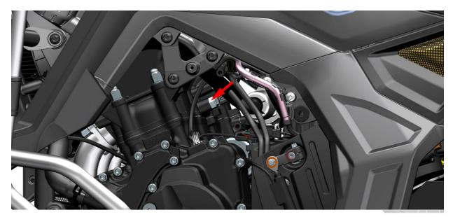
Use a multimeter with two pins of room temperature resistance values:  $3.74 \sim 1.22 k\Omega$  ( $10 \sim 40^{\circ}$ C);  $1.22 \sim 0.27 k\Omega$  ( $40 \sim 90^{\circ}$ C).
