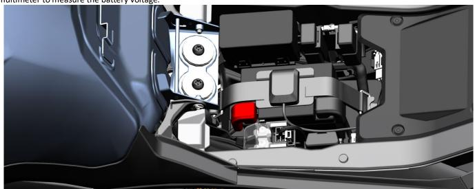
The charging voltage of the charger shall not be higher than 15V. When you do not use the motocycle for a long time, you should charge it regularly according to the requirements of the driving manual. If the battery loss effect is properly handled by a professional recycling agency, do not discard it at will to avoid pollution to the environment.
