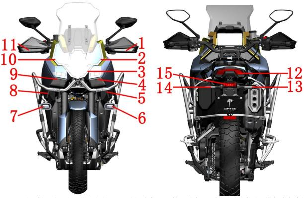
1-Left front turn signal 2-Left position light 3- Center position light 4-Left headlight 5- Left corner light 6- Left fog light (high-end version) 7- Right fog light (high-end version) 8- Right corner light 9-Right headlight 10- Right position light 11-Right rear turn signal 12- Rear position light 13- Right rear turn signal 14- Left rear turn signal 15- Rear taillight/license plate light
