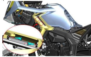
g. Gently pull the lower part of the left envelope in the direction pointed by the arrow with your hand, and remove the self-tapping screws behind the envelope with a cross batch. Lift it up slightly and remove the lower part of the envelope. The right side is removed in the same way.
