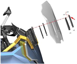
b. Remove the left and right trim covers, windshields, and windshield bracket pads from the windshield in turn.
