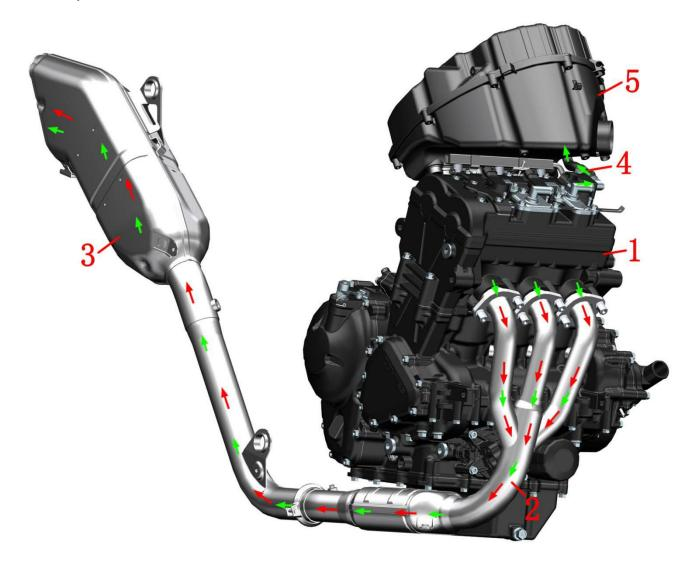
1-cylinder head 2-front muffler 3-rear muffler 4-exhaust gas snorkel 5-air filter assembly Exhaust system:
