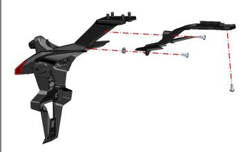
f. First, use the 4# hexagon to loosen the 2 M6×14 inner torx shaft shoulder screws, then slowly pull out the tail lamp and remove it, then pull out the rear fender bracket, and remove the 4 M8×18 non-standard torx groove bolts.
