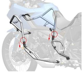
e. Use a T50 Allen socket with a mid-hole to remove one M10×20 bolt and remove the left guard.
