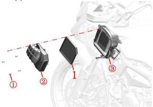
b. Replace the new air filter element (1) with the left air intake chamber (3), and then replace the left air intake chamber cover (2) and fix it with 5 self-tapping nails (1).
