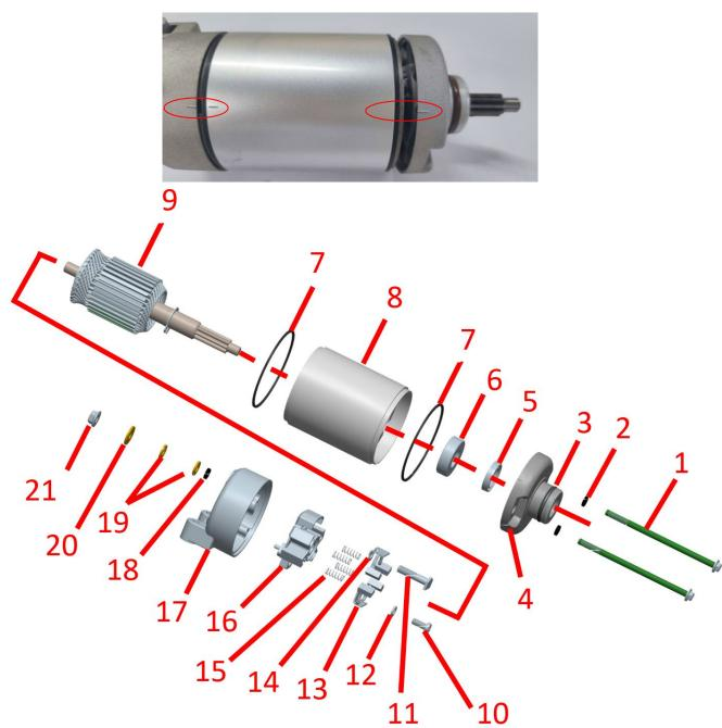
1-M5×98 bolt× 2 2-O ring×2 3-O ring 4-starter motor front cover 5-oil seal 6-bearing 7-rectangular sealing ring 8-starter motor outer shell 7-rectangular sealing ring 9-electric pestle 10-screw ×2 11-head screw with limit 12-washer 13-negative brush×2 14-positive brush×2 15-worm spring ×4 16-insulating brush frame 17-starter motor back cover 18-sealing rubber ring 19-insulating gasket 20 anti-loosening gasket 21 nut
