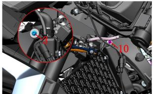
b. Untile the 2 wire clamps (5) on the main water tank, and remove the wire harness fixed on the water tank after arranging.
