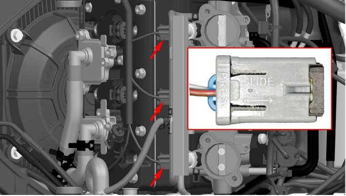
The static coil resistance measured with a multimeter should be  $12\pm0.6\Omega$ , otherwise the injector will fail and need to be replaced.
