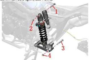
b. One person fixes the head of the bolt with a 14# sleeve, and one person uses a 14# sleeve to remove the nut, remove the bolt, and remove the rear shock absorber and triangle bar assembly. Nut torque: 65±5N.m (6.6±0.5 kgf.m, 48±4 lbf.ft).
