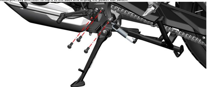
b.Remove the bolt with the 8# sleeve and remove the spring pad and flat pad.
