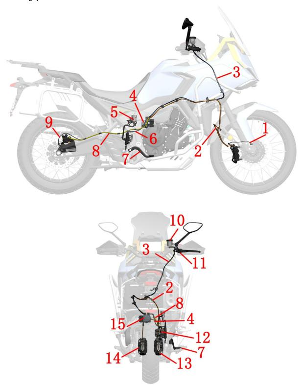
1- Wheel speed sensor (front wheel) 2- FC-HU brake hose 3- FMC-HU brake hose 4- RMC-HU brake hose 5- Rear disc brake master cylinder 6- Rear brake switch 7- Brake pedal 8- RC -HU brake hose 9- Wheel speed sensor (rear wheel) 10- Front disc brake master cylinder 11- Front brake switch 12- Rear disc brake assembly 13- Front disc brake assembly (right) 14- Front disc brake assembly (left) 15- Hydraulic control unit
