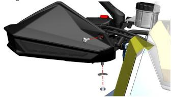
b. After grasping the front brake main cylinder, remove the 2 bolts with the 8# sleeve to remove the front disc brake half cover and the rearview mirror assembly.
