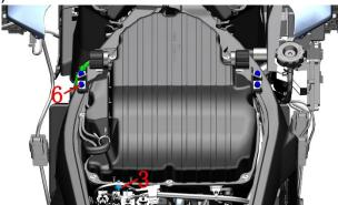
b. Use hoop forceps to remove the hoop (2) on the air filter housing and pull out the rubber tube (3); Use hoop forceps to remove the clamp (4) on the rubber tube of the stepper motor (7), and pull out the rubber tube (7) of the stepper motor;
