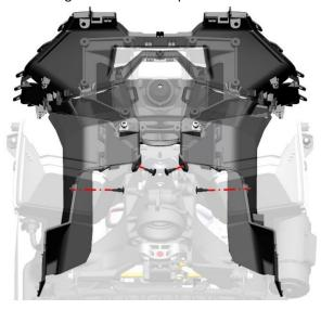
b. Use the T25 plum blossom hexagon to remove an M6×14 axle shoulder bolt bolt on the left side of the vehicle, note: the right M6×14 bolt has been removed when disassembling the wiring version.
