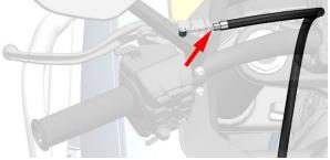
c.If lubrication does not solve the problem of high resistance, the throttle cable needs to be replaced.
