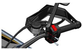
c. Tilt the front brake main cylinder so that the bolts are facing up, wear waterproof gloves, remove the bolts with a 12# sleeve, remove the copper pad and remove the FMC-HU oil pipe, and pour out the brake fluid in the main cylinder. Bolt standard torque: 32N.m (3.3 kgf.m, 24 lbf.ft).
