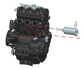
b.When re-installing, pay attention not to omit the O ring of the starter motor, and align the teeth of the electric starting reduction gear. Note that the O-ring should be properly fitted into the box and properly lubricated, as cutting edges may cause leakage. Torque of the two bolts that fix the starter motor: 12±1.5 N.m. and mark with a marker.
