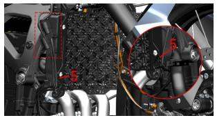
c. use hoop pliers to remove the hoop (12) of  $\varphi$ 22 and the hoop (13) of  $\varphi$ 32 on the small circulating water pipe (12) and the engine water inlet pipe (14); Then use hoop pliers to remove the hoop (12) of  $\varphi$ 22 and the hoop (13) of  $\varphi$ 32 on the water inlet pipe (16) of the water inlet pipe (15) of the main water tank; Once the hoop is removed, the entire main tank can be removed.
