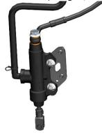
c. Use a Phillips screwdriver to remove the expansion pegs that hold the rear brake oil cup in place.
