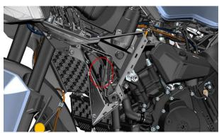
d. Use the 8# sleeve to remove the 4 bolts (9) on the inlet and outlet pipes of the engine; Then use the 8# sleeve to remove the 1 bolt (10) that holds the oil cooler in place. Then rotate the oil cooler to the appropriate position in the direction of the front of the motocycle. Note: Inlet and outlet tubing
