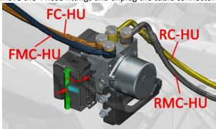
c. Use the 8# sleeve to remove the 2 bolts on the left side of the main frame, and remove the hydraulic control unit and bracket assembly from the motocycle.
