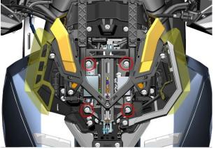
b. Use 4# hexagon socket to remove the two expansion nails on the left and right sides, and use T25 socket torx wrench to loosen two M6×14 shaft shoulder bolts and two M6×16 shaft shoulder bolts. Loosen the left and right trims of the hood and pull them apart slightly to remove the windshield lifter.
