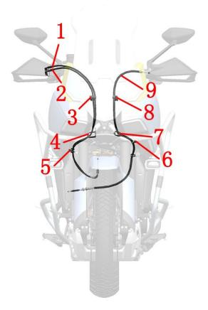
1- Refueling line 2- Oil return line 3-Right handlebar wiring bracket 4- Throttle cable limit bracket 5 - Throttle cable clamp 6 - Clutch cable clamp 7-Clutch cable limit bracket 8-Left handlebar wiring bracket 9-Clutch cable
