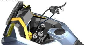
b. Other parts are hidden here for ease of explanation. Move the washer (1) up first, and then loosen the adjusting nut (2a).
