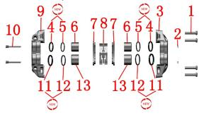
1-bolt 2-Circlip 3-Caliper inner housing 4-φ30 Oil seals 5-φ30 Dust-sealed 6-φ30 piston 7-Brake pads 8-Brake pad spring pads 9-Caliper outer housing 10-Pin shaft 11-φ34 Oil seals 12-φ34Dust-sealed 13-φ34 piston
