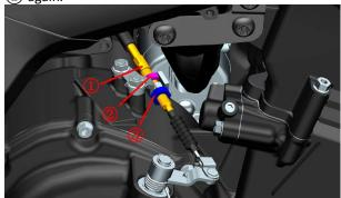
c.If neither of these adjustments is effective, a new clutch cable will need to be replaced.
