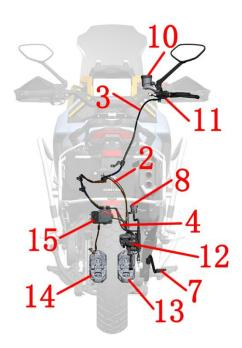
1- Wheel speed sensor ( front wheel ) 2- FC-HU brake hose 3- FMC-HU brake hose 4- RMC-HU brake hose 5- Rear disc brake master cylinder 6- Rear brake switch 7- Brake pedal 8- RC -HU brake hose 9- Wheel speed sensor ( rear wheel ) 10- Front disc brake master cylinder 11- Front brake switch 12- Rear disc brake assembly 13- Front disc brake assembly (right) 14- Front disc brake assembly (left) 15- Hydraulic control unit
