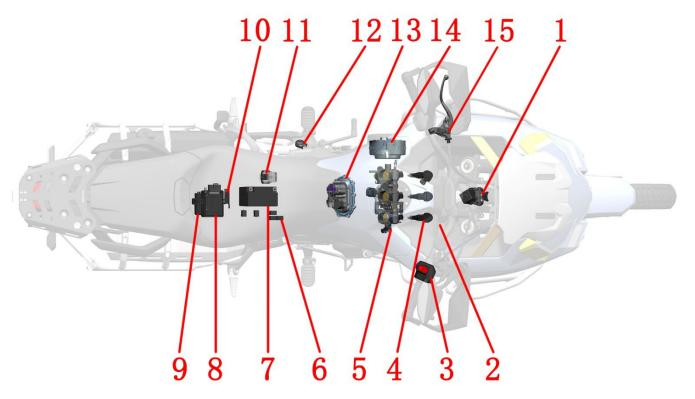
1-Faucet locks 2-Oxygen sensor 3-Right-hand handle switch 4-Ignition coil 5-Throttle assembly 6-Relays 7-accumulator8-PKE host 9-ECU 10-Tilt switch 11-Starting relay 12-Side bracket flameout switch 13-oil pump 14-Magneto 15-Clutch rocker
