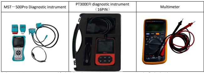
•Both diagnostic instruments can read fault codes; the PT300 diagnostic instrument can be flashed with programs.
