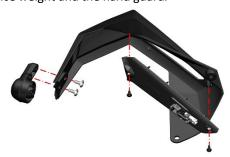
c. If necessary, use a 10# socket to remove the upper nut and remove the left hand guard bracket. Use a 12# open-end wrench to remove the bottom adapter stud. The standard torque of the nut and adapter stud is 8~10N.m.
