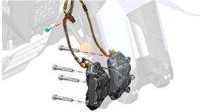
c. Use a T25 torx wrench to remove the 4 bolts on the left and right sides of the front fender (1); Then use the 5# hexagon to remove the 2 bolts (2) on both sides. Detach the tubing from the retaining clip in the rear left side of the fender.
