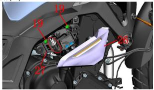
e. After tidying up the wiring harness, use the hoop pliers to remove the  $\varphi$ 36 hoop (28) connecting the thermostat (25) from the gap removed from the charging port base, and then grab one end of the main water tank water inlet pipe (15) to pull out the main water tank water inlet pipe (15).
