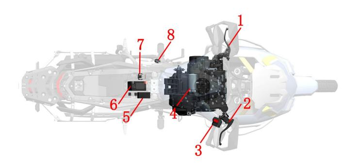
1-Clutch rocker arm (clutch switch) 2-Front disc brake main cylinder (front brake switch) 3-Right handle switch 4-Starter motor 5-Fuse box 6-Battery 7-Starter relay 8-Side bracket power out switch
