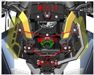
b. After removing the enclosing panel, use a Phillips screwdriver to remove the self-tapping screws as shown. Remove the left and right sides in the same way.
