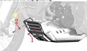
c. Use the plum T25 hexagon inside hex to remove the 3 bolts (1) and flanging bushing (2) of the engine guard, and remove the engine guard.
