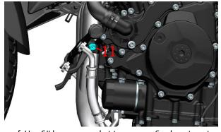
f. Use 6# hexagon socket to remove 6 exhaust port nuts (3).
