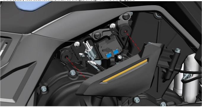
Remove the rubber plug and insert the DC plug of the charger that comes standard with the original factory. Then plug the AC socket into a 110-220V power supply. If the battery is damaged by using an inferior charger, it is not within the scope of the three guarantees.
