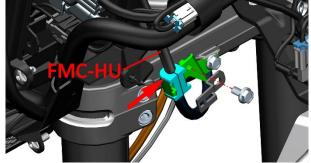
c. Remove the bolts that fix the tubing with a 10# sleeve, and remove the FMC-HU tubing and FC-HU tubing.
