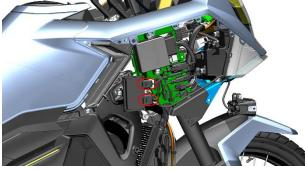
c. Arrange the wiring harness next to it, use the plum T25 hexagon to remove the 2 shoulder bolts (1) that fix the fog lamp drive box and remove the fog lamp drive box (2).
