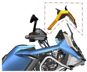
d. The entire decorative cover assembly can be disassembled by using the cross batch, and the installation position relationship is shown in the figure below.
