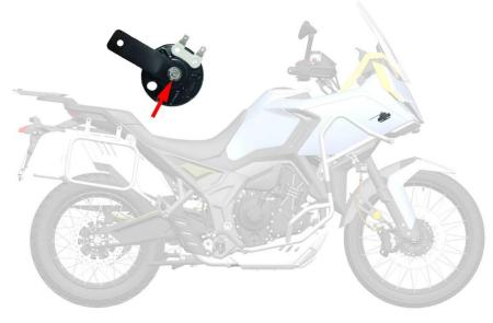
If you need to remove the horn, if the bumper has been installed, insert a T25 wrench into the front mounting bracket of the bumper above the front fender to remove the bolts. Pull out the horn and unplug it to remove. it.
