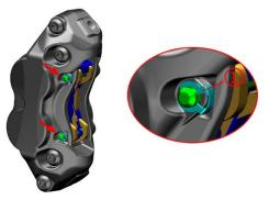
b. Use a T25 hexagon torx wrench to remove the upper pin (2) and then remove the lower pin in turn.
