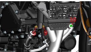
e. Use a T50 pattern wrench with a middle hole to remove the 2 bolts (11) on the lower guard bar mounting bracket and remove the lower guard bar mounting bracket.
