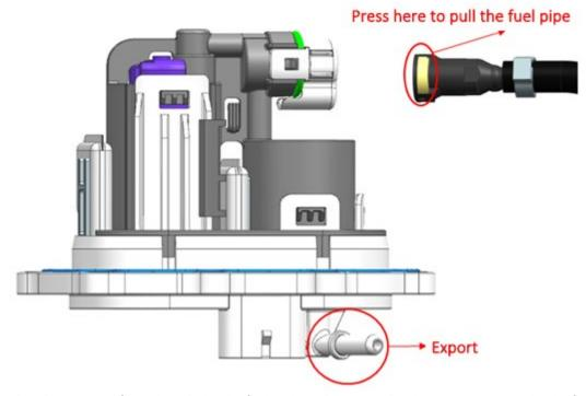
If the fuel pump needs to be removed from the vehicle, the fuel tank can be emptied with a suction pump. Flip the fuel tank assembly to the back and remove the 9 bolts with the 10# sleeve to remove the fuel pump.
