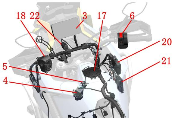
20-LCM Lighting Controller 21-Fog Lamp Controller 22-USB charging cable
