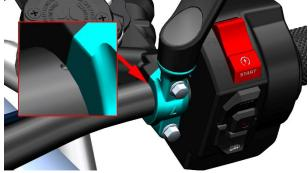
d. Align the long scale on the direction handle with the upper surface of the cushion block and reinstall the pressure block.
