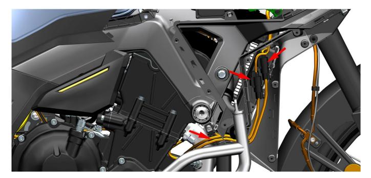
After removing the cover, you can see that the oxygen sensor is fixed as shown in the figure above, squeeze the mushroom head out of the fixing hole, unplug the oxygen sensor connection plug to measure, and use a multimeter to measure the pin resistance of the pin corresponding to the purple wire and the white wire of the oxygen sensor, the standard value is  $12.5\pm1.7\Omega$ ; If the resistor is small or infinite, it needs to be replaced.
