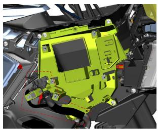
e. Use a T25 Allen Torx wrench to remove four M6×14 shoulder bolt bolts (1) and one M6×16 shoulder bolt bolt (2).
