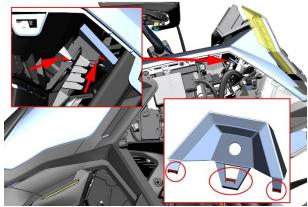
c. Remove the meter assembly
