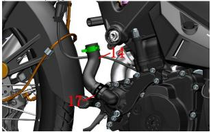
b. Remove the auxiliary water tank decorative cover (18) forcefully in the horizontal direction; use the plum blossom T25 hexagon to remove the two shoulder bolts (19) that fix the auxiliary water tank; then use the needle-nose pliers to loosen the  $\phi$ 10.5 hoop (22) on the auxiliary water tank connecting water pipe (23), remove the auxiliary water tank (20) and the auxiliary water tank leaking pipe (21).
