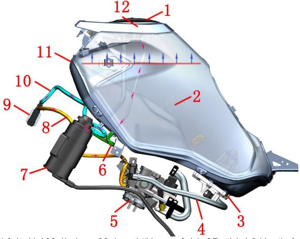
1-Electronic fuel tank lock 2-Fuel level sensor 3-Fuel pump 4- High pressure fuel pipe 5-Throttle body 6- Adsorption /vent pipe 7-Carbon canister 8-Solenoid valve outlet pipe 9-Carbon canister solenoid valve 10-Solenoid valve inlet pipe 11-Fuel tank 12-Oil-gas separator (inside the fuel tank lock)
