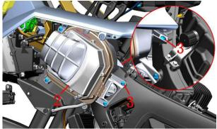
b. Use the 4# hexagon to pass through the  $\Phi$ 59×9 pipe hoop assembly (4) on the connecting pipe assembly (5) of the air filter through the gap of the air inlet cavity assembly (2) on the left side of the air filter, and then pull out the air inlet cavity assembly (2) on the left side of the air filter in the direction of the arrow, and remove the air inlet cavity assembly (2) on the left side of the air filter.
