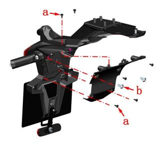
b. Use a Phillips screwdriver to remove the two self-tapping screws that fix the blind zone radar, loosen the blind zone radar and the plug interface, and pull out the blind zone radar.
