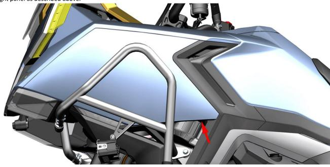
Use a Phillips screwdriver with a diameter of 6mm and a length of  $150\sim200$ mm to align the sawtooth of the dimming bolt, rotate it counterclockwise to turn it down, and turn it clockwise to turn it up.
