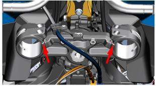
b. Use a flathead screwdriver to pry open a gap in the upper plate, insert the corresponding shock absorber, and adjust the shock absorption to just expose the end cap (as shown in the figure). Remove the flathead screwdriver after installing the shock absorber in place. Use 6# hexagon to tighten the bolt at the upper plate, torque standard: 25N.m.
