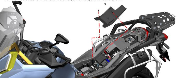
Press the anti-disengagement clip and pull the plug out. Use the 4# hexagon socket to remove the two bolts to remove the dump switch.
