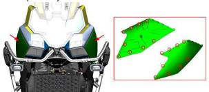
c. Remove the 2 torx groove plate head bolts (3) with a hole torx wrench, and remove the 2 fuel tank flat pads (4) and glue pressing (5). Remove 2 inner torx shoulder bolts (1) with T25 torx socket sockets. Remove 2 expansion nails (2) with a cross batch.
