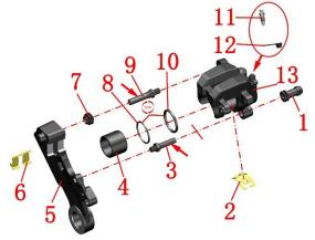
1-Caliper mounting plate pin cap 2-Bouncy cards 3-Lower slide axis 4-piston 5-Caliper mounting plate 6-card 7-Caliper pin cap 8-Dust-sealed 9-Upper sliding axes 10-Oil seals 11-Bleed nozzle 12-Bleed nozzleGlue caps 13-Caliper housing
