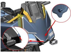
b. Use a cross batch or other suitable tool to reach through the gap in the front of the motocycler to push the buckles of the hood panel open, and pull all the buckles open to remove the hood panel.
