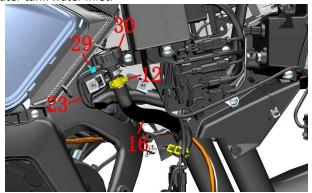
Use an 8# torx wrench to remove the bolts (25) of M2 M6×22 on the thermostat (3), and then take out the thermostat (25).
