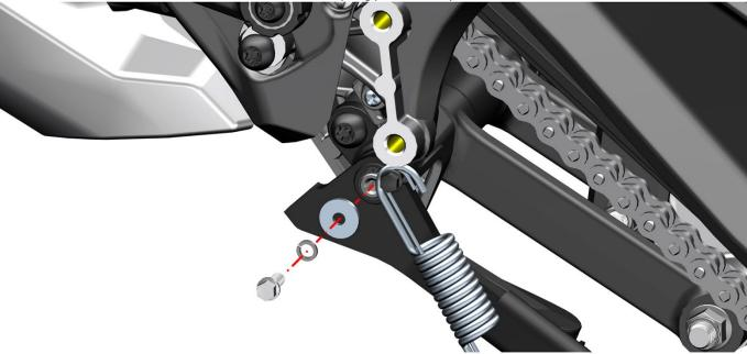
c.Refer to the method of removing the side bracket spring to remove the main bracket spring. After removing the bolt on the front of the main bracket (a) in a counterclockwise direction with a T50 plum blossom socket with holes, rotate the main bracket down until the other bolt is exposed (b in the figure)
