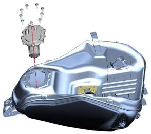
Note that you should not press the oil outlet pipe shown in the red circle, and once damaged, you can only replace the entire fuel pump assembly.
