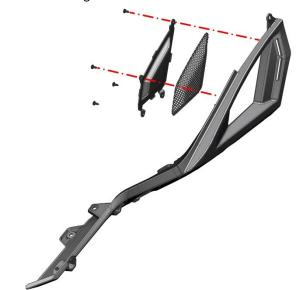
f. Remove the expansion nail fixed on the right tail skirt and the right cover, and then remove the right cover.
