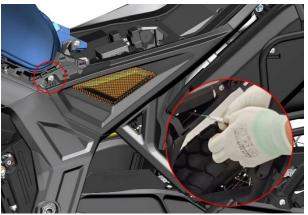
c. Unplug the decorative cover of the auxiliary water tank, and use the T25 plum hexagon to remove 2 M6×12 bolts (1), 1 M6×16 bolt (2), 1 M6×16 shoulder bolt (3), and 1 M6×14 shoulder bolt (4).
