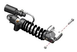
c. If you need to replace the rear shock-absorbing straight connecting rod, you can remove the straight connecting rod according to "Maintenance - Main Bracket". Note: A jack or support is required to support the vehicle.
