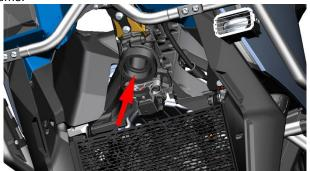
b. Place the lubricated bearings, shaft rings, and dust cover above the lower connecting plate in sequence, then screw in one steering column adjusting nut. Use a four jaw socket to tighten the steering column adjusting nut to a torque of 50N. m (5.1 kgf. m, 37 lbf. ft), ensuring that the upper connecting plate does not move up and down. Loosen the steering column adjusting nut counterclockwise by 1/4
