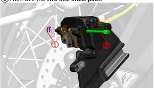
b. With the help of a tool, push the piston in the direction of the arrow to the end. If the resistance is very large, you can refer to the method of adding brake fluid to the front brake main cylinder, remove the upper cover and then push it. If the spring blade on the caliper falls off, it needs to be replaced in the direction shown.
