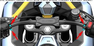
b. Buckle down the 4 decorative buckles on the pressure block, use 6# hexagon socket to remove the 4 bolts, remove the pressure block, and pick up the handlebar.
