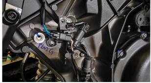
b. The RMC-HU removal method is detailed in the section on removing the rear disc brake caliper at the front. Directly remove the RMC-HU tubing. Pull the RC-HU tubing and wheel speed sensor out of the three-piece tubing clamp
