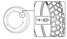
The sidewall triangle ( $\triangle$ T.W.I.) markings indicate the position of the wear strips. If it is worn to the marked point, it means that it has been worn to the limit, and it will be a safety hazard to continue driving, and it must be replaced with new tires of the same specification.
