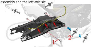
c. Use a T25 torx wrench to remove 7 bolts, and remove the tubing clamp and wear block. Use a 13# open-end wrench to remove the two bolts and nuts in the grooves of the rear flat fork.
