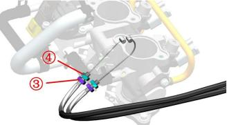
If neither of these adjustments is effective, a new throttle cable will need to be replaced.
