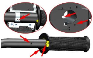
c. When installing the front disc brake half cover or clutch rocker arm half cover, align the joint surface of the half cover and the disc brake master cylinder or the half cover and the clutch rocker arm with the round hole on the handlebar, and then use an 8# sleeve to tighten the bolts. Note that you need to tighten the top bolts first, then tighten the bottom.
