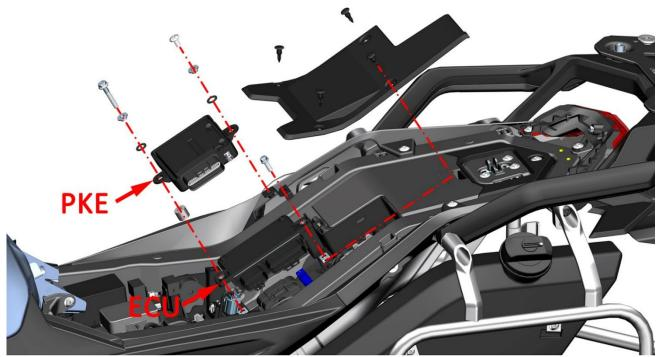
Note: To replace the ECU, you need to shut down the whole vehicle and wait for 10 seconds before operating to avoid the abnormality of the EFI system.
