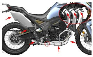
b. If there is a slight air leakage at the connection between the engine and the muffler, you can first try to tighten the exhaust nut (3) with 6# hexagon socket; If the problem is not resolved, the muffler needs to be removed and replaced with a new engine exhaust gasket (4). The specific disassembly method can refer to the disassembly of the muffler.
