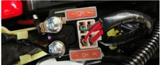
When reinstalling the relay, the red wire is installed on the threaded hole of the relay marked "B", and the black wire is installed on the threaded hole of the relay marked "M". Make sure the protective cap is closed after the screws are tightened, and then plug in the relay connector.
