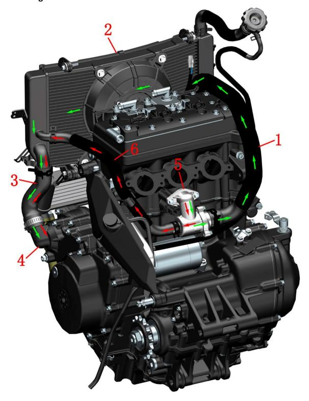
1-Main water tank inlet pipe 2-Main water tank 3-Engine water inlet pipe 4-Water pump assembly 5-Thermostat assembly 6-Small circulation water pipe
