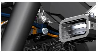
d. Remove the bolts that hold the tubing with 5# hexagon socket and loosen the FC-HU tubing.
