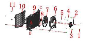
1-Fan motor bolt\*3 2-Fan motor 3-Fan passport bolt\*4 4-Spring pad\*4 5-Gasket\*4 6-Fan guard 7-Fan 8-Fan nut 9-Water tank 10-Water tank front guard 11-Shoulder bolt\*4
