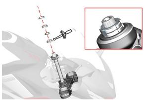
d. After the upper plate assembly is installed, the nut (5) is tightened with the decorative nut tooling, and the torque: 100N.m. Use a T45 torx wrench with holes to tighten the bolt (6) on the upper plate, torque: 25N.m.
