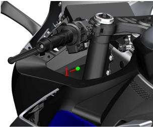
c. Under the front of the motorcycle, use a hook needle to remove the two expansion pins (1) that secure the surrounding interior trim. Then, use a T25 torx wrench to remove the two M6×14 shoulder bolts (2).
