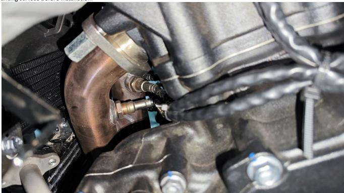
The new sensor threads are coated with a special paste thread anti-sintering agent to prevent air leakage and facilitate subsequent re-disassembly. If the old inspection is fine, it is necessary to apply an appropriate amount of anti-sintering agent to the thread before installation. Torque standard: 18±1.5N.m.
