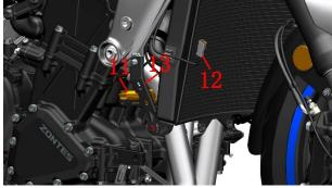
d. Use an 8# socket wrench to remove the M6×12 bolt (7) securing the right lower bracket (13) of the main radiator, and then take out the right lower bracket (13). Use an 8# socket wrench to remove the one M6×22 bolt (1) securing the main radiator. Use a hose clamp pliers to move the  $\phi$ 32 hose clamp (10) and  $\phi$ 9 hose clamp (14) to a suitable position, then disconnect the water pipes, and finally remove the main radiator assembly.
