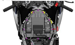
b. Remove the old air filter and put the new air filter on the new one.
