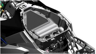
c. Use the T25 plum blossom hexagon to remove the 2 shoulder bolts (1) that fix the lower cover of the air filter, and then use the 6# hexagon to remove the 6 pieces of M6×16 bolts (2) at the outlet pipe of the air filter; Finally, take out the lower cover of the air filter and the air outlet pipe of the air filter and arrange the wiring harness. Note: Do not leak the air filter outlet pipe during installation.
