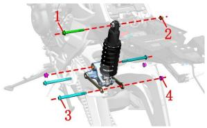
b.One person uses a 14# sleeve to fix the head of the bolt, and one person uses a 14# sleeve to remove the nut, remove the bolt, and remove the rear shock absorber and triangle bar assembly. Nut torque: 65±5N.m (6.6±0.5 kgf.m, 48±4 lbf.ft)
