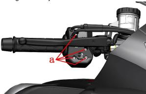
b. Use a Phillips screwdriver to remove the three bolts securing the rear cover of the left handlebar switch, and then take off the rear part of the left handlebar switch. Disconnect the heater harness connector and remove the bolt securing the front part to detach the front of the switch.
