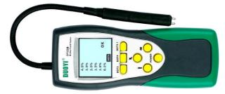
The picture above shows the brake fluid moisture content tester, the picture comes from the Internet, and the copyright belongs to the author of the original picture. Do not use for any other purpose.
