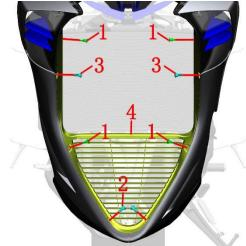
b. Remove the middle of the bracket (4).
