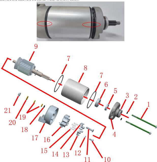
1-M5×98 bolt× 2 2-O ring×2 3-O ring 4-starter motor front cover 5-oil seal 6-bearing 7-rectangular sealing ring 8-starter motor outer shell 7-rectangular sealing ring 9-electric pestle 10-screw ×2 11-head screw with limit 12-washer 13-negative brush×2 14-positive brush×2 15-worm spring ×4 16-insulating brush frame 17-starter motor back cover 18-sealing rubber ring 19-insulating gasket 20 anti-loosening gasket 21 nut
