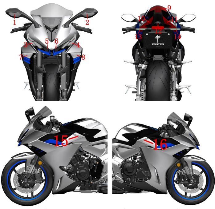
1-Right turn signal 2-Left turn signal 3-Right daytime running light 4-Left daytime running light 5-Right front position light 6-Left front position light 7-Right front headlight 8-Left front headlight 9-Brake light 10-Left position light 11-Right position light 12-Rear license plate light 13-Left rear turn signal 14-Right rear turn signal 15-Frame left grid atmosphere light 16-Frame right grid atmosphere light
