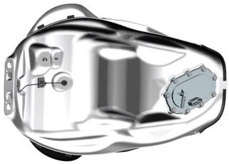
When disassembling and assembling the fuel tank, after removing the fixing screws of the fuel tank, you must first gently lift it from the tail of the fuel tank, raise it until your hand can just reach into it, and then pull out the high-pressure oil pipe connected to the oil pump.
