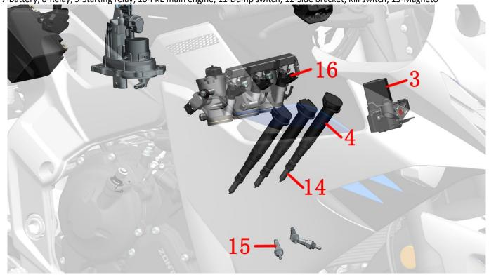
14-spark plug 15-oxygen sensor 16-fuel injector
