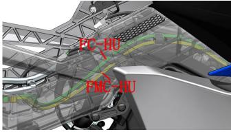
e. Check whether the cable is damaged, if there is wear and tear on the cable sheath, it needs to be wrapped with electrical tape to avoid short circuit and motorcycle failure. Wrap it with electrical tape to avoid short circuits and motorcycle breakdowns.
