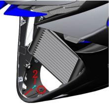
d.Use a T25 Allen Torx wrench to remove 1 M6×12 bolt as shown.
