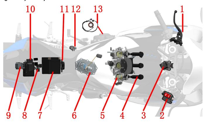
1-Clutch rocker arm assembly; 2-Right hand handle switch; 3-Faucet lock; 4- Ignition coil; 5-Throttle assembly; 6-Oil pump pump; 7-Battery; 8-Relay; 9-Starting relay; 10-PKE main engine; 11-Dump switch; 12-Side bracket; Kill switch; 13-Magneto
