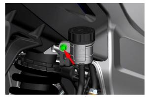
b. Unscrew the upper cover of the main pump counterclockwise and take out the rubber sleeve inside. Add the right amount of brake fluid
