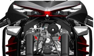
b. Reserve enough position for the shock absorber port of the upper plate to insert the corresponding shock absorber, and adjust the shock absorber to the position of just exposing the end cover (as shown in the figure). Use a T45 torx wrench with holes to tighten the bolts at the upper plate, torque standard: 25N.m.
