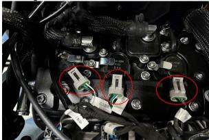
e. Use a 10# sleeve to fix the nut (3) and the pressing plate (4) and (5) of the ignition coil at 3 places, and then take out 3 ignition coils.
