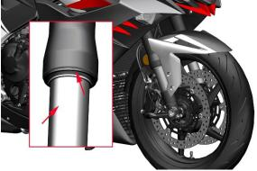
b. Check whether the bottom cylinder is peeling off the paint; Signs of whether the mounting points of the front fenders, front wheel hollow shaft and front brake calipers are broken or cracked. Check the bottom of the bottom barrel for leaks.
