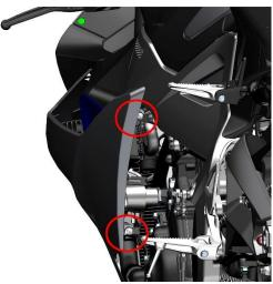
h. On the left side of the vehicle, carefully pull the buckle or mushroom peg indicated by the arrow from top to bottom, and remove the left bracket panel assembly.
