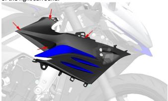
c. Use a T25 Allen Torx wrench to remove 2 M6×14 shoulder bolts.
