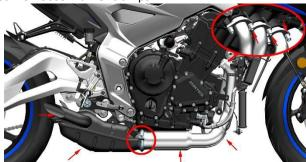
b. If there is a slight air leakage at the connection between the engine and the muffler, you can first try to tighten the exhaust nut (3) with 6# hexagon socket; If the problem is not resolved, the muffler needs to be removed and replaced with a new engine exhaust gasket (4). The specific disassembly method can refer to the disassembly of the muffler.
