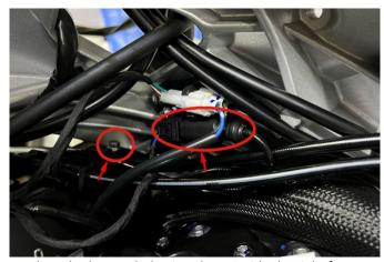
d. Undo the two-hole pipe clamp inside the right frame and pull the two tubing out of the front.
