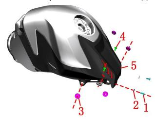
b. Use a Phillips screwdriver to remove the 4 non-standard Phillips self-tapping screws (1) fixed on the inner lining of the fuel tank interior cover, and remove the left and right decorative cover liners (2), and then remove the fuel tank middle cover (3).
