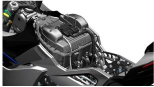
b. Refer to "Removal of Air Filter" to remove the upper cover of the air filter. And put the wiring harness in order.
