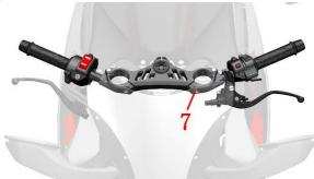
c. Use 6# hexagon to loosen 4 M8×35 bolts (8) for 5-8 turns, pry open the gap on the lower plate with a flathead screwdriver (as shown in the arrow), and remove the left front shock absorber and right front shock absorber.
