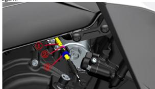
c. If the above two adjustments are invalid, a new clutch cable needs to be replaced.
