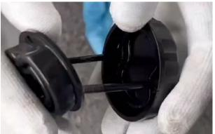
d. Use the brake fluid moisture content tester to measure the water content, if it is > 2%, all brake fluid needs to be replaced; If 2% is ≤, add freshly opened DOT 4 brake fluid to 3/4 of the clear viewing window of the front disc brake main cylinder. It is recommended that the water content should be less than 1.5%. TOTAL Total HBF 4 (DOT 4) brake fluid 0.22L (0.23 US qt, 0.19 Imp qt, 0.06 US gal, 0.05 Imp gal).
