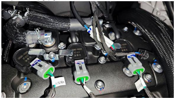
Remove the nut with the 10# sleeve and remove the ignition coil pressure plate. Remove the ignition coil. Use the 14# sleeve to remove the spark plug. If the fit is tight, you can shake it slightly from side to side to take out the ignition coil.
