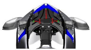
h. After removing the head lower liner, find the wiring harness connector of the left and right position lights and unplug them.
