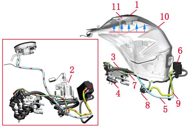
1-Fuel Tank Lock2-Fuel Pump 3-High Pressure Oil Hose 4-Throttle Valve Body Assembly 5-Adsorption/Snorkel 6-Carbon Canister 7-Solenoid Valve Outlet Pipe 8-Carbon Canister Solenoid Valve 9-Solenoid Valve Intake Pipe 10-Fuel Tank 11-Oil-Oil Separator (Inside Fuel Tank Lock)
