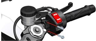
b. Tilt the front brake main cylinder so that the bolts are facing upward, remove the bolts with a 12# sleeve after wearing waterproof gloves, remove the copper pad and
