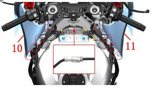
e. Grab the head of the fuel tank and lift the fuel tank, use the vise to loosen the exhaust pipe buckle, pull out the exhaust pipe, and then pull out the high-pressure oil pipe (12) and the power cord of the oil pump, and then remove the fuel tank.
