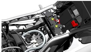
b. Then find the ventilation tube (2) of the carbon canister from the solenoid valve of the canister and pull it out, and take out the canister.
