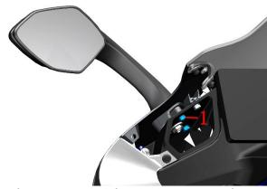
g. After removing the left and right surrounds of the interior, use a crochet needle to remove the 3 expansion nails (1) that hold the head lower liner in place, and remove the head bottom liner.
