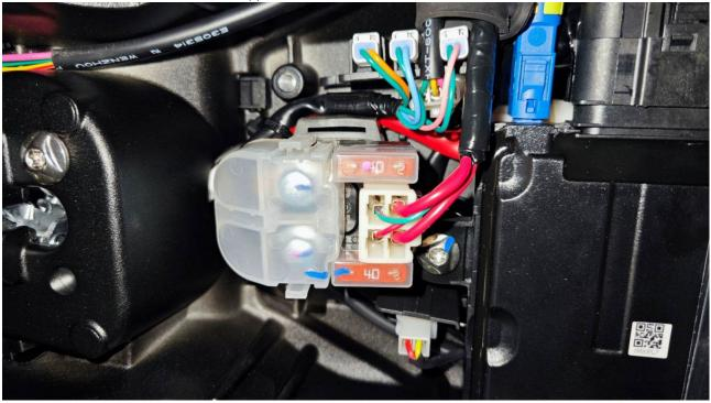
b. Unlock the vehicle, the engine shutdown switch hits "", retract the side bracket, pinch the brake handle and press the start button should be able to hear the sound of the starting relay sucking, otherwise the starting line should be checked.
