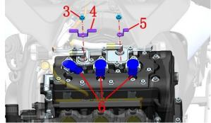
f. Use a dust blow gun to blow off the dust and debris near the spark plug.
