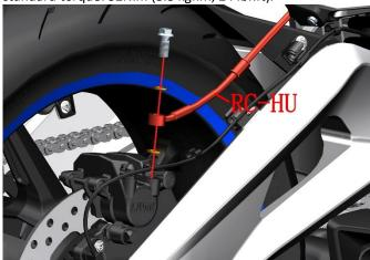
b. Remove the rear caliper and brake pads first by following the steps for removing the rear wheel and replacing the brake plate.
