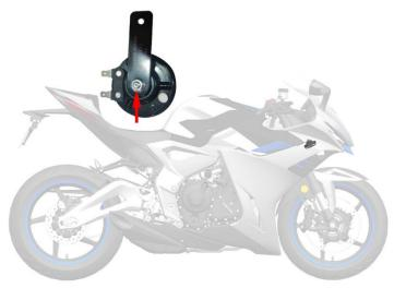
If you need to remove the horn, use the T25 Torx wrench to remove the 2 bolts. Pull the horn out and remove it after pulling the plug.
