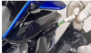
g. Use a T25 Allen Torx wrench to remove the 2 bolts of the  $M6 \times 12$ .
