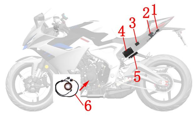
1- Charging port holder 2- Starter relay (40A) 3- Fuse box 4-Battery 5- Rectifier 6-Magneto
