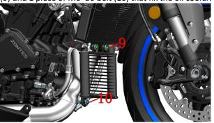
d. Use the 8# sleeve to remove the 4 bolts on the engine inlet and outlet pipes (11); Remove the oil cooler from the vehicle. Then adjust the inlet and outlet pipes to the appropriate position. Note: A small amount of oil may drip when the oil cooler is removed; When installing, please pay attention to whether the O-ring on the inlet and outlet pipes is damaged, and replace it immediately if there is a cut edge or damage.
