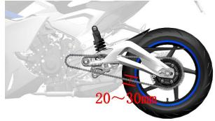
d. The tightness of the drive chain is incorrect, and it is adjusted according to the following procedure.
