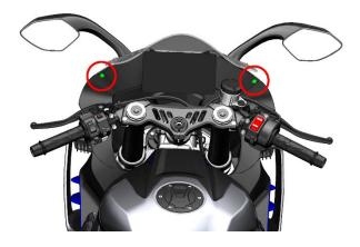
b. Use a crochet hook to remove one expansion nail from each of the left and right envelopes the interior (1).
