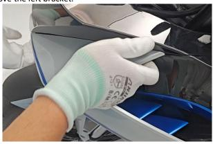
f. Use a crochet hook to remove the 2 expansion nails on the left side of the front panel.
