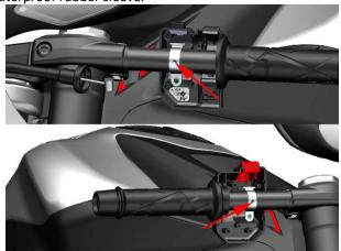
d. When installing the front disc brake half cover or clutch rocker arm half cover, the half cover and the disc brake main pump or the combination of the half cover and the clutch rocker arm need to align the round hole on the direction handle, and then use the 8# sleeve to tighten the bolts. Note that the top bolt needs to be tightened first, and then the bottom bolt should be locked.
