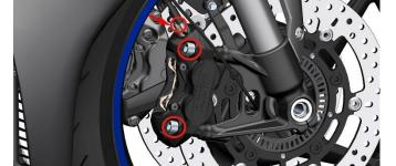
c. Front disc brake caliper disassembly
