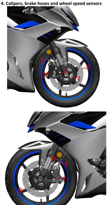
1-Brake hose left and right caliper interchange section 2-Disc brake caliper (front right) 3-Wheel speed sensor (front wheel) 4-ABS induction coil (front wheel) 5-Brake disc (front right) 6-FC-HU Brake hose 7-Disc Brake Caliper (Front Left) 8-Brake Disc (Front Left)
