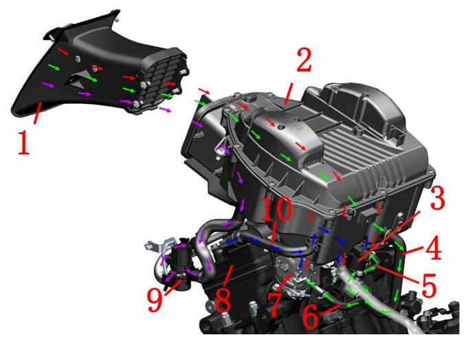
1-Stamping intake pipe assembly 2-Air filter assembly 3-Throttle fill valve 4-Stepper motor rubber hose (2) 5-Stepper motor rubber hose (3) 6-Stepper motor rubber tube (1) 7-Throttle valve body 8-Cylinder head 9-Secondary make-up valve 10-Exhaust gas snorkel
