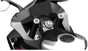
b. For the sake of illustration, other components are hidden here. Move the washer (1) up first, and then loosen the adjusting nut (2a).
