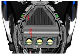
d. Unplug the 3 connectors on the ignition coil. And tidy up the wiring harness.
