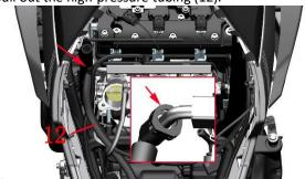
g. Install the high-pressure tubing (12) back according to the above steps.
