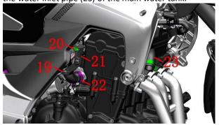
c. Use a T50 torx wrench with a middle hole to remove the bolts (19) of 1 M10×20 and 2 bolts (20) of M10×35 that fix the left hanging piece (24) of the main frame, and remove the left hanging piece (24) of the main frame; Then use the 8# sleeve to remove the bolts (1) of the two M6×22 fixing the thermostat (25), and take out the thermostat assembly (25).
