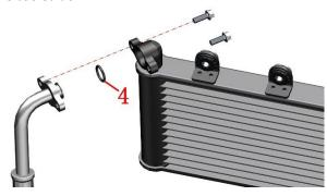
c. If the O-ring (8) on the oil pipe cannot solve the oil leakage phenomenon, the corresponding oil leakage oil pipe needs to be replaced.
