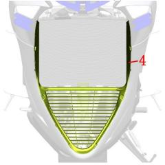
c.Use a T25 Allen Torx wrench to remove one of the shoulder bolts (2) of M6×14, and use a crochet hook to pry open the hook locks surrounding the left and right sides.
