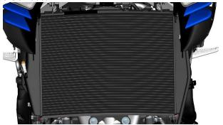
b. Use a flat carving knife or a small flathead screwdriver to straighten the deformed fins. If the fins are deformed by more than 20%, a new radiator will need to be replaced.
