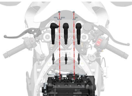
When installing the ignition coil back, first insert the ignition coil back into the bottom, and turn the ignition coil plug towards the position shown in the figure above, then put it back into the pressure plate, and put the nut back tight, and the torque standard is 11.5±1N.m.
