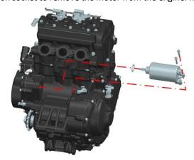
b. When reinstalling, pay attention not to miss the O ring of the starting motor, and align the teeth of the electric starting reduction gear. Note that the O-ring should be properly fitted into the box and properly lubricated, as cutting edges may cause leakage. Torque of the two bolts that fix the starter motor: 12±1.5 N.m. and mark with a marker.
