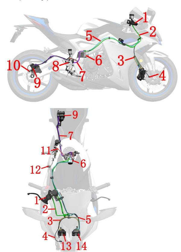
Front disc brake main cylinder 2- FMC-HU brake hose 3-Brake hose left and right caliper interchange section 4- Wheel speed sensor (front wheel) 5- FC-HU Brake Hose 6-ABS Hydraulic Control Unit 7- RC-HU Brake Hose 8-Rear disc brake main cylinder 9-Rear disc brake caliper 10-Wheel speed sensor (rear) 11- RMC-HU Brake Hose 12-Rear brake pedal 13-Front disc brake caliper (right) 14-Front disc brake caliper (left)
