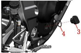
g. After waiting for the oil to flow out completely, wipe the oil drain bolts with a clean non-woven fabric, check whether there are scratches on the joint surface of the oil drain bolts, and replace them. Then use a clean non-woven fabric to wipe the joint surface of the engine and oil drain bolts.
