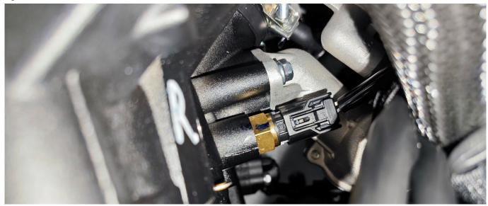
The two-pin resistance value of the multimeter at room temperature is:  $3.74^{\circ}1.22k\Omega(10^{\circ}40^{\circ}C)$ ;  $1.22^{\circ}0.27k\Omega(40^{\circ}90^{\circ}C)$ . Due to limited space, it is recommended to use a 72-tooth 17# ratchet torx wrench counterclockwise to remove the water and oil common sensor and remove the 9×2 EPDM O-ring. When reassembling, replace the O-ring with a new one to avoid leakage.
