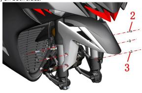
d. Remove the wheel speed sensor and brake hose from the front fender. Remove the M25 bolt (6×16) on the wheel speed sensor with a T4 torx wrench and remove the sensor. Remove the front brake caliper.
