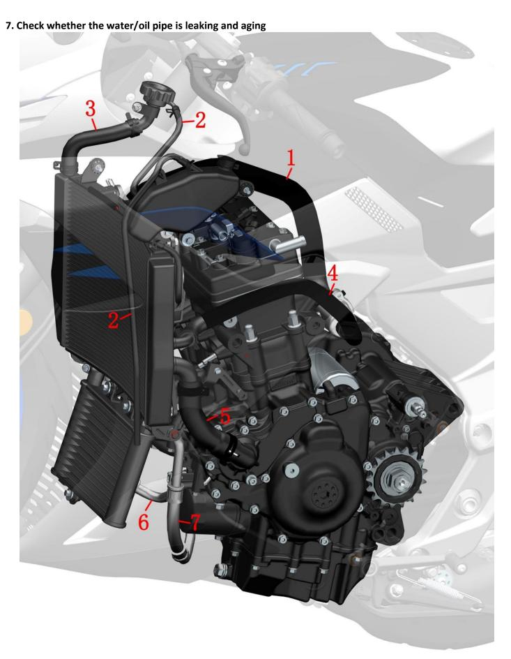
1- ZT703-F main water tank inlet pipe 2- ZT310-R auxiliary water tank leakage pipe 3- ZT703-RR water tank water inlet connection water pipe 4-ZT703-F small circulation water pipe 5-ZT703-RR engine water inlet pipe 6- ZT703-RR engine oil inlet pipe 7-ZT703-RR engine oil outlet pipe
