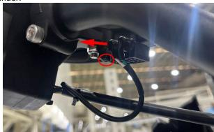
d. Use a 5# Allen wrench to remove the bolt (1) and remove the nut (2) to replace the clutch handle.
