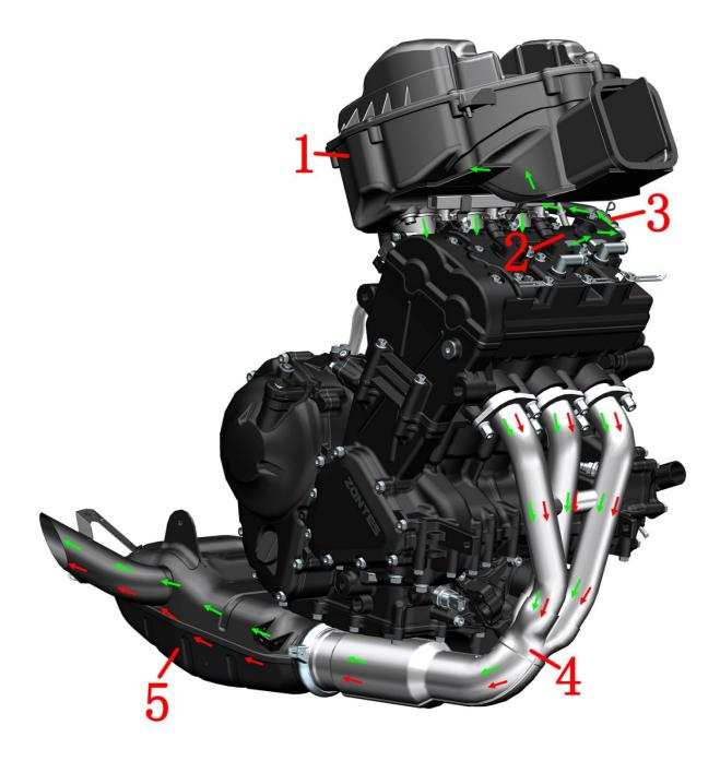
1-Air filter assembly 2-Cylinder head 3-Exhaust gas snorkel 4-Front muffler 5-Rear muffler Exhaust system:
