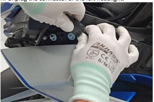
i. Use the 8# T-type sleeve to remove 1 M6×16 bolt (1), 2 M6×22 bolts (2), and remove the left headlight (3).
