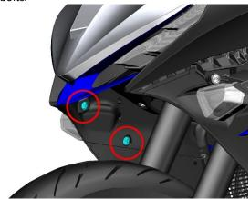
b. Carefully pull the buckle or mushroom staple at the point indicated by the arrow and remove the upper assembly of the right surround.
