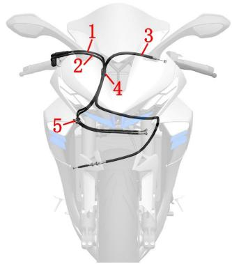
1-Refueling line, 2-Oil return line, 3-Clutch line, 4-Throttle line, limit bracket, 5-Throttle cord clamp
