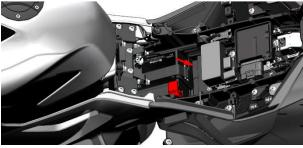
b. After pulling out the battery, first disconnect the negative terminal by removing the black protective cap, followed by the positive terminal. Then, remove the battery.
