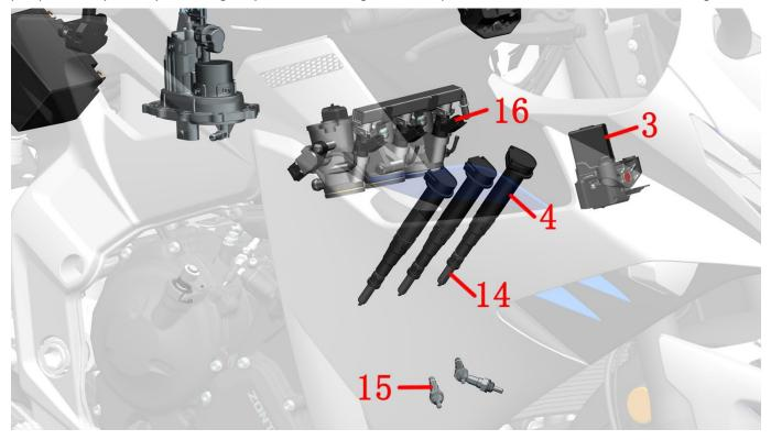
14-spark plug 15-oxygen sensor 16-fuel injector Note:
