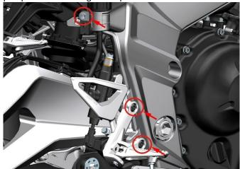
b. Use the 8# sleeve to remove the two bolts on the rear brake switch bracket and the bolt fixed on the rear section of the rear brake pedal by the rear brake main cylinder, wear
