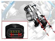
Simple test method: take out the stepper motor after turning off the power, do not loosen the cable plug, press the power-out switch at start-up, do not ignit, check whether the motor plug can shrink back and forth, and finally turn off the power-out switch to see if the plug returns to its original position. To check whether the stepper motor is abnormal, measure whether the resistance at both ends A and B is  $53\pm5.3\Omega$ .
