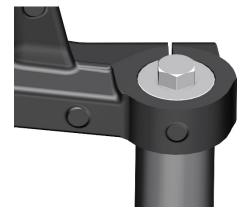
c.Install the two M8×30 bolts on the lower link plate, and use the same method to install the other shock absorber.
