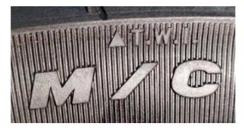
The tread bulge has a wear mark height of 1.6 mm (0.06 in). The sidewall triangle (IT.W.I.) markings indicate the position of the wear strips. If it is worn to the marked point, it means that it has been worn to the limit, and it will be a safety hazard to continue driving, and it must be replaced with new tires of the same specification.
