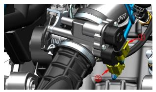
e.Use a short Phillips screwdriver to remove the 2 bolts (3) and the anti-release card (4) that come with the throttle body assembly, and then remove the stepper motor (4).
