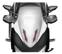
b.Use a T25 Allen Torx wrench to loosen the 4 M6×16 bolts on the left and right decorative covers of the windshield. Take out the left and right trim covers, windshields, and windshield bracket rubber pads from the windshield in turn.
