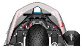
b.Use the T25 torx wrench to remove the 4 M6 ×14 shaft shoulder bolts (2) on the left and right sides of the rear tail light assembly. Unplug the wiring harness connector connecting the left and right parts of the rear tail light, and then remove the rear tail light assembly.
