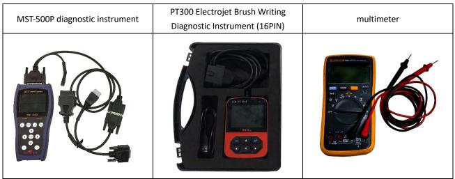
•Both of the above diagnostic instruments can read fault codes; The PT300 diagnostic device can be flashed into the program. 8.Each motorcycle has different driving conditions and maintenance conditions, so it is not possible to list all the fault phenomena and troubleshooting procedures. Only some of the more common faults can be listed. Maintenance personnel themselves also need to have a certain amount of professional knowledge and experience accumulation process.
