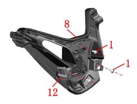
**2.Disassemble the direction to put the assembly** a.Use a T25 Allen Torx wrench to remove the 2 bolts (1).
