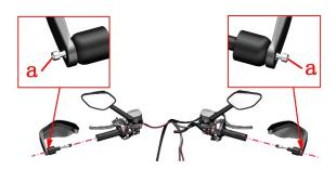
c.Remove 4 M6×30 bolts (2) with 5# hexagon socket,
