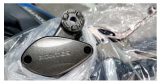
d.After wearing waterproof gloves, remove the bolt (1) with a Phillips screwdriver, and remove the upper cover (2), cover plate (3), and sealant gasket (4).
