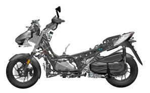
c.Refer to the steps of disassembling the engine, and unplug the wiring harness plug, oil pipe interface and water pipe interface on the engine. Remove the plug from the rear wheel speed sensor. Refer to the "Throttle Cable" procedure to remove the throttle cable from the turntable. Park the motorcycle in a flat and wide area, turn the steering bar to the right, place the stool at the appropriate height under the arrow, and tiptoe the rear wheels of the motorcycle off the ground.
