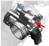
g.Install the stepper motor back on the valve body, taking care not to miss the sealing ring. Plug the plug back.
