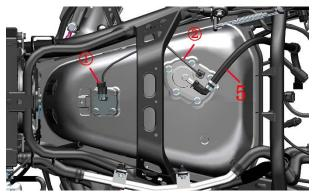
g.Use pliers to remove the clamp on the canister that connects to the oil and gas sensor and remove the hose.
