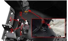
e.Use a T25 torx wrench to remove the 4 M6×14 shoulder bolts (1) of the box panel assembly, and then take out the box panel assembly.
