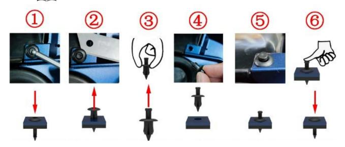
①Press down the center cylinder with 4# hexagon or other tools, you can hear a sound or the center cylinder moves axially by 2mm (0.079 in);
