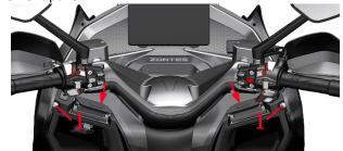
**Disassembly of windshield motor components** a.Use the 8# socket to remove the 2 M6×22 bolts (1), remove the bushing (2), buffer glue (3), controller (4) and flasher bracket assembly (5).
