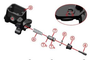
④Piston pushrods ⑤Dust cap ⑥Retaining rings ⑦Piston assembly (⑦a Outer seal ⑦b Inner seals) ⑧spring
