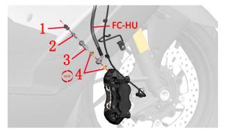
c.Remove the brake pads. d.Disassemble the front disc brake caliper.
