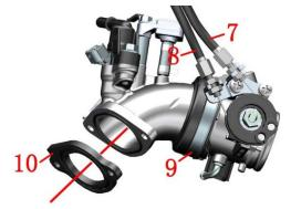
g.Use throttle body cleaner to clean the carbon deposits on the intake manifold and the throttle body outlet. Do not soak the throttle body assembly and intake manifold assembly directly in any liquid.
