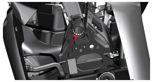
b.Put in the direction column dust cover (1) and the direction column adjustment nut (2) in turn. Then use the adjusting nut tooling to tighten the torque. Tighten 50N.m (5.1kgf.m, 37 lbf.ft), loosen 1/4 turn, then tighten 15N.m (1.2kgf.m, 11 lbf.ft).
