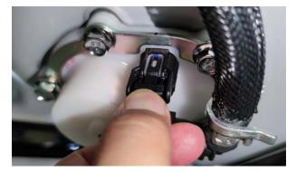
Note that you should not press the outlet pipe shown in red, and once damaged, you can only replace the entire fuel pump assembly.
