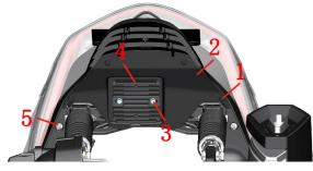
**Disassembly of the rear taillight assembly** a.Use a T25 Torx wrench to remove the 2 M6×16 bolts (1) at the bottom of the rear taillight assembly.
