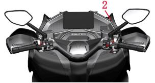
c.Turn on the motorcycle and open the left and right locks. Use a T25 Allen Torx wrench to remove the bolts (1) of the 2 M6×14 shaft shoulders as shown in the figure, and remove the front panel.
