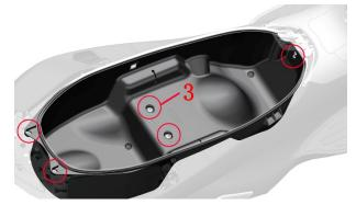
c.Lift the rear of the locker slightly until the wiring connector on the left side of the locker is exposed, unplug the
