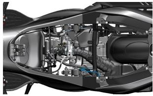
b.Use a T25 torx wrench to remove the 4 shoulder bolts (1) of M6×14 on both sides and the 4 expansion nails (2) in the middle. Remove the bottom of the lower bracket (3).
