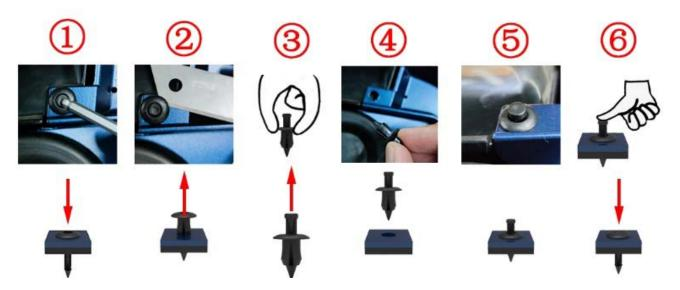
①Press the center cylinder with 4# hexagon or other tools, you can hear a sound or the center cylinder moves axially by 2mm; ②Use a razor, fingernail or carving knife to pry open the gap and remove it; If space permits, reach for the back and push it out;
