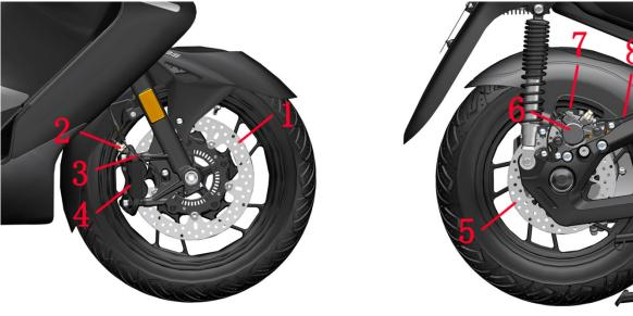
1-Front brake discs2-FC-HU Brake hoses3-Wheel speed sensor (front)4-Front disc brake calipers5-Rear brake disc6-Rear disc brake calipers7-Wheel speed sensor (rear)8-RC-HUBrake hoses
