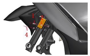
d.First, press down on both sides of the front mud board according to the small arrow, press the bulge at the front mud board arrow inward, and then move the front mud board up to the appropriate part and pull it out according to the direction of the big arrow.
