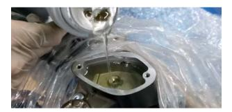
f.Observe whether the liquid level of the main pump is at 3/4 of the transparent inspection place, if not, it needs to be added or pumped out or discharged with a syringe.
