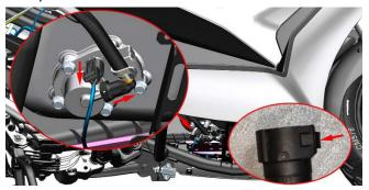
If you need to remove the fuel pump from the vehicle, you can use a siphon pump to drain the fuel from the fuel tank.After lifting the vehicle, press the plug clip as shown in the diagram to disconnect the wiring.Using a 10mm socket, remove the 5 bolts from the bottom, then remove the highpressure fuel line bracket. Once the bracket is removed, the fuel pump can be taken out.
