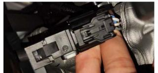
The resistance value of the heating element measuring the two white wires with a multimeter is  $9\pm 2k\Omega$ ; or measure its current should be  $\leq$  2.1A. Otherwise, it can be judged that the oxygen sensor is faulty. The ceramic inside the oxygen sensor
