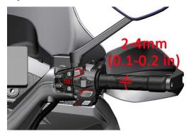
d.After starting the engine, turn the steering knob left and right to make sure the idle speed does not change during steering, and then turn off the ignition.
