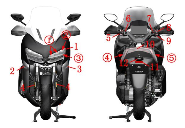
1-headlight (1)-low beam position 2)-High beam position 3)-Position light/daytime running light position 2-Right turn signal 3-Left turn signal 4-side reflector 5-Left hand handle switch 6-Left hand handle sub switch 7-Right hand handle sub switch 8-Right hand handle switch 9-Handle the heating switch 10-Rear tail light (4)-Rear left turn signal 5)-Rear right turn signal 11-rear reflector 12-rear license plate lamp
