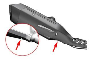
•The oil, mud and other stains on the surface of the muffler should be cleaned off in time.
