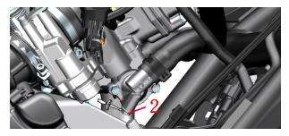
**4.Drain the coolant** a.Place the oil tray at the bottom, wear waterproof gloves
