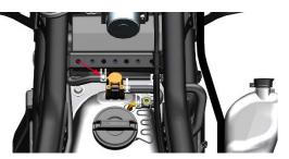
h.Use a ratchet wrench + 10# socket to remove 4 M6×16 bolts (6), and remove the springpad (7) and washer (8).
