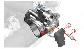
Simple test method: connect the whole motorcycle to the diagnostic instrument, press the ignition switch (no need to ignite), turn the throttle handle from the initial position to full open, this process to see if the throttle position signal follows the change from 0 to 100.
