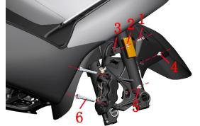
c.Use the 5# hexagon socket to remove 1 M6×30 bolt (1) and remove the spacer (2). Use a T45 Torx Allen wrench to remove the shoulder bolt (4) of one M6×14.
