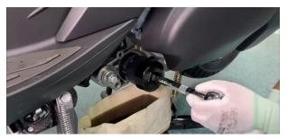
c.Drain the oil inside the fine filter.
