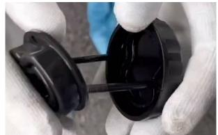
d. Use the brake fluid moisture content tester to measure the water content, if it is > 2%, all brake fluid needs to be replaced; If 2% is  $\le$ , add freshly opened DOT 4 brake fluid to 3/4 of the clear viewing window of the front disc brake main cylinder. It is recommended that the water content should be less than 1.5%. TOTAL Total HBF 4 (DOT 4) brake fluid 0.22L
