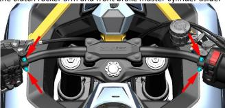
b. Buckle down the 4 decorative buckles on the pressure block, use 6# hexagon socket to remove the 4 bolts, remove the pressure block, and pick up the handlebar.
