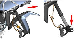
e. Use a T25 torx wrench to remove the two bolts under the lower fender, and remove the fender, flanging bushing, and flanging bushing buffer glue of the lower link.
