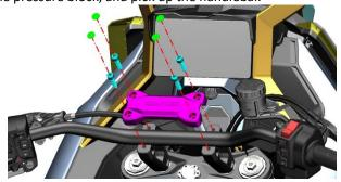
c. Use a Phillips screwdriver to remove the three bolts on the back cover of the right-hand switch, then remove the bolts that secure the throttle cable, and separate the front and rear parts of the right-hand switch.
