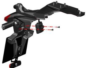
c. Use the 4# hexagon to remove the two M6×16 non-standard inner plum bolts in front of the billboard, and unscrew out the two GB6177 nuts that fix the bolts, take out the rear billboard obliquely, and use the 4# hexagon to unscrew out an M6×14 inner plum shaft shoulder screw, remove the rear reflector bracket and the rear reflector.
