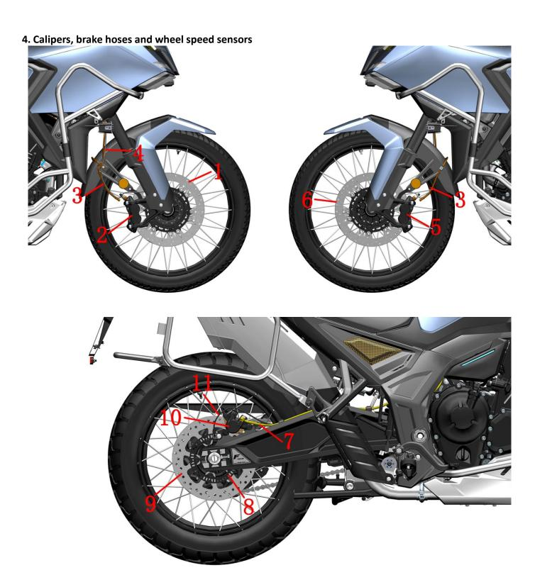
1- Brake disc assembly (front right) 2-Disc brake caliper (front right) 3-FC-HU brake hose 4-Wheel speed sensor (front wheel) 5-Disc brake caliper (front left) 6-Brake disc assembly (front left) 7-RC-HU brake hose 8 - Rear wheel A BS induction coil 9 -Brake disc (rear) 10-Rear disc brake caliper 11-Wheel speed sensor (rear wheel)
