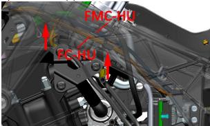
f. Find the plug of the wheel speed sensor on the right side of the vehicle (near the upper right guard), press the anti-disengagement card and pull out the plug.
