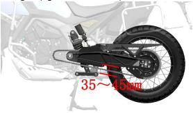
d. The tightness of the drive chain is incorrect, and it should be adjusted according to the following procedures.
