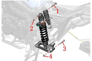
b. One person fixes the head of the bolt with a 14# sleeve, and one person uses a 14# sleeve to remove the nut, remove the bolt, and remove the rear shock absorber and triangle bar assembly. Nut torque:  $65\pm5$ N.m ( $6.6\pm0.5$  kgf.m,  $48\pm4$  lbf.ft).
