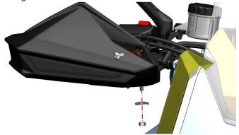
b. After grasping the front brake main cylinder, remove the 2 bolts with the 8# sleeve to remove the front disc brake half cover and the rearview mirror assembly.
