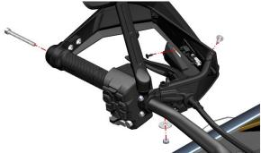
b. Use a cross screwdriver to remove the two self-tapping screws on the handlebar guard and remove the turn signal. Use a T25 plum wrench to remove the two bolts and separate the balance weight and the hand guard.
