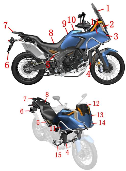
1. Windshield 2.Front right position light 3.Right surround upper part 4.Right bracket lower part 5.Right side cover 6.Rear fender 7. Rear armrest 8.Seat cushion 9.Fuel tank 10.Fuel tank trim cover 11.Right bumper panel 12.Windshield lining 13.Headcover panel 14.Front left headlight 15.Guard
