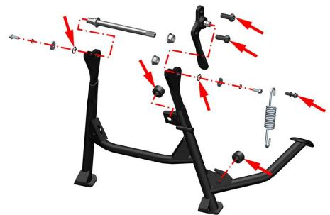
Inspect the parts indicated by the arrows in the picture above, and the disassembly method is detailed below.
