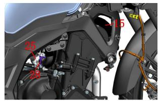
f. Find the fog lamp drive box on the right side of the vehicle and use the Torx T25 hexagon to remove 2 fixed axle shoulder bolts (19), remove the fog lamp drive box.
