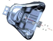
When reassembling, it is necessary to pre-tighten diagonally and then tighten 4 bolts, otherwise the sealing rubber ring of the oil level sensor is compressed unevenly, which will easily lead to leakage and cause potential safety hazards.
