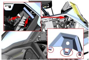
c. Remove the meter assembly
