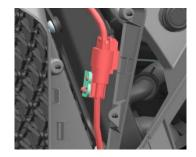
0.9V, if the voltage signal has been low or high, you need to check whether the oxygen sensor circuit is damaged and tie iron, If the cable is normal, the oxygen sensor needs to be replaced.
