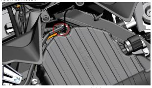
c.Remove the canister assembly (1) from the air inlet cavity assembly (2) on the left side of the air filter according to the direction of the large arrow, and pull out the rubber tube (1) on the canister assembly (1) in the direction of the small arrow, and remove the canister assembly (1).
