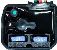
•Note: When reassembling the battery or fuse, please remember to reset the EFI hardware, as detailed in the service information in this section.
