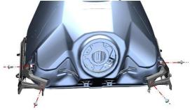
d. Push the left and right cover mesh lining plate assembly in the direction of the arrow, and remove the assembly after pushing to the hole position.
