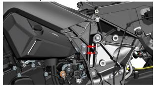
d. After grasping the hydraulic control unit, use a T25 torx wrench to remove the two M6×16 bolts, and the hydraulic control unit can be removed. If you need to replace the bracket, you will need to remove the flanging bushing and cushioning glue.
