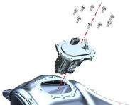
When reassembling, it is necessary to pre-tighten diagonally and then tighten 9 bolts, otherwise the uneven compression of the sealing rubber ring of the fuel pump will easily lead to leakage and potential safety hazards.
