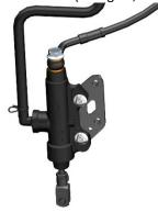
c. Use a Phillips screwdriver to remove the expansion pegs that hold the rear brake oil cup in place.
