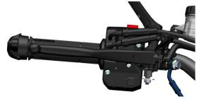
b. Use a syringe to absorb the sewing machine oil and inject a small amount of oil into the gap between the throttle cap and the core several times, and turn the throttle while injecting.
