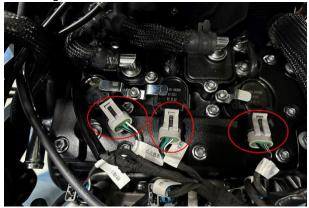
d.Use a 10# sleeve to remove 2 ignition coil pressure plates, and take out 3 ignition coils.
