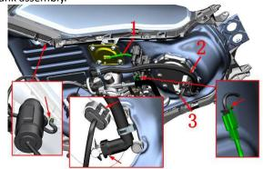
i.Refer to the steps of removing the air filter, remove the air filter first, press the anti-release lock in the direction of the arrow, and then pull out the high-pressure oil pipe. After replacing the high-pressure oil pipe with a new one, follow the disassembly steps to restore.
