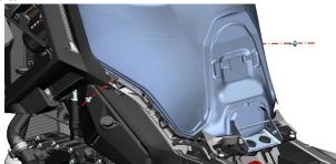
f. Use the hexagon tool to remove the 2 expansion nails in the direction pointed by the arrow pointing to the lower part of the left surround, and remove the right side in the same way.
