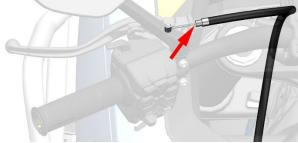
c.If lubrication does not solve the problem of high resistance, the throttle cable needs to be replaced.
