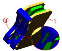
i.Press and hold the piece at the point of arrow (5) inward with hand, and insert the pin (2) into the hole position to fix
