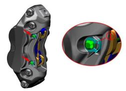
b. Use a T25 socket torx wrench to remove the upper pin (2) and then the lower pin in turn.
