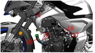
b. Use the T50 torx wrench with a middle hole to remove the bolts (19) of 2 M10×20 and 1 bolt (20) of M10×35 that fix the right suspension piece (21) of the main frame, and remove the right suspension piece (21) of the main frame; Use the clamps to remove the  $\varphi$ 36 clamp (22) and pull out the water inlet pipe (23) of the main water tank.
