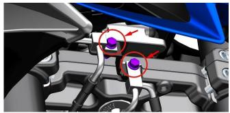
c. Use a T25 torx wrench and an 8# open-end wrench, remove the following two bolts, remove the front brake hose directional upper bracket, and pull out the front wheel speed sensor socket in the frame. For details, please refer to the air filter assembly removal procedure, and the air filter can be removed before finding the socket fixed on the right frame. Press the anti-loosening socket to pull it out.
