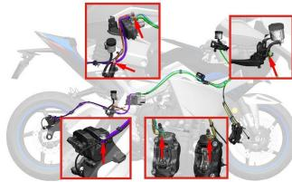
c. Measure the thickness of the front and rear brake discs, and replace them if they are less than 4.5 mm (rear brake discs are less than 4.0 mm). Suspend the front wheels
