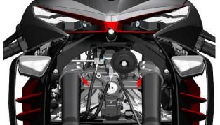
b. Reserve enough position for the shock absorber port of the upper plate to insert the corresponding shock absorber, and adjust the shock absorber to the position of just exposing the end cover (as shown in the figure). Use a T45 torx wrench with holes to tighten the bolts at the upper plate, torque standard: 25N.m.
