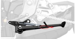
c. Grab the side bracket with one hand and pull the other hand in the direction of the arrow to remove the spring.
