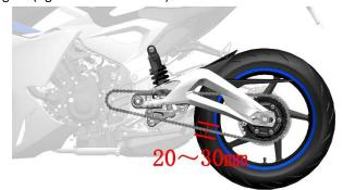
d. The tightness of the drive chain is incorrect, and it is adjusted according to the following procedure.
