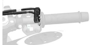
c. If the fault of high resistance cannot be solved after lubrication, the throttle cable needs to be replaced.
