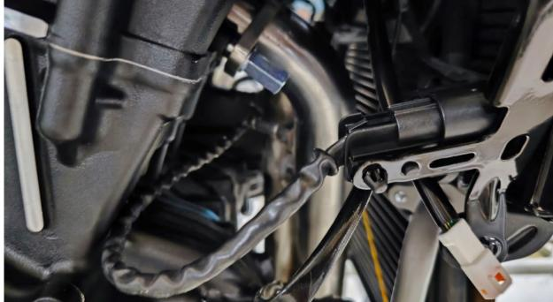
After removing the cover, you can see that the oxygen sensor is fixed as shown in the figure above, the mushroom head is extruded from the fixing hole, the oxygen sensor connection plug can be unplugged, and the pin resistance corresponding to the purple line and the white wire of the oxygen sensor can be measured with a multimeter, and the standard value is  $12.5\pm1.7\Omega$ ; If the resistor is small or infinite, it needs to be replaced.
