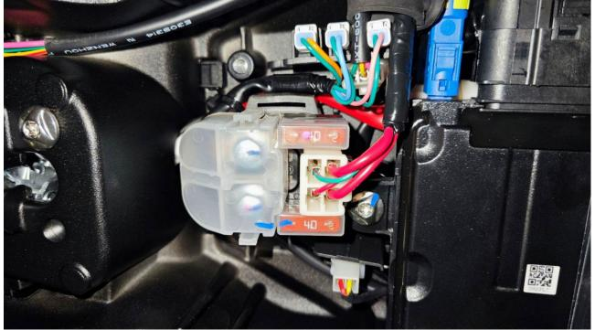
b. Unlock the vehicle, the engine shutdown switch hits "", retract the side bracket, pinch the brake handle and press the start button should be able to hear the sound of the starting relay sucking, otherwise the starting line should be checked.
