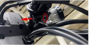
a. Pull out the two plugs of the front brake switch in the direction of the arrow, without distinguishing between positive and negative poles.
