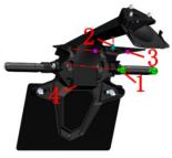
b. Use a T25 torx wrench to remove the 3 inner torx M6 bolts (1) that fix the subframe, and then remove the rear fender assembly from the subframe.
