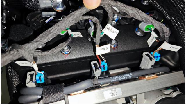
The static coil resistance measured with a multimeter should be  $12\pm0.6\Omega$ , otherwise the injector will fail and need to be replaced.
