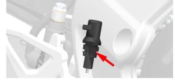
**3.Lubricate the movable parts of the brake handle and brake pedal**
