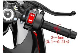
d. After starting the engine, turn the steering knob left and right to ensure that the idle speed remains unchanged during the steering process, and then turn off the engine.
