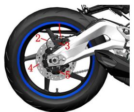
1-RC-HU brake hose 2-Wheel speed sensor (rear) 3-Rear disc brake caliper 4-Brake disc (rear) 5-Rear wheel sensing ring gear
