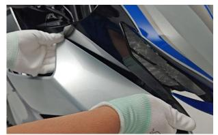
c. Use a crochet hook to remove the 2 expansion pegs on the right side of the front panel.
