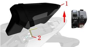
b. and use the 5# hexagon that has just been taken out to remove the 2 fixing screws (1), 2 flanging bushings (2) and 2 flanging bushing buffer glues (3) that fix the main cushion, gently push back the main cushion (4) with your hand, and remove the main cushion (4); For more information, please watch the saddle removal video.
