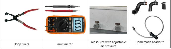
\* It can be plugged with a soft rubber plug, or folded in half with a hose and tied with a rope or wire as a plug for a small tube to test the tightness of the water tank filling port. A section of the water pipe with an inner diameter of 16mm can be found and assembled firmly with a suitable air pipe joint and clamp at one end to test the tightness of the water tank filling port and the main water tank and small water tank.
