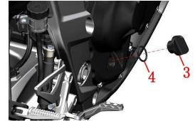
g. After waiting for the oil to flow out completely, wipe the oil drain bolts with a clean non-woven fabric, check whether there are scratches on the joint surface of the oil drain bolts, and replace them. Then use a clean non-woven fabric to wipe the joint surface of the engine and oil drain bolts.
