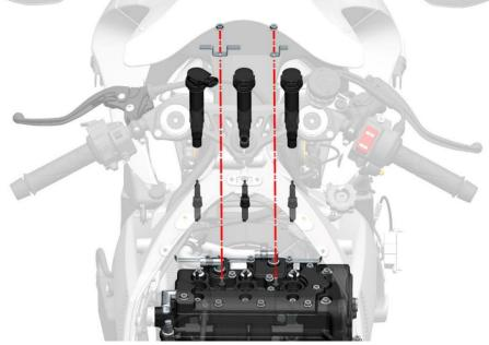
When installing the ignition coil back, first insert the ignition coil back into the bottom, and turn the ignition coil plug towards the position shown in the figure above, then put it back into the pressure plate, and put the nut back tight, and the torque standard is 11.5±1N.m.
