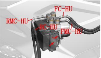
c. Use the T45 torx wrench with holes to remove the 2 bolts of the hydraulic control unit bracket, and remove the hydraulic control unit and the bracket assembly from the car.
