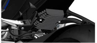
b. Unplug the 3 wires. Check the plug for looseness or corrosion.
