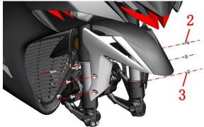
d. Remove the wheel speed sensor and brake hose from the front fender. Remove the M25 bolt (6×16) on the wheel speed sensor with a T4 torx wrench and remove the sensor. Remove the front brake caliper.
