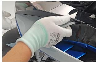
f. Use a crochet hook to remove the 2 expansion nails on the left side of the front panel.
