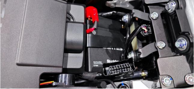
The charging voltage of the charger should not be higher than 15V. When the motorcycle is not used for a long time, it should be charged regularly in accordance with the requirements of the driver's manual. If the battery fails to be properly disposed of by a professional recycling organization, do not throw it away to avoid polluting the environment.
