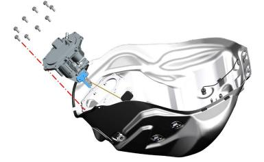
When reassembling, it is necessary to pre-tighten diagonally and then tighten 9 bolts, otherwise the uneven compression of the sealing rubber ring of the fuel pump will easily lead to leakage and potential safety hazards.
