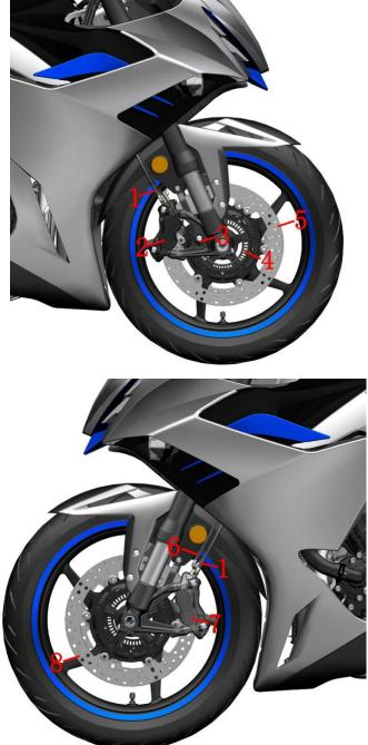
1-Brake hose left and right caliper interchange section 2-Disc brake caliper (front right) 3-Wheel speed sensor (front wheel) 4-ABS induction coil (front wheel) 5-Brake disc (front right) 6-FC-HU Brake hose 7-Disc Brake Caliper (Front Left) 8-Brake Disc (Front Left)
