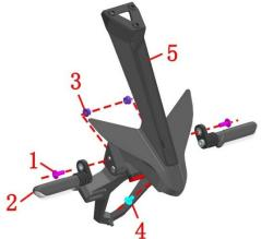
e. First, use a Phillips screwdriver to remove one nonstandard Phillips screw (1) that fixes the license plate light, then remove the license plate light (2), remove the rear reflector (3) from the rear fender assembly, and then take out two splint nuts (4); For more information, please watch the video of the rear fender assembly disassembly.
