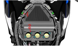
d. Unplug the 3 connectors on the ignition coil. And tidy up the wiring harness.
