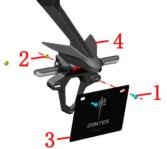
d.Use a T25 torx wrench to remove the two M6×16 inner torx shaft shoulder bolts (1) on the left and right sides, remove the left and right turn signals (2), then remove the two M6 nuts (3), and use the T25 torx wrench to remove one M6 bolt (4) that fixes the rear fender bracket (5), and then take out the rear fender bracket (5).
