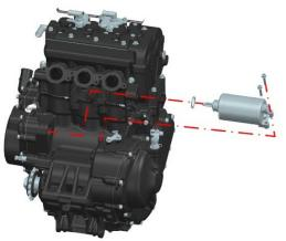
b. When reinstalling, pay attention not to miss the O ring of the starting motor, and align the teeth of the electric starting reduction gear. Note that the O-ring should be properly fitted into the box and properly lubricated, as cutting edges may cause leakage. Torque of the two bolts that fix the starter motor: 12±1.5 N.m. and mark with a marker.
