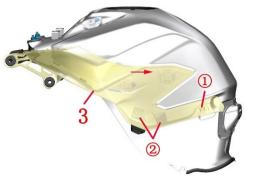
d. Break the buckle (1) first, then break open 2 mushroom tower buckles (2), and then pull gently in the direction of the arrow to remove the right decorative cover (4).
