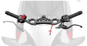
c. Use 6# hexagon to loosen 4 M8×35 bolts (8) for 5-8 turns, pry open the gap on the lower plate with a flathead screwdriver (as shown in the arrow), and remove the left front shock absorber and right front shock absorber.
