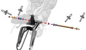
c.Use a 13# open-end wrench to remove the two bolts and nuts in the grooves of the rear flat fork.
