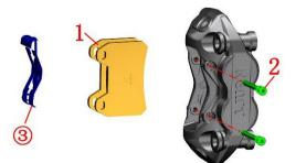
c. Remove the shrapnel (3), remove the brake pad (1).
