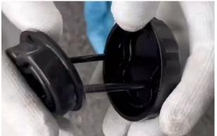
d. Use the brake fluid moisture content tester to measure the water content, if it is > 2%, all brake fluid needs to be replaced; If 2% is  $\leq$ , add freshly opened DOT 4 brake fluid to 3/4 of the clear viewing window of the front disc brake main cylinder. It is recommended that the water content should be less than 1.5%. TOTAL Total HBF 4 (DOT 4) brake fluid 0.22L (0.23 US qt, 0.19 Imp qt, 0.06 US gal, 0.05 Imp gal).
