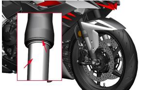
b. Check whether the bottom cylinder is peeling off the paint; Signs of whether the mounting points of the front fenders, front wheel hollow shaft and front brake calipers are broken or cracked. Check the bottom of the bottom barrel for leaks.
