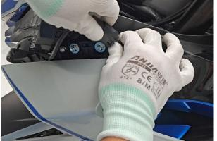
i. Use the 8# T-type sleeve to remove 1 M6×16 bolt (1), 2 M6×22 bolts (2), and remove the left headlight (3).
