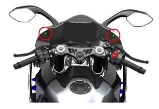
b. Use a crochet hook to remove one expansion nail from each of the left and right envelopes the interior (1).
