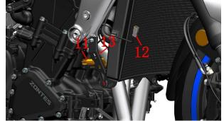
d. Use an 8# socket wrench to remove the M6×12 bolt (7) securing the right lower bracket (13) of the main radiator, and then take out the right lower bracket (13). Use an 8# socket wrench to remove the one M6×22 bolt (1) securing the main radiator. Use a hose clamp pliers to move the  $\varphi$ 32 hose clamp (10) and  $\varphi$ 9 hose clamp (14) to a suitable position, then disconnect the water pipes, and finally remove the main radiator assembly.
