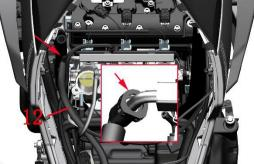
g. Install the high-pressure tubing (12) back according to the above steps.
