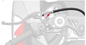
c. If the fault of high resistance cannot be solved after lubrication, the throttle cable needs to be replaced.
