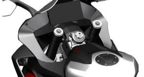
b. For the sake of illustration, other components are hidden here. Move the washer (1) up first, and then loosen the adjusting nut (2a).
