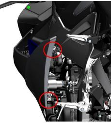
h. On the left side of the vehicle, carefully pull the buckle or mushroom peg indicated by the arrow from top to bottom, and remove the left bracket panel assembly.
