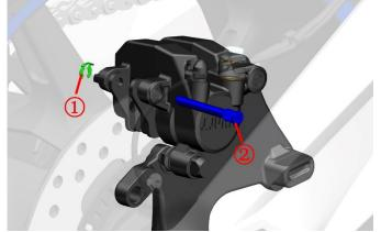
b. With the help of a tool, push the piston in the direction of the arrow to the end. If the resistance is very large, you can refer to the method of adding brake fluid to the front brake main cylinder, remove the upper cover and then push it. If the spring blade on the caliper falls off, it needs to be replaced in the direction shown.
