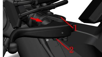
a. Remove the nut by turning it counterclockwise with a 10# torx wrench(2).
