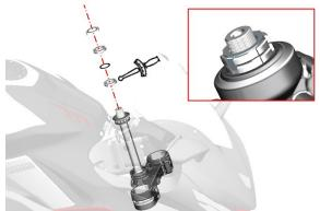
d. After the upper plate assembly is installed, the nut (5) is tightened with the decorative nut tooling, and the torque: 100N.m. Use a T45 torx wrench with holes to tighten the bolt
