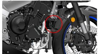
c. Use the 8# sleeve to remove 2 pieces of M6×22 bolts (9) and 1 piece of M6×30 bolt (10) that fix the oil cooler.
