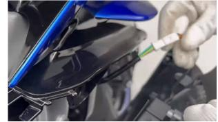
g. Use a T25 Allen Torx wrench to remove the 2 bolts of the M6×12.
