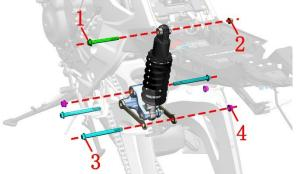
b.One person uses a 14# sleeve to fix the head of the bolt, and one person uses a 14# sleeve to remove the nut, remove the bolt, and remove the rear shock absorber and triangle bar assembly. Nut torque: 65±5N.m (6.6±0.5 kgf.m, 48±4 lbf.ft)
