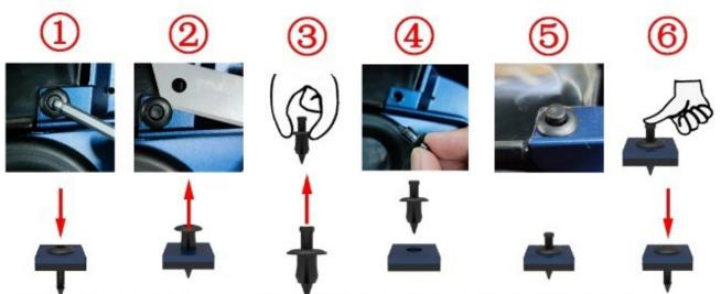
(1) Press the center cylinder with 4# hexagon or other tools, you can hear a sound or the center cylinder moves axially by 2mm (0.079 in);
