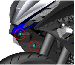
b. Carefully pull the buckle or mushroom staple at the point indicated by the arrow and remove the upper assembly of the right surround.
