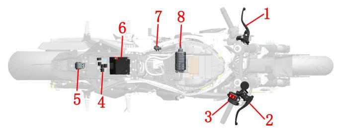
1-Clutch rocker arm (clutch switch) 2-Front disc brake main cylinder (front brake switch) 3-Right hand handle switch 4- Fuse box 5- Starter relay 6-Battery 7- Side bracket power out switch 8- Starter motor
