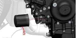
b. Drain the oil from the filter.
