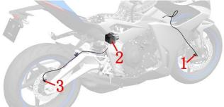
1-Front wheel speed sensor 2-ABS hydraulic control unit 3-Rear wheel speed sensor
