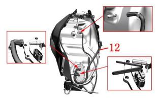
f. Refer to the steps in "Replacing the Spark Plug" to remove the entire air filter. Press and hold the tubing buckle to pull out the high-pressure tubing (12).
