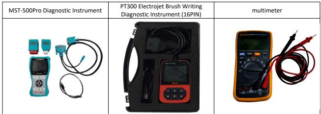
•Both of the above diagnostic instruments can read fault codes; The PT300 diagnostic device can be flashed into the program.
