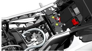
b. Then find the ventilation tube (2) of the carbon canister from the solenoid valve of the canister and pull it out, and take out the canister.
