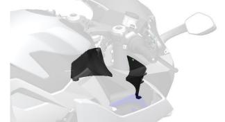
e. After removing the interior surrounding, remove the joints of the left and right mirrors from the interior panels.
