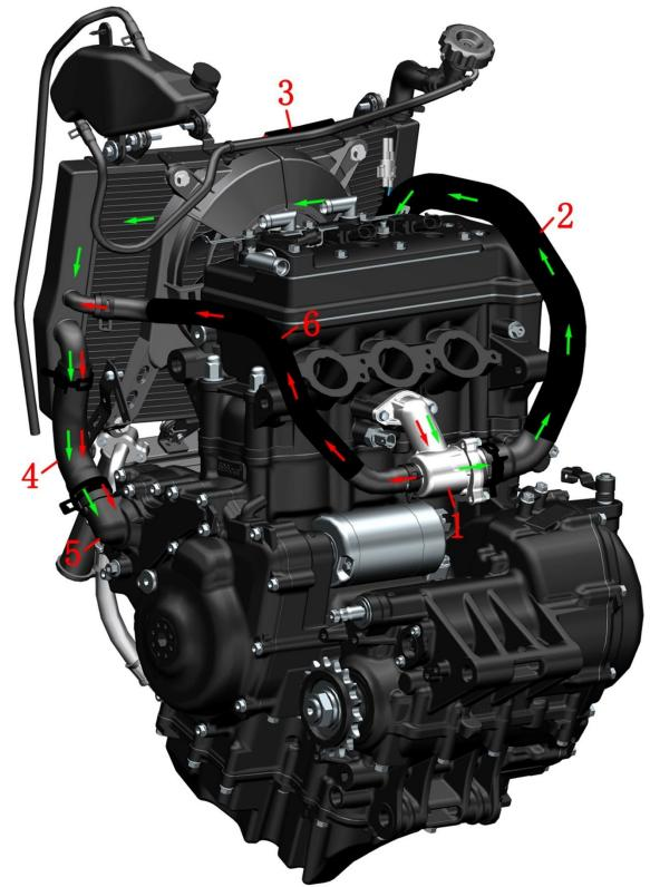
1-Thermostat assembly 2-Main water tank inlet pipe 3-Main water tank 4-Engine water inlet pipe 5-Water pump cover assembly 6-Small circulation water pipe
