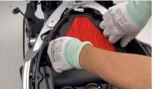
c.After changing the air filter, install the upper shell of the air filter back, and check the wiring harness, and use the cross batch to install 10 self-tapping nails (1) back and fix.
