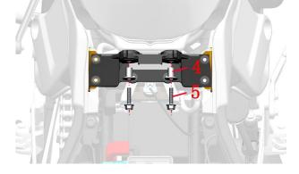
b. Use a T25 torx wrench to remove 2 M6  $\times$  14 shaft shoulder bolts (6).
