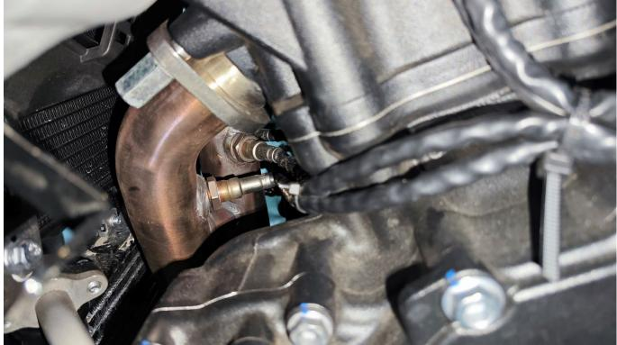
The new sensor threads are coated with a special paste thread anti-sintering agent to prevent air leakage and facilitate subsequent re-disassembly. If the old inspection is fine, it is necessary to apply an appropriate amount of anti-sintering agent to the thread before installation. Torque standard: 18±1.5N.m.
