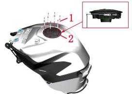
c. Break the buckle (1) first, then break the 2 mushroom buckles (2), and then pull in the direction of the arrow to remove the left decorative cover (3).
