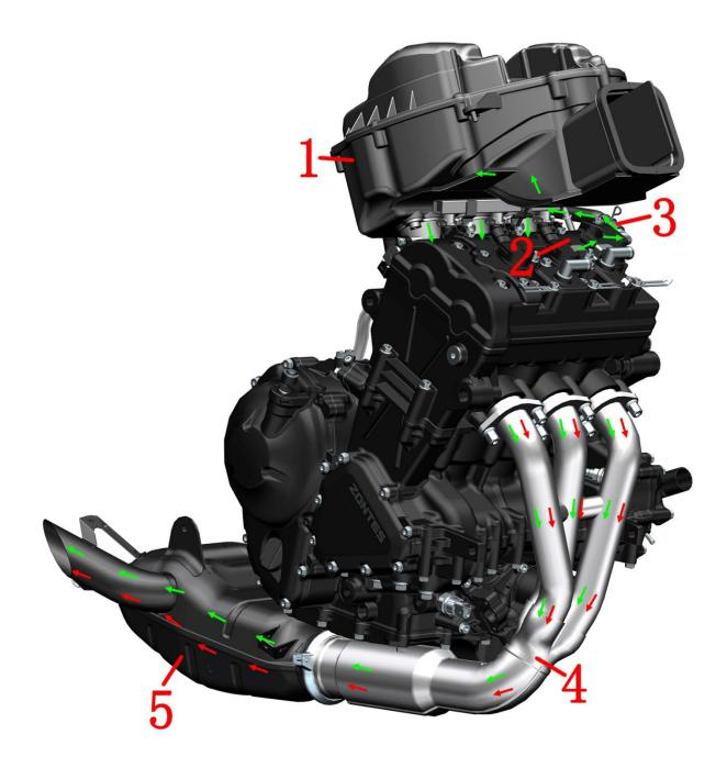
1-Air filter assembly 2-Cylinder head 3-Exhaust gas snorkel 4-Front muffler 5-Rear muffler Exhaust system: The main exhaust gas emission flow direction Cylinder heads→ front mufflers→ rear mufflers
