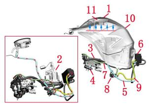
1-Fuel Tank Lock 2-Fuel Pump 3-High Pressure Oil Hose 4-Throttle Valve Body Assembly 5-Adsorption/Snorkel 6-Carbon Canister 7-Solenoid Valve Out 6 Air Hose 8-Carbon Canister Solenoid Valve 9-Solenoid Valve Intake Pipe 10-Fuel Tank 11-Air-Oil Separator (Inside Tank Lock)
