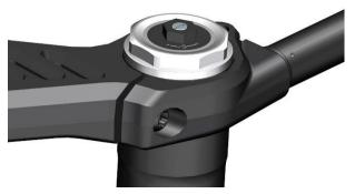
c. Attach the two M8×35 bolts to the lower plate and insert the other shock absorber in the same way.
