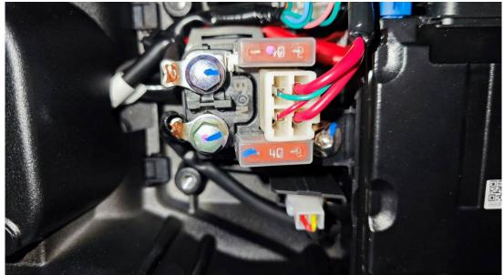
When reinstalling the relay, the red wire is installed on the threaded hole of the relay marked "B", and the black wire is installed on the threaded hole of the relay marked "M". Make sure the protective cap is closed after the screws are tightened, and then plug in the relay connector.
