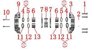
1-Bolt 2-Circlip 3-Caliper inner housing 4- $\phi$ 30 oil seal 5- $\phi$ 30 dust seal 6- $\phi$ 30 piston 7-brake pad 8-brake pad spring 9caliper outer housing 10-pin 11- $\phi$ 34 oil seal 12- $\phi$ 34 dust seal 13- $\phi$ 34 piston
