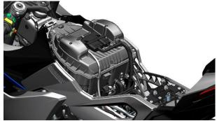
b. Refer to "Removal of Air Filter" to remove the upper cover of the air filter. And put the wiring harness in order.
