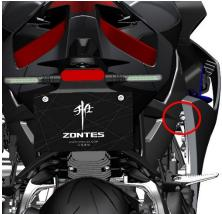
e. On the right side of the vehicle, carefully pull the buckle or mushroom staple indicated by the arrow from top to bottom, and remove the right bracket panel assembly.
