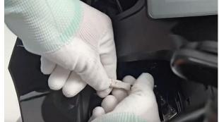
f. Use an 8# torx wrench to remove the two M6×12 hexagonal bolts (1) to remove the rearview mirror, pay attention to the rearview mirror before removing the bolt to stabilize the rearview mirror to prevent it from falling. The method of removing the left and right mirrors is the same.
