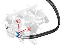
If neither of these adjustments is effective, a new throttle cable will need to be replaced.
