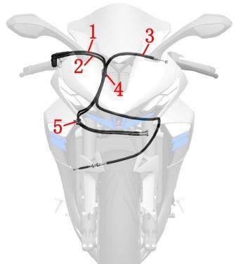
1-Refueling line, 2-Oil return line, 3-Clutch line, 4-Throttle line, limit bracket, 5-Throttle cord clamp
