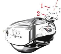
When reassembling, it is necessary to pre-tighten diagonally and then tighten 9 bolts (1), otherwise the sealing rubber ring of the fuel pump (2) is compressed unevenly, which will easily lead to leakage and cause potential safety hazards.
