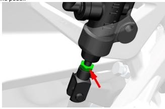
Big adjustment: Loosen the bolt on the brake pedal, adjust the brake pedal to the angle that the driver is comfortable with, and then tighten the bolt.
