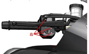
b. Use a Phillips screwdriver to remove the three bolts securing the rear cover of the left handlebar switch, and then take off the rear part of the left handlebar switch. Disconnect the heater harness connector and remove the bolt securing the front part to detach the front of the switch.
