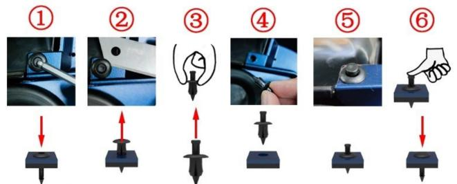
(1) Press the center cylinder with 4# hexagon or other tools, you can hear a sound or the center cylinder moves axially by 2mm;
