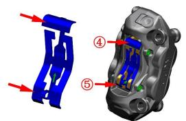
J. hold down the piece at the point of the arrow (4) to the direction of the arrow with the hand, and insert the pin (2) into the hole position to fix the brake pad (1). Tighten the pin (2) with a T25 hexagon torx wrench.
