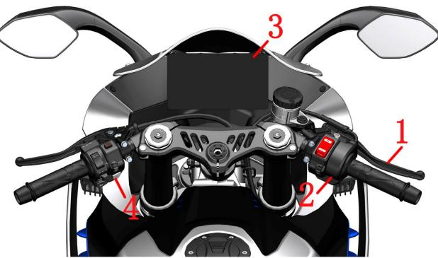
1.Front brake handle 2.Right hand handle switch 3.Meter 4.Left hand handle switch a. Park the motorcycle on flat ground or on a lifting platform, lower the main bracket and retract the side brackets. b. The function of the right-hand handle switch is shown in the figure below
