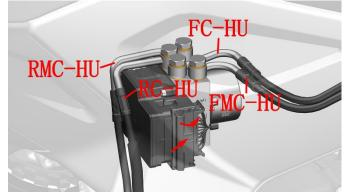
FMC-HU: Front disc brake main pump - hydraulic control unit
