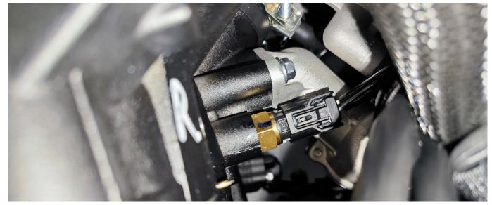
The two-pin resistance value of the multimeter at room temperature is: 3.74~1.22kΩ(10~40°C);1.22~0.27kΩ(40~90°C). Due to limited space, it is recommended to use a 72-tooth 17# ratchet torx wrench counterclockwise to remove the water and oil common sensor and remove the 9×2 EPDM O-ring. When reassembling, replace the O-ring with a new one to avoid leakage.
