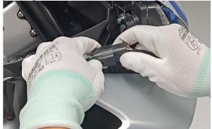
k. Use the 8# T-type sleeve to remove 1 M6×16 bolt (1), 2 M6×22 bolts (2), and remove the right headlight (4).
