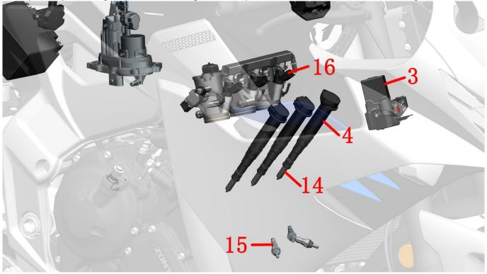
14-spark plug 15-oxygen sensor 16-fuel injector
