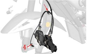
e. Move the front mud board up to the appropriate part and pull it out and remove it in the direction of the big arrow.
