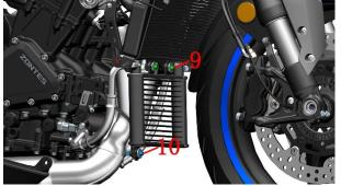
d. Use the 8# sleeve to remove the 4 bolts on the engine inlet and outlet pipes (11); Remove the oil cooler from the vehicle. Then adjust the inlet and outlet pipes to the appropriate position. Note: A small amount of oil may drip when the oil cooler is removed; When installing, please pay attention to whether the O-ring on the inlet and outlet pipes is damaged, and replace it immediately if there is a cut edge or damage.
