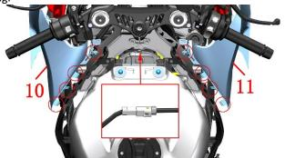
e. Grab the head of the fuel tank and lift the fuel tank, use the vise to loosen the exhaust pipe buckle, pull out the exhaust pipe, and then pull out the high-pressure oil pipe (12) and the power cord of the oil pump, and then remove the fuel tank.
