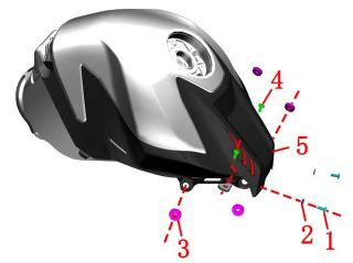
b. Use a Phillips screwdriver to remove the 4 non-standard Phillips self-tapping screws (1) fixed on the inner lining of the fuel tank interior cover, and remove the left and right decorative cover liners (2), and then remove the fuel tank middle cover (3).
