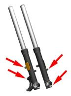
c. If there is a large amount of hydraulic oil attached to the front fork tube, wipe it clean and observe after riding. If there is no oil stain or slight oil stain, it is the hydraulic oil
