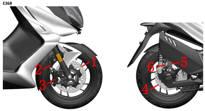
1-Front brake disc components 2-Wheel speed sensor (Font Wheel) 3-front disc brake caliper 4-Rear brake disc components 5- Rear disc brake caliper 6- Wheel speed sensor (rear wheel)
