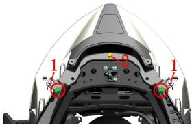
e. Remove the 2 expansion nails on the left and right sides connecting the rear fender and the rear skirt bottom plate.
