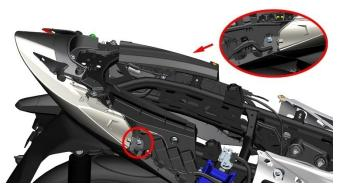
d. Buckle down the two expansion nails as shown in the picture, use a 10# sleeve to remove the two M6×16 bolts on the left and right sides of the fixed taillight(1), and use a 10# sleeve to remove one M8× bolt that fixes the rear light 30 bolts (2).
