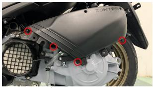
d. Remove the air filter housing.
