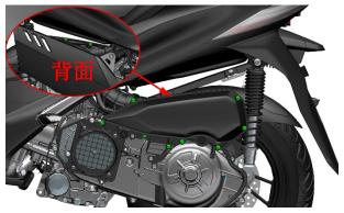
b. Remove the air filter housing.
