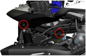
f. Unplug the wire harness connector on the left side of the rear of the motorcycle, arrange the wire harness and remove the rear fender assembly of the taillight.
