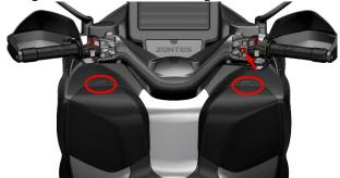
b. Use 4# inner hexagon to remove 2 pieces of M6×14, then you can take off the panel assembly of the storage box,
