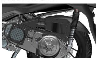
c. Replace the new filter element and sealing strip.
