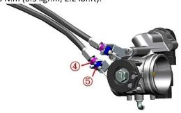
c. If the above two adjustments are invalid, replace the throttle cable with a new one.
