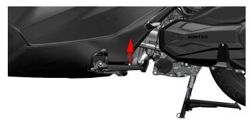
c. Check whether the flameout switch function is normal. The vehicle should not be started when the side bracket is lowered (parking position); the vehicle cannot be started when the side bracket is retracted (driving position) without pinching the front or rear brake handle; After starting the vehicle, put down the side brackets, and the flame should be automatically turned off, otherwise it is necessary to troubleshoot the flameout switch or brake switch failure.
