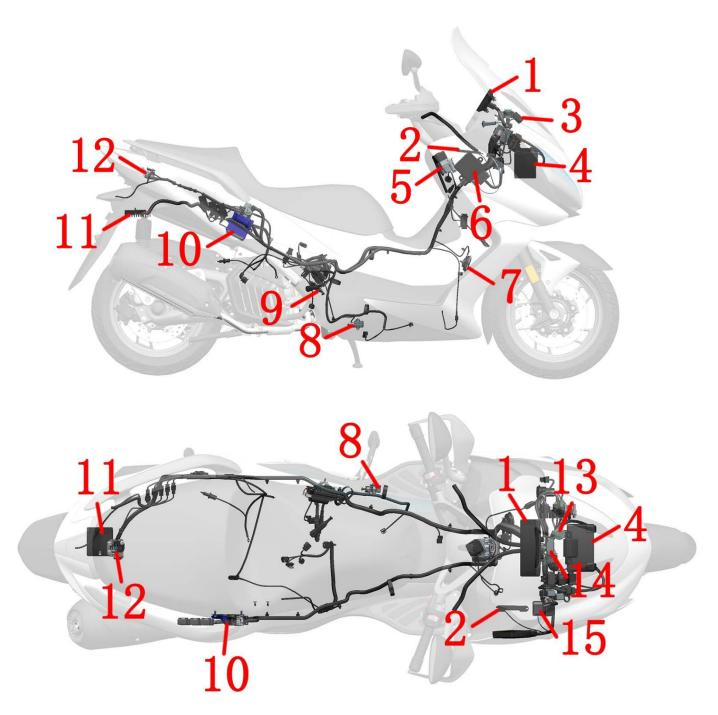
1-TFT Meter 2-Non-inductive antenna 3-Windshield motor controller 4-Battery 5-Main lock 6-PKE 7-Horn 8-Side bracket flame-out switch 9-Carbon canister solenoid valve 10-Engine controller (ECU) 11-Rectifier 12-Seat lock 13-Flash 14-Dump switch 15- GPS antenna
