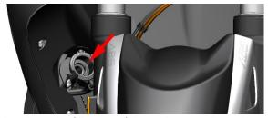
d. Tighten the filler cap of the Radiator. Tighten the exhaust bolt; torque:  $8\sim$ 10N.m (0.8 $\sim$ 1 kgf.m,  $6\sim$ 7 lbf.ft).
