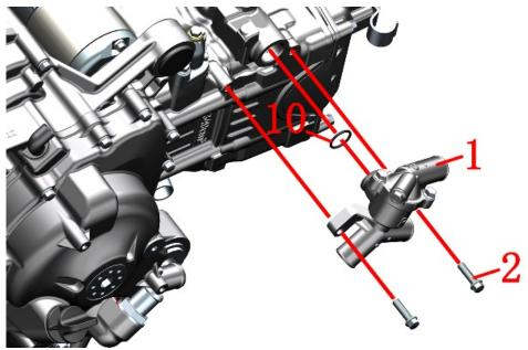
Before reassembly, the joint surface should be cleaned. Note that the O-ring cannot be missing and must be correctly assembled in place. The hoop should be clamped inside the boss to prevent loosening. Bolt(2) Torque: 12±1.5 N.m (1.2±0.2 kgf.m, 9±1 lbf.ft).
