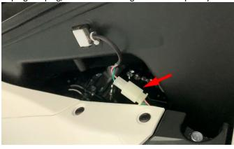
d. Unplug the plug of the stepping motor  $\bigcirc$  and the sensor  $\bigcirc$
