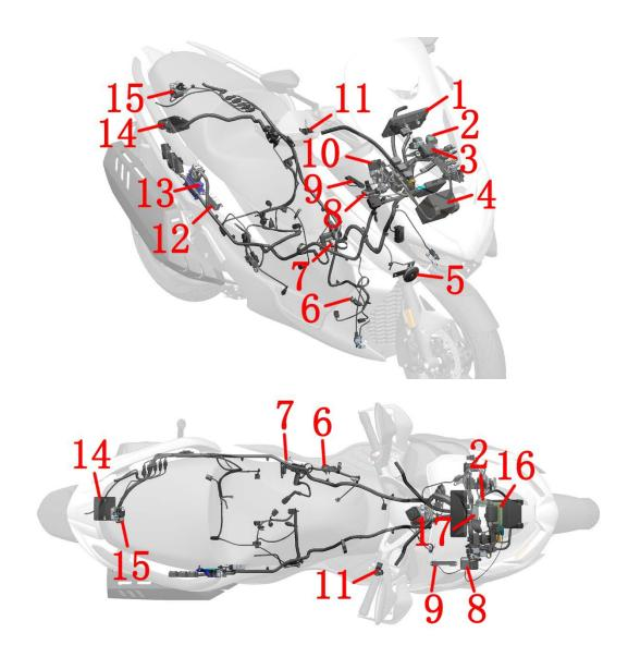
1-TFT instrument 2-Flasher 3-Windshield motor controller 4-Battery 5-Horn 6-Side bracket flame-out switch 7-Carbon canister solenoid valve 8-GPS antenna 9-Non-inductive antenna 10-Main lock 11-Electric Heat Handle bar Switch 12-Tire pressure receiving host 13-Engine controller (ECU) 14-Rectifier 15-Seat lock 16-PKE 17-Dump switch
