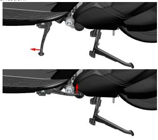
c. Check whether the flameout switch function is normal. The vehicle should not be started when the side bracket is lowered (parking position); the vehicle cannot be started when the side bracket is retracted (driving position) without pinching the front or rear brake handle; After starting the vehicle, put down the side brackets, and the flame should be automatically turned off, otherwise it is necessary to troubleshoot the flameout switch or brake switch failure.
