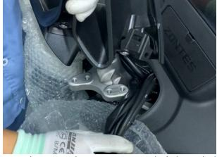
g. Use the 4# inner hexagon to remove the bolts on the left and right storage box brackets.
