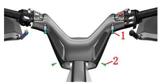
c. Use 6# inner hexagon to remove the left and right handles and switch components.
