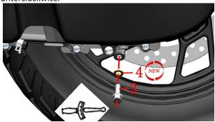
c. Remove the oil  $\alpha$ .  $\mathfrak{solt}(3)$  and the copper pad(4).
