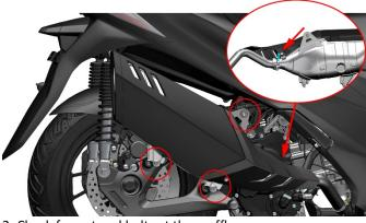
Check for nut and bolts at the muffler
