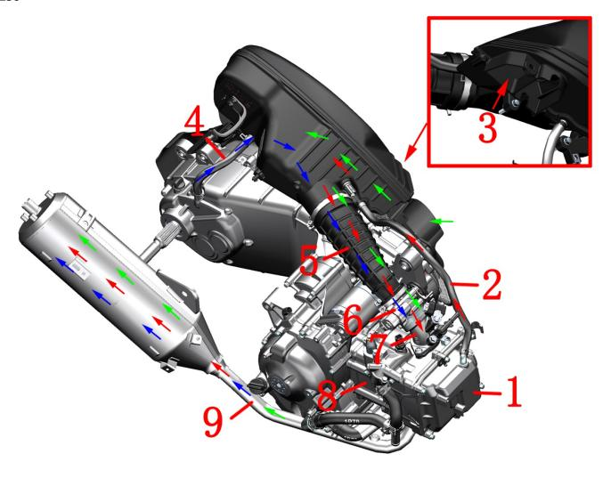
1- Cylinder head 2-Cylinder head exhaust pipe3- Air filter intake inlet 4-Crankshaft Box exhaust pipe5-Air filter outlet pipe6-Throttle valve body assembly 7-Intake manifold8- Cylinder 9- Muffler
