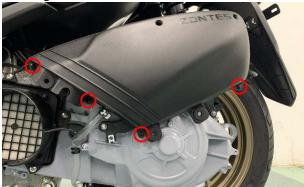
d. Remove the air filter housing.
