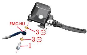
e.Remove the upper cover according to the steps of adding brake fluid, and remove the brake switch and brake handle according to the steps of removing the brake switch and brake handle.
