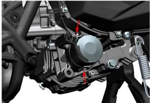
b. Place an oil pan under the fine filter cover.Remove the fine filter using a 14-side, 65mm cap filter wrench +1/2" (12.5mm) ratchet wrench counterclockwise. The filter wrench has a Skadden model 97401. Replacement every 1,000 km or 3 months (whichever comes first) and every 8,000 km or 30 months (whichever comes first).
