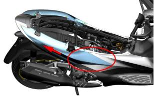
c. Disassemble and assemble the left and right rear skirt components in the same way.
