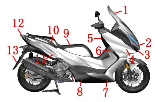
1. Windshield 2. Headlights 3. Lower part of the hood 4. Right panel of the hood 5. Front right panel 6. Right side cover 7. Right pedal decorative cover 8. Lower deflector right 9. Seat 10. Right rear armrest 11. Right part of tail skirt 12. Rear tail light 13. Rear fender
