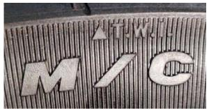
b. The height of the wear mark on the tread protrusion is 1.6mm (0.06 in). The triangle ( $\triangle$ T.W.I.) mark on the sidewall indicates the location of the wear bar. If the wear reaches the mark point, it means that it has been worn to the limit. If you continue to drive, there will be a safety hazard. You must replace with new tires of the same specification.
