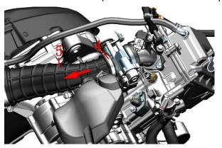
e. Use 5# inner hexagon to remove 2 bolts(6) and then remove the valve body assembly from the engine.
