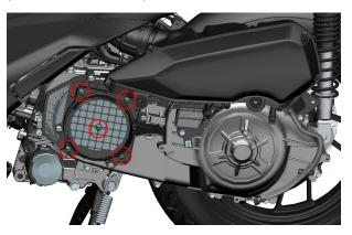
b. Remove the sponge and replace it with a new filter element. Note that the black side faces the engine and the white side faces outward.
