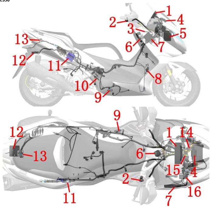
1-TFT Meter 2-Electric Heat Handle bar Switch 3-Non-inductive antenna 4-Windshield motor controller 5-Battery 6-Main lock 7-PKE 8-Horn 9-Side bracket flame-out switch 10-Carbon canister solenoid valve 11-Engine controller (ECU) 12-Rectifier 13-Seat lock 14-Flash 15-Dump switch 16- GPS antenna
