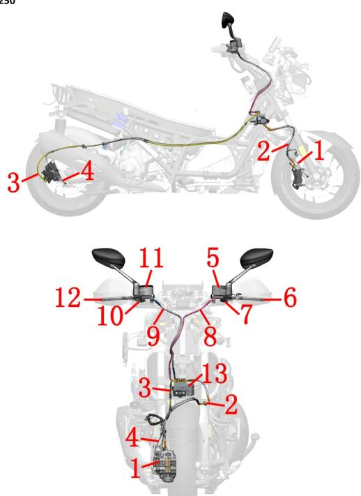
1-Wheel speed sensor (front wheel) 2-FC-HU brake hose 3-RC-HU brake hose 4-Wheel speed sensor (rear wheel) 5- Rear disc brake main pump 6-Rear brake lever 7-Rear brake switch 8- RMC -HU brake hose 9-FMC-HU brake hose 10-Front brake switch 11-Front disc brake main pump 12-Front brake handle 13-Hydraulic control unit
