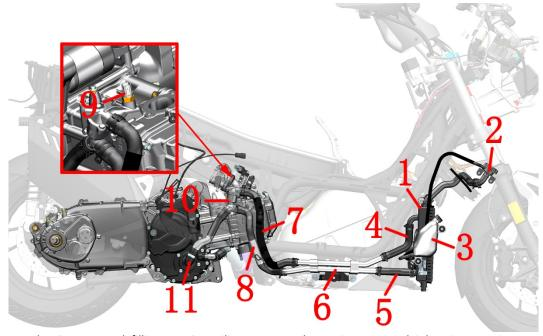
1-Main water tank 2-Water tank filling port 3-Auxiliary water tank 4-Main water tank inlet pipe 5-Main water tank outlet pipe 6-Aluminum water pipe 7-Thermostat outlet pipe 8-Engine inlet pipe 9-Water and oil common sensor 10-Thermostat 11-Water pump cover assembly
