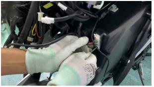
j. Use 4# inner hexagon to remove 2 M6×14 bolts (2), use 6# inner hexagon to remove 2 M6×25 bolts (1) to fix the main lock, and pull out the main lock connector.
