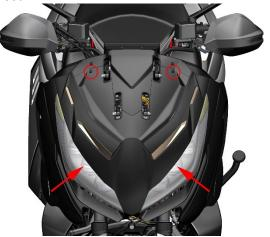
b. Lower the windshield to a low position, use 4# inner hexagon to remove the 2 front bolts, the 2 expansion bolts on the left and right sides of the rear, and the 2 left and right expansion nails on the inner side, and remove the rear of the windshield liner.
