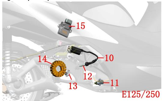
1 - Dump switch 2 - PKE 3 - relay 4 - main lock 5 - right handle bar auxiliary switch 6 - right handle bar switch 7 - battery 8 - fuse box 9 - start relay 10 - ignition coil 11 - side bracket flameout switch 12 - spark plug 13 - crankshaft position sensor 14 - magneto stator 15 - ECU
