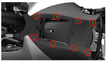
d. Lift out the pedal rubber pad and the pedal rubber pad pressure plate using a one-word batch, press and pull up the pedal rubber pad and the pedal rubber pad pressure plate until the pedal rubber pad and the rear pedal rubber pad pressure plate are taken out. Disassemble the left and right sides in the same way.
