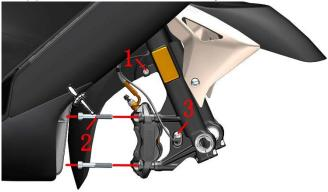
c. Use the 4# Allen to remove the 2 M6 $\times$ 14 shaft shoulder bolts (4) on the left and right sides of the front clay plate; Then use the 5# Allen to remove 1 M6 $\times$ 30 bolt (1) and remove the bullet pad (5).
