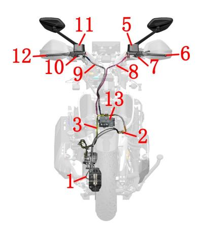
1-Wheel speed sensor (front wheel) 2-FC-HU brake hosepipe 3-RC-HU brake hosepipe 4-Wheel speed sensor (rear wheel) 5-Rear disc brake main pump 6-Rear brake handle 7-Rear brake switch 8-RMC-HU brake hosepipe 9-FMC-HU brake hosepipe 10-Front brake switch 11-Front disc brake main pump 12-Front brake handle 13-Hydraulic control unit
