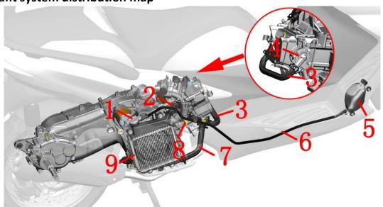
1- water tank water inlet 2-main water tank inlet pipe 3-engine inlet pipe.4-Water pump cover inlet pipe 5-Secondary water tank 6- auxiliary water tank connection water pipe 7- water tank outlet pipe 8-Water and oil shared sensor 9-Main water tank
