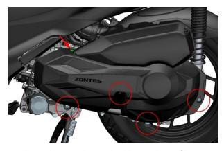
c. Pull out the 2 mushroom buckles on the air filter decoration cover and remove the air filter decoration cover.
