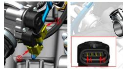
c. Use a short Phillips screwdriver to remove the 2 GB9074.4 M5×16 bolts (3) that comes with the throttle valve body assembly, and then remove the the anti-off card (4), and then take off the stepper motor. It is forbidden to soak the sensor with any liquid.
