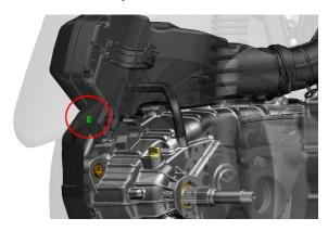
b. Use a T30 torx wrench to remove the 4 hexagonal small flanges M6×16 torx bolts shown in the figure.
