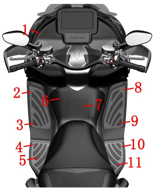
1. Instrument panel 2. Front left pedal rubber pad pressure plate 3. Front left pedal rubber pad 4. Rear left pedal rubber pad pressure plate 5. Rear left pedal rubber pad 6. Fuel tank decorative cover 7. Fuel tank cover 8. Front right pedal rubber pad pressure plate 9. Front right pedal rubber pad 10. Rear right pedal rubber pad pressure plate
