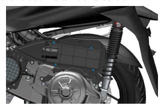
b. Remove the old air filter element. Blow the dust inside the air inlet pipe with a dust blower, and then wipe the inner wall with a clean non-woven cloth.
