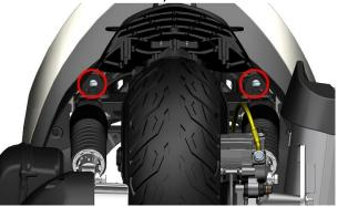
c. Use a 4# inner hexagon to remove the two M6 $\times$ 14 bolts on the left and right sides of the motorcycle that fix the taillights.
