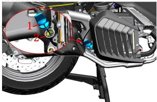
d. After placing an oil pan under the oil drain bolt, use a 14# sleeve to remove the oil drain bolt(3) and the combined seal gasket(4). Use a 24# sleeve to remove the strainer cover (5) at the bottom, take off the 34.5×3.5 acrylate rubber Oring(6), the  $\varphi$ 25.8×34.2×1.8 strainer spring(7) and the outer diameter  $\varphi$ 22×21 cap-shaped strainer(8). Drain the oil from the crankcase.
