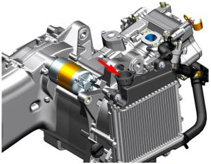
e. Tighten the filler cap of the Radiator. Tighten the exhaust bolt; torque:  $8\sim$ 10N.m (0.8 $\sim$ 1 kgf.m,  $6\sim$ 7 lbf.ft).
