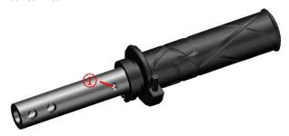
c. When installing the secondary handle bar switch, it is necessary to align the joint surface of the counter-handle bar switch and the main pump of the disc brake with the triangle mark on the handle bar switch, and then use 5# hexagon to tighten  $4 \text{ M6}{\times}30$  bolts.
