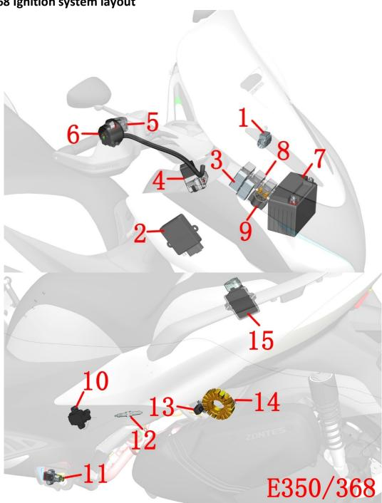
1 - Dump switch 2 - PKE 3 - relay 4 - main lock 5 - right handle bar auxiliary switch 6 - right handle bar switch 7 - battery 8 - fuse box 9 - start relay 10 - ignition coil 11 - side bracket flameout switch 12 - spark plug 13 - crankshaft position sensor 14 - magneto stator 15 - ECU
