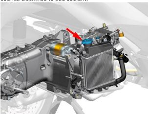
c. Use a 10# sleeve to loosen the thermostat bleed bolt (2) counterclockwise by 4 to 5 turns, do not completely remove it. Note that a small container is required to receive the coolant overflowing from the exhaust bolt. Do not allow the coolant to drip directly onto the surface of the part.
