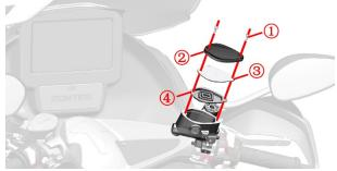
e. Use the brake fluid water content tester to measure the water content, if it is more than 2%, all brake fluid needs to be replaced; if it is less than or equal to 2%, add newly opened DOT 4 brake fluid to the transparent observation window of the front disc brake main pump 3/4 places. It is recommended that the water content should be less than 1.5%. Total 0.23L(0.24 US qt,0.2 lmp qt,0.06 US gal ,0.05 lmp gal ) TOTAL HBF 4 (DOT 4) brake fluid is added to this vehicle from the factory.
