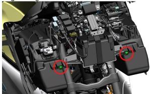
k. Remove the 4 expansion nails on the left and right sides that fix the panels of the front storage box.
