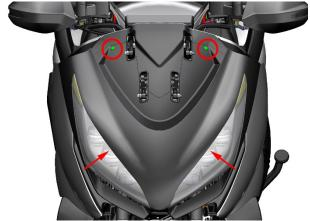
b. Lower the windshield to a low position, use 4# inner hexagon to remove the 2 front bolts, the 2 expansion bolts on the left and right sides of the rear, and the 2 left and right
