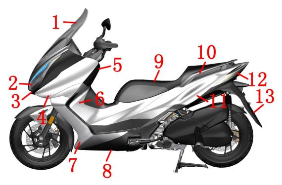
Windshield 2. Headlights 3. Lower part of the hood 4. Left plate of the hood 5. Front left panel 6. Left side cover 7. Left pedal decorative cover 8. Lower fairing left 9. Seat 10. Left rear armrest 11. Left part of the tail skirt
