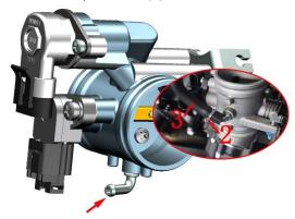
d. Loosen the bolt of the  $\mathsf{clamp}(4)$  with a 4# inner hexagon and pull out the air filter outlet  $\mathsf{pipe}(5)$  and  $\mathsf{clamp}(4)$  in the direction of the arrow to pull out the throttle valve body.
