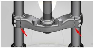
b. Use a batch to pry open a gap on the upper plate, put in the corresponding shock absorber, install the shock absorption in place, and remove the next word batch. Screw in the bolt (6) of M8×35 and tighten using the 6# Allen. Torque: 25N.m (2.6 kgf.m, 18 lbf.ft).
