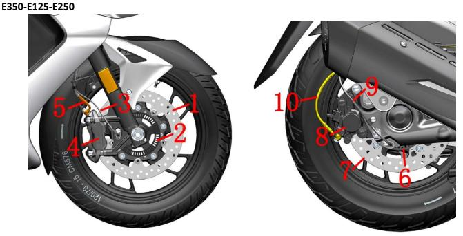
1-brake disc (front) 2- front whell ABS induction ring gear 3-wheel speed sensor (front wheel) 4-front disc brake caliper 5-FC-HU brake hose 6- rear whell ABS induction ring gear 7-brake disc (rear) 8-rear disc brake caliper 9-wheel speed sensor (rear wheel) 10-RC-HU brake hose
