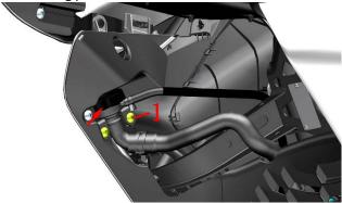
b. Use a 10# sleeve to loosen the thermostat bleed bolt (2) counterclockwise by 4 to 5 turns, do not completely remove it. Note that a small container is required to receive the coolant overflowing from the exhaust bolt. Do not allow the coolant to drip directly onto the surface of the part.
