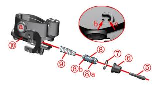
(5) Piston push rod (6) dust cap (7) retainer ring (8) piston assembly (8) a outer seal ring (8) b inner seal ring) (9) spring (10) main pump housing
