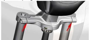
c. Install the bolts (6) of the two M8×35 lower plates and use the same method to load another shock absorber.
