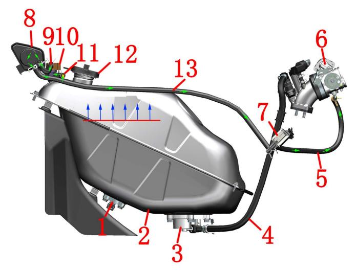
1-Oil level sensor 2-Fuel tank 3-Built-in fuel pump 4-High pressure oil pipe 5-Carbon canister solenoid valve outlet pipe 6-Throttle valve body assembly 7-Canister solenoid valve 8-Carbon tank 9-Carbon canister adsorption tube 10-External oil and gas separator 11- Fuel tank breather pipe 12- Fuel tank cover 13-Carbon canister solenoid valve intake pipe
