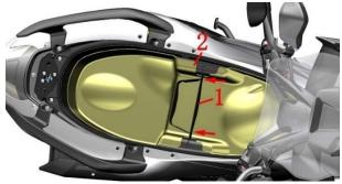
b. Old model: Use 4# inner hexagon to remove the 4 shoulder bolts at the rear and the middle (1), remove the front hexagonal bolt decorative buckle (2) and then remove the bolts (1).
