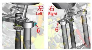
c. Use 6# hexagon to remove the 4 bolts (6) of M8×35, pry open the gap on the lower coupling with a batch of words, and remove the left front shock absorption and right front shock absorption.
