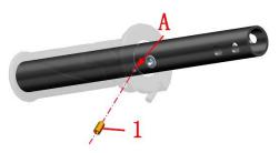
b. When installing the left hand handle switch, it is necessary to align the bolt (a) with the positioning hole 1 on the directional handle, and then tighten it with a cross batch. When installing the right-hand handle bar, align the mounting hole of the heating switch with the positioning hole 1 on the directional handle, and then tighten the bolt 2 with a cross batch. Use the 5# Allen to tighten the bolts (b), (c), (e), and (f) that hold the left and right handle switches in turn.
