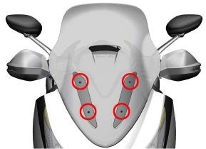
b. Use the 4# inner hexagon to loosen the 4 M6×14 shoulder bolts on the left and right decorative covers of the windshield.
