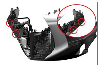
c. Press and pull out the 8 expansion nails at the bottom of the fairing, and remove the bottom of the lower fairing.
