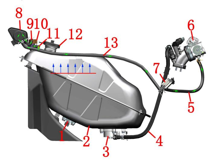
1-Oil level sensor 2-Fuel tanks 3-Fuel pump 4-High-pressure tubing 5-Solenoid valve outlet pipe 6-Throttle body assembly 7-Canister solenoid valve 8-Carbon canisters 9-Carbon canister adsorption tube 10-External oil and gas separator 11-Fuel tank snorkel 12-Fuel tank cap 13-Solenoid valve intake pipe
