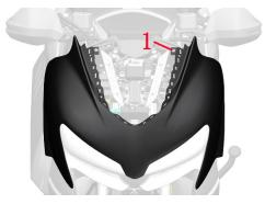
b.Use a cross batch to remove the 2 expansion nails (2) on the lid in the front panel.
