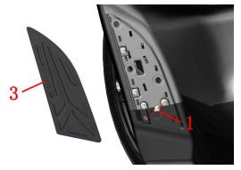
d.Take out the decorative cover (4) after breaking out the buckle of the decorative cover of the left pedal. The disassembly method of the left and right pedal decorative covers is the same, and the right decorative cover is disassembled with reference to the above steps.
