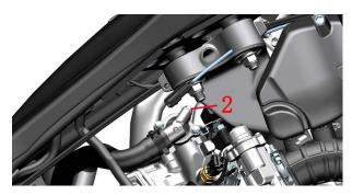
c.Wear waterproof gloves and use the extended funnel to add coolant to the main tank inlet. The coolant level is visible at the water inlet until the coolant is spilled at the stable position of the thermostat bleed bolt.
