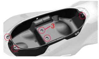
c.Lift the rear of the locker slightly until the wiring connector on the left side of the locker is exposed, unplug the
