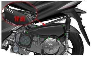
b.Remove the air filter housing.
