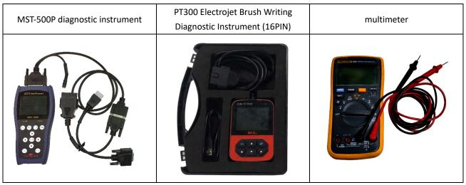
•Both of the above diagnostic instruments can read fault codes; The PT300 diagnostic device can be flashed into the program.
