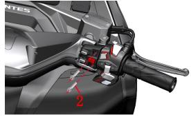
d.Tilt the front brake main cylinder so that the bolt (1) is facing up, remove the bolt (1) with a 12# sleeve after wearing waterproof gloves, remove the copper pad (3) and remove the FMC-HU oil pipe, and pour out the brake fluid in the main cylinder. Bolt (1) Standard torque: 32N.m (3.3 kgf.m, 24 lbf.ft).
