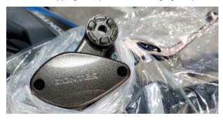
d.After wearing waterproof gloves, remove the bolt (1) with a Phillips screwdriver, and remove the upper cover (2), cover plate (3), and sealant gasket (4).
