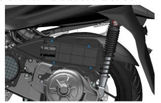
b.Remove the old air filter cartridge. Use a dust gun to blow the dust on the inside of the air intake pipe, and then wipe the
