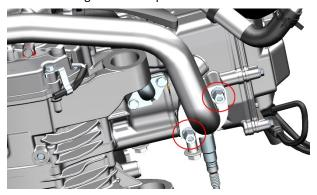
a.If there is a slight air leakage, you can try to tighten the exhaust nut with 6# hexagon socket first; If the problem is not solved, the muffler needs to be removed and replaced with a new engine row air port gaskets.
