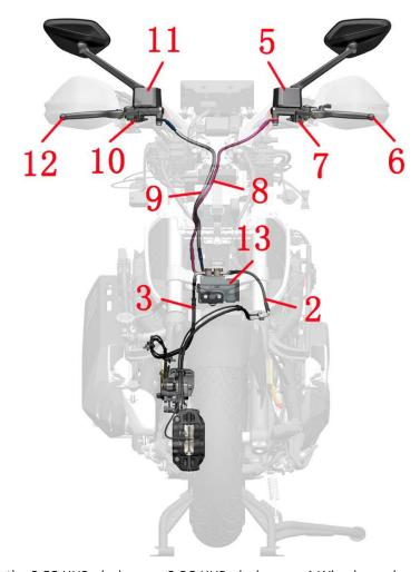
1-Wheel speed sensor (front) 2-FC-HUBrake hoses 3-RC-HUBrake hoses 4-Wheel speed sensor (rear) 5-Rear disc brake main pump 6-Rear brake handle 7-Rear brake switch 8-RMC-HU Brake hoses 9-FMC-HU Brake hoses 10-Front brake switch 11-Front disc brake main pump 12-Front brake handle 13-Hydraulic control unit
