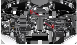
d.Use the cross batch to remove the 4 bolts (16), remove the briquetting (15), the left rocker arm (10), the right rocker arm (11), the buffer glue (14), the motor (12) and the sheath (13).
