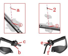
c.When installing the off-hand handlebar switch, you need to align the combination of the off-hand switch with the disc brake main cylinder to align the triangle logo on the handlebar switch, and then use the 5# hexagon socket to tighten 4 M6×30 bolts.
