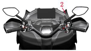
c.Turn on the motorcycle and open the left and right locks. Use a T25 Allen Torx wrench to remove the bolts (1) of the 2 M6×14 shaft shoulders as shown in the figure, and remove the front panel.
