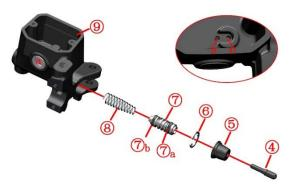
4) Piston pushrods 5) Dust cap 6) Retaining rings 7) Piston assembly (7) a Outer seal 7) b Inner seals ) 8) Spring 9) Main pump housing
