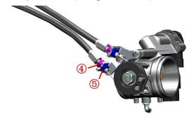
c.If neither of these adjustments is effective, a new throttle cable will need to be replaced.
