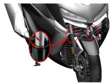
b.Check whether the bottom cylinder is peeling off the paint; Signs of whether the mounting points of the front fenders, front wheel hollow shaft and front brake calipers are broken or cracked. Check the bottom of the bottom barrel for leaks.
