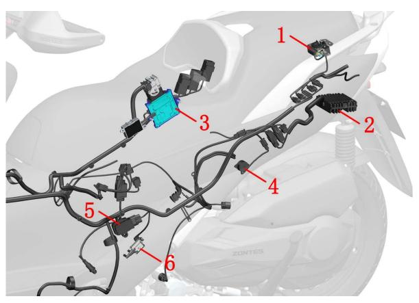
1-Cushion lock 2-rectifier 3-Engine controller (ECU) 4-buzzer 5-Ignition coil body 6-Canister solenoid valve 24 / 135
