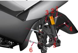
c.Use the 5# hexagon socket to remove 1 M6 $\times$ 30 bolt (1) and remove the spacer (2). Use a T45 Torx Allen wrench to remove the shoulder bolt (4) of one M6 $\times$ 14.
