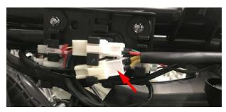
b.Check the connector for looseness or corrosion.
