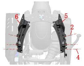
d.Use a T25 torx wrench to remove 2 expansion nails (7). Take out the left rear tail skirt liner (5) and the right rear tail skirt liner (6).
