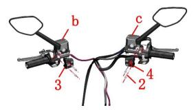
d.Refer to the "Throttle Clue" step and loosen the throttle
