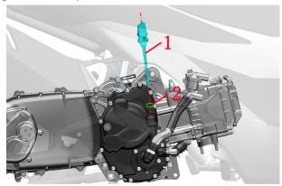
e.Wipe the oil dipstick clean, rotate clockwise by hand to replace the oil dipstick (1) and O ring (2) into the right crankcase cover of the engine.
