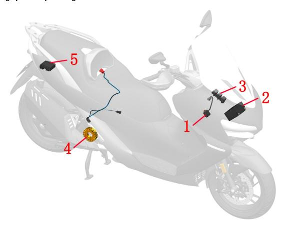
1-Charging port (PKE) 2-Battery, 3-Main fuse (25A), 4-Magneto 5-Rectifier
