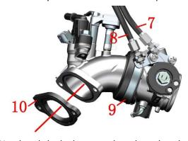
g.Use throttle body cleaner to clean the carbon deposits on the intake manifold and the throttle body outlet. Do not soak the throttle body assembly and intake manifold assembly directly in any liquid.
