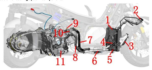
1-Main water tank 2-Water tank filling port 3-Auxiliary tank 4-Main tank inlet pipe 5-Main tank outlet pipe 6-Aluminum water pipes 7-Thermostat outlet pipe 8-Engine water inlet pipe 9-Water and oil share sensors 10-Thermostats
