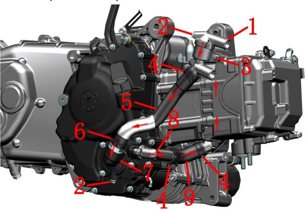
1-Thermostat assembly-M6×12 bolt\*2 3- M6×22bolt\*2 4-Water pipe hoop( $\phi$ 26)\*3 5-Water pump cover inlet pipe 6-Water pipe clamp( $\phi$ 24) 7-Water pump cover assembly 8-Water pump cover outlet pipe joint 9-Water pump cover outlet pipe
