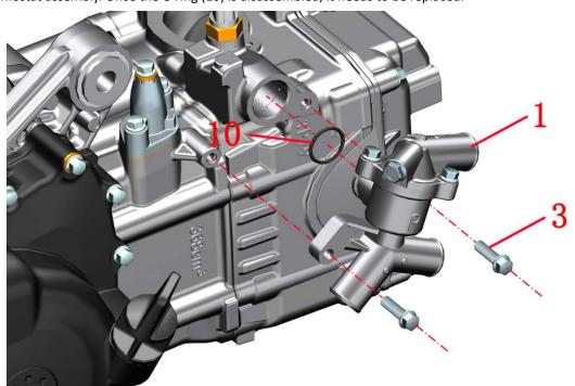
The joint surface should be cleaned before reassembly, and it should be noted that the O-ring should not be missed and  $95\ /\ 135$
