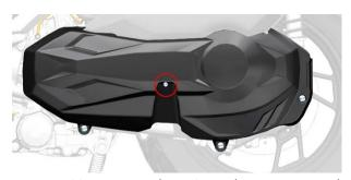
c.Use a T30 torx wrench or 8# socket to remove the 3 M6×16 hexagonal small flange torx bolts, flanging bushings and buffer glue as shown in the figure, and be careful not to lose the bushing and buffer glue. Or use 4# hexagon to remove 3 M6×14 shaft shoulder bolts. Press the center pin of the expansion nail of the air filter decoration cover with a 4# hexagon socket to remove the expansion nail. Then remove the trim cover.
