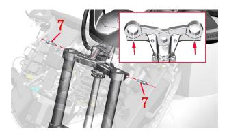
c.Use the 6# hexagon to remove 4 M8×30 bolts (7), pry open the gap on the lower plate with a lot, and remove the left front shock absorber and right front shock absorber.
