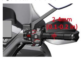
d.After starting the engine, turn the steering knob left and right to make sure the idle speed does not change during steering, and then turn off the ignition.
