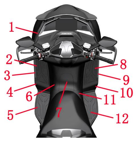
1.Front compartment panel front 2.Front left pedal pad 3.Left pedal decorative cover lining 4.Left pedal upper 5.Rear left pedal pad 6.Front compartment panel rear 7.Fuel tank cover 8. Front right pedal rubber pad
