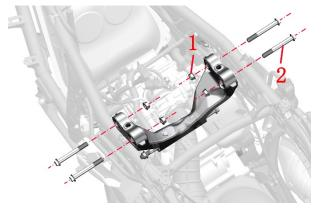
e.Use a 14# wrench to fix the nut (3), and use a 14# socket + ratchet wrench to loosen the bolt (4). Remove the 2 nuts (3). One person holds the rear wheel, and the other person removes the two bolts (4) on the rear shock absorber, and the rear wheel can be gently placed on the ground after removing the bolts. One person holds the engine up, and the other removes the 4 bolts from the frame (2). After removing the bolts, the engine can be gently placed on the ground.
