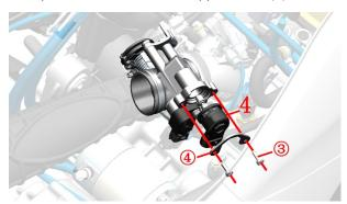
f.Use a throttle cleaner to clean up carbon deposits from the stepper motor head. Spray a small amount of cleaning agent into the valve body bore. It is forbidden to soak the stepper motor with any liquid.
