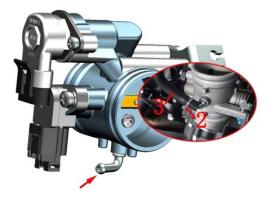
d.Loosen the bolt of the clamp (4) with a 4# hexagon socket and pull out the throttle valve body according to the direction of the arrow after the air filter outlet pipe (5) and clamp (4).
