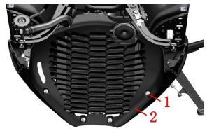
b.Use a T25 torx wrench to remove the shoulder bolts (1) and 4 expansion nails (4) that surround the bottom 4 M6 $\times$ 14 and remove the enveloping bottom (3).
