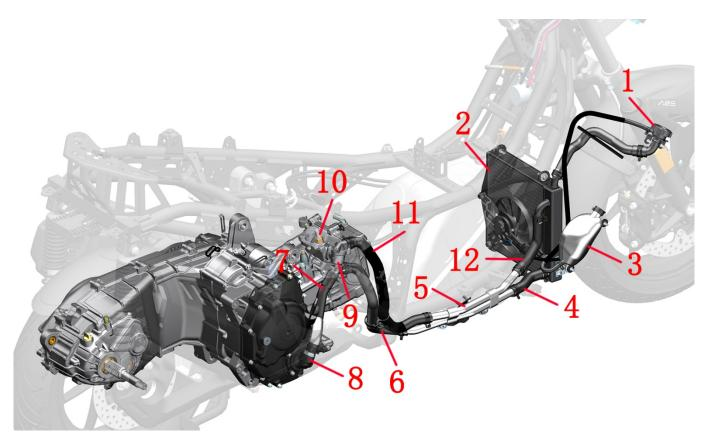
1-Main tank filler 2-Main water tank 3-Auxiliary tank 4-Main tank outlet pipe 5-Aluminum water pipes 6-Engine water pipes 7-The water pump covers the inlet pipe 8-Water pump cover assembly 9-Thermostat assembly10-Water and oil share sensors 11-Thermostat outlet pipe 12-Main tank inlet pipe
