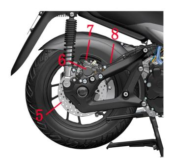
1-Front brake discs 2-FC-HU Brake hoses 3-Wheel speed sensor (front) 4-Front disc brake calipers 5-Rear brake disc 6-Rear disc brake calipers 7-Wheel speed sensor (rear) 8-RC-HUBrake hoses
