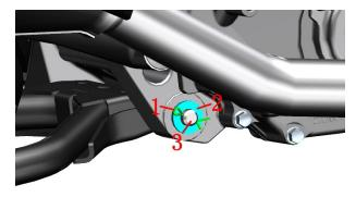
b.Remove the spring from the main bracket.
