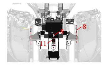
e.Use a T25 socket torx wrench to remove 3 M6 $\times$ 14 shaft shoulder bolts (2) and remove the wire box (12).
