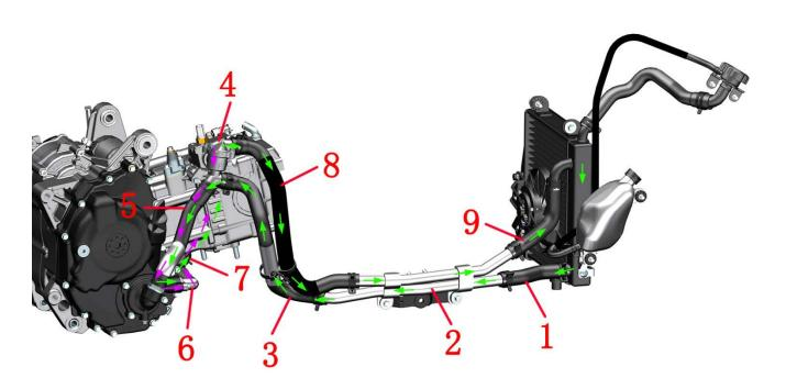
1-Main tank outlet pipe 2-Aluminum water pipes 3-Engine water pipes 4-Thermostats 5-The water pump covers the inlet pipe 6-Water pump cover outlet pipe joint 7-The water pump covers the outlet pipe 8-Thermostat outlet pipe 9-Main tank inlet pipe
