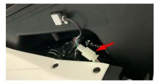
d.Unplug the stepper motor (1) and sensor (2).
