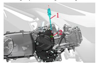
d.After placing the oil receiving pan under the oil drain bolt, remove the M12×1.5×15 oil drain bolt (3) and  $12\times\varphi20\times2$  combined sealing (4) pad with a 14# sleeve.
