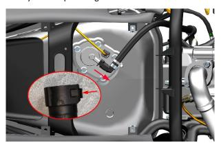
d. After pressing the anti-release lock at the fuel injector, pull out the high-pressure oil pipe in the direction of the arrow.
