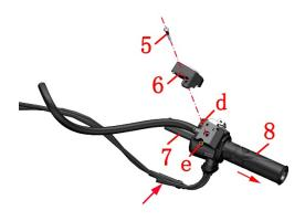
e.Use a 2.5# hexagon tool to remove the set bolt (10) below the left handle rubber sleeve (9), use the 5# hexagon to remove the bolt G and bolt H below the left handle switch, and then use the cross batch to remove the bolt F, and separate the left hand switch up and down. Separate the left handle (11) and the left hot handle (9).
