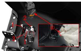
e.Use a T25 torx wrench to remove the 4 M6×14 shoulder bolts (1) of the box panel assembly, and then take out the box panel assembly.
