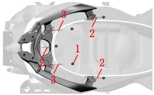
b.Use a T25 torx wrench to remove the 8 M6×12 bolts
