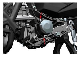
b. Place an oil pan underneath the fine filter cover. Use a 14-sided 65mm cap-style filter wrench (with a Shida model number of 97401) combined with a 1/2" (12.5mm) ratchet wrench to rotate counterclockwise and remove the fine filter.
