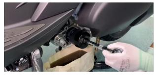
c.Drain the oil inside the fine filter.
