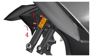
d.First, press down on both sides of the front mud board according to the small arrow, press the bulge at the front mud board arrow inward, and then move the front mud board up to the appropriate part and pull it out according to the direction of the big arrow.
