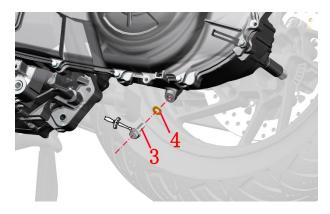
c.Remove the M8×25 oil drain bolt (3) and the  $8.3\times16\times1.5$  copper pad (4).
