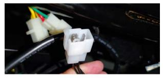
d.After disconnecting the yellow 3P connector, use the multimeter to measure the voltage between the red positive wire and the green negative wire. It should match the battery voltage. Use the multimeter's buzzer mode to check if the green negative wire is continuously connected to the ground (the ground wire can be any stud directly connected to the frame).
