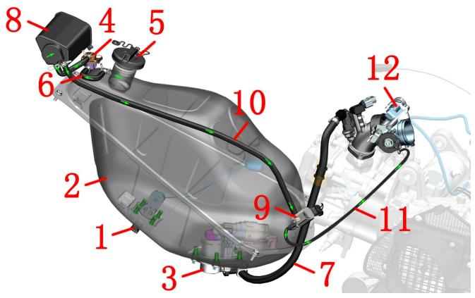
1-Oil level sensor 2-Fuel tanks 3-Fuel pump 4-Air-oil separator (welded inside the tank) 5-Fuel tank cap 6-Adsorption/ventilation tubes7-High-pressure tubing 8-Carbon canisters 9-Canister solenoid valve 10-Solenoid valve intake pipe 11-Solenoid valve outlet pipe 12-Throttle body assembly
