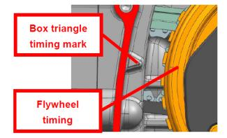
The triangle is aligned with the flywheel timing mark
