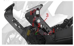
b.Use a T25 Torx wrench to remove the shoulder bolts (1) of the two M6×14 fixed to the lining (3) of the left decorative cover, and remove the inner lining (3) of the left decorative cover.
