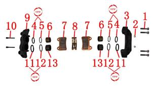
1-Bolt 2-Circlip 3-Caliper inner housing 4- $\phi$ 30 oil seal 5- $\phi$ 30 dust seal 6- $\phi$ 30 piston 7-brake pad 8-brake pad spring 9-caliper outer housing 10-pin 11- $\phi$ 34 oil seal 12- $\phi$ 34 dust seal 13- $\phi$ 34 piston
