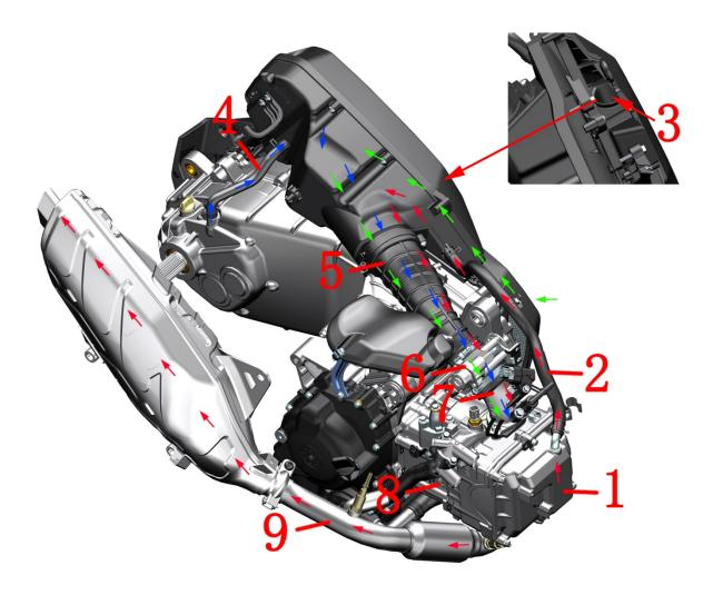
1-cylinder head 2-cylinder head exhaust pipe 3-Air filter intake 4-Gearbox exhaust pipe 5-Air filter outlet pipe 6-Throttle body assembly 7-intake manifold 8-cylinder 9-muffler
