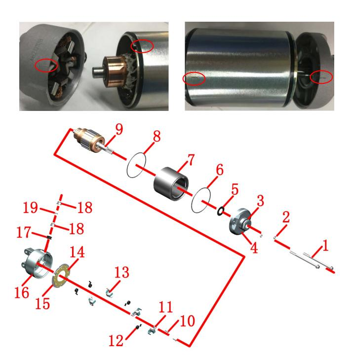
1-M6×90 bolt×2 2-O ring×2 3-O ring 4-starter motor front cover 5-gasket 6-rectangular sealing ring 7-starter motor outer shell 8-rectangular sealing ring 9-electric pestle 10-screw ×2 11-negative brush ×2 12-worm spring ×4 13-positive brush ×2 14-brush rack 15-brush holder insulating gasket 16-starting motor back cover 17-insulating pad 18-nut×2 19-gasket
