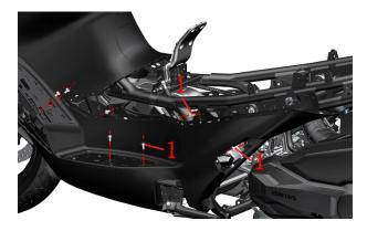
b.Remove the rubber pad on the rear right pedal. Use a T25 Torx wrench to remove 7 M6×14 shoulder bolts (1). Remove the right pedal assembly.
