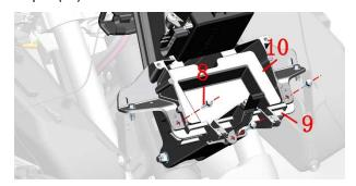
d.Use the 8# sleeve to remove 3  $M6\times16$  bolts (8) and remove the bracket (11).
