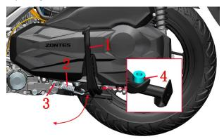
1.Main bracket 2.Main bracket spring 3.Main bracket return spring column 4.Buffer glue
