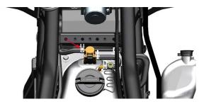
h.Use a ratchet wrench + 10# socket to remove 4 M6×16 bolts (6), and remove the springpad (7) and washer (8).
