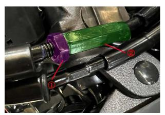
b.If the above adjustments cannot achieve the desired effect, you can remove the throttle body assembly according to the description in "Removing the Throttle Valve Body Assembly and Cleaning the Carbon Deposition". Use a 10# open-end wrench to loosen the 2 nuts on the bracket to adjust. Torque: 3.0 N.m (0.3 kgf.m, 2.2 lbf.ft).
