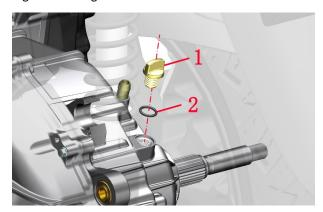
b.Place the oil pan under the rear of the engine on the left side.Use a 14# sleeve to loosen the oil drain bolt (3) counterclockwise.
