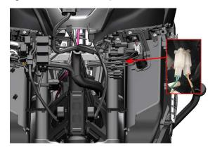
b.Use a T25 torx wrench to remove the shoulder bolts (1) and 1 expansion nail (2) of the 2 M6×14 on the inside of the left decorative cover.
