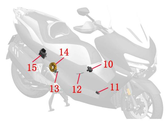
1-Tilt switch 2-PKE 3-Relays 4-Steering lock 5-The right hand handles the secondary switch 6-Right-hand handle switch 7-accumulator 8-Fuse box 9-Start the relay 10-Ignition coil 11-Side bracket kill switch 12-spark plug 13-Crankshaft position sensor 14-Magneto stator 15-ECU
