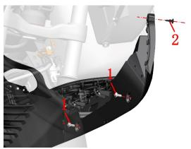
c.After taking out the left pedal rubber pad (3), use a T25 torx wrench to remove the shoulder bolt (1) of 1 M6 $\times$ 14 on the left pedal.
