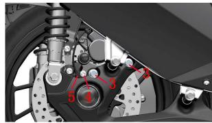
c.Remove the brake pads first.
