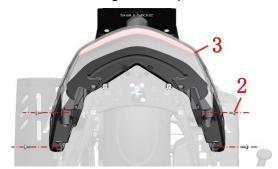
c.Use the joint on the left rear tail skirt lining (5) and the right rear tail skirt lining (6) to pull out, and use a T25 torx
