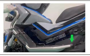
• As shown in the picture, put the ZT368T—G back shirt bottom middle cover in the back. The bottom of the tail skirt is lined with the bottom, aim at the left first, and then press it from the right.
