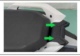
• As shown in the picture, ZT250—S M8 bolts decorative buckle (frosted black) is installed in the assembly.
