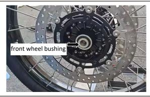
After lifting the vehicle to the appropriate height, the front wheel axle is aimed at the front shock absorber. After installing the hole, put it into the front wheel axle and then use the No. 17 Allen wrench. Torsion standard: 50N\*M
