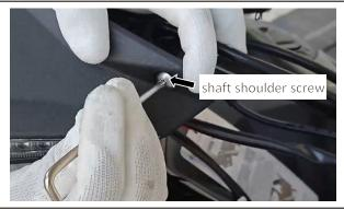
Connect the front left and right turn signal harness and fix the harness connector on the line insede the buckle, turn the ZT703—F right turn signal box and the ZT703—F left install the light wire box on the handguard and alit the installation hole, and put the two non standard self tapping screws ST3.9×12 (black zinc) into the installing hole, then use the ten cross screw driver to fasten.
