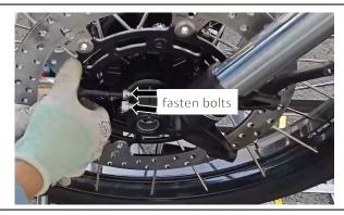
Align the mounting hole of the right caliper and use a No. 8 Allen wrench to fasten the two bolts up and down. torision standard: 45 N\*M
