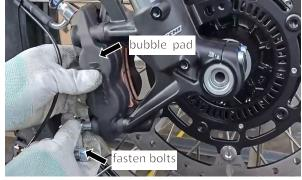
Align the mounting hole of the wheel speed sensor and use T25 Allen wrench tightens the fixing bolt. tenance standard: 10 shi 2 N\*M
