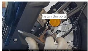
After allising the oil pipe bracket with the mounting hole of the front fender, put it in a GB70.1M6×16 hexagon screw (stainless steel) ust No. 5 Allen wrench to fasten.
