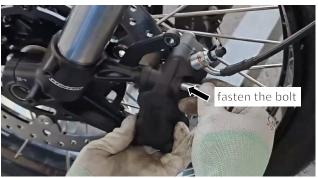
Open the front fender packaging and push the fender in from the back to make it the empty space matches the front shock absorber and stuck the left caliper oil pipe into the fixing clamp.
