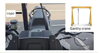
Note: make sure that the rope is tight, until the village belts on both sides and use the No. 12 sleeve to remove the bracket and pressure plate.
