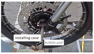
Use the No. 6 Allen wrench to tighten the front shock absorber left and right bolts twice. Torsion standard: 20N\*M
