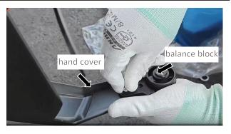
Align the left and right handguards with the installation hole in the direction on the left and right put a
