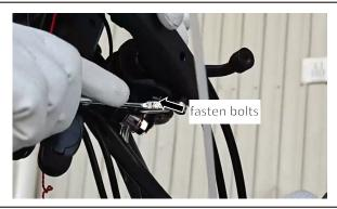
Put two ZT703—F hand shield transfer studs into the same hole position, use a 12 opening wrench to tighten.
