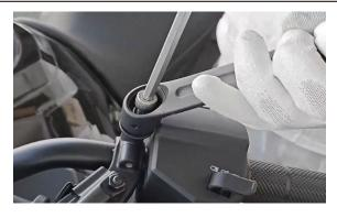
Align the left and right installation of the fender, and use T25 Allen wrench fasten the left side and the right side shaft shoulder screws M6×16+ φ8.5×5(stainless steel) torsion standard:10±2N\*M
