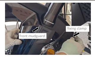
Alim the left stone installation hole of the fender, and use T25 Allen wrench tightens the left and right two inner plum blossom shaft shoulder screws left M6\*16 plus φ8.5\*5 (304 stainless steel). torsion standard: 10±2 N\*M
