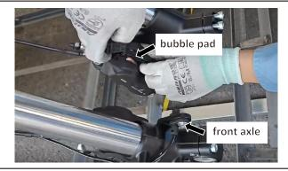
Use the No. 8 Allen wrench to remove the fixing screws of the left and right brake calipers, remove the left and right brake calipers.
