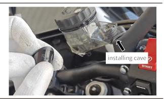
Two square flange thread bushings M6×5- ф10×3 (environmentally friendly color) fix to the right and left inner sides of the front fender, so that the front fender and reduce alim the hole position of the shock installation, and put one GB70.1M6×16 hexagon screw (stainless steel) on the left and right side, Use No.5 Allen wrench to fasten.
