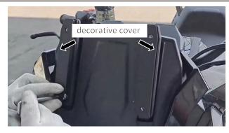
Take out the ZT703-F windshield ( II ) from the accessory box, aim ZT703-F windshield ( II ) and the mounting hole of the windshield bracket, use the T25 Allen wrench to put the original screw back. torsion standard: 10±2N\*M
