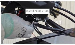
Two inner plum blossom shaft shoulder screws M5×13—φ7×3 (304 stainless steel) installed above the left and right handguards, useing T25 Allen wrench to fasten. (torsion standard: 10 ±2N\* M)
