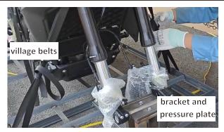
Use the No. 17 Allen wrench to remove the front axle and use scissors to remove it. Open the bubble pad.
