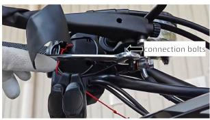
Install the ZT703—F left turn signal hand cover assembly (MES) \ ZT703—F right turn signal hand cover assembly (MES) and ZT703-F left hand balance block (210g) \ ZT703-F right hand handle balance block (210g) with two inner plum blossom shaft shoulder screws M5×13—φ7×3 (304 stainless steel) part installed, use T25 Allen wrench fasten \( \) (torsion standard: 10±2Nm)
