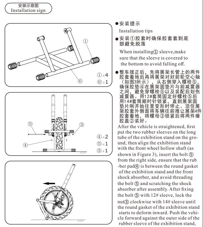
let the four rubber sleeves of the exhibition stand land, lock the nut ③ and install the two rubber covers ②.
