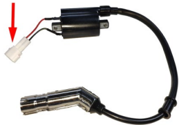
ZT310 EFI ignition coil (with high voltage line)
