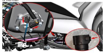
If the fuel pump needs to be removed from the vehicle, the fuel pump can be used to drain the fuel in the fuel tank. After lifting the vehicle, press the plug buckle as shown in the figure to pull out the cable. Remove 5 bolts from the bottom with a 10# sleeve, and then remove the fuel pump after removing the high-pressure fuel pipe bracket. Be careful not to press the fuel outlet pipe shown in the red circle. Once damaged, you can only replace the entire fuel pump assembly.
