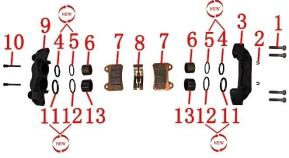
1- Bolt 2- Circlip 3- Inner side caliper housing 4- $\phi$ 30 oil seal 5- $\phi$ 30 dust seal 6- $\phi$ 30 piston 7- Disc brake pad 8- brake spring 9- Out side caliper housing 10-Pin 11- $\phi$ 34 oil seal 12- $\phi$ 34 dust seal 13- $\phi$ 34 piston
