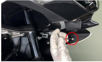
b. Start the motorcycle, open the left glove box, and use a 4# inner hexagon to remove one M6×14 shoulder bolt and one expansion nail as shown in the picture
