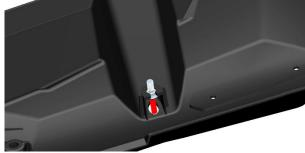
d. Align the left bolt with the mounting hole and tighten it. Put the 4 bolts back in with the 4# inner hexagon.
