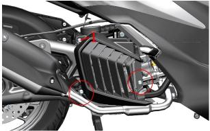
b. unscrew the cover of the water filling port counterclockwise to add coolant.
