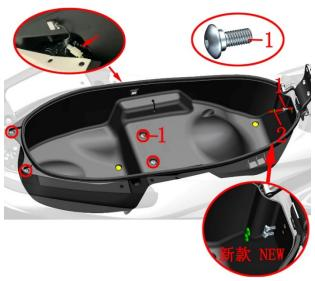
c. Slightly lift the back of the glove box until the harness connector on the left side of the glove box is exposed, unplug the ambient light plug on the left side of the glove box, unplug the plug, and take out the glove box completely.
