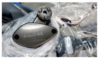
d. After wearing waterproof gloves, use a Phillips screwdriver to remove the bolt (1), and remove the upper cover (2), the cover (3), and the sealing rubber gasket (4).
