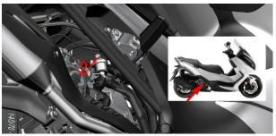
d. Put on waterproof gloves and add coolant to the water inlet of the Radiator with the help of an extended funnel. Until the position of the vent bolt of the thermostat is stably overflowed with coolant, the coolant level can be seen at the water filling port.
