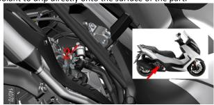
c. Put on waterproof gloves and add coolant to the water inlet of the Radiator with the help of an extended funnel. Until the position of the vent bolt of the thermostat is stably overflowed with coolant, the coolant level can be seen at the water filling port.
