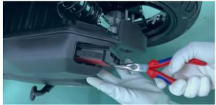
c. Replace the new filter element and sealing strip.
