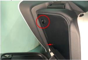
c. Gently pat the left head side panel forward with your hand to remove it, and use the same method to remove the right side panel.
