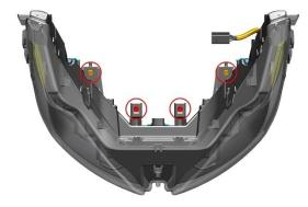
c. Use the 4 expansion nails on the left and right sides as shown in the figure to remove.
