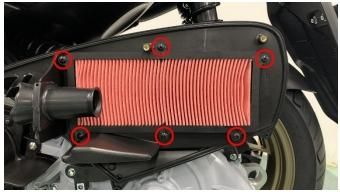
b. Remove the old air filter element. Blow the dust inside the air inlet pipe with a dust blower, and then wipe the inner wall with a clean non-woven cloth.
