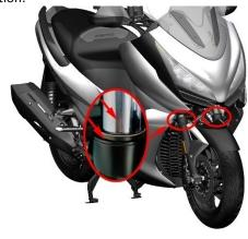
b. Check whether the bottom tube is painted off; whether the installation points of the front fender, the front wheel hollow shaft and the front brake caliper are broken or cracked. Check if there is any leakage at the bottom of the bottom cylinder.
