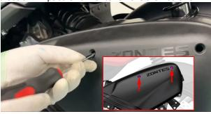
c.Use a Phillips screwdriver to remove the 4 screws that fix the housing of the air filter.
