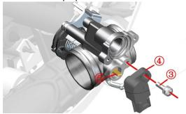
Simple test method: connect the whole vehicle to the diagnostic instrument, press the flameout switch (no need to ignite), turn the throttle handlebar from the initial position to full open, this process to see if the throttle position signal follows the change from 0 to 100.
