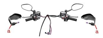
c. Remove 4 M6×30 bolts (2) with 5# Allen, remove the left deputy handle switch (3), rear disc brake main pump assembly b, right deputy handle switch (4), front disc brake main pump assembly c.
