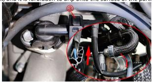
c. Find the circlip at the bottom of the valve body (2) pinch both ends of the circlip with your hands and move it out, and then pull out the desorption tube (3).
