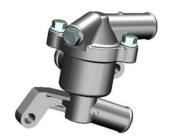
When the temperature reaches 80°C (176 F), the heating rate slows down, and the thermostat works normally. If the water temperature has been rising rapidly, when the internal pressure reaches a certain level, the sudden overflow of boiling water indicates that the valve is stuck.
