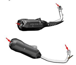
•Keep the drain hole at the bottom of the muffler unblocked to prevent condensation water from accumulating in the muffler cavity.
