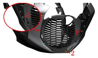
b. Use a 4# inner hexagon to remove 2 bolts on the left and right sides, pull off the lining plate of the right decorative cover and the water tank filling port, and remove the lining plate on the left side.
