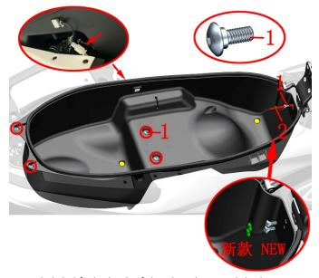
c. Slightly lift the back of the glove box until the harness connector on the left side of the glove box is exposed, unplug the ambient light plug on the left side of the glove box,
