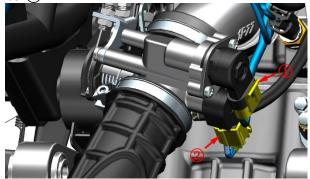
b. Place the small container under the high-pressure oil pipe, press the buckle indicated by (3) and pull out the high-pressure oil pipe(1) in the direction of the arrow at the same time. A small amount of fuel will flow out when it is pulled out, and it is forbidden to drip onto the surface of the part.
