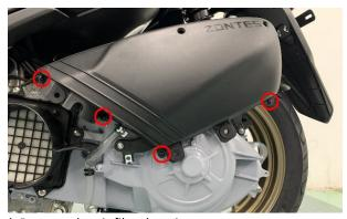
d. Remove the air filter housing.
