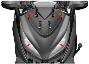
b. Lower the windshield to a low position, use 4# inner hexagon to remove the 2 front bolts, the 2 expansion bolts on the left and right sides of the rear, and the 2 left and right
