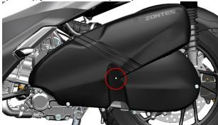
c.Use 4# inner hexagon to remove the 3 M6×14 bolts as shown in the figure.Use 4# inner hexagon to remove theswell nail.
