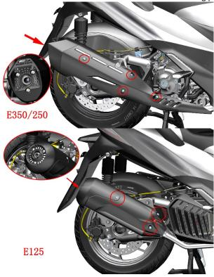
2. Check for nut and bolts at the muffler
