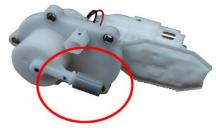
When reassembling, you need to pre-tighten diagonally and then tighten the 5 bolts. Otherwise, the uneven compression of the seal rubber ring of the fuel pump may cause leakage and cause safety hazards.
