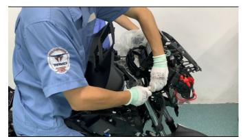
n. Pass the handle assembly through the front storage box panel, and remove the front storage box panel assembly.
