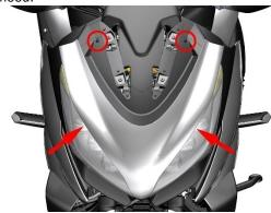
b. Lower the windshield to a low position, use 4# inner hexagon to remove the 2 front bolts, the 2 expansion bolts on the left and right sides of the rear, and the 2 left and right expansion nails on the inner side, and remove the rear of the windshield liner.
