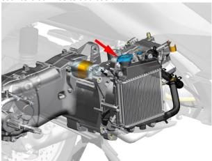
c. Use a 10# sleeve to loosen the thermostat bleed bolt (2) counterclockwise by 4 to 5 turns, do not completely remove it. Note that a small container is required to receive the coolant overflowing from the exhaust bolt. Do not allow the coolant to drip directly onto the surface of the part.
