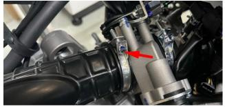
d. Pull the air outlet pipe to the right side of the motorcycle to expose the two M6×30 bolts that fix the starter motor, and remove them with an 8# sleeve. After removing the bolts, remove the starter motor from the engine in the direction indicated by the big arrow.
