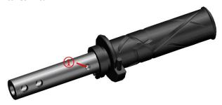
c. When installing the secondary handle bar switch, it is necessary to align the joint surface of the counter-handle bar switch and the main pump of the disc brake with the triangle mark on the handle bar switch, and then use 5# hexagon to tighten 4 M6×30 bolts.
