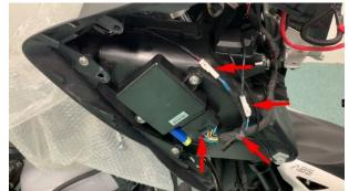
i. Open the buckle and remove the OBD diagnostic connector
