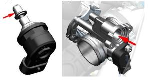
g. Install the stepper motor back to the valve body, paying attention not to miss the sealing ring. Plug the plug back in.
