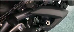
d.inspection O ring(2)Whether there is damage or aging, if not, wipe it clean, if any, replace it.
