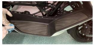
e. Remove 3 M6 $\times$ 16 bolts (2) with 5# inner hexagon, remove 1 M6 $\times$ 14 bolt (3) on the rear side with 4# inner hexagon, and remove 1 expansion nail at the front and rear (1).
