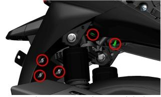
b. Use 4# inner hexagon to remove the 2 M6×14 bolts that fix the rear fender assembly on the frame.
