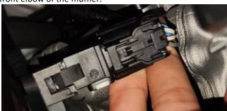
Use a multimeter to measure the resistance of the heating element of the two wires to  $9\pm2k\Omega$ ; E350 model can measure the current should be less than or equal to 2.1A. Otherwise, it can be judged that the oxygen sensor is faulty. The ceramic inside the oxygen sensor is hard and brittle. It is forbidden to knock with hard objects or blow with strong gas, otherwise it is easy to cause damage.
