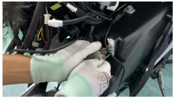
j. Use 4# inner hexagon to remove 2 M6 $\times$ 14 bolts (2), use 6# inner hexagon to remove 2 M6 $\times$ 25 bolts (1) to fix the main lock, and pull out the main lock connector.
