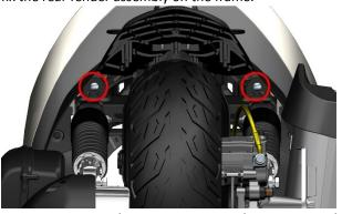
c. Use a 4# inner hexagon to remove the two M6 $\times$ 14 bolts on the left and right sides of the motorcycle that fix the taillights.
