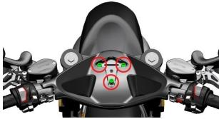
f. Pull out the cable fixed on the steering handle. Remove the steering handle.
