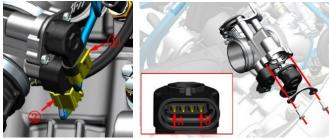
c. Use a short Phillips screwdriver to remove the 2 GB9074.4 M5×16 bolts (3) that comes with the throttle valve body assembly, and then remove the the anti-off card (4), and then take off the stepper motor. It is forbidden to soak the sensor with any liquid.
