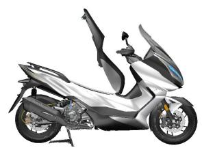
b. Use a 10# sleeve to remove the 4 M6 nuts that the seat is fixed on the seat installation plate, grasp the seat with both hands and pull out the seat obliquely upwards according to the angle of the studs. Note: When the angle is wrong and the seat cannot be pulled out, do not use brute force to forcibly pull the seat out to prevent damage to the thread on the seat installation stud.
