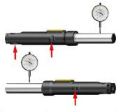
For slight deformation of less than 0.2mm (0.008 in), the front fork tube can be supported by a V-shaped iron block, and soft rubber, rubber, copper, etc. should be placed on the contact surface to prevent the front fork tube from being
