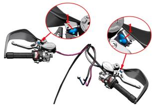
b. Use the 5# Allen to loosen the balance block bolt A 5-8 turns, and remove the left and right hand guards and the balance block assembly.
