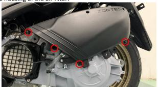
d. Remove the air filter housing.
