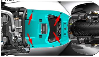
c.Use 4# inner hexagon to remove the  $M6 \times 14$  bolts.
