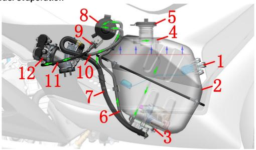
1- Fuel level sensor 2- Fuel tank 3- Fuel pump 4- Oil-air separator (welded inside the fuel tank) 5- Fuel tank cap 6- Adsorption/vent pipe 7-High pressure fuel pipe 8-Carbon tank 9-Carbon tank solenoid valve 10- Solenoid valve intake pipe 11-solenoid valve outlet pipe 12-throttle valve body assembly Fuel evaporation:
