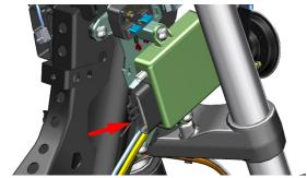
d. Pull out the RC-HU hose and wheel speed sensor wire from the rear inner mud plate.
