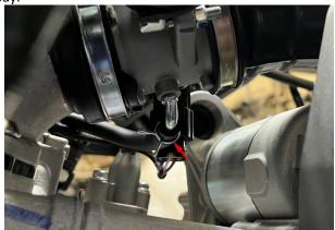
h. Remove one M6  $\times$  12 bolt (1) fixing the wheel speed sensor on the rear rocker arm with 4 # hexagon socket. Take out the wheel speed sensor and take it out of the fixing clamp. Then use 14 # sleeve to remove the two M8  $\times$  37 bolts (2) fixing the brake caliper. Pass the brake caliper and wheel speed sensor through the middle of the shock absorber in the direction of the arrow.
