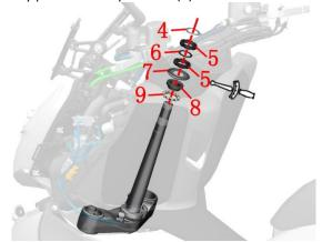
c. Install the steering handle seat block and lower yoke plate, put in the gasket (3), and finally screw in the cap nut (2) with a torque of 100N. m (10.2 kgf. m, 74 bf. ft)
