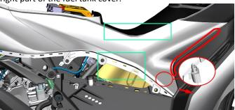
c. Use the same method to remove the left part of the fuel tank cover plate.
