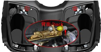
e. Turn over to the back and remove 3 ST4.2  $\times$  12 with 5 # hexagonal socket After self tapping, remove the front storage box switch from the panel. Remove the latch from the switch.
