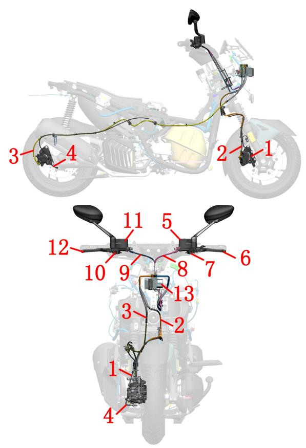
1-wheel speed sensor (front wheel) 2-FC-HU brake hose 3-RC-HU brake hose 4-wheel speed sensor (rear wheel) 5-rear brake lever 6-rear brake switch 7-RMC -HU brake hose 8-rear disc brake main pump 9-FMC-HU brake hose 10-front brake switch 11-front disc brake main pump 12-front brake handle 13-hydraulic control unit
