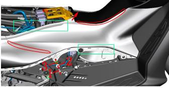
c. Grasp the mark (green rectangle) on the right decorative cover of the fuel tank cover by hand and pull it out in the direction of the arrow until the mushroom button (red circle) on the fuel tank cover is pulled out, and then remove the right part of the fuel tank cover.
