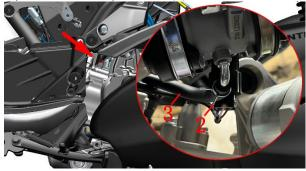
d. Loosen the bolt of the clamp(4) with a 4# inner hexagon and pull out the air filter outlet pipe(5) and clamp(4) in the direction of the arrow to pull out the throttle valve body.
