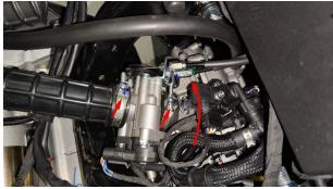
e.Rotate the throttle body so the stepper motor plug is facing up.Unplug the plug of the stepping motor  $\bigcirc$  1.
