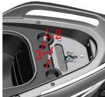
c. Grasp the tail skirt of the storage box and pull it upward obliquely, paying attention to the cables in the battery compartment. Pull up to see the left side of the glove box atmosphere lamp thread, unplug the thread and remove the glove box assembly.
