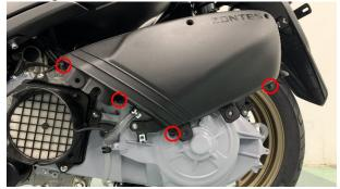
d. Remove the air filter housing.
