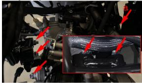
c. Check whether the engine nut is loose.
