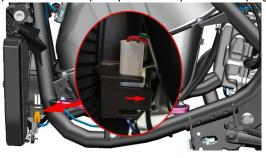
g. Remove 2 M6's on both sides with 8 # socket  $\times$  Take down the water tank assembly after 22 bolts (1).
