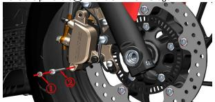
b. Remove the brake pads.
