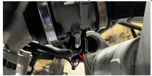
k. Remove one M6 fixing the wheel speed sensor on the rear rocker arm with the 4 # hexagonal socket × Take out the wheel speed sensor and take it out of the fixed clamp. Then use 14 # sleeve to remove 2 M8× 37 fixed brake calipers bolt (2), pass the brake caliper and wheel speed sensor through the shock absorber in the direction of arrow.
