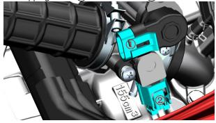
c. Use a short Phillips screwdriver to remove the 2 bolts (3) that comes with the throttle valve body assembly, and then remove the three-in-one sensor (4). It is forbidden to soak the sensor with any liquid.
