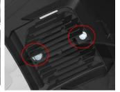
e. Pull down the rectifier and pull the cable out of the hole in the front of the rear mud board. Remove the rectifier from the car. When pulling out the cable, be careful not to pull it forcibly to avoid damaging the plug or pulling off the wire.
