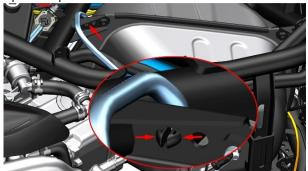
f. Use a 10# sleeve to remove the 4 M6imes12 bolts (1) that fix the fuel tank.
