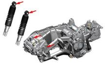
d. Check whether the weld at the bottom of the shock absorber is leaking.
