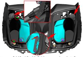
g. Remove 2 M6× 16 with 5 # hexagonal socket. Separate the right storage box lock bracket from the right storage box lock.
