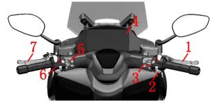
1. Front brake handle 2. Right handle switch 3. Right auxiliary switch 4. Meter 5. Left auxiliary switch 6. Left handle switch 7. Rear brake handle
