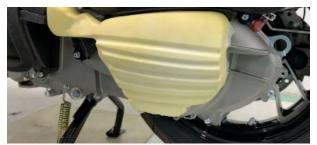
d. Clip M6×14 bolts to the inner step hole of the engine left cover, and then use a 4# inner hexagon to penetrate from the outside and hold the bolt
