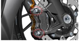
b. Place the oil drain pan under the front disc brake caliper. First remove the screw rubber cap (1), wear waterproof gloves, and then remove the bolt (2) with 8 # box wrench, remove the bolt (3) with 14 # box wrench, and remove two copper washers (4).
