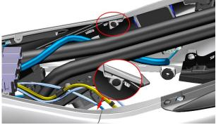
b. Remove one M6 on the right part of the fuel tank cover plate with 8 # socket × 22 bolts (1), remove bushing (2) and buffer rubber (3); Grasp the mark on the right part of the fuel tank cover plate (green rectangle) and pull it diagonally upwards in the direction of the arrow until the buckle of the right part of the fuel tank cover plate is separated from the middle part of the fuel tank cover plate and the right part of the tail skirt (red area).
