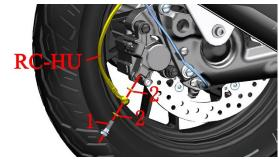
b. Use a 14# sleeve to remove the bolt (3). Standard torque of bolt (3): 24N.m (2. 4kgf.m, 18 lbf.ft).
