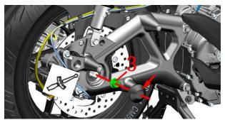
c.D350/D250:Use 4# hex socket to remove the M6×14 bolt (5) on the right middle of the rear inner mudguard, use 4# hex socket to remove the front M6×12 bolt(4) and the rear M6×14 bolt(5). Remove the two M6×12 bolts(4) at the bottom of the rear rocker arm, and remove the wheel speed sensor(6). Pull out the staples on the position indicated by the arrow and remove the decorative cover(7) of the engine right cover.
