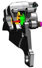
d. Grasp the outer brake pad with your left hand and insert the pin 2 with your right hand, being careful not to insert it to the end. Install the inner brake pad in place, then insert the pin to the end and use the 5# inner hexagonal lock pin 2. Be careful not to install it backwards, the grooved side faces the brake disc; the black metal back plate faces the caliper.
