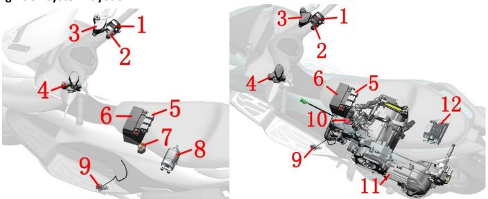
1-Right-handle switch (stop switch, start button) 2-Right-handle secondary switch (to unlock the vehicle) 3-Front disc brake main pump (front brake switch) 4-Rear disc brake main pump (rear brake switch) 5-Fuse box 6-Battery 7-Starting relay 8-Starting motor(D125/D350/D250) 9-Side bracket flameout switch 10- starter relay(D155) 11- start-stop engine (D155) 12- start-stop controller(D155)
