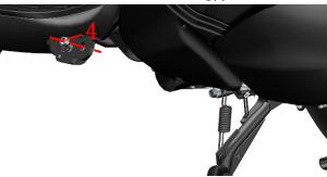
f. Use diesel or kerosene, or a clean cloth to wipe off the remaining grease. Apply a proper amount of grease to the two installation planes inside the side bracket and the surface that matches the flameout switch, and try not to apply it to the threaded holes.
