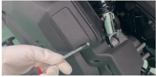
b. Remove the old air filter element. Blow the dust inside the air inlet pipe with a dust blower, and then wipe the inner wall with a clean non-woven cloth.
