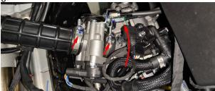
b. After unplugging the desorption pipe at the bottom, pull out the air filter outlet pipe and then remove the throttle valve body assembly.
