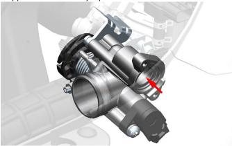
h. Install the stepper motor back to the valve body, paying attention not to miss the sealing ring. Plug the plug back in.
