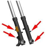
c. If there is a large amount of hydraulic oil attached to the front fork tube, wipe it clean and observe after riding. If there is no oil stain or slight oil stain, it is the hydraulic oil accumulated during the assembly of the dust seal, and it can be judged that the oil seal is not leaking. If there is a small amount of oil stains or sludge mixture, remove the dust seal and wipe clean the front fork tube and oil seal surface, first compress the front shock absorber and then wipe clean and
