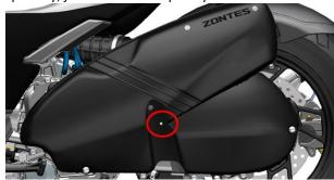
c.Use 4# inner hexagon to remove the 3 M6 $\times$ 14 bolts as shown in the figure. Use 4# inner hexagon to remove the swell nail.
