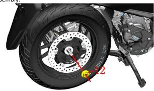
g. Replacing the rear brake disc
