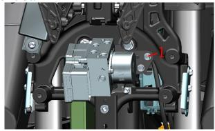
d. After holding the hydraulic control unit firmly, use 4# inner hexagon to remove the bolt(2), then the hydraulic control unit(5) can be removed. If you need to replace the bracket(4), you need to remove the flanging bushing(3) and the cushion rubber(6).
