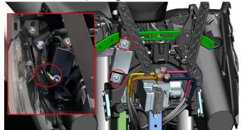
b. Remove the two M6× 16 on the hydraulic control unit bracket with 8 # socket. Remove the hydraulic control unit with bolts. Remove M8 from horn bracket with 6 # hexagonal socket  $\times$  30, remove the horn.
