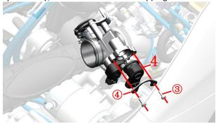
f. Use throttle cleaner to clean the carbon deposits on the head of the stepper motor. Spray a small amount of cleaning agent into the valve body hole. It is forbidden to soak the stepper motor with any liquid.
