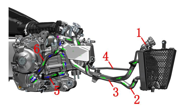
1 - Water inlet pipe 2 - Water outlet pipe of main water tank 3 - Water inlet pipe of main water tank 4 - Connecting pipe of auxiliary water tank 5 - Water inlet pipe of cylinder 6 - Water inlet pipe of water pump cover
