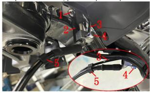
d. Check whether the surface of the removed hose is aging, cracked, damaged, abraded, etc. Wipe up the remaining brake fluid with a non-woven cloth, and then wrap the ends of the hose with cling film or a plastic bag to prevent foreign matter from entering. Check whether the cable sheath of the wheel speed sensor cable is damaged. If the sheath is frayed, it can be glued with electrical tape to prevent short-circuit.
