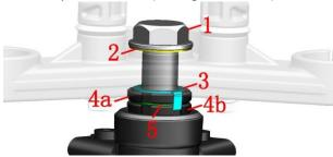
e. The front wheel is hung in the air to straighten the direction handle, and gently push and pull the direction handle by hand to feel whether the steering mechanism is smooth and free of jams. When the front fork assembly is slightly tilted to one side, it should be able to slowly deflect to the end under its own weight. If it is quickly to the end, it needs to be readjusted.
