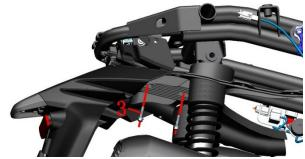
d.Production of vehicles after September 2023:Secure the top nut with 10# plum wrench.Remove 2 bolts from the bottom with 8 # short socket,and then remove the two gaskrts andbushing.
