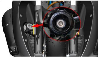
b. Use a 10# sleeve to loosen the thermostat bleed bolt (2) counterclockwise by 4 to 5 turns, do not completely remove it. Note that a small container is required to receive the coolant overflowing from the exhaust bolt. Do not allow the coolant to drip directly onto the surface of the part.
