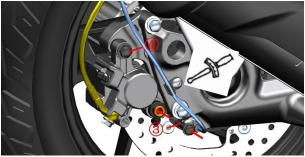
c. Push the piston to the end in the direction of the arrow with the help of a tool. If the resistance is high, you can refer to the method of adding brake fluid to the front brake main pump to remove the upper cover and then push. If the spring on the caliper falls off, it needs to be reinstalled in the direction shown in the figure.
