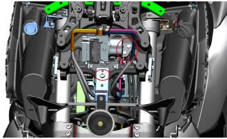
c. Grasp the windshield base assembly and remove 3 M8  $\times$  25 bolts with 12 # socket, remove the windshield base assembly from the motorcycle.
