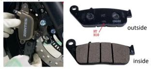
e. Observe from both sides whether the upper part of the brake pad has hit the shrapnel, otherwise the position needs to be readjusted.
