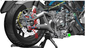
d. One person uses 21 # socket to extend into the front of the fine filter to fix one nut (2) on the left side of the motorcycle to fix the engine, and the other person uses 24 # socket to replace one bolt (1) on the right side of the motorcycle to fix the engine
