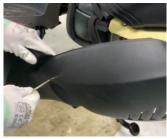
c. Align the left bolt with the mounting hole and tighten it.
