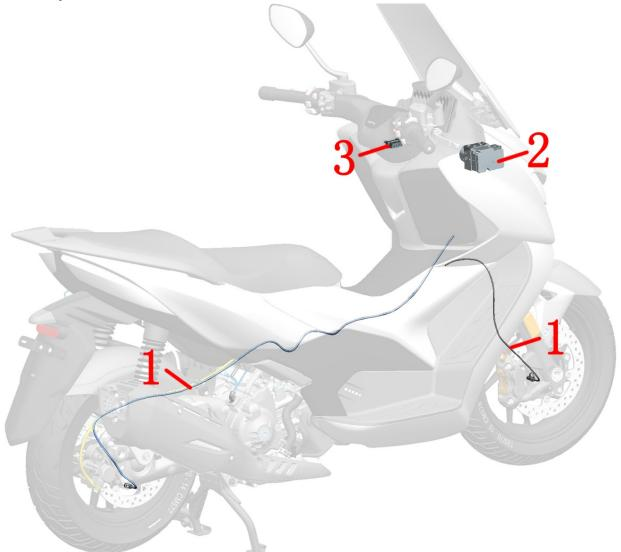
1-Front and rear wheel speed sensor 2-ABS hydraulic control unit 3-OBD diagnostic interface
