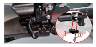
The replacement procedure of the front brake switch is the same as that of the rear brake switch. The throttle cable needs to be removed to facilitate the removal of the bolt (1).
