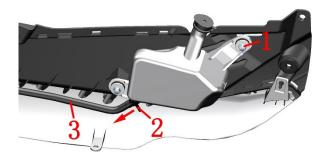
b. Pull the two water pipes out of the water pipe clamp, which is made of plastic, and pay attention to the strength.
