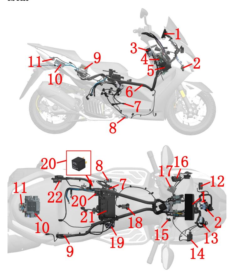
1-TFT meter 2-Speaker 3-Faucet lock 4-Charging port holder 5-PKE 6-Main cable 7- ignition coil 8-Side bracket flameout switch 9-Engine Controller (ECU) 10- start-stop controller 11-seat lock 12-Tipping switch 13-Windshield Motor Controller 14-Flash 15-Induction antenna 16-USB charging cable 17-Front storage compartment lock 18-Electronic tank lock 19 - carbon can solenoid valve 20 - starter relay (auto start-stop exclusive) 21 - battery 22 - PKE buzzer.
