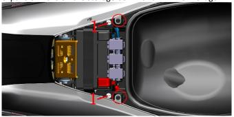
b. Remove 2 bolt decorative buckle (2), and then use 4# hexagon socket to remove 2 M6×16 bolts (1).
