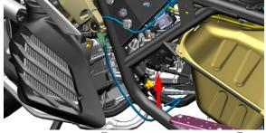
c.Unplug the sensor ① and the stepper motor ② on the throttle valve body according to the steps in Dismantling the throttle valve body assembly to remove the carbon deposit.
