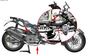
b. Pull out the plug of high voltage package on the engine head.
