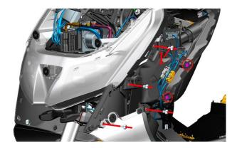
c. Unhook the plug fixed on the left panel lining and arrange it to one side. Remove the bottom lining of the left panel.
