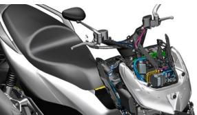
b.Take out the handle switch harness and brake hose in the direction wire clip from the direction of the wire clip gap one by one, until the direction is taken out all the wire harnesses in the wire clip, and then use the 4# inner hexagon to remove the M6×12 bolt that fixed direction wire, take out the direction of the wire clamp.
