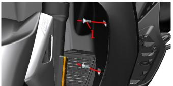
d. Use the 4 # hexagonal socket to remove the 1 M6× 14 Shoulder bolt  $\ ^{(1)}$  at the left of the surrounding base plate connection; Then use the 4 # hexagonal socket to remove the 2 expansion nails (2) at the left part of the surrounding base plate connection.
