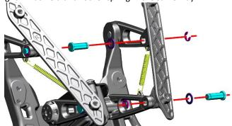
e. Remove 2 M6× 16 with 4 # hexagonal socket. Remove the spring washer. Separate the windshield motor pressing plate, windshield motor assembly and windshield base assembly.
