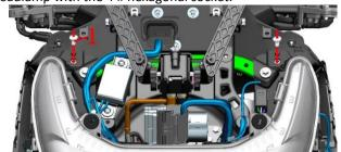
b. Remove the M6× 14 Shoulder bolt (1) at the left of the headlamp with the 4 # hexagonal socket. Remove the expansion nail with 4 # hexagonal socket. Remove the bolts and expansion nails on the other side in the same way.
