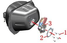
When re-assembling, you need to pre-tighten the corners and then tighten the 5 bolts. Otherwise, the uneven compression of the sealing rubber ring of the fuel pump will easily cause leakage and cause safety hazards.
