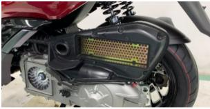
c. Replace the new filter element and sealing strip.
