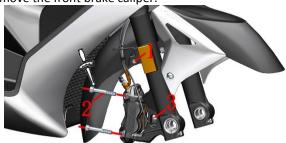
c.Use 4# inner hexagon to remove the two M6×14 bolts(4) on the left and right sides of the front fender; then use 5# inner hexagon to remove one M6×30 bolt(1), take out the gasket(5).
