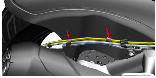
e. Pull out the wheel speed sensor from the clamp(4), remove the bolt(5) with a 4# inner hexagon, and then
