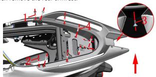
b. Put down the rear right foot pedal, and use the 4 # hexagonal socket to remove the right cover to connect one M6 × 14 of the rear right foot pedal bracket. Shoulder bolt (3) and 1 expansion nail,; Grasp the mark of the left cover (green rectangle) with your hand, and pull it out alternately from the outside to the inside in the direction of the small arrow until all five mushroom buttons (red circle) on the left cover are pulled out, and then remove the left cover.
