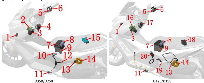
1 - Dump switch 2 - PKE 3 - relay 4 - main lock 5 - right handlebar auxiliary switch 6 - right handlebar switch 7 - battery 8 - fuse box 9 - start relay 10 - ignition coil 11 - side bracket flameout switch 12 - spark plug 13 - crankshaft position sensor 14 - magneto stator 15 - ECU 16 - PKE(D125) 17 - main lock(D125) 18 - ECU(D125) 19 - spark plug(D125) 20 - ignition coil
