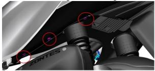
f.Remove the 3 expansion pins connecting the right and middle of the tail skirt using a 4# inner hexagon.
