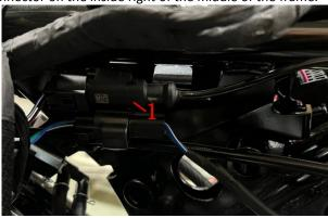
b. First remove the 3 pieces of wire clamp(3), and then pull out the wheel speed sensor(1) and the RC-HU hose from the 3 pieces of oil pipe clamp(2). If you need to remove the tubing clamp(2), you can use 4# inner hexagon to remove the bolts and then you can take it off.
