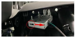
e. Disassemble the left storage box outer cover according to the steps of the right storage box outer cover.
