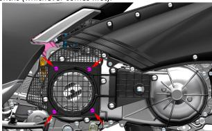
b. Remove the sponge and replace it with a new filter element. Note that the black side faces the engine and the white side faces outward
