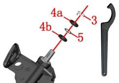
c. Screw the adjusting nut (4b) clockwise to 50N.m (5.1 kgf.m, 37 lbf.ft), turn the front of the car to feel tight to normal, loosen 1/4 turn counterclockwise, and screw clockwise again to 15N.m (1.2kgf.m, 11 lbf.ft). Continue to turn the front of the car, slightly tight or slightly loose, then fine-tune about 1/6 turn.
