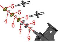
c. Install the semi-circular key in the groove of the lower link plate, then align the gap between the spacer and the base with the semi-circular key, and finally screw in the cap nut, torque: 100N.m (10.2 kgf.m, 74 bf.ft)
