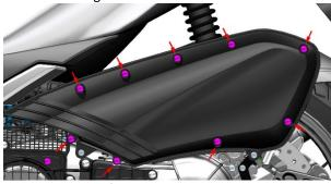
b. Remove the air filter housing.
