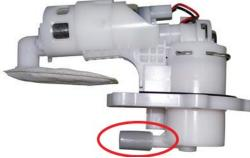
When reassembling, you need to pre-tighten diagonally and then tighten the 5 bolts. Otherwise, the uneven compression of the seal rubber ring of the fuel pump may cause leakage and cause safety hazards.
