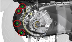
b.Use 4# inner hexagon to remove the M6×14 bolt as shown in the figure. The bolt here cannot be removed temporarily, just loosen it completely.
