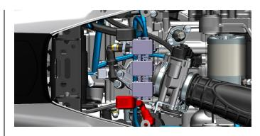
b. Remove a total of 4 pcs swell nails indicated by the arrow. For instructions on disassembly and assembly of swell nails, please refer to the pre-service instructions in this chapter.
