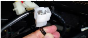
d. After unplugging the yellow 3P plug, measure the red positive wire and green negative wire with a multimeter, and the battery voltage should be measured. Use the buzzer file of the multimeter to check whether the green negative wire and the ground wire (the ground wire can be found in any stud directly connected to the frame) are always conducting.
