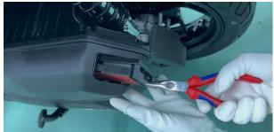
c. Replace the new filter element and sealing strip.
