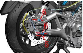
d. Insert the high-voltage package at the front of the engine back, and install one M12 nut back on the cradle to fix the engine, use 17# torx wrench to fix M12 nut, another person uses 15# socket to tighten bolt, torque: 65N.m (6.5 kgf.m, 48 lbf.ft).
