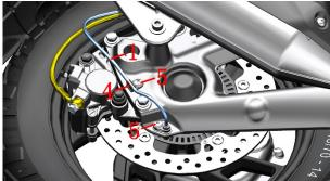
f. Check whether the surface of the removed hose is aging, cracked, damaged, abraded, etc. Wipe up the remaining brake fluid with a non-woven cloth, and then wrap the ends of the hose with cling film or a plastic bag to prevent foreign matter from entering. Check whether the cable sheath of the wheel speed sensor cable is damaged. If the sheath is frayed, it can be glued with electrical tape to prevent short-circuit.
