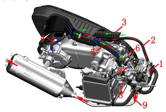
1- Cylinder head 2-Cylinder head exhaust pipe 3- Air filter intake pipe 4- Crankshaft Box exhaust pipe 5-Air filter outlet pipe 6-Throttle valve body assembly 7- Intake manifold 8-Cylinder 9- Muffler
