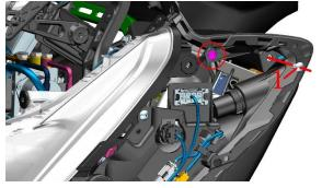
c. Grasp the speedometer panel with one hand and lift it slightly in the direction of the big arrow, and pull out the speedometer plug connected to the speedometer with the other hand.
