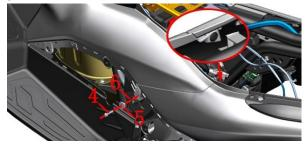
f. Start by snapping the 4 decorative bolt buckles. Remove the 4 M6×14 shoulder bolts (1) of the windshield with 4# Allen. Remove the windshield cover, windshield pad, and sun visor.
