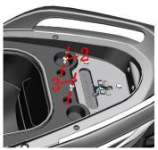
c. Grasp the tail skirt of the storage box and pull it upward obliquely, paying attention to the cables in the battery compartment. Pull up to see the left side of the glove box atmosphere lamp thread, unplug the thread and remove the glove box assembly.
