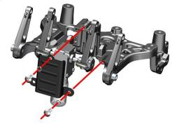
f. Use a Phillips screwdriver to remove two M4  $\times$  16 bolts, separate the rocker arm pressure block from the right lower rocker arm. Remove 2 pieces of rocker arm buffer rubber from the rocker arm pressure block. Remove the left lower rocker arm in the same way.
