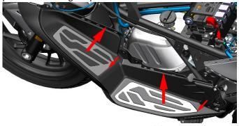
b. Remove the M6× 14 Shoulder bolt (1) at three places on the left pedal with the 4 # hexagonal socket. Remove the pedal together with the left surround.
