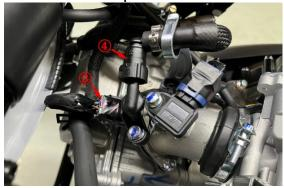
e.Locate and unplug the crankshaft position sensor plug 5, the magneto stator charging cable 6, and the water temperature sensor 7 in front of the tank on the right side of the frame.
