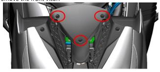
h. Press the center cylindrical pin of the 4 expansion nails with 4# Allen and remove the expansion nails. Remove the screws with a cross-cut (7). Remove the 2 M6×14 shoulder bolts (1) of the windshield with 4# Allen. Finally, remove the blue part of the picture together.
