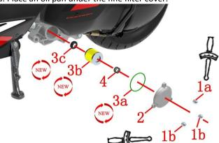
b. Use a 10# sleeve to loosen the 2 nuts (1b) at the bottom of the fine filter cover; use a 10# torx wrench to remove the upper nut (1c). Then remove the nut (1b) at the bottom.
