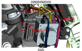
FMC-HU: Front disc brake main pump-hydraulic control unit FC-HU: Front disc brake caliper-hydraulic control unit RMC-HU: Rear disc brake main pump-hydraulic control unit RC-HU: Rear disc brake caliper-hydraulic control unit
