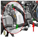
f. Reconnect the plugs of the stepper motor and the threein-one sensor on the throttle valve body; reconnect the
