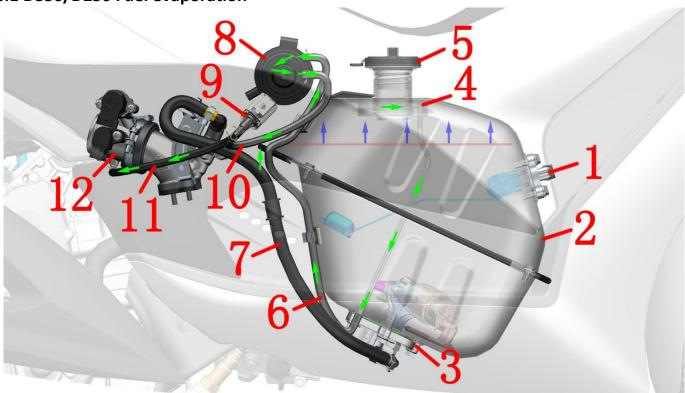
1- Fuel level sensor 2- Fuel tank 3- Fuel pump 4- Oil-air separator (welded inside the fuel tank) 5- Fuel tank cap 6- Adsorption/vent pipe 7-High pressure fuel pipe 8-Carbon tank 9-Carbon tank solenoid valve 10- Solenoid valve intake pipe 11-solenoid valve outlet pipe 12-throttle valve body assembly
