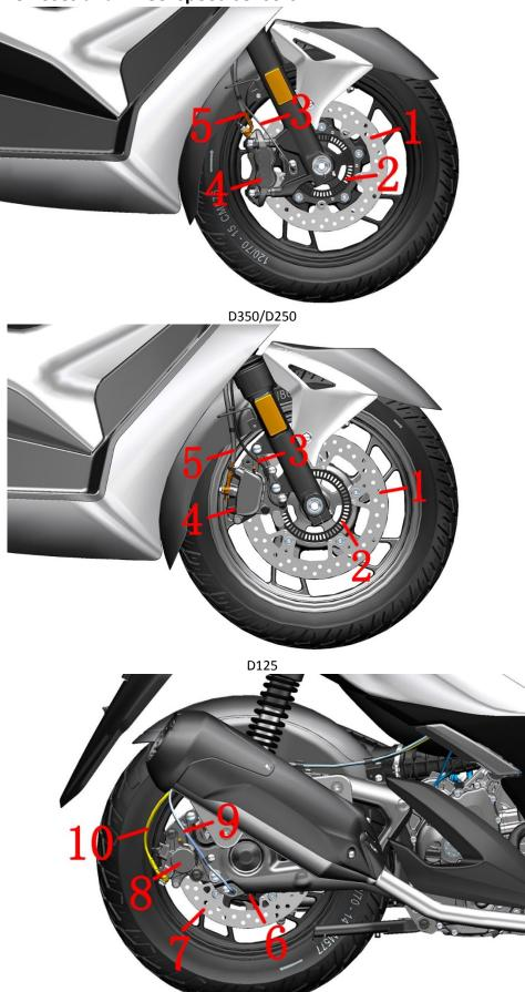
1-brake disc (front) 2- front whell ABS induction ring gear 3-wheel speed sensor (front wheel) 4-front disc brake caliper 5-FC-HU brake hose 6- rear whell ABS induction ring gear
