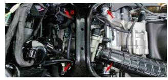
c. Check whether the engine nut is loose.
