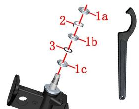
c. If the steering is heavy, loosen the adjusting nut (1c) counterclockwise. First screw it clockwise to 35N.m (3.6 kgf.m, 26 lbf.ft), then loosen 1/4 turn counterclockwise, and then screw it to D125:15N.m (1.5 kgf.m, 11 lbf.ft)/D125(2024):13N.m (1.3 kgf.m, 10 lbf.ft).
