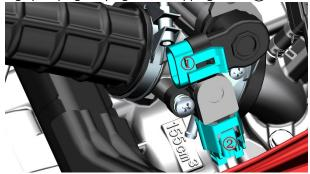
f. Use a short Phillips screwdriver to remove the 2 GB9074.4 M4×12bolts(3) and the anti-off card(4) that come with the throttle valve body assembly, and then remove the stepping motor.
