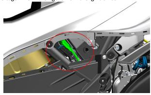
c. Press the arrow and pull out. Unplug the connector of ignition coil (5). Then use 8 # open-end wrench or ratchet wrench to remove the two bolts (4). Replace ignition coil.
