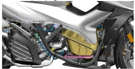
b.Use a dust blow gun to blow away the dust and debris near the spark plug.
