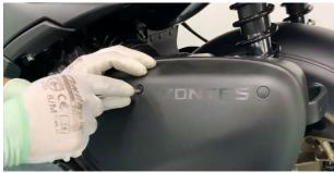
b. Use a Phillips screwdriver to remove the 2 screws.
