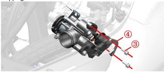
g. Use throttle cleaner to clean the carbon deposits on the head of the stepper motor. Spray a small amount of cleaning agent into the valve body hole. It is forbidden to soak the stepper motor with any liquid.
