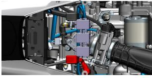
b. Unplug the fuel pump and start the engine to idle until the engine stops. Turn the engine stop switch to "", power off the vehicle and lock the vehicle. After putting on waterproof and oil-proof gloves, press the anti-trip lock and pull out the high-pressure oil pipe in the direction of the arrow.
