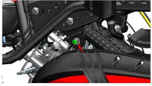
e. Install the rear pedal on the right side of the vehicle to a suitable position, install two M8×25 bolts, and tighten them with a 14# sleeve; connect the small water tank inlet pipe to the corresponding pipeline, and tighten it with a single batch Clamp; then connect the engine water inlet pipe back to the corresponding pipe, and use the water clamp clamp to fix the clamp to the appropriate position to prevent leakage of coolant.
