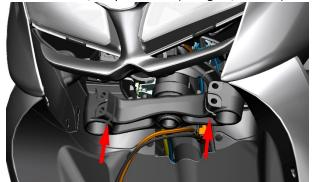
b. Use the same method to install another shock absorber. c. Pick up the front wheel and install the bushing, align the mounting holes between the two shock absorbers, penetrate the front wheel axle, and tighten the front wheel axle with a 17# inner hexagon. Torque: 50N.m (5.1 kgf.m, 37 lbf.ft). If one of the shock absorbers is not installed in place, the front axle will not be tightened or can not be inserted into the right
