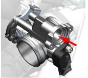
g. Install the stepper motor back to the valve body, paying attention not to miss the sealing ring. Plug the plug back in.
