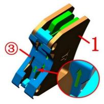
g. Press the blade pointed by the arrow (10) inward in the direction of the arrow with your hand, and insert the pin (2) into the hole to secure the brake pad (1). Tighten the pin shaft with a T25 Allen torx wrench (2).
