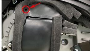
b. Use 4# inner hexagon to remove the 3 M6 $\times$ 14 bolts as shown in the figure.
