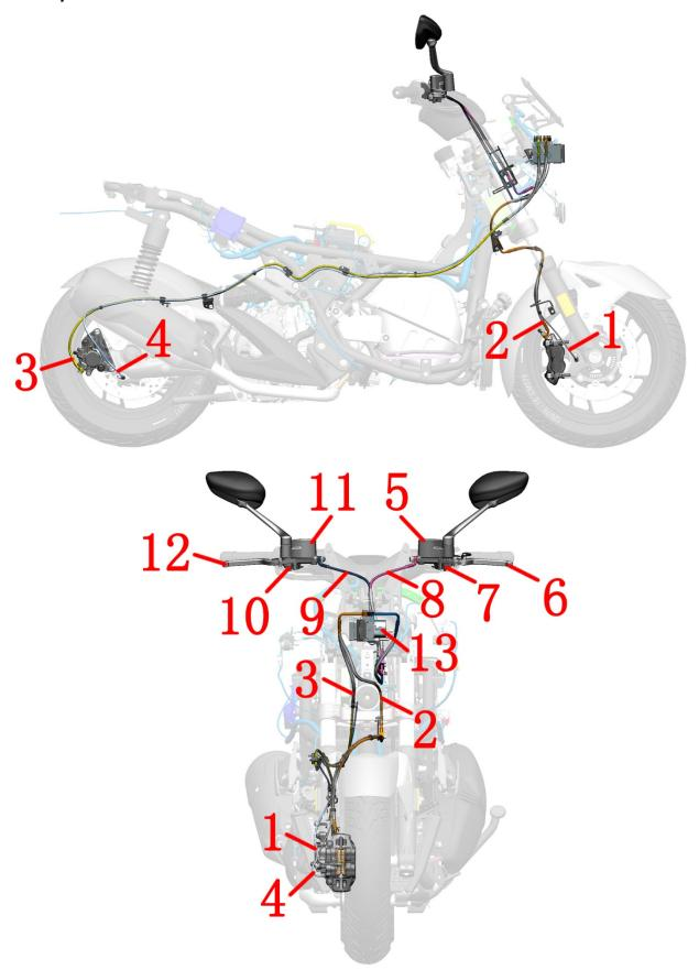
1-wheel speed sensor (front wheel) 2-FC-HU brake hose 3-RC-HU brake hose 4-wheel speed sensor (rear wheel) 5- rear disc brake main pump 6- rear brake lever 7- rear brake switch 8- RMC -HU brake hose 9-FMC-HU brake hose 10-front brake switch 11-front disc brake main pump 12-front brake handle 13-hydraulic control unit
