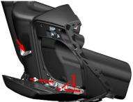
b. Take down the circlip with pointed nose pliers and pull out the rotary shaft. Remove the torsion spring and damping. Pay attention to the position of the torsion spring during installation.
