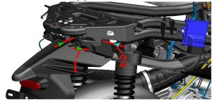
b. Find and remove the connectors of the rear license plate lamp, left turn light lamp and rectifier from the rubber sleeve on the left side of the frame.
