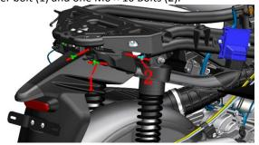
c.Production of vehicles by September 2023: Remove 2 bolts from the bottom with 8 # short socket, and then pull the rectifier and rear fender assembly down for a certain distance to facilitate the extraction of rectifier cable.
