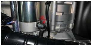
i. Locate and unplug the plug of the cylinder head water temperature sensor (10) on the right side of the throttle valve body.
