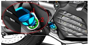
e. Wipe clean the oil dipstick, and turn the oil dipstick(1) and O-ring(2) clockwise by hand to replace the right crankcase cover of the engine.
