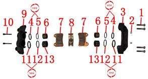
1- Bolt 2- Circlip 3- Inner side caliper housing 4- $\phi$ 30 oil seal 5- $\phi$ 30 dust seal 6- $\phi$ 30 piston 7- Disc brake pad 8- brake spring 9- Out side caliper housing 10-Pin 11- $\phi$ 34 oil seal 12- $\phi$ 34 dust seal 13- $\phi$ 34 piston
