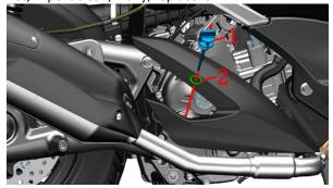
e. Wipe clean the oil dipstick, and turn the oil dipstick(1) and O-ring(2) clockwise by hand to replace the right crankcase cover of the engine.
