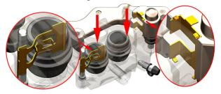
d. Take out the new brake pad and install it back. You need to hold the bottom of the brake pad (through hole end) with your hand. Be careful not to install it backwards, the side with 3 grooves faces the brake disc; the black metal back plate faces the caliper.
