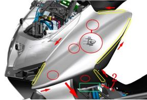
c. Use the same method to remove the front right panel.
