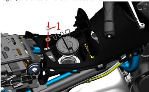
b. Grasp the mark (green rectangle) on the middle cover of the fuel tank and pull it out in the direction of the arrow until the mushroom button (red circle) on the middle cover of the fuel tank is pulled out.
