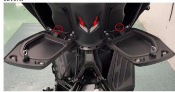
b. Turn the steering handle to the left and remove M8 with 6 # hexagonal socket × 35 bolts (6). Using the same method, turn the steering handle to the right and remove the bolt (6). Pry the gap on the upper connecting plate with a screwdriver.
