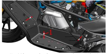
c. Use 4 # hexagonal socket to remove the two M6 $\times$  14 Shoulder bolt (1) parts on the left of the middle part of the enclosure.
