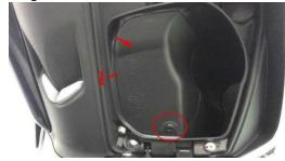
Open the rubber plug and insert it into the original standard charger DC plug. Then plug the AC socket into the 110-220V power supply. The battery damage caused by using inferior charger is not included in Three Replacement Policy.
