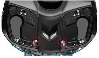
b. Find and unplug the front left storage box lock connector and front storage box switch on the front storage box next to the tap lock on the left side of the front storage box panel.
