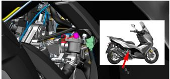
c. Put on waterproof gloves and add coolant to the water inlet of the Radiator with the help of an extended funnel. Until the position of the vent bolt of the thermostat is stably overflowed with coolant, the coolant level can be seen at the water filling port.
