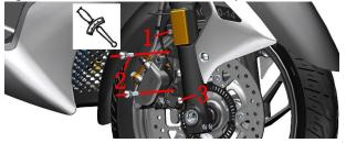
c. Use 4# inner hexagon to remove the two M6×14 bolts( $^4$ ) on the left and right sides of the front fender; then use 5# inner hexagon to remove one M6×30 bolt( $^1$ ), take out the gasket( $^5$ ).
