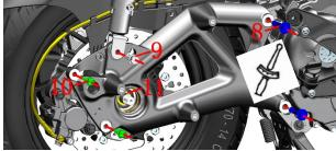
f. Remove the shaft sleeve (12) and take off the rear wheel assembly.
