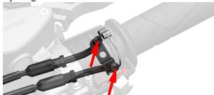
c. If the problem with high resistance cannot be solved after lubrication, the throttle cable needs to be replaced.
