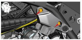
b. One person uses a 17# torx wrench to insert a M12 nut that fixes the engine on the left side of the vehicle from the front of the air filter, and another person uses a 15# sleeve to remove a M12×1.25×290 bolt that fixes the engine on the right side of the vehicle, pull out the bolt from the frame.
