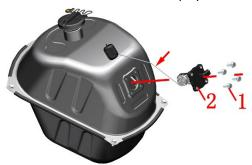
When reassembling, you need to pre-tighten the corners and then tighten the 4 M6 $\times$ 16 bolts. Otherwise, the uneven compression of the sealing rubber ring of the oil level sensor may cause leakage and cause safety hazards.
