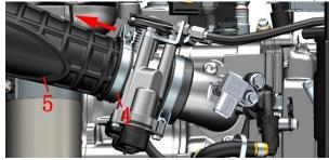
e. Use 5# inner hexagon to remove 2 bolts(6) and then remove the valve body assembly from the engine.
