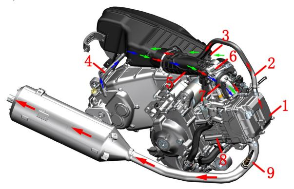
1- Cylinder head 2- Cylinder head exhaust pipe 3- Air filter intake inlet 4- Crankshaft Box exhaust pipe 5- Air filter outlet pipe 6- Throttle valve body assembly 7- Intake manifold 8- Cylinder 9- Muffler Intake system (indicated by the green arrow):
