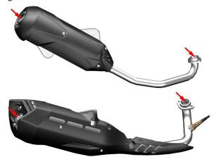
b. If there is no sign of air leakage, use 6# inner hexagon to check whether the M8 nut at the exhaust port of the engine is loose.
