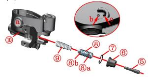
(5) Piston push rod (6) dust cap (7) retainer ring (8) piston assembly (18) a outer seal ring (8) b inner seal ring (9) spring (10) main pump housing
