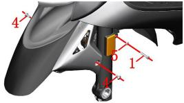
d.First press the two sides of the front mud board according to the small arrow, press the protrusion on the front mud board arrow inward, and then move the front mud board up to a suitable position and then pull it out in the direction of the big arrow.
