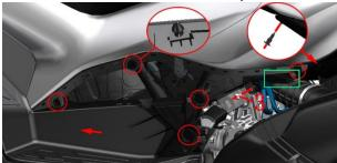
d. Remove two expansion nails and two bolts (5) at the connection between the left and right part of the fuel tank cover plate and the tail group respectively with 4 # socket head and 8 # sleeve, and remove the bushing (6) and buffer
