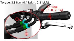
b. If the above adjustment fails to achieve the desired effect, please refer to the description in "Remove the throttle valve body assembly to clean up carbon deposits" to remove the throttle valve body assembly. Use a 10# open-end wrench to loosen the 2 nuts on the bracket to adjust. Torque: 3.0 N.m (0.3 kgf.m, 2.2 lbf.ft).
