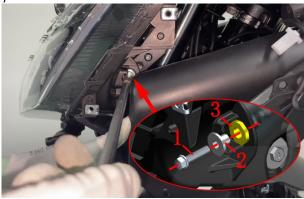
d. Hold the headlamp with one hand and take it out for a distance, pull out the headlamp plug with the other hand and take out the headlamp completely.
