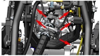
c. Check whether the engine nut is loose.
