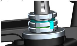
f. The front wheel is hung in the air to straighten the direction handle, and gently push and pull the direction handle by hand to feel whether the steering mechanism is smooth and free of jams. When the front fork assembly is slightly tilted to one side, it should be able to slowly deflect to the end under its own weight. If it is quickly to the end, it needs to be readjusted.
