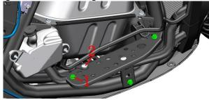
c. Press the anti-trip buckle of the plug of the oil level sensor and pull out the plug.
