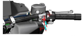
d. Tilt the front brake main pump so that the bolt(1) faces upward, wear waterproof gloves and use a 12# sleeve to remove the bolt(1), remove the copper pad(3), remove the FMC-HU oil pipe, and remove the brake fluid in the main pump. Pour out. Bolt(1) Standard torque: 32N.m (3.3kgf.m, 24 lbf.ft).
