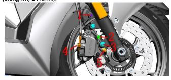
b. After wearing waterproof gloves, loosen the bolt(4) with a 12# sleeve, and turn the caliper upside down so that the head of the bolt(4) is facing down to drain the brake fluid into the oil pan. Remove the bolt(4) and the copper pad and then remove the FC-HU oil pipe. Refer to the brake fluid steps to remove the upper cover of the front disc brake main pump to speed up the discharge of brake fluid.
