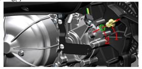
c. Use a 14# sleeve to loosen the oil drain bolt(3) counterclockwise, and remove the bolt(3) and copper pad(4).
