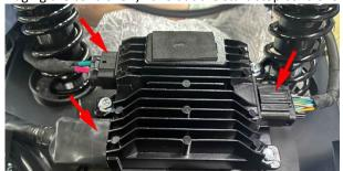
D155:After firmly removing the start-stop controller, remove two M6  $\,\times\,$  16 bolts and two bushings at the bottom with 10 # sleeve, and then remove the start-stop controller assembly.Remove 3 M6  $\,\times\,$  16 bolts with 10 # sleeve to separate the start-stop controller from the bracket.
