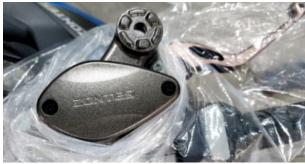
d. After wearing waterproof gloves, use a Phillips screwdriver to remove the bolt ①, and remove the upper cover ②, the cover ③, and the sealing rubber gasket ④.
