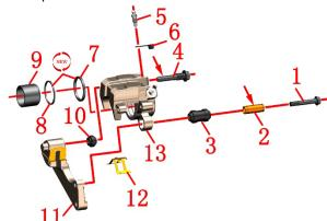
1- caliper mounting plate pin 2- bushing 3- rubber cap 4-caliper pin 5- vent nozzle 6-vent nozzle rubber cap 7-oil seal 8-dust seal 9-piston 10-caliper pin rubber cap 11- Caliper mounting plate 12- Brake pad spring 13- Caliper housing
