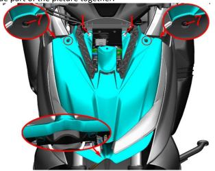
i. Remove the M6×14 shoulder bolt (1) of the left panel of the front with #14 Allen. Remove the M6×12 bolts (8) connecting the front left panel to the front left panel backing with 4# Allen. Press the center cylindrical pin of the expansion nail with 4# Allen and remove the expansion nail. Remove the front panel.
