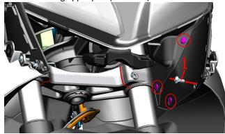
b. Remove 3 expansion nails (red circle) from the bottom lining of the left panel with 4 # hexagonal socket; Remove 2 bolts (1) and 2 bolts (4) from the bottom lining of the left panel with 4 # hexagonal socket, and remove the bushing (2) and buffer rubber (3).
