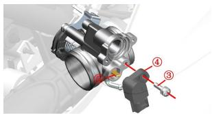
Simple test method: connect the whole vehicle to the diagnostic instrument, press the flameout switch (no need to ignite), turn the throttle handlebar from the initial position to full open, this process to see if the throttle position signal follows the change from 0 to 100.
