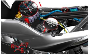
d. Press down the central cylindrical pin of 8 expansion nails with 4 # hexagonal socket, then take down the expansion nails, and take down the left and right parts, middle parts and left and right tail lights (blue part) of the rear tail group.
