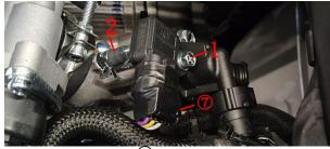
Loosen the connector 7 and check whether the pin is skewed or broken. The vehicle is connected to the diagnostic instrument without ignition. Check the engine parameters to see whether the pressure parameters are consistent with the local atmospheric pressure.
