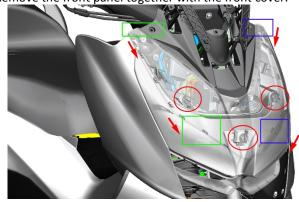
c. Remove 4 M6  $\times$  14 from the front cover plate with 4 # socket head Shoulder bolt (1). Separate the front panel from the front cover.
