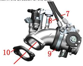
g. Use throttle valve body cleaning agent to clean the carbon deposits on the intake manifold and throttle valve body outlet respectively. It is forbidden to directly soak the throttle valve body assembly and intake manifold assembly with any liquid.
