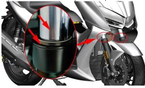
b. Check whether the bottom tube is painted off; whether the installation points of the front fender, the front wheel hollow shaft and the front brake caliper are broken or cracked. Check if there is any leakage at the bottom of the bottom cylinder.
