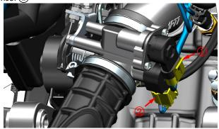
e. Use a short Phillips screwdriver to remove the 2 bolts 3 and the anti-off card 4 that come with the throttle valve body assembly, and then remove the stepping motor (4).
