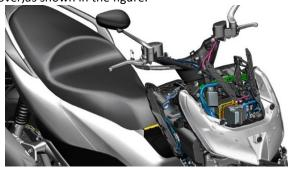
b. Untie the binding band, and then take out the handle switch harness and brake hose in the steering handle clamp from the notch of the steering handle clamp one by one until all harnesses in the steering handle clamp are removed.
