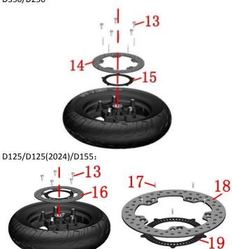
h.Refer to the order of disassembly to restore. Note that bolts with torque requirements need to be calibrated according to standard values.
