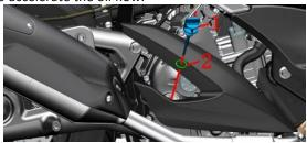
d. After placing an oil pan under the oil drain bolt, use a 14# sleeve to remove the oil drain bolt(3) and the combined seal gasket(4).
