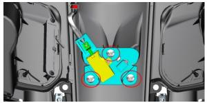
f. Remove 2 expansion nails with 4 # hexagonal socket, and remove the left and right cover plates of the storage box. Use a cross screwdriver to remove the two cross tapping screws on the front left storage box cover, and remove the non inductive antenna. Remove the 2 front left storage box rear glues. Loosen the plastic nut pointed by the arrow, take out the USB charging cable, and remove the matching charging port rubber sleeve.
