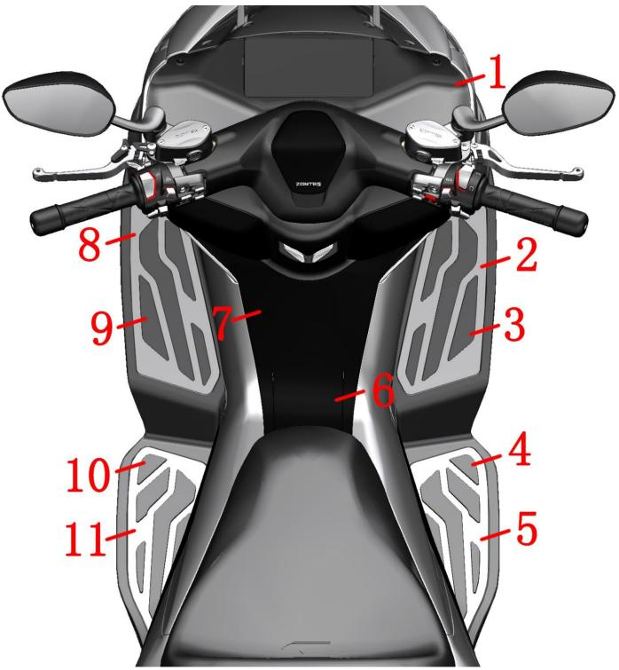
1.Instrument panel 2.Front right pedal pad pressure plate 3.Front right pedal pad 4.Rear right pedal pad 5.Rear right pedal pad presser 6.Fuel tank cover 7.Middle part of the fuel tank cover 8.Front left pedal pad pressure plate 9.Front left pedal rubber pad 10.Rear left pedal rubber pad 11.Rear left pedal pad presser
