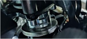
b. For the convenience of explanation, other parts are hidden here. First use a 38-42 hook wrench with a thickness of 6mm (0.24 in) to loosen the adjusting nut (1a); move the lock washer(2) up and then loosen the adjusting nut (1b).
