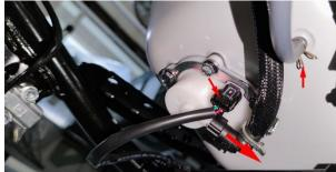
e. Use needle-nose pliers to slightly clamp the cable tie and push it up to remove it from the bracket.
