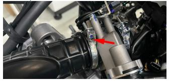
d. Pull the air outlet pipe to the right side of the vehicle to expose the two M6×30 bolts that fix the starter motor, and remove them with an 8# sleeve. After removing the bolts, remove the starter motor from the engine in the direction indicated by the big arrow.
