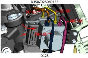
c. Remove the 2 bolts that were put back in the front (1) Remove the hydraulic control unit and bracket assembly from the car.
