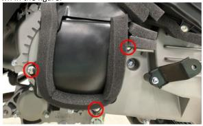
c. Remove the air inlet cover and the air inlet filter element together. Remove the rubber strip on the box.
