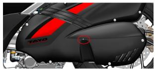
b. Use 4# inner hexagon to remove the 4 M6×14 bolts as shown in the figure.
