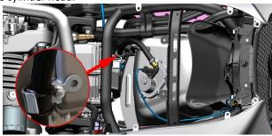
g. Pull out the high-pressure oil pipe in the direction of the arrow after pressing down the anti-dropping lock.
