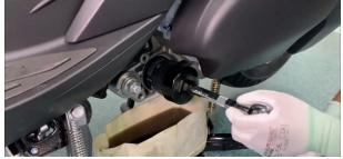
c. Drain the oil inside the fine filter.
