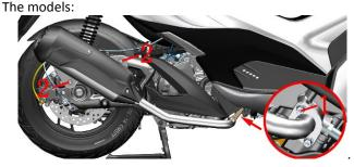
b. Remove the rubber cover then one person pinches the rear brake handle, and one person uses 21# sleeve + impact wrench to remove the rear wheel nut(3). Standard torque of nut(3): 125N.m (12.8 kgf.m, 92 lbf.ft).
