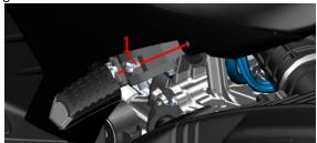
b. Pull out in sequence in the direction of the arrow (from the rear wheel to the front wheel). Note that there are 5 staples at the red circle and a circle of buckles around. It takes a lot of force to pull out.
