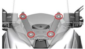
b. Use 4# inner hexagon to loosen the 4 M6×14 bolts on the left and right decorative covers of the windshield.
