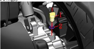
b. Use a 14# sleeve to loosen the oil drain bolt(3) counterclockwise.
