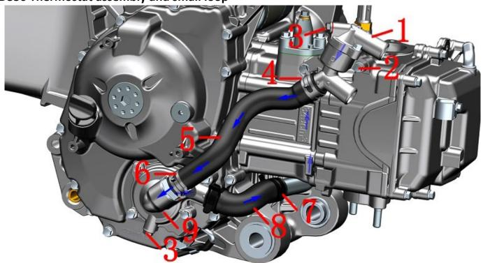
1-Thermostat assembly 2-M6  $\times$  22 Bolt \* 2 3-M6  $\times$  12 bolts \* 2 4-water pipe hoop (  $\Phi$  25) 5 - Water pump cover inlet pipe 6 - Water pipe hoop (  $\Phi$  24) 7-Water pipe hoop (  $\Phi$  26) \* 2 8-Water pump cover outlet pipe 9-Water pump cover assembly
