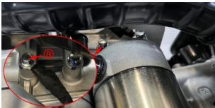
h. Use an 8# sleeve to remove a bolt on the starter motor, and take out the positive wire (9) on the bolt.
