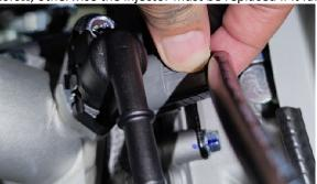
If you need to replace the fuel injector, wait until the engine and muffler have cooled down. After placing the oil container at the bottom, refer to the steps for removing the high-pressure oil pipe to pull out the high-pressure oil pipe at the end of the fuel pump to discharge the remaining fuel. Use a 10# sleeve to remove the bolt(1), remove the injector holder(2), and then take off the injector(3).
