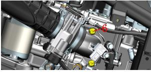
f. Remove the heat insulation pad and O-ring assembly, and remove the O-ring(10). Use a 4# inner hexagon to loosen the clamp(9) and separate the intake manifold from the valve body assembly. Use 2 10# open-end wrenches to loosen the two nuts of the fuel line(8) and then pull them out to remove them from the bracket; take out the cylinder end of the throttle line from the turntable. After the two nuts of the oil return line(7) are loosened, completely loosen the nut
