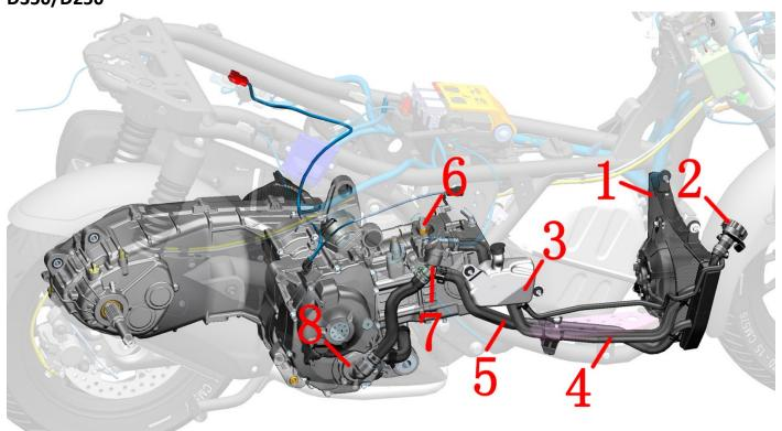
1 - Main water tank 2 - Water tank filler 3 - Auxiliary water tank 4 - Water inlet pipe of main water tank 5 - Water outlet pipe of main water tank 6 - Water oil shared sensor 7 - Thermostat 8 - Water pump cover assembly
