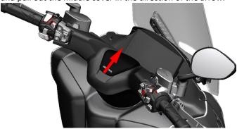
b. Use a cross screw to remove the two self-tapping ST3.9  $\times$  12 screws at the lower cover, and use a straight screw to pry off the buckles at (1) and (2).
