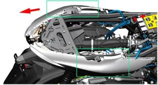
d. Remove the three non-standard M6× 14 Shoulder bolt (4) connecting the left part of the tail skirt and the left tail lamp with the 4 # hexagonal socket and an expansion nail; Use the 4 # hexagonal socket to remove the 2 M6× 12 Bolts (1) connecting the left part of the tail skirt and the middle part of the tail skirt, remove one bushing (2) and one buffer rubber (3). Take off the left part of the tail skirt.
