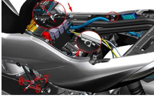
e. Remove the 3 expansion pins connecting the left and middle of the tail skirt using a 4# inner hexagon.
