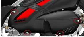
c. Pull out the front part of the left engine cover first and then move it about 30mm (1.2 in) in the direction of the rear mudguard to remove it. The bolts removed in the second step will fall off at this time.
