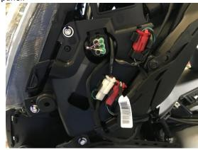
c. Find and unplug the PKE connector of PKE on the right side of the front storage box panel, and find and unplug the OBD connector on the left side of the front storage box panel. Remove the front storage box panel.
