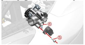
Connect the diagnostic instrument to the whole vehicle, press the flameout switch (without ignition), turn the throttle handle from the initial position to fully open, and check whether the throttle position signal changes from 0 to 100. e. Check whether the external intake pressure sensor is damaged
