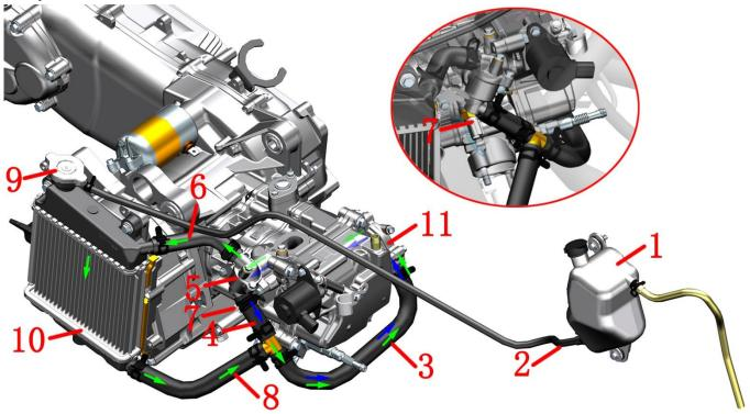
1- Secondary water tank 2-Secondary water tank link pipe 3-Engine inlet pipe 4- Thermostat outlet pipe 5- Thermostat 6- Water tank inlet pipe 7- Water and oil shared sensor 8- Water tank outlet pipe 9- Water tank filling port 10- Radiator assembly 11- Water pump cover assembly
