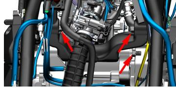
c. Check whether the engine nut is loose.
