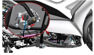
f. Pull out the high-pressure oil pipe from the bracket at the cylinder head.
