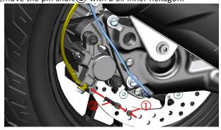
b. Use a 12# sleeve to remove the bolt ③, turn the caliper assembly clockwise around the bolt ④, and remove the brake pad. Note that the bolt ④ does not need to be disassembled.
