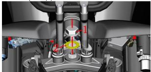
b. Other components are omitted here for ease of explanation. Move the washer (3) upwards and loosen the adjusting nut (4A) with a 38-42 hook wrench within 6mm (0.24 in); Finally loosen the adjusting nut (4b). Pull out the directional handle and uplink plate assembly. If it is difficult to pull out, you can use a flat screwdriver to pry the upper plate slotted slightly and then pull it out at the same time. Move the orientation handle and the uplink plate assembly away and place it.
