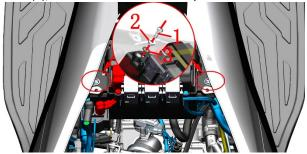
b. Remove the left cover according to the section "Maintenance - Remove Spark Plug". Unplug the high-voltage wire in the figure from the ignition coil.
