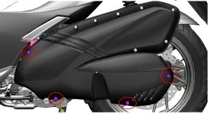
d. Remove the front part of the left engine cover. The bolts removed in the second step will fall off at this time.
