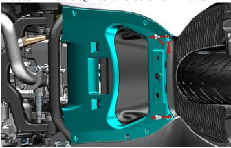
d. Pull down the surrounding bottom plate in the center of the front part (near the front wheel) with one hand, and pull down the surrounding bottom plate after pulling about 20mm (0.8 in) toward the rear wheel with the other hand. There is a bracket at the place shown in the small picture, so it cannot be pulled down directly.
