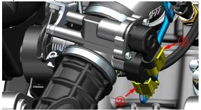
d. Locate and unplug the plugs of the high-pressure fuel pipe 3 and the fuel injector 4 at the front end of the throttle valve.
