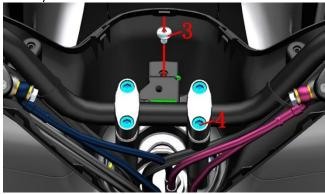
c. Use 5# inner hexagon to remove the bolts (5a) and (5b) that come with the right-hand handle under the switch, and then use the cross-batch to remove the bolts (5c), and separate the upper and lower parts of the right-hand handle.
