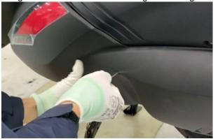
f. Before installing other bolts, install the exposed sponge and plug it back into the left cover.
