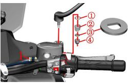
c. After grasping the front brake main pump, remove the 2 bolts (2) with a 5# inner hexagon, and remove the right auxiliary switch.
