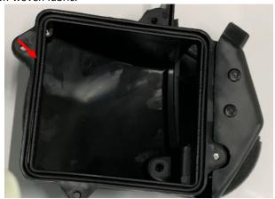
b. Replace with 2 new rubber strips (one is installed in the air inlet cover, the other is installed in the box). Take out the new air inlet filter element and install it into the air inlet cover in the direction shown.
