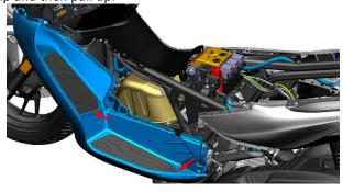
k. Respectively use 4# inner hexagon to remove the 3 M6  $\times$  14 bolts at the front pedal.
