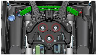
d. Remove 2 circlips with pointed nose pliers, grasp the left windshield bracket, take down the pin shaft and buffer rubber, and take down the rocker arm spring. Remove the right windshield and rocker spring in the same way.
