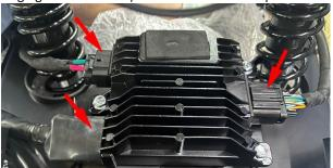
b.After firmly removing the start-stop controller, remove two M6  $\times$  16 bolts and two bushings at the bottom with 10 # sleeve, and then remove the start-stop controller assembly.Remove 3 M6  $\times$  16 bolts with 10 # sleeve to separate the start-stop controller from the bracket.
