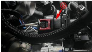
g. Locate and unplug the tube connecting the throttle valve body to the canister from the lower part of the throttle valve body
