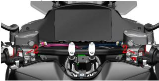
b. Use 4# inner hexagon to remove the M6×14 bolt(3); then use 6# inner hexagon to remove 4 M8×35 bolts(4), remove 2 pressure blocks, and take out the direction handle assembly.
