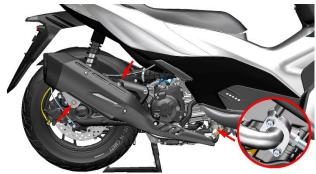
a. If there is a slight air leak, first try to tighten the exhaust port nut with 6# inner hexagon; if the problem is not solved, remove the muffler and replace with a new engine exhaust port gasket.
