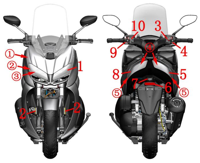
1 - Headlights ((1) - Front turn light position (2) - Position light / daytime running light position (3) - High and low beam position)
