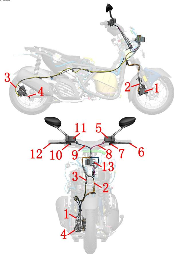
1-wheel speed sensor (front wheel) 2-FC-HU brake hose 3-RC-HU brake hose 4-wheel speed sensor (rear wheel) 5-rear brake lever 6-rear brake switch 7-RMC -HU brake hose 8-rear disc brake main pump 9-FMC-HU brake hose 10-front brake switch 11-front disc brake main pump 12-front brake handle 13-hydraulic control unit
