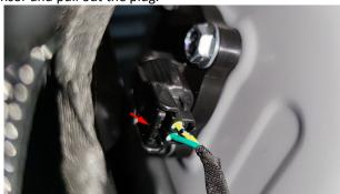
d. Remove the oil pump plug in the same way. Pinch the snorkel clamp and move it down, and pull out the snorkel. Press the anti-release buckle of the high-pressure oil pipe at the end of the oil pump, and pull the high-pressure oil pipe along the axis of the oil outlet of the oil pump.
