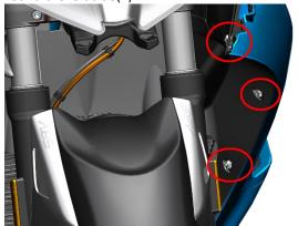
n. Use 4# inner hexagon to press down the center cylindrical pins of the 2 swell nails on the left, and then remove the swell nails. Remove the bolt on the left front part with a 4# inner hexagon For instructions on disassembly and assembly of swell nails, please refer to the pre-service instructions in this chapter
