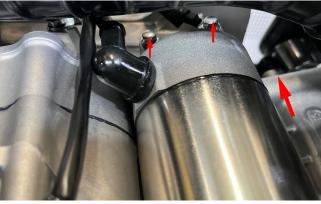
e. When reassembling, make sure not to omit the O ring that comes with the starter motor, and align the teeth of the electric starter reduction gear. Note that the O-ring needs to be correctly assembled into the box, as it will cause leakage if cut edges occur. Torque of the two bolts for fixing the starter motor: 12±1.5 N.m (1.2±0.2 kgf.m, 9±1 lbf.ft). And mark with a marker.
