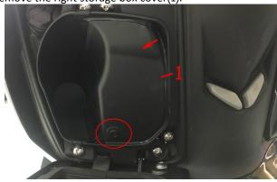
Pull out the OBD plug, connect the diagnostic tool to read the fault code. Different batches of OBD plugs may have different colors, including black and white, with the same functions. If the OBD plug has a protective cover, remove it first.
