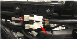
b. Check whether the plug is loose or corroded.
