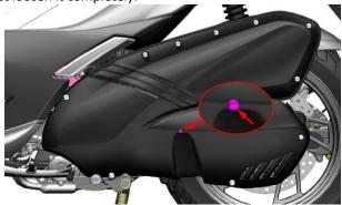
b. Use 4# inner hexagon to press down the center cylindrical pins of the 2 swell nails, and then remove the swell nails and the engine rear decorative cover.
