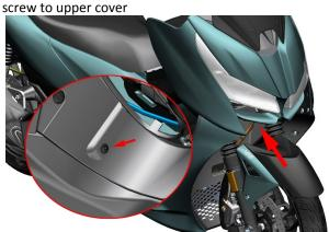
e. Remove the M6×22 bolts (4) of the rear compartment with a # sleeve, remove the bushing (5) and seating glue (6). Press the center cylindrical pin of the expansion nail on the left side of the tank cover plate with 4# Allen and remove the expansion nail. Finally, remove the left part of the fuel tank cover.
