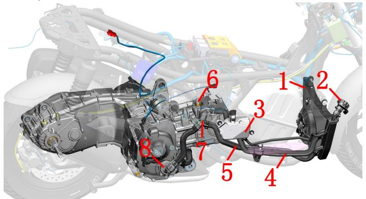
1-Main water tank 2- Water tank filling port 3- Secondary water tank 4- Main water tank water inlet pipe 5- Main water tank water outlet pipe 6- Water and oil shared sensor 7- Thermostat 8- Water pump cover assembly
