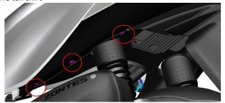
b. Use the 4 # hexagonal socket to remove the 3 expansion nails (purple) connecting the right apron and the middle of the tail group.
