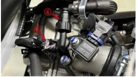
e. Find and pull off the crankshaft position sensor plug ⑤ at the right inner side of the frame, and find and pull off the oxygen sensor plug ⑥ under the right foot bracket
