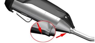
•Clean up the dirt, dirt and other stains on the surface of the muffler in time.
