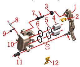
1- Caliper mounting plate 2- Brake pad holder 3- Caliper pin rubber cap 4- Piston 5-dust seal 6-oil seal 7-caliper pin 8bleed nozzle 9-bleed nozzle rubber cap 10-caliper housing 11-caliper mounting plate pin rubber cap 12-brake spring
