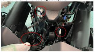
d. Turn to the back and pull the cable out of the lock frame in the direction of the arrow. Turn back the front and remove M6× 14 with 4 # hexagonal socket bolts. At the same time, grasp the right storage box lock assembly 1 and the electronic front storage box lock assembly 2 on the back.
