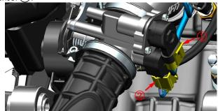
b. Place the small container under the high-pressure oil pipe, press the buckle indicated by (3) and pull out the high-pressure oil pipe(1) in the direction of the arrow at the same time. A small amount of fuel will flow out when it is pulled out, and it is forbidden to drip onto the surface of the part.
