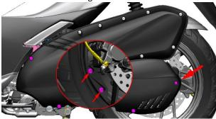
c. Use 4# inner hexagon to remove the 4 pcs Hexagon socket head screw M6×14 bolts as shown in the figure.
