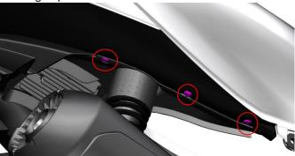
c. Grasp both sides of the tail skirt and pull out the left and right tail skirts together with the left and right tail lamps and the middle of the tail skirt in the direction of the arrow. Note: Pull out carefully to avoid scratching the cover and tail lamp.
