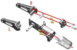
g. Remove M8× 16 Bolts with 6 # hexagonal socket, remove the gasket, bearing and upper rocker arm.
