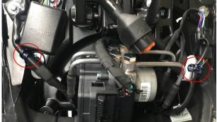
c. Push the storage box away slightly, use 8 # socket to remove the bolt (1), and remove the bushing (2) and buffer rubber (3). Remove the bolts on the other side in the same way.
