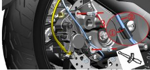
g. Pull out the rear caliper assembly and check the wear of the brake pads. If it is nearly worn or worn to the limit position, new brake pads must be replaced in pairs.
