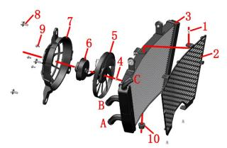
1 - Water tank front cover screw \* 3 2 - Water tank front cover 3 - Water tank 4 - Fan sheet nut 5 - Fan sheet 6 - Fan motor 7 - Fan cover 8 - Fan cover bolt \* 3 9 - Fan motor bolt \* 3 10 - Buffer rubber
