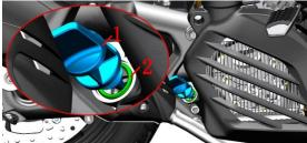
d. After placing an oil pan under the oil drain bolt, use a 14# sleeve to remove the oil drain bolt(3) and the combined seal gasket(4). Use a 24# sleeve to remove the strainer cover (5) at the bottom, take off the 34.5×3.5 acrylate rubber Oring(6), the  $\varphi$ 25.8×34.2×1.8 strainer spring(7) and the outer diameter  $\varphi$ 22×21 cap-shaped strainer(8). Drain the oil from the crankcase.
