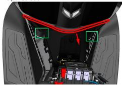
c. Find and unplug the fuel tank lock connector from the left side of the fuel tank, and sort out the harness of the fuel tank lock.
