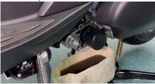
b. Remove the fine filter using a 14-side, 65mm cap filter wrench +1/2" (12.5mm) ratchet wrench counterclockwise. The filter wrench has a Skadden model 97401. Replacement every 1,000 km or 3 months (whichever comes first) and every 8,000 km or 30 months (whichever comes first).
