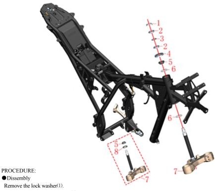
Remove the top adjusting nut (2) by using a hook wrench tools.
