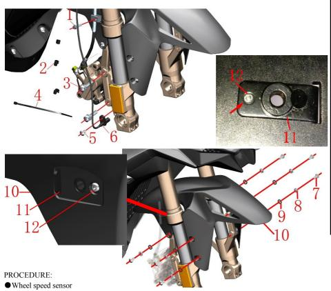
Pull out the plug of the wheel speed sensor(6); then remove the clamp(2). Cut the tie (4); remove the bolt (3) and remove the sensor(6).
