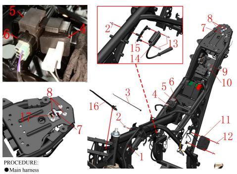
Different plug-in methods are different, please unplug all the electrical components connected to the main thread according to the actual operation. It needs to use a word screwdriver, forceps, scissors and other tools to assist. The binding(3) and (16)can be picked out by using scissors.
