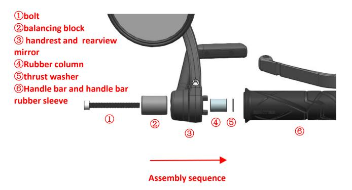
Note: The quantity of thrust washers (5) has been matched and screwed on the handle with bolt (1). When assembling, please make sure not to install the wrong quantity gaskets (5), The rubber column (4) is recommended to be replaced every two years (If the handle bar vibration becomes large during use, it can be replaced in advance); Bolt tightening torque is 3-4N, the torque should not be too large, otherwise it will affect the vibration of the handle bar.
