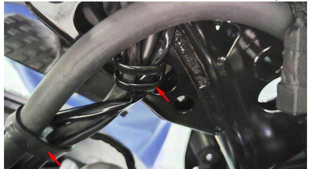
c. Loosen the clamp bolt shown in the figure with a 4# inner hexagon counterclockwise, and pull the air filter
