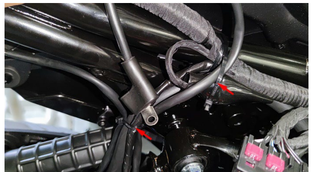
M125 loosen the rubber buckle and the wire clamp.
