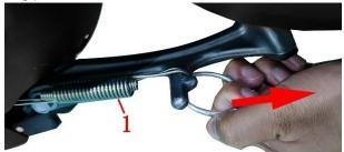
C. Grasp the side bracket with one hand, and pull it in the direction of the arrow with the other hand to remove the spring.
