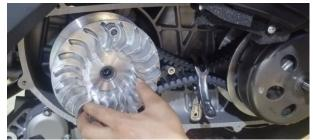
g. Put the  $\varphi$ 12.3× $\varphi$ 40×4 washer on the M12×1.25×35 hexagon flange bolt, and then screw the M12×1.25×35 hexagon flange bolt into the crankshaft threaded hole.
