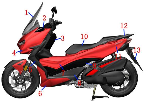
1. Windshield 2.Left front turn light 3. Left cover front storage box 4. Front left panel 5. Front storage box panel left decorative cover 6. Left pedal decorative cover 7.Left fuel tank cover plate 8. Left pedal 9. Left side cover 10. Cushion 11. Tail skirt left part 12. Rear rack 13. Rear mudguard
