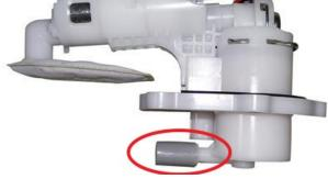
When reassembling, you need to pre-tighten diagonally and then tighten the 5 bolts. Otherwise, the uneven compression of the seal rubber ring of the fuel pump may cause leakage and cause safety hazards. **4. Carbon canister solenoid valve**
