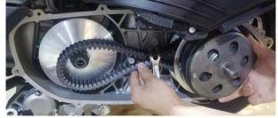
f. Put the side of the driving wheel drive disc with the wind blades facing outwards, align the spline holes in the middle with the splines on the crankshaft, and then assemble it on the crankshaft and assemble it in place.
