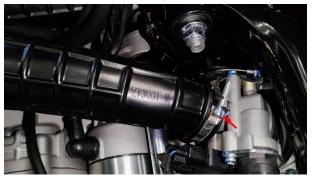
d. Pull the air outlet pipe to the right side of the vehicle to expose the two M6×30 bolts that fix the starter motor, and remove them with an 8# sleeve.
