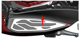
b. Remove 5 non-standard M6x16 bolts<sup>(5)</sup> on the left pedal with 5# inner hexagon, and remove bushing<sup>(2)</sup>and buffer glue<sup>(3)</sup>. **Caution:** one of them is only with bushing, without buffer glue.
