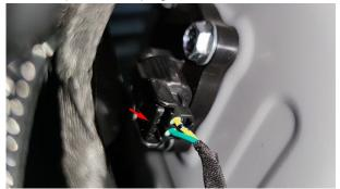
d. Remove the oil pump plug in the same way. Pinch the snorkel clamp and move it down, and pull out the snorkel. Press the anti-release buckle of the highpressure oil pipe at the end of the oil pump, and pull the high-pressure oil pipe along the axis of the oil outlet of the oil pump.
