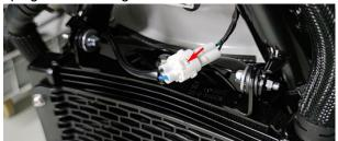
d. Use an 8# sleeve to remove the 3 M6×22 bolts (1) shown in the figure.
