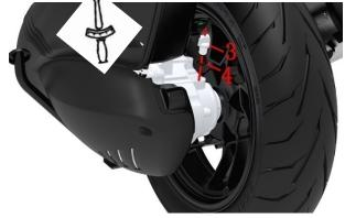
c. Remove the oil drain bolt (1) and the copper pad (2).
