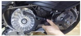
j. Tighten the M12×1.25×35 hexagon flange bolts clockwise with a torque wrench (or wind batch) and a 17# sleeve. The tightening torque must reach 103±10N.m (10.5±1 kgf.m, 76±7). lbf.ft) range. Then tighten the M14×1 hexagonal flange nut clockwise with a torque wrench (or wind batch) and a 19# sleeve. The tightening torque must reach 75±7N.m (7.65±0.7 kgf.m, 55±5 lbf.ft) )scope.
