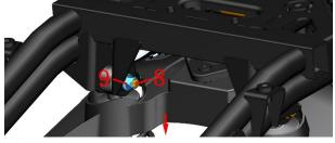
f. Grasp the rear right shock absorber and use a 12# sleeve to remove the bolt (10), and remove the rear right shock absorber. On the left side, pull the air filter out to expose the bolt head and then remove the bolt (10). Standard torque: 24N.m (2.4 kgf.m, 18 lbf.ft).
