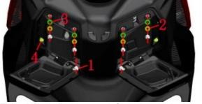
c. Extend the 10# torx wrench from the gap in the storage box, remove the two M6×20 bolts on the faucet lock support (5), remove the faucet lock and faucet lock support, no need to connect the faucet lock and the faucet Remove the lock and put it in a suitable place next to it.
