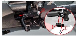
The replacement procedure of the front brake switch is the same as that of the rear brake switch. The throttle cable needs to be removed to facilitate the removal of the bolt 1.
