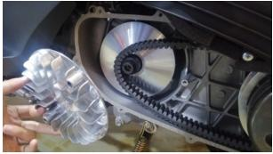
f. Remove the driven wheel clutch cover from the drive shaft.
