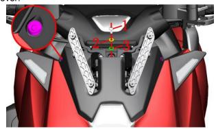
b. Raise the windshield rocker arm to the highest position, then grab the mark on the front cover (green rectangle) with your hand, and pull it up in the direction of the small arrow; pull out the two mushroom buttons (blue circles) on the front cover After exiting; continue to grasp the mark on the front cover (green rectangle) and pull it diagonally upward according to the big arrow until the 6 buckles on both sides of the front cover (yellow area, 3 on the left and right) are all pulled out.
