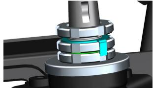
f. The front wheel is hung in the air to straighten the direction handle, and gently push and pull the direction handle by hand to feel whether the steering mechanism is smooth and free of jams. When the front fork assembly is slightly tilted to one side, it should be able to slowly deflect to the end under its own weight. If it is quickly to the end, it needs to be readjusted.
