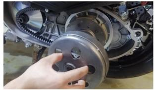
g. Pinch the middle part of the V-shaped drive belt, and remove the belt and the driven pulley pulley together.
