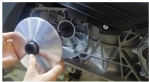
i. Finally, take out the  $\varphi$ 23.2× $\varphi$ 40×3.25 washer, then have completed the disassembly of the continuously variable clutch sub-assembly.
