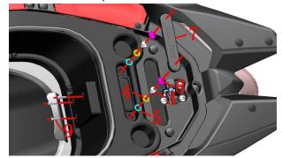
j. Remove the decorative buckle (8) of the M6 hexagon socket bolt; remove the bolts on both sides with 4# hex socket (3), remove the bushing (4) and the cushion rubber (5).
