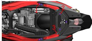
c. Use 4# inner hexagon to remove 2 bolts (4); after grasping the rear armrest, use 12# sleeve to remove 5 bolts (5), and then take off the rear armrest assembly.
