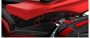
c. Use your fingers or a plastic crowbar to insert the arrow indication point, first pry the arrow indication point open the gap and then pull up.
