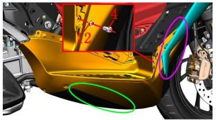
b. Fasten the buckle on the front of the right pedal decoration cover (the blue mark) into the corresponding position, and then use the 4# inner hexagon to install the right pedal decoration cover (gold) to connect the two M6×16 bolts (1) surrounding the middle part, Pay attention to the bolt belt traversing the bushing (2), cushioning glue (3).
