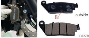
e. Observe from both sides whether the upper part of the brake pad has hit the shrapnel, otherwise the position needs to be readjusted.
