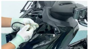
d. Remove the front right turning light by the same methods.
