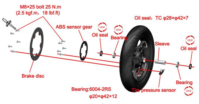
Inspection and maintenance of front wheel assembly: Caution:
