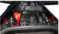
c. Take off 2 psc decorative buckle,then use 4# inner hexagons to remove 2 pcs M6x16 bolts(1), and take out the bushing(2) and buffer glue(3).
