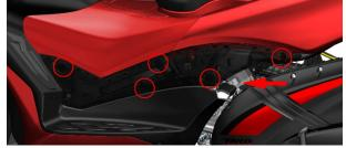
c. Use 5# inner hexagon to remove 2 bolts (4), take off the bushing (2) and cushion rubber (3). Starting from the bottom where the left cover plate of the fuel tank (5) and the tail skirt intersect, pull the left cover plate outward with one hand and press the front part of the tail skirt with the other hand; pull out the upper part of the left cover plate after pulling out the bottom. Then
