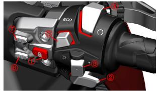
c. The left switch button test. If you need a more detailed understanding of each button function, you can check the driver's manual. Here is only a brief description of how to test whether it is normal. ①SET key: Short press SET to enter the main menu/confirm selection. Long press to return to the main interface. Operate this button when driving a vehicle is prohibited.
