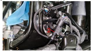
c. First remove the 3 pieces of wire clamp (4), and then pull out the wheel speed sensor (2) and the RC-HU hose from the 4 pieces of oil pipe clamp (3). If you need to remove the tubing clamp (3), you can use 4# inner hexagon to remove the bolts and then you can take it off.
