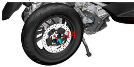
g. Remove bolts (15) with 6# inner hexagon respectively, and then take off the brake disc (16). If you need to replace the ABS gear ring, remove the bolt (15) and then replace it. Bolt (15) standard torque: 25N.m (2.6 kgf.m, 18 lbf.ft).
