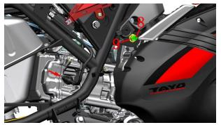
e. Install the rear pedal on the right side of the vehicle to a suitable position, install two M8×25 bolts (7), and tighten them with a 14# sleeve; connect the small water tank inlet pipe to the corresponding pipeline, and tighten it with a single batch Clamp; then connect the engine water inlet pipe back to the corresponding pipe, and use the water clamp clamp to fix the clamp to the appropriate position to prevent leakage of coolant.
