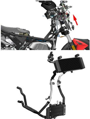
j. If you need to remove the water filler fixing bracket, you can use an 8# sleeve to remove the bolt (12). Grasp the bracket (13) and use an 8# sleeve to remove the bolt (1), and remove the lower mounting bracket (13) of the main water tank.
