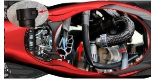
c. Connect the high-pressure oil pipe of the original car to the pressure gauge, and find another highpressure oil pipe to connect the pressure gauge and the fuel injector.
