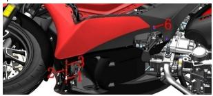
j. Press the blue part inward at the junction of green and blue as shown in the figure; pull the red and green components outward. Then apply force from the rear wheel to the front wheel along the junction of the red and blue parts, push the red part outwards, and force the blue parts inward to break apart. Remove the left pedal and left pedal trim cover assembly.
