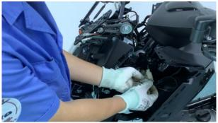
c. Find out and unplug the PKE bullet connector, PKE connector, and PKE antenna connector on the right side of the front storage box panel.
