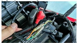
When re installing, the yellow/red and green/red wires of the relay correspond to the color of the main cable, and the nuts are not distinguished. Be sure to close the protective cap after tightening the nut.
