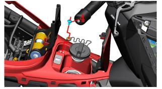
c. Find out and unplug the tank lock connector under the cushion stand and make the tank lock wire harness well.
