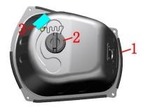
Use a multimeter to measure the voltage of the fuel pump plug cable end, unlock the vehicle, and when the engine stop switch is turned to "", the fuel pump will accumulate pressure for about 5 seconds, during which time the battery voltage should be able to be measured.
