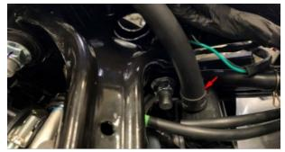
I. Use a 4# inner hexagon to remove one M6×12 bolt (5) that fixes the wheel speed sensor on the rear rocker arm, take out the wheel speed sensor and take it out of the fixed clamp. Then use a 14# sleeve to remove the two M8×37 bolts (6) that fix the brake caliper, and pass the brake caliper and wheel speed sensor in the direction of the arrow from the middle of the shock absorber.
