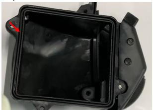
b. Replace with 2 new rubber strips (one is installed in the air inlet cover, the other is installed in the box). Take
