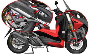
2. Check engine fastenersStandard torque of 5 M12 nuts of engine cradle:65N.m (6.6 kgf.m, 48 lbf.ft).
