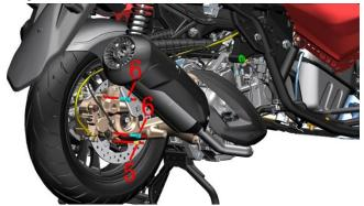
d. Insert the high-voltage package at the front of the engine back, and install one M12 nut back on the cradle to fix the engine, use 17# torx wrench to fix M12 nut (9), another person uses 15# socket to tighten bolt (8), torque: 65N.m (6.5 kgf.m, 48 lbf.ft).
