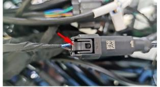
a. Locate the plug of the wheel speed sensor on the left side of the frame, and pull out the plug after pressing the anti-release card.
