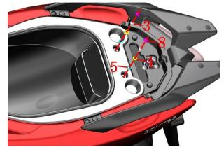
k. Grasp the tail skirt of the storage box and pull it upward obliquely, paying attention to the cables in the battery compartment. Pull up to see the left side of the glove box atmosphere lamp thread, unplug the thread and remove the glove box assembly.
