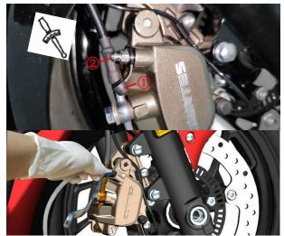
c. Put the other end of the hose into the oil pot.d. Remove the upper cover of the front brake mainpump referring to the previous step of adding brake fluid.
