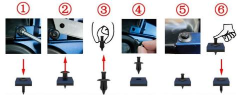
①Press the center cylinder with 4# inner hexagon or other tools, you can hear a sound or the center cylinder moves axially by 2mm (0.079 in);
