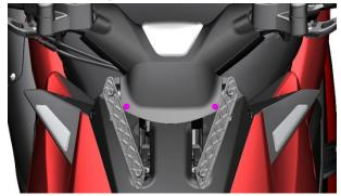
b. Hold the mark on the front sun visor (green rectangle) with your hand, pull it up in the direction of the arrow, and take out the front sun visor.
