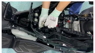
d. Remove the oil tank cover; Press the cushion bracket with one hand and take out the middle of the tank cover plate with the other hand.
