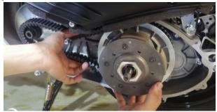
h. Pinch the sliding plate of the driving wheel and the ramp plate inside, and remove it together with the distance tube.
