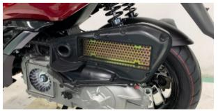
c. replace the new filter element and sealing strip. **7. Inspection air filter waste oil pipe**
