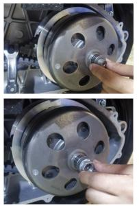
i.Same as the first step during disassembly, use a special clamp to clamp the driving wheel drive disc and the driven wheel clutch cover to prevent them from rotating freely.
