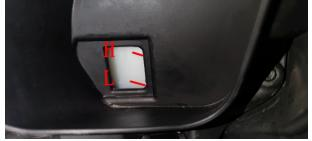
d. Reinstall the rubber plug after checking. Close the right storage box cover.
