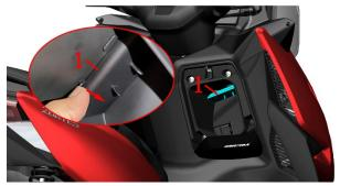
Open the protective cap ①, pull out the PKE insurance ③, first insert the DC output plug of the charger provided with the car into the PKE charging port; then connect the charger input AC terminal to 110-220V household AC.
