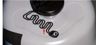
•Pay attention to protect the oil outlet of the oil pump, and only pull out the high-pressure oil pipe axially. Be careful not to pull or press the oil port radially.
