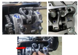
h. After replacing the four valve adjusting gaskets, check and confirm the four valve gaps again. If there is a deviation from the standard, repeat step (6) and (7) to adjust again until it meets the standard range.
