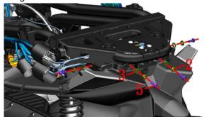
b. Find out and unplug the joint of rear license plate light, left turn signal and rectifier from the rubber cover on the left side of the frame.
