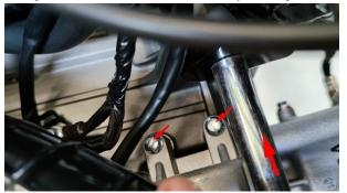
e. When reassembling, make sure not to omit the O ring that comes with the starter motor, and align the teeth of the electric starter reduction gear. Note that the O-ring needs to be correctly assembled into the box, as it will cause leakage if cut edges occur. Torque of the two bolts for fixing the starter motor:  $12\pm1.5$  N.m  $(1.2\pm0.2$  kgf.m,  $9\pm1$  lbf.ft). And mark with a marker.
