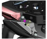
d. Find out and unplug the taillight plug (3P) from the plastic cover on the left side of the frame, hold both ends of the taillight and pull it out diagonally in the direction of the arrow to remove the taillight.
