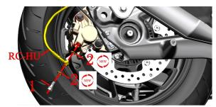
b. Use a 14# sleeve to remove the bolt (3). Standard torque of bolt (3): 24N.m (2.4kgf.m, 18 lbf.ft).
