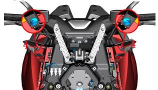
b. Grasp the marked place (green rectangle) on the Speedometer panel with one hand and lift it up in the direction of the big arrow. With the other hand, press the front storage box panel at the junction of the front storage box panel and the Speedometer panel,Until the 8 buckles(Yellow area, 4 places on the left and right) connecting front storage box panel and the Speedometer panel are separated
