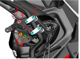
c. Use 5# inner hexagon to remove the bolts (8a) and (8b) that come with the right-hand handle under the switch, and then use the cross-batch to remove the bolts (8c), and separate the upper and lower parts of the right-hand handle.
