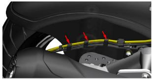
f. Pull out the wheel speed sensor from the clamp (5), remove the bolt (6) with a 4# inner hexagon, and then remove the wheel speed sensor from the car. If you need to remove the clamp (5), you can use 4# inner hexagon to remove the bolt (6) that fixes the clamp.
