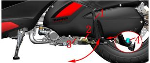
1. Main support 2. Main support spring 3. Main support return spring post 4. Cushioning glue
