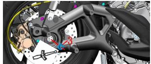
c. Use 4# hex sucket to remove the bolt (5) on the right middle of the rear inner mudguard, remove the bushing (6) and cushion rubber (7), use 4# hex socket
