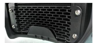
b. Pull the deformed fins straight with a flat engraving knife or a small flat-blade screwdriver. If the deformed fins exceed 20%, a new heat sink needs to be replaced.
