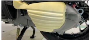
d. Clip M6×16 bolts + flanged bushing + flanged bushing cushioning glue to the inner step hole of the engine left cover, and then use a 4# inner hexagon to penetrate from the outside and hold the bolt
