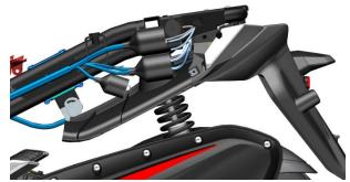
c. One person uses 14# sleeve to fix the nonstandard M10×1.5×55 bolt(11) from upper of the rear shock absorption, one person uses 14# sleeve + ratchet wrench or box wrench to remove the non-standard M10×1.5 nut(12), from the upper part of the rear shock absorption of the frame inside; nut (12) torque: 30N.m (3.1 kgf.m, 22 lbf.ft) .Remove bolts and nuts on the other side using the same method.
