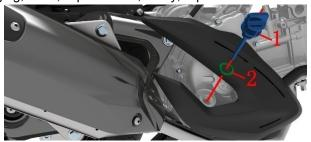
e. Wipe clean the oil dipstick, and turn the oil dipstick (1) and O-ring (2) clockwise by hand to replace the right crankcase cover of the engine.
