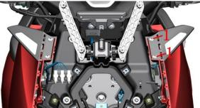
b. Use 4# inner hexagon to remove 1 expansion nail on the top of the front left turn signal; use a cross screw to remove 1 self-tapping nail<sup>(6)</sup> on the top rear of the front left turn signal.
