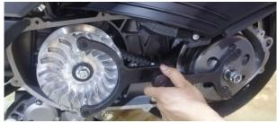
b. Use a torque wrench (or wind screw) and a 17# sleeve to remove the M12×1.25×35 hexagon flange bolts counterclockwise.
