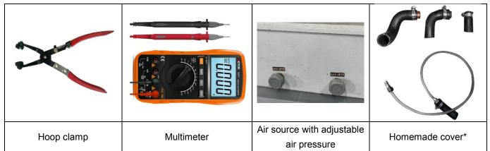
\*It can be blocked with a soft rubber plug, or folded in half with a hose and tied up with a rope or wire as a plug for the small pipe to test the sealing of the water tank filling port. You can find a water pipe with an inner diameter of 16mm to cut off a section, and use a suitable air pipe joint and clamp to assemble it firmly at the other end to test the air tightness of the water tank filling port, the main water tank, and the small water tank.
