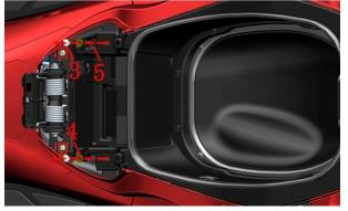
i. According to this step for National IV models, Euro V models skip directly to the next step. Use your fingers or a plastic crowbar to pry the glove box rubber strip (7) from one end and remove it. Remove the decorative
