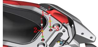
d.Lift the rear of the storage box slightly until the harness connector on the left side of the storage box is exposed, and unplug the ambient light plug (2P) on the left side of the storage box; unplug the plug and take out the whole storage box .
