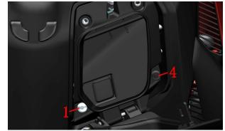
c. Grasp the upper part of the storage box with one hand, and remove the bottom bolt (1) with the 4# inner hexagon with the other hand.
