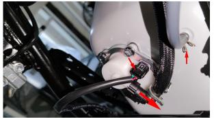
e. Use needle-nose pliers to slightly clamp the cable tie and push it up to remove it from the bracket.
