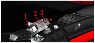
b. Pull out in sequence in the direction of the arrow (from the rear wheel to the front wheel). Note that there are 5 staples at the red circle and a circle of buckles around. Need to use a lot of force to pull out.
