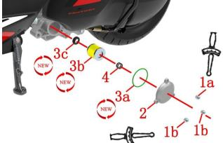
b. Use a 10# sleeve to loosen the 2 nuts (1b) at the bottom of the fine filter cover; use a 10# torx wrench to remove the upper nut (1c). Then remove the nut (1b) at the bottom.
