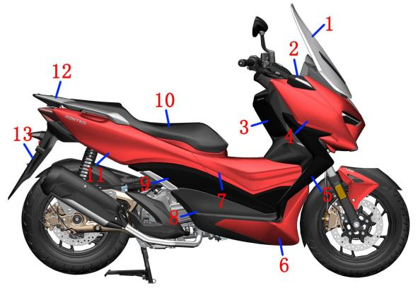
1. Windshield 2.Right front turn light 3. Right cover front storage box 4. Front right panel 5. Front storage box panel right decorative cover 6. Right pedal decorative cover 7.Right fuel tank cover plate 8. Right pedal 9. Right side cover 10. Cushion 11. Tail skirt right part 12. Rear rack 13. Rear mudguard
