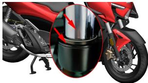
b. Check whether the bottom tube is painted off; whether the installation points of the front fender, the front wheel hollow shaft and the front brake caliper are broken or cracked. Check if there is any leakage at the bottom of the bottom cylinder.
