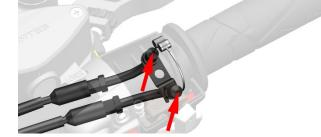
c. If the problem with high resistance cannot be solved after lubrication, the throttle cable needs to be replaced.
