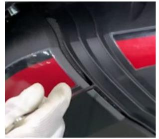
g. Use 4# inner hexagon to install the other 4 M6×16 bolts + flanged bushing + flanged bushing buffer glue. Replace the decorative buckle.
