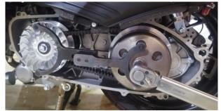
d. Remove M12×1.25×35 hexagon flange bolts and  $\varphi$ 12.3× $\varphi$ 40×4 washer. Then remove the M14×1 hexagon flange nut and  $\varphi$ 14.5× $\varphi$ 25×16 driven wheel bushing.
