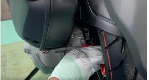
d. Pull the tail of the air filter outward with one hand, and press the rear inner mud plate inward with the other hand. Separate the air filter from the rear inner mud plate.
