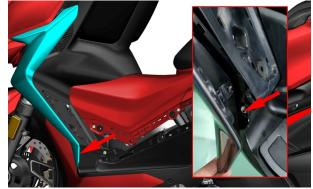
g. Use 5# inner hexagon to remove bolt (4), remove bushing (5).
