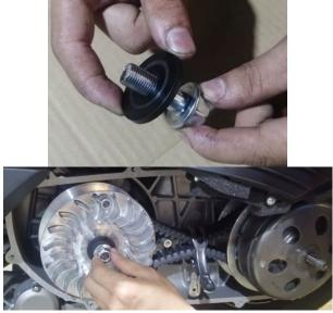
h. Point the stepped end of the  $\varphi$ 14.5× $\varphi$ 25×16 driven wheel bushing toward the driven wheel, and install it on the exposed optical axis of the drive shaft. Then screw on the M14×1 hexagon flange nut on the drive shaft thread.
