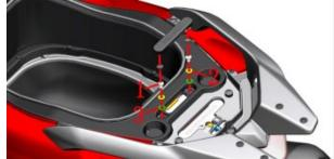
f. Lift the glove box slightly until the ambient light connector is exposed on the left side of the glove box, unplug the connector and take out the entire glove box.
