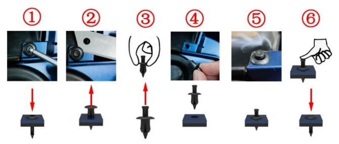
①Press down the center cylinder with 4# inner hexagon or other tools, you can hear a sound or the center cylinder moves axially by 2mm;
