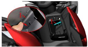
Pull out the OBD plug, connect the diagnostic tool to read the fault code
