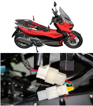
b. Check whether the plug is loose or corroded.
