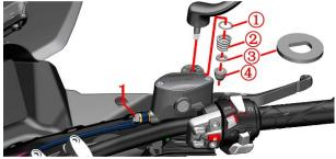
c. After grasping the front brake main pump, remove the 2 bolts (2) with a 5# inner hexagon, and remove the right auxiliary switch.
