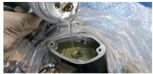
f. Observe whether the liquid level of the main pump is at 3/4 of the transparent inspection, if it is not necessary to add or withdraw or discharge with a syringe.
