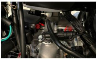
e. Locate and unplug the crankshaft position sensor
