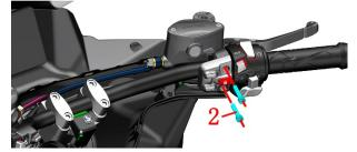
d. Tilt the front brake main pump so that the bolt (1) faces upward, wear waterproof gloves and use a 12# sleeve to remove the bolt (1), remove the copper pad (3), remove the FMC-HU oil pipe, and remove the brake fluid in the main pump. Pour out. Bolt (1) Standard torque: 32N.m (3.3kgf.m, 24 lbf.ft).
