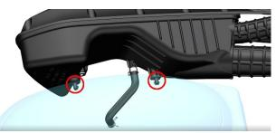
e. Use an 8# sleeve to remove the 12 M6×30 hexagonal flange bolts as shown in the figure. The two box bolts at the bottom of the air filter need to be removed to expose the air filter.
