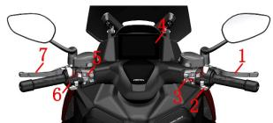
1. Front brake handle 2. Right handle switch 3. Right auxiliary switch 4. Meter 5. Left auxiliary switch 6. Left handle switch 7. Rear brake handle
