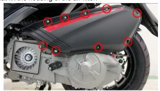
b. Remove the air filter housing.
