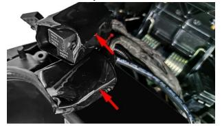
There are a total of 8 relays, the model is: KH-1A4T. g. Unplug the two wires of the starting relay. Open the red and black protective caps of the starting relay, and remove the nuts with a 10# sleeve.
