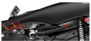
Grasp the left tail skirt and remove the expansion nail (3), and take off the left tail skirt.
