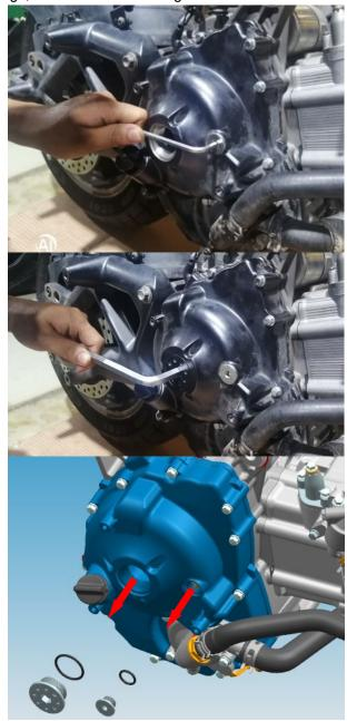
c. Insert the 14#T-shaped socket wrench from the M30×1.5 aluminum screw plug hole and set it on the hexagonal head of the flywheel bolt, and then turn the crankshaft clockwise to align the T-point engraved line on the flywheel with the mark of the M14×1.5 screw plug hole gap. At the same time, the top dead center
