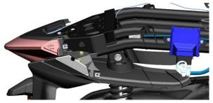
C. Use 4# inner hexagon to remove the 2 expansion nails which connected to the rear clay board with the taillight
