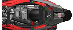
d. Remove the bolt (6) at the front of the left tail skirt with a 5# inner hexagon, and remove the bush (7) and cushion rubber (8). Remove the 2 expansion(3) nails at the bottom.
