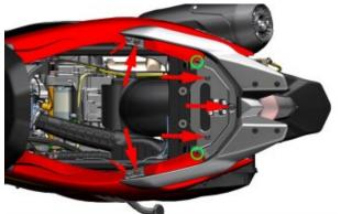
b. After putting down the right rear pedal, use a 4# inner hexagon to remove 1 M6×16 bolt (1) on the pedal, remove the bushing (2), cushion rubber (3), then grasp the end of the side cover with your hand, and press the arrow Pull out in the direction (from back to front) until the 5 mushrooms (in the green circle) on the side cover are pulled out, and then take out the side cover.
