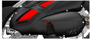
b. Use 4# inner hexagon to remove the 4 M6×16 bolts
