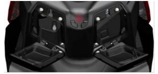
b. Use 4# inner hexagon to remove 6 M6×16 bolts (1), among which 4 M6×16 bolts above the storage box are covered with bushings (2), cushion rubber (3); then use 4# inner hexagon or other tools to remove The two expansion nails on the lower storage box (4), take out the left and right storage boxes, the left storage box has a line connection, do not pull it vigorously, just place the foot pedal.
