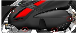
c. Pull out the front part of the left engine cover first and then move it about 30mm (1.2 in) in the direction of the rear mudguard to remove it. The bolts removed in the second step will fall off at this time. If the shock-proof sponge shown in the picture has been dropped, proceed to the next step, otherwise you must remove it first.
