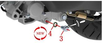
e. Wipe clean the joint surface with a non-woven fabric. Inspect the oil drain bolt (1) whether the joint surface is scratched; if there is any, replace it with a new one, if not, wipe it clean.
