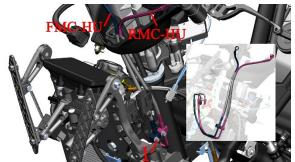
FC-HU and wheel speed sensor (front wheel)
