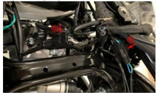
f. Locate and pull out the plug of the magneto stator charging cable  $\ensuremath{\overline{\mathcal{O}}}$  at the left frame.
