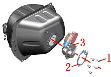
When re-assembling, you need to pre-tighten the corners and then tighten the 5 bolts. Otherwise, the uneven compression of the sealing rubber ring of the fuel pump will easily cause leakage and cause safety hazards.
