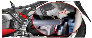
d. Loosen the bolt of the clamp (4) with a 4# inner hexagon and pull out the air filter outlet pipe (5) and clamp (6) in the direction of the arrow to pull out the throttle valve body.
