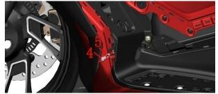
h. Use 5# inner hexagon to remove 4 bolts (4)Remove the bushing (2) and the cushion rubber (3).
