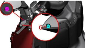
c. Take out the front left turn signal with one hand, and unplug the 2 bullet joints of the front left turn signal with the other hand.
