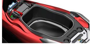
c. Tighten the two M6×16 bolts (1) at the front of the storage box with 4# inner hex. Note that the bolts must be equipped with bushings (2) and cushion rubber (3); then connect the middle cover of the fuel tank to the storage box (green mark) Place) Use 2 expansion nails to fix; tighten the 2 M6×16 bolts at the rear of the storage box (1) with 4# inner hexagon. Note that the bolts need to be equipped with bushings (2), cushioning glue (3), and finally buckle with decorative glue.
