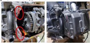
k. Put the 13×2.8 O-ring on the M14×1.5 screw plug, screw it into the corresponding screw hole of the right crankcase cover, and tighten it with a 5# Allen key. The torque value is  $10\pm2N.m(1\pm0.2 \text{ kgf.m}, 7.4\pm1.5 \text{ lbf.ft})$ ; After putting the 27.4×2.65 O-ring on the M30×1.5 aluminum screw plug, screw it into the corresponding screw hole of the right crankcase cover, tighten it with a 10# Allen key, the torque value is  $16\pm2N.m$  ( $1.6\pm0.2$ kgf.m,  $12\pm1.5$  lbf.ft).
