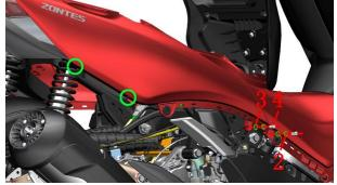
c. Put back the 2 expansion nails (green mark) on the inner and tail of the right tail skirt. Finally, check again to check whether the assembly gap between the right tail skirt and the surrounding parts is too large or interference, if the assembly gap is too large or interference, re-assembly is required.
