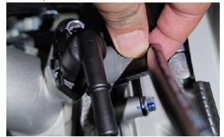
If you need to replace the fuel injector, wait until the engine and muffler have cooled down. After placing the oil container at the bottom, refer to the steps for removing the high-pressure oil pipe to pull out the high-pressure oil pipe at the end of the fuel pump to discharge the remaining fuel. Use a 10# sleeve to remove the bolt (1), remove the injector holder (2), and then take off the injector (3).
