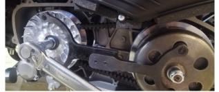
c. Loosen the M14×1 hexagonal flange nut counterclockwise with a torque wrench (or wind screw) and a 19# sleeve.
