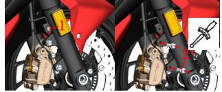
e. Pull out the front brake caliper assembly and check the wear of the brake pads. If worn or nearly worn to the limit position, new brake pads must be replaced in pairs.
