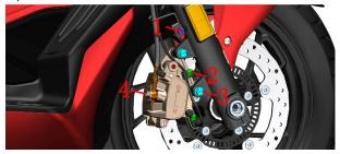
b. After wearing waterproof gloves, loosen the bolt (4) with a 12# sleeve, and turn the caliper upside down so that the head of the bolt (4) is facing down to drain the brake fluid into the oil pan. Remove the bolt (4) and the copper pad (5) and then remove the FC-HU oil pipe. Refer to the brake fluid steps to remove the upper cover of the front disc brake main pump to speed up the discharge of brake fluid.
