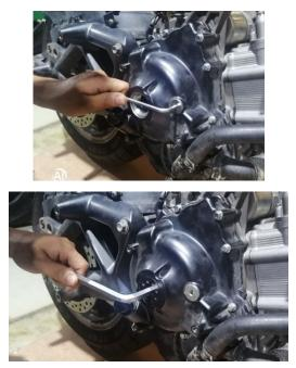
I. So far, the adjustment operation of the valve clearance is completed.
