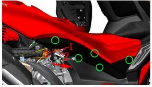
c. Use 5# inner hexagon to remove the 2 nonstandard M6×16 bolts (4) on the tail skirt, remove the bushing (2), cushion rubber (3), and then use 4# inner hexagon to remove the 2 expansion nails under the tail skirt (green circle Logo).
