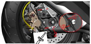
g. Pull out the rear canper assembly and check the wear of the brake pads. If it is nearly worn or worn to the limit position, new brake pads must be replaced in pairs.
