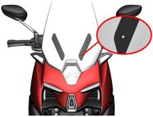
c. Take out the left and right decorative covers of the windshield, the windshield, and the rubber pads of the windshield bracket in turn.
