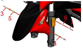
d.First press the two sides of the front mud board according to the small arrow, press the protrusion on the front mud board arrow inward, and then move the front mud board up to a suitable position and then pull it out in the direction of the big arrow.
