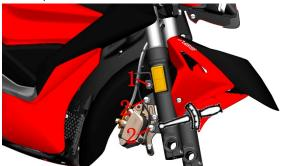
c.Use 4# inner hexagon to remove the two M6×12 bolts on the left and right sides of the front fender (3), remove the 2 bushings (4), cushion rubber (5); then use 5# inner hexagon to remove one M6×30 bolt (1), take out the gasket (6).
