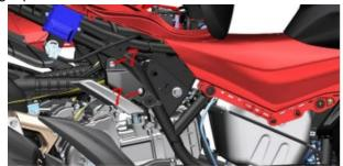
b. One person uses a 17# torx wrench to insert a M12 nut <sup>(9)</sup> that fixes the engine on the left side of the vehicle from the front of the air filter, and another person uses a 15# sleeve to remove a M12×1.25×290 bolt that fixes the engine on the right side of the vehicle <sup>(8)</sup>, pull out the bolt from the frame.
