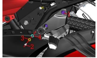
d. Check whether the engine nut (5) is loose.
