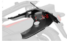
d. Pull down the rectifier and pull the cable out of the hole in the front of the rear mud board. Remove the rectifier from the car. When pulling out the cable, be careful not to pull it forcibly to avoid damaging the plug or pulling off the wire.
