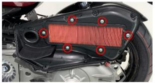
b. Remove the old air filter element. Blow the dust inside the air inlet pipe with a dust blower, and then wipe the inner wall with a clean non-woven cloth.
