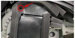
b. Use 4# inner hexagon to remove the 3 M6×16 bolts
