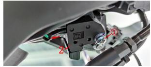
3. Lubricate the movable parts of the brake handle 3.1 Lubricate the front brake handle.
