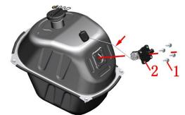
When reassembling, you need to pre-tighten the corners and then tighten the 4 bolts. Otherwise, the uneven compression of the sealing rubber ring of the oil level sensor may cause leakage and cause safety hazards.
