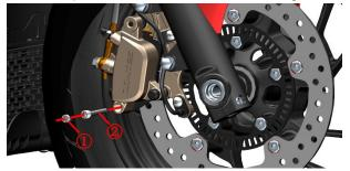
b. Remove the brake pads.
