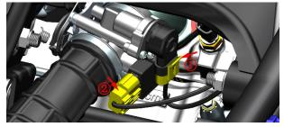
m. Use a short Phillips screwdriver to remove the 2 bolts 1 and the anti-off card 2 that come with the
