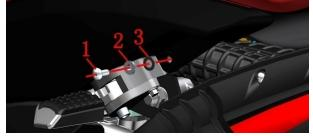
b. Pull out in sequence in the direction of the arrow (from the rear wheel to the front wheel). Note that there are 5 staples at the red circle and a circle of buckles around. It takes a lot of force to pull out.
