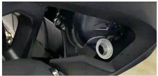
d.inspection O ring (2)Whether there is damage or aging, if not, wipe it clean, if any, replace it.
