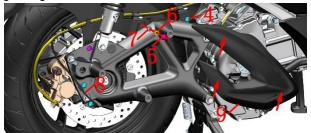
d. In the gap between the left air filter and the rear inner mud board, hold the air filter housing with one hand, and press the rear inner mud board at the position 2 indicated by the arrows with the other hand. Separate the rear inner mud plate from the staples on the air filter and lift it up to facilitate subsequent removal of the rear rocker arm.
