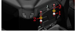
b. Remove the expansion nail (4). For instructions on disassembly and assembly of expansion nails, please refer to the pre-service instructions in this chapter.
