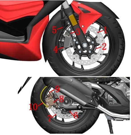
1-Brake disc (front) 2-ABS induction ring gear (55 teeth) 3-wheel speed sensor (front wheel) 4-front disc brake caliper 5-FC-HU brake hose 6-ABS induction ring gear (54 Teeth) 7-brake disc (rear) 8-rear disc brake caliper 9-wheel speed sensor (rear wheel) 10-RC-HU brake hose
