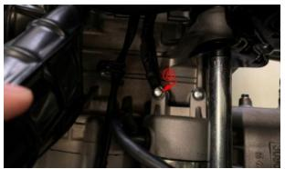
h. Use an 8# sleeve to remove a bolt on the starter motor, and take out the negative wire (8) on the bolt. **Caution:** The negative wire of the early production model is fixed on the bolt around the starter motor.
