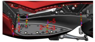
c. Remove the two M6x16 bolts(1) of the left pedal decorative cover with 4# inner hexagon and take out the bushing (2)and buffer glue(3).
