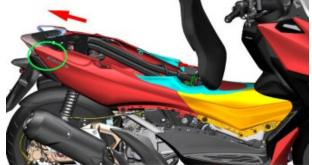
f. Refer to steps a-j in the steps of "Removing the spark plug" to remove the left and right pedals and the left and right trim cover components.
