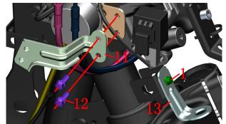
k. After loosening the hoop with hoop pliers, disassemble the radiator assembly. The distribution diagram of each hoop is shown in the figure below.
