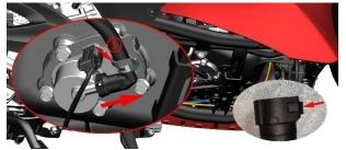
g. Pull out the high-pressure oil pipe from the bracket at the cylinder head.
