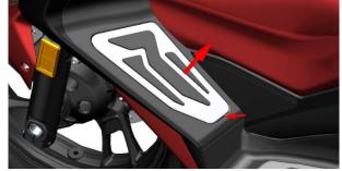
c. Use 4# inner hexagon to remove the two M6×12 bolts<sup>(4)</sup> connecting the left decorative cover of the front storage box panel on the front storage box panel.
