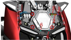
b. Hold the headlight with one hand and take it out for a certain distance, pull out the 3P plug (green and white wire) behind the headlight with the other hand, and take out the headlight completely.
