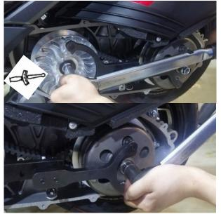
k. At this point, the assembly of the stepless variable speed sub-assembly is completed.
