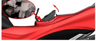
d. Open the black negative protection cap of the main wiring harness, use a cross-battery or 10# sleeve to remove the battery's own bolts and move the negative line away from the battery; then open the red positive protection cap and remove the positive bolts. Remove the positive wire. Remove the battery upwards. Folding rear storage box:
