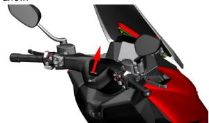
b. Use a cross screw to remove the two self-tapping screws (1) at the lower cover, and use a straight screw to pry off the buckles at (1) and (2).
