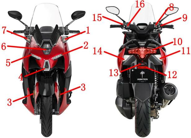
1-Left front turn signal 2-Left daytime running light 3-Side reflector 4-Position light 5-Right daytime running light 6-Headlight 7-Right front turn signal 8-Right-hand handle auxiliary switch 9-Right-hand handle switch 10-Rear tail light/system Moving lamp 11-Rear right turn signal 12-Rear reflector 13-License plate lamp 14-Left rear turn signal 15-Left handle switch 16-Left handle assistant switch
