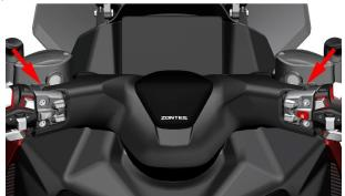
b. Park the vehicle on a flat ground or a lifting platform, and lower the main support. Check whether there is brake fluid leakage at the oil pipe joints of the main pump, ABS hydraulic control unit and caliper. The endoscope with LED can be used to check the oil pipe joints of the ABS hydraulic control unit and the main pump, or to remove the corresponding cover for inspection.
