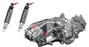
d. Check whether the weld at the bottom of the shock absorber is leaking.
