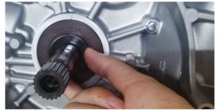
b. Then check whether the 8 Puli beads are completely placed in the Puli groove of the driving wheel sliding disk (Figure 1 below), and then assemble the slope plate with the four guide blocks corresponding to the position of the driving wheel sliding disk guide post on the driving wheel. The wheel slides on the disc (picture 3 below).
