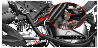
c. Press the buckle indicated by the arrow to pull out
