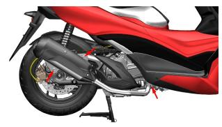
a. If there is a slight air leak, first try to tighten the exhaust port nut with 6# inner hexagon; if the problem is not solved, remove the muffler and replace with a new engine exhaust port gasket.
