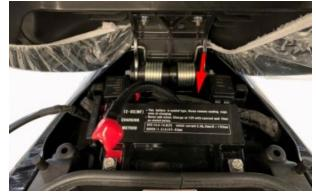
e. Remove the decorative glue at the back of the storage box, and then take out the decorative buckle on the bolts, use 4# inner hexagon to remove the 2 M6×16 bolts that fix the storage box (1), take out the bushing (2), cushion rubber (3).
