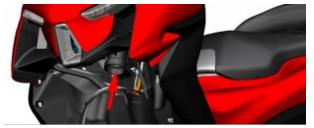
b. Put the greased bearing (9), shaft ring (10), and dust cap (11) on the upper link plate in turn, and then screw in a steering column adjusting nut (12), and tighten the steering column adjusting nut (12) with a four-jaw socket. Torque: 35N.m(3.6 kgf.m,26 lbf.ft), make sure that the upper link plate does not move up and down, loosen the direction column adjusting nut (12) counterclockwise by 1/4 turn, and finally tighten it with a torque wrench. Torque: 15N.m (1.2 kgf.m, 11 lbf.ft).
