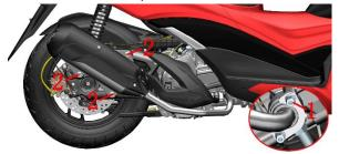
b. One person pinches the rear brake handle, and one person uses 21# sleeve + impact wrench to remove the rear wheel nut (3). Standard torque of nut (3): 125N.m (12.8 kgf.m, 92 lbf.ft).
