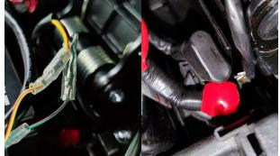
h. Straighten out the cables in the battery compartment. For the National IV model, remove the bolts on both sides (3) with 4# inner hexagon according to Figure 1, and remove the bushing (4) and cushion rubber (5). For Euro V models, remove the bolts on both sides (3) with a 4# inner hexagon according to Figure 2.
