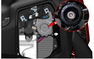
c. Use a 10# sleeve to loosen the thermostat bleed bolt (5) counterclockwise by 4 to 5 turns, do not completely remove it. Note that a small container is required to receive the coolant overflowing from the exhaust bolt. Do not allow the coolant to drip directly onto the surface of the part.
