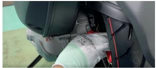
d. Pull the tail of the air filter outward with one hand, and press the rear inner mud plate inward with the other hand. Separate the air filter from the rear inner mud plate.
