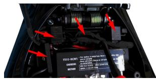
f. Pull out the two relay wires
