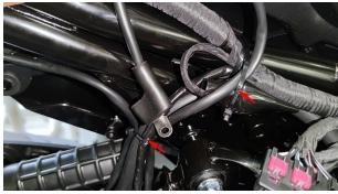
c. Loosen the clamp bolt shown in the figure with a 4# inner hexagon counterclockwise, and pull the air filter outlet pipe toward the rear wheel to pull out the throttle valve body.
