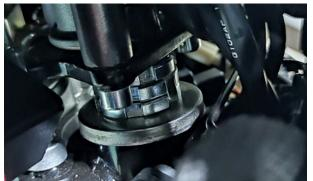
b. For the convenience of explanation, other parts are hidden here. First use a 38-42 hook wrench with a thickness of 6mm (0.24 in) to loosen the adjusting nut (1a); move the lock washer <sup>(2)</sup> up and then loosen the adjusting nut (1b).
