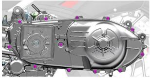
f. Remove the left crankcase cover (2) and the left crankcase cover gasket (4). The left crankcase cover gasket (4) must be replaced when reinstalling, and the hollow positioning pin (3) must not be omitted.
