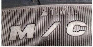
b. The height of the wear mark on the tread protrusion is 1.6mm (0.06 in). The triangle ( $\Delta$ T.W.I.) mark on the sidewall indicates the location of the wear bar. If the wear reaches the mark point, it means that it has been worn to the limit. If you continue to drive, there will be a safety hazard. You must replace with new tires of the same specification.
