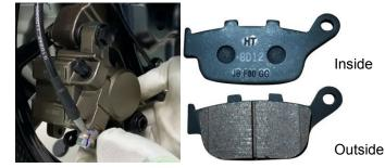
e. After adjusting the position of the brake pad, reinstall the bolt ③ and lock it with a 12# sleeve. Standard torque: 24N.m (2.4 kgf.m, 18 lbf.ft).
