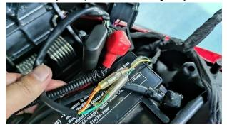
b. Unlock the vehicle, turn the engine shutoff switch to "O", retract the side bracket, pinch the brake handle and press the start button. You should hear the sound of the start relay picking up, otherwise you should check the start circuit.
