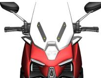
b. Use 4# inner hexagon to loosen the 4 M6×16 bolts on the left and right decorative covers of the windshield.
