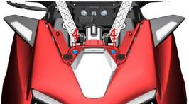
b. Grasp the mark on the front front cover (green box) with your hands, and pull out according to the arrow until the mushroom head (blue circle) on the right side of the front front cover is pulled out; use the same method to remove it The mushroom head on the left side of the front front cover.
