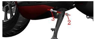
e. Remove the side bracket bushing (4) from the frame.
