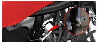
h. Pull out the high-pressure oil pipe in the direction of the arrow after pressing down the anti-dropping lock. Note that there are high-pressure fuel pipe brackets and cable ties at the intake manifold of vehicles produced after March 2021. The vehicles produced before are only lashed with cable ties.
