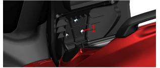
b. Use 4# inner hexagon to press down 4 expansion nails (2) center cylindrical pins, and then a total of 4 expansion nails on the left and right sides (2).
