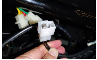
d. After unplugging the yellow 3P plug, measure the red positive wire and green negative wire with a multimeter, and the battery voltage should be measured. Use the buzzer file of the multimeter to check whether the green negative wire and the ground wire (the ground wire can be found in any stud directly connected to the frame) are always conducting.
