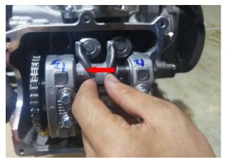
g. The adjusting shim is small and easy to fall into the engine when it is taken out. The original adjusting shim can be sucked out with a magnet rod. Then use tweezers to put in the adjustment shim to be replaced. After replacing the two adjusting shims on the same side, push the valve rocker back to the side of the spark plug to press the valve adjusting shims to prevent them from sliding out. Then replace the valve clearance adjustment gasket on the other side in the same way.
