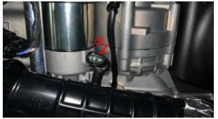
i. Locate and unplug the plug of the cylinder head water temperature sensor (10) on the right side of the throttle valve body.
