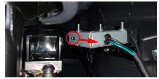
c. Remove 3 M6x16 bolts<sup>(1)</sup> on the front left storage box with a 4# inner hexagon , remove the bushing and buffer glue;**Caution:** only the upper 2 bolts have bushing + buffer glue, and the bottom 1 bolt does not have bushing<sup>(2)</sup> + buffer glue<sup>(3)</sup>.Remove the 1 nail securing the front left storage box with a 4# inner hexagon.
