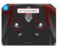
1 工具:6号内六角扳手 Tool:6# Hexagon wrench 取下车辆后尾下的2个螺栓,如图 a所示;取下小靠背上的2个螺栓。 Remove two bolts under the rear cover as shown in Picture a;remove two bolts of the seat back.
