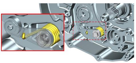
•Use 10#T rod sleeve to remove bolt (1), remove stopper (2), washer (3), torsion spring (4).
