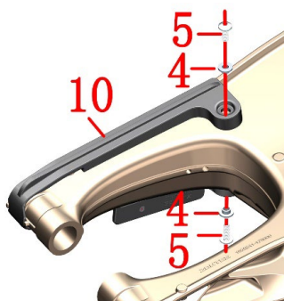
Old rear fork anti-bearing block
