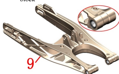
Old rear fork anti-bearing block
